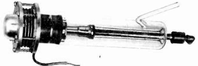
Fig. 7—Photograph of experimental tube with domed window permitting 180-degree solid-angle X-ray beam.
