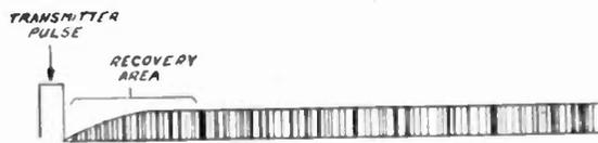
Fig. 15—Receiver-recovery characteristics, class-A oscilloscope pattern.
