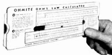
The new calculator provides a simple and handy means of solving resistance calculations. With one setting of the slide it gives the answer to any Ohm's Law problem. It will also solve parallel-resistance and series-capacitance problems, and will multiply, divide, and find squares and square roots. On the reverse side is printed the Resistor Color Code.
