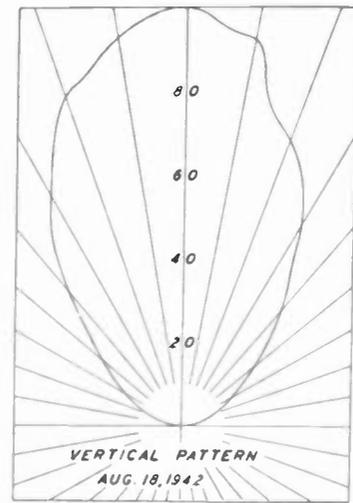
Fig. 6—Slot-lengthwise pattern of antenna of Fig. 4. Data by U. S. Navy.
