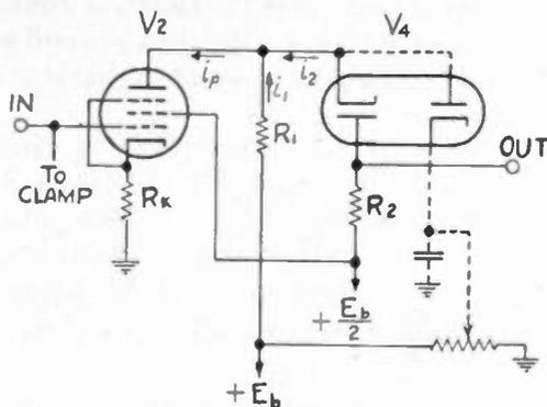
Fig. 20—Schematic diagram of linear clipper.
