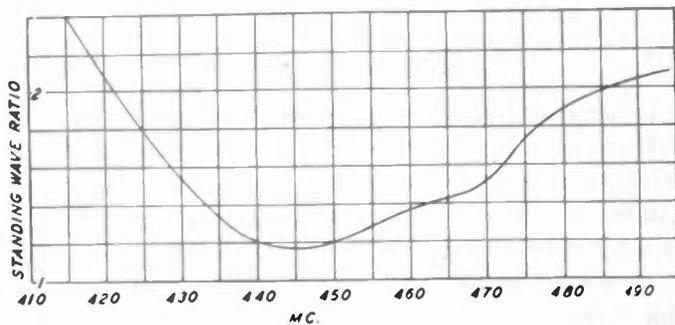
Fig. 16—Standing-wave-ratio curve of the antenna of Fig. 15.
