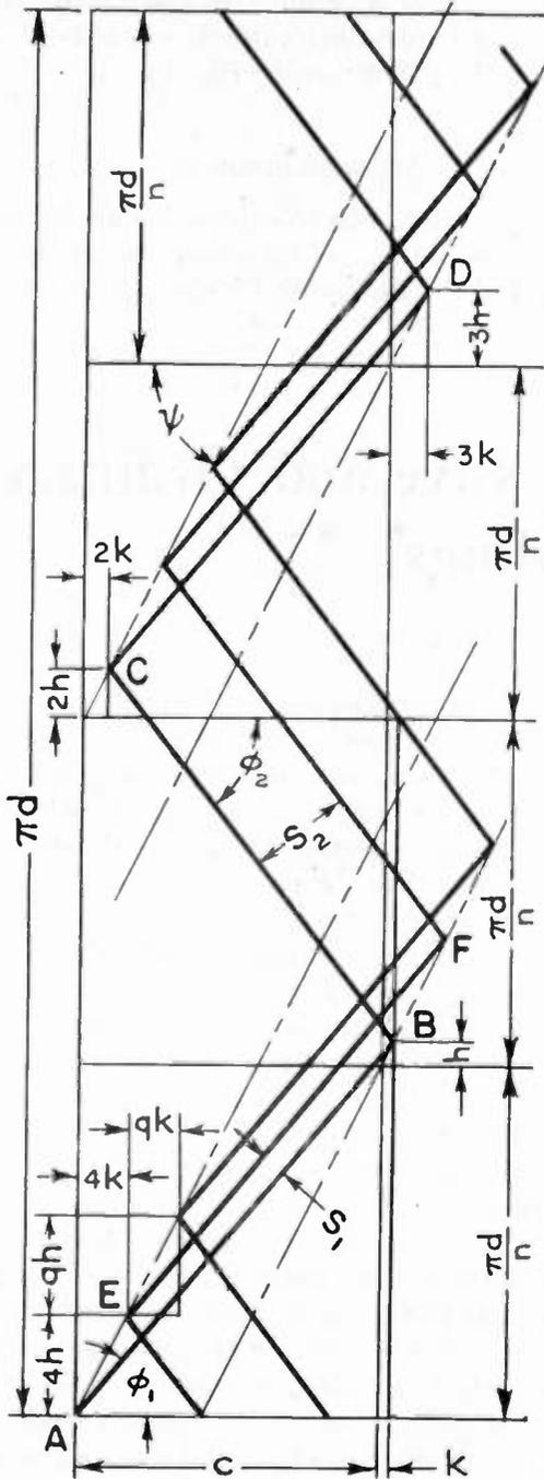
Fig. 1—Developed plane diagram of a progressive universal coil with progressive layering.
