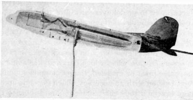
Fig. 7—One-half of a model with antenna and receiver in position. A fiber rod for adjusting the receiver tuning projects from the tail.
