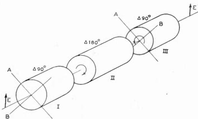
Fig. 3—Adjustable phase changer.
