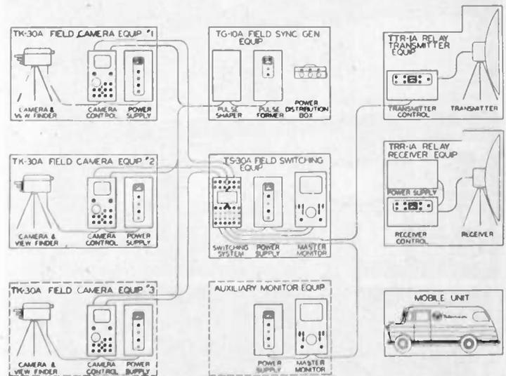
Fig. 1—Block diagram of field-pickup equipment.
