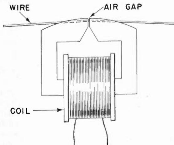
Fig. 1—Schematic illustration of a conventional magnetic-wire recording-reproducing head.
