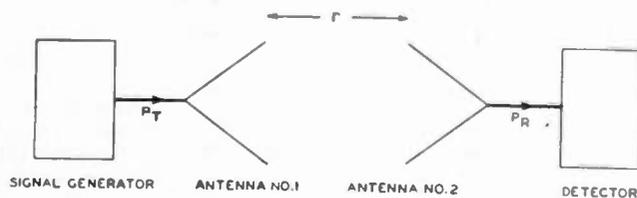
Fig. 2—Gain measurement by the transmission method.
