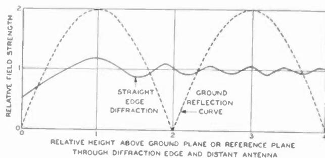
Fig. 14—Function of field strength versus height for antenna-testing site.
