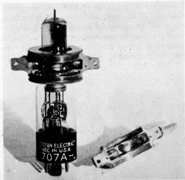
Fig. 2.—W.E. 707A tube with typical resonator. A part of the resonator is shown attached. The other portion, containing the output coupling, is also shown. Frequency adjustment, exclusive of that produced by variations of the repeller voltage, is made by plugs screwed into the cavity.
