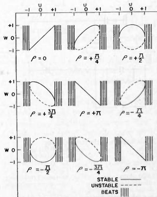
Fig. 2—Forms of the  $U$ - $W$  curve in the region of synchronization.
