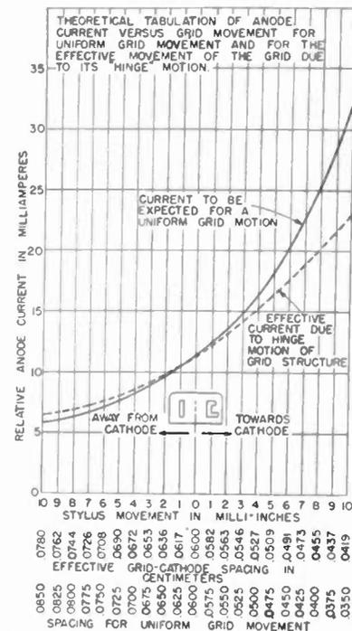
Fig. 3—The theoretical computation approximates practice for changes in anode current due to grid position. The variations from these computations where the grid draws current and the anode voltage is reduced are responsible for the increasing linearity of operation, as indicated by the curves of Fig. 10(a), (b), and (c).
