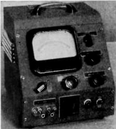
The manufacturer claims that this instrument cannot be damaged by any degree of overload. Five sensitivity ranges, of from 0.01 microamperes full-scale to 100 microamperes full-scale, are provided, with 40 millivolts full-scale input on all ranges. This unit may also be used as a null-detecting galvanometer, with a sensitivity of approximately 100 millivolts full-scale, or 0.0005 microamperes per division.
