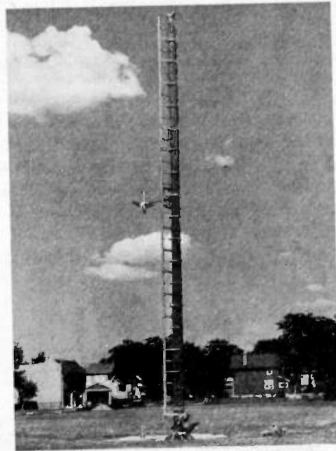
Fig. 2—The vertical pole used to support models for measurements of antenna patterns at low frequencies.
