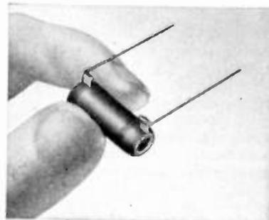
Although this small unit has been available on special order, the 5-watt size (1/8 by 1 inch) may now be obtained from regular stock in resistance values from 1 to 10,000 ohms. Standard tolerance is ±10 per cent. The new 5-watt resistors are of all-welded construction and have 1 1/2-inch copper-wire leads. Write to the manufacturer for Bulletin 132.
