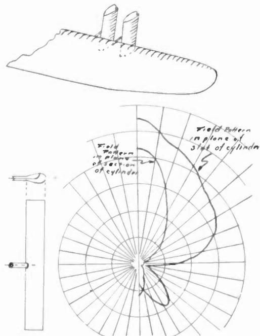
Fig. 1—Open-ended and streamlined, slotted cylinder antennas mounted in front of leading edge of airplane wing. Polarization perpendicular to cylinders. Polar radiation diagrams for one antenna element are included.
