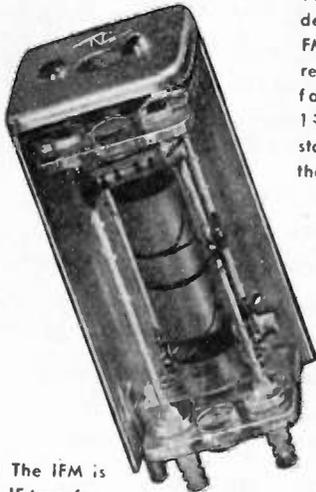
● The IFM is an IF transformer with a 150 KC bandwidth at 1.5 db attenuation. Approximate stage gain of 30 is obtained when used with 6SG7 tube.
