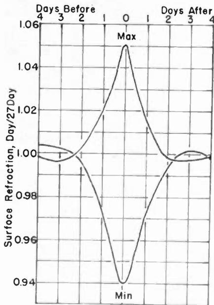
Fig. 6—Change of atmospheric surface refraction grouped around epochs of maximum and minimum fields.
