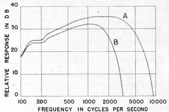
Fig. 8—Comparison of frequency-response curves for (A) an abrupt change in the field, and (B) a gradual change in the field as the medium leaves the recording head.
