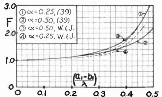
Fig. 2—Frequency-correction factor from equation (39).
