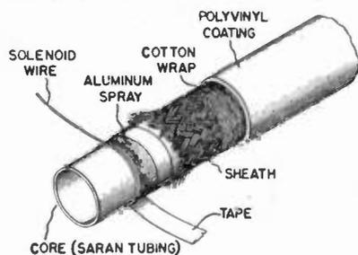
Fig. 1—Details of construction of continuous delay line.
