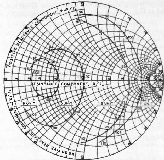
Fig. 6—Measured variation of normalized impedance with frequency across the terminals of the lowest radiating unit for one, two, five, and eight radiating-unit cloverleaf antennas when unit separation is optimum for 98 Mc.
