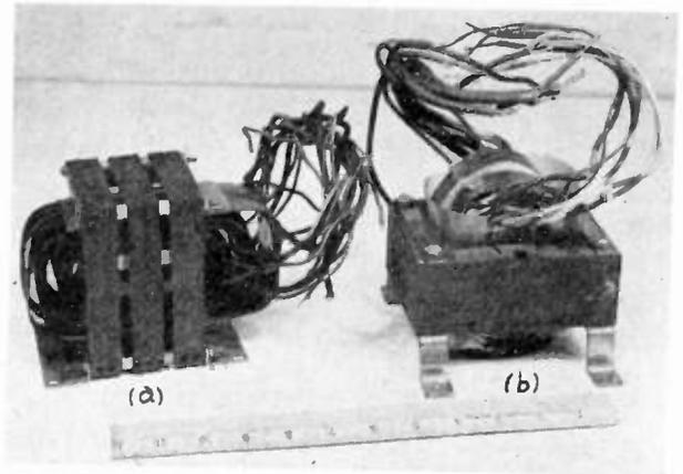
Fig. 12—(a) Prewar design of a forced-air-cooled power transformer. (b) New design.
