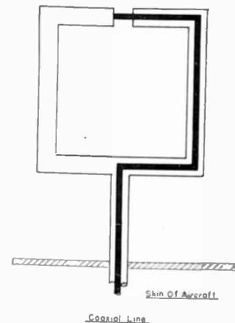
Fig. 8—Method of connecting a balanced loop antenna to a coaxial line.
