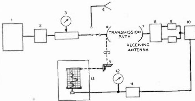
Fig. 16—Complete system for gain-pattern and cross-polarization measurement.
