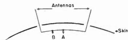
Fig. 9—Method of feeding simple two-element antenna arrays. Feed connection is at *A* for antenna currents in phase, and at *B* for phase opposition.
