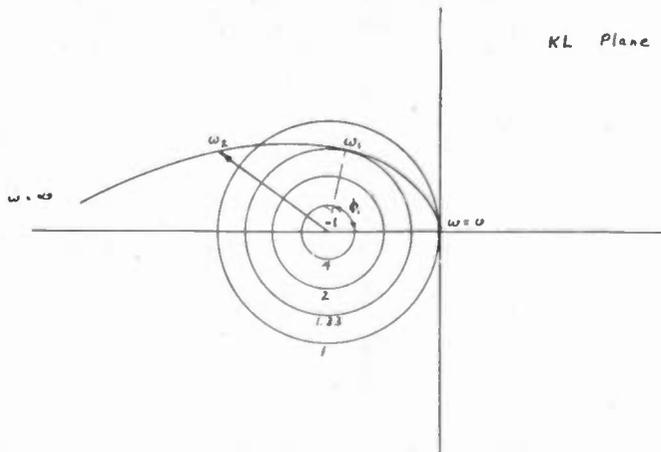
Fig. 3— $kL$  plane, showing typical  $kL$  contour and damping-ratio circles.
