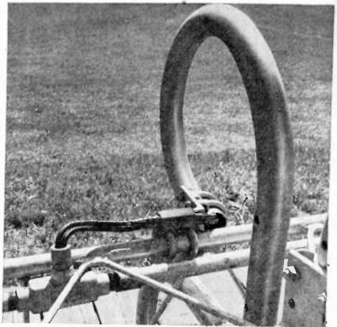
Fig. 13—Single radiating element of a cloverleaf antenna, showing a Calrod heater element for sleet removal.
