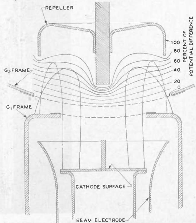
Fig. 8—Typical electrostatic field plot for the repeller space, showing calculated electron paths.
