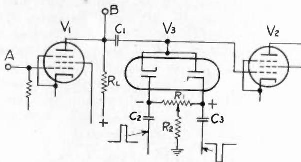
Fig. 17—Schematic diagram of clamp circuit.
