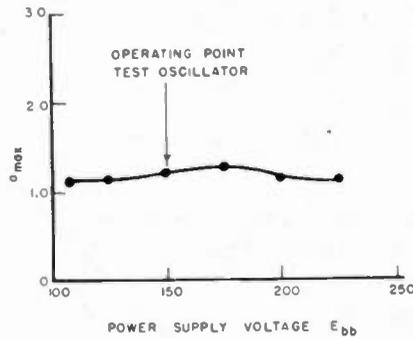
Fig. 9— $a_{\max}$  as a function of test oscillator  $E_{bb}$  for fixed injected voltage.
