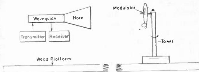
Fig. 5—Diagram of equipment for a new method of measuring antenna patterns.
