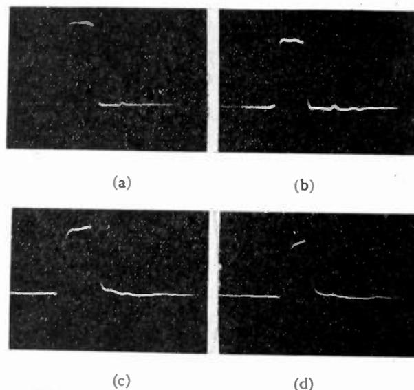
Fig. 2—Effect of delay on a 1-microsecond pulse. (a) 1-microsecond pulse generated by discharge of a double-layer delay line. (b) 1-microsecond pulse delayed 1 microsecond in a single-layer line. (c) 1-microsecond pulse delayed 3 microseconds. (d) 1-microsecond pulse delayed 5 microseconds.
