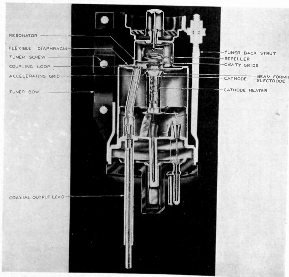
Fig. 9—Structural details of the 2K25 beating oscillator designed to cover a frequency range from 8500 to 9660 Mc. The output coaxial line of this tube is designed to be coupled directly into a wave guide.
