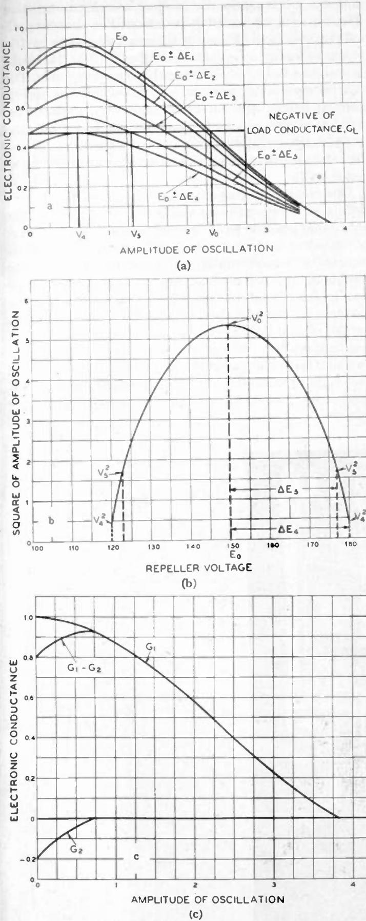
Fig. 7—Type of electronic-conductance and power-output characteristics which may occur where hysteresis is present. (a) Electronic conductance as a function of amplitude of oscillation for various values of repeller voltage. (b) Resulting power output versus repeller voltage curve. (c) Effect of an out-of-phase source of conductance on the total electronic conductance.
