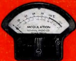
Percentage Modulation meter, calibrated from 0 to 133 per cent. Additional db scale. Switch selects positive or negative peaks or full-wave indication. For FM, 100% modulation corresponds to 75 kc deviation; for television, internal adjustment changes calibration to 100% at 25 kc deviation.
