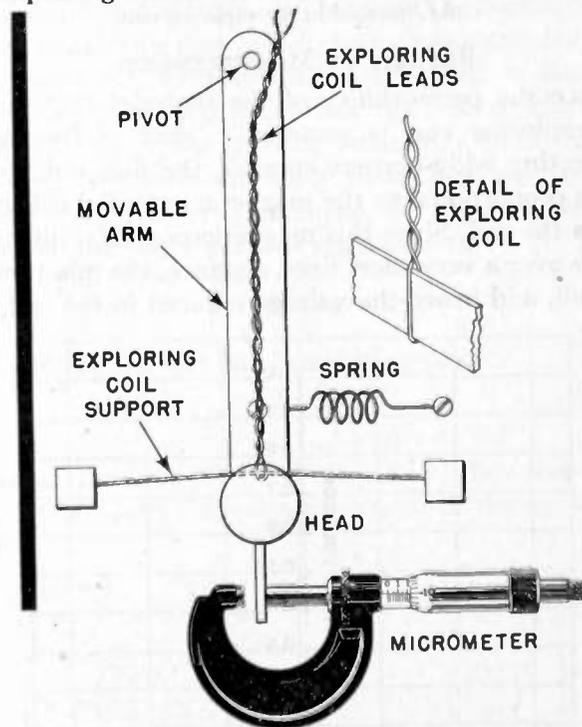
Fig. 2—Mechanical arrangement for positioning the head with respect to the exploring coil.
