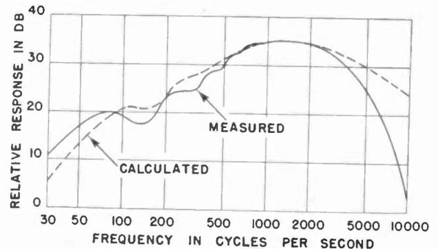
Fig. 6—Frequency-response curve calculated from field-distribution data compared with measured frequency-response curve.
