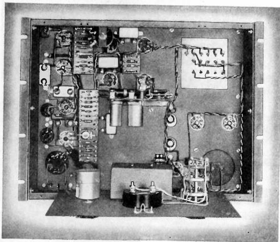
1 Selector switch and meter provide both output level indicator (not for "riding gain") and plate current readings for all tubes.
