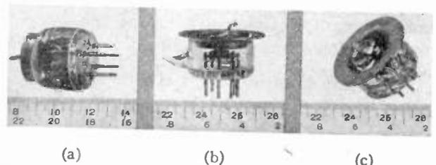
Fig. 4—(a) Early phonotube model. (b) and (c) Two views of the experimental model discussed in the text.
