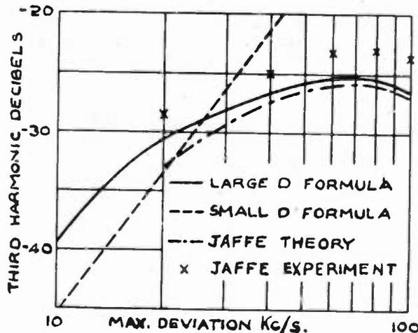
Fig. 1—Third-harmonic distortion in a single resonant circuit.
