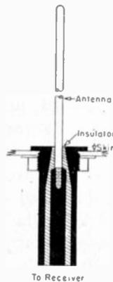
Fig. 6—A cross section of a typical model antenna.
