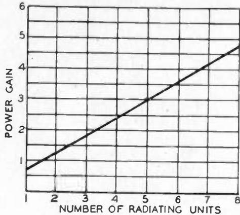
Fig. 8—Computed free-space-antenna power gain, referred to a dipole, versus number of radiating units of a cloverleaf antenna.
