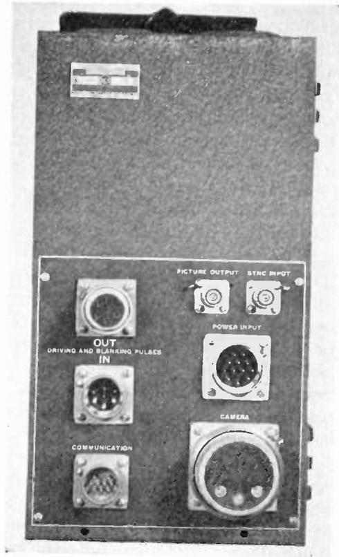
Fig. 11—Rear of the camera control.
