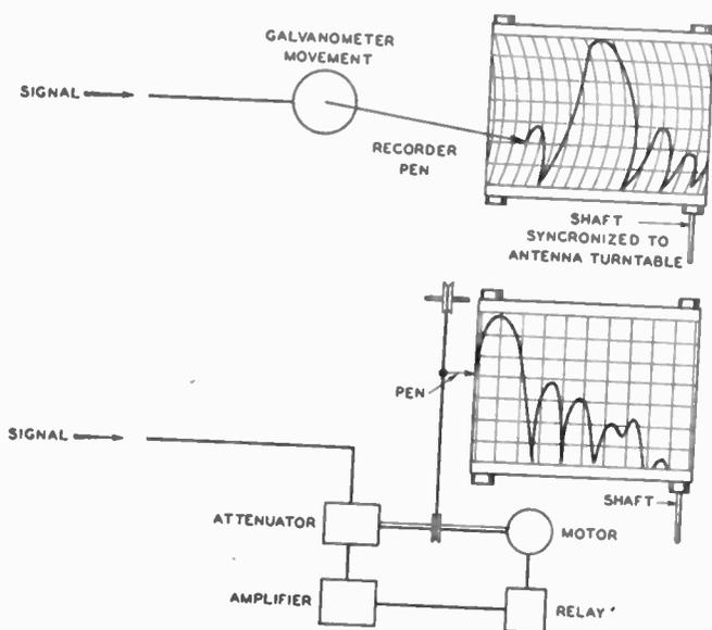
Fig. 6—Automatic pattern-recorder systems.
