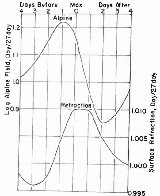
Fig. 7—Upper curve: W2XMN field intensities around epochs of greatest refraction. Lower curve: atmospheric surface refraction around epochs of maximum fields of W2XMN.
