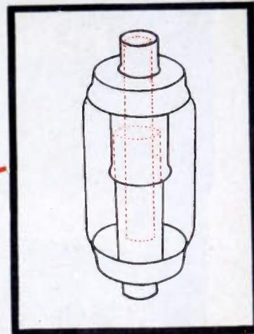
Jonah pulled a good trick when he got a round trip ticket into the whale . . . and we think we pulled a good one when we found a way of putting a heater inside our vacuum condensers to increase efficiency of our out-gassing.
