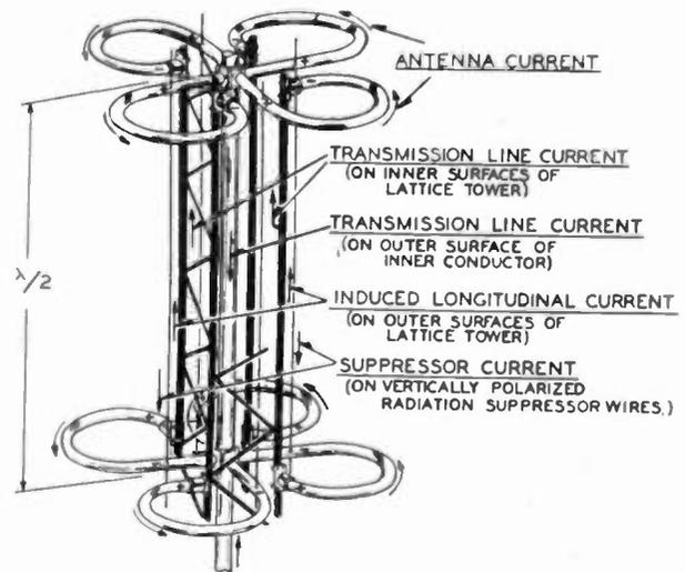
Fig. 10—Instantaneous current relations in two adjacent radiating units and in interconnecting transmission lines of a cloverleaf antenna.
