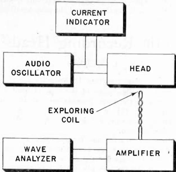
Fig. 3—Block diagram of the electrical setup for measuring e.m.f. induced in the exploring coil.
