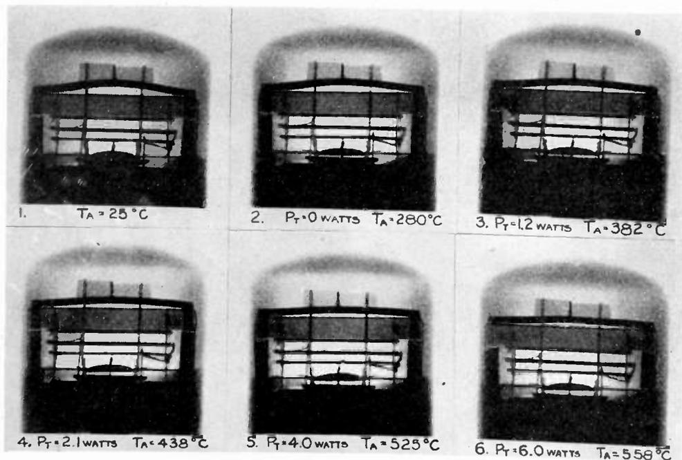
Fig. 14—X-ray views of an operating 2K45 tube, demonstrating the movement of the thermal-tuning mechanism for various input powers.
