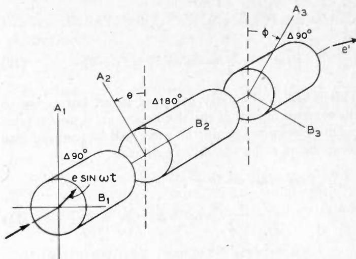
Fig. 12—Generalized phase changer.
