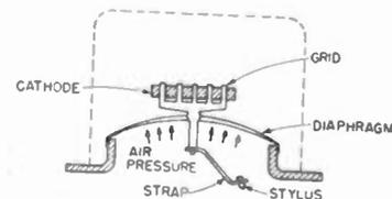
Fig. 5— Because of the forked structure and the vertically stiff diaphragm, plus the vertically compliant stylus strap, very little vertical motion actually reaches the grid structure.
