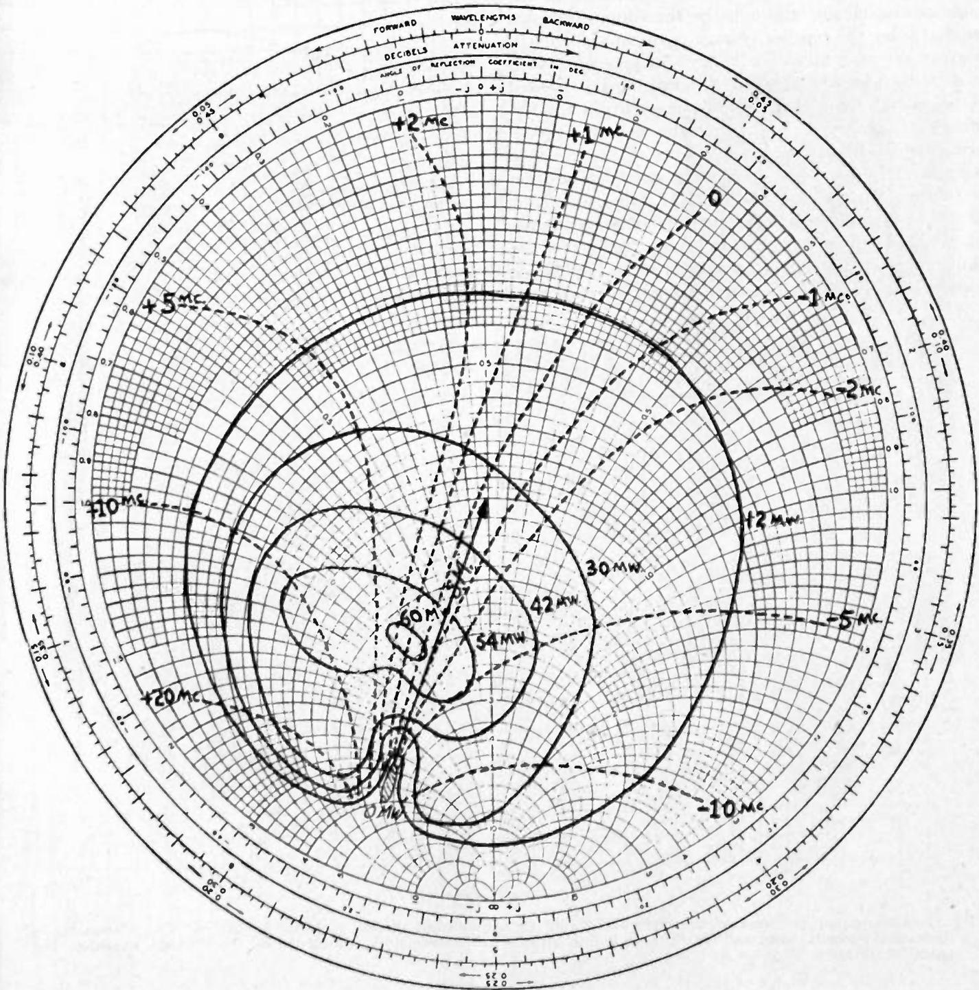
Fig. 10—Impedance performance diagram of a 2K25 tube. Loci of constant power are shown by the solid closed curves. The dashed lines show the loci of constant frequency deviation from the nominal frequency. The tube is operating in mode A, which mode is shown in Fig. 11. Sink margin is indicated by the line SM. This diagram is for mode A,  $F=9360$  Mc., and  $E_{RES}=300$  volts.
