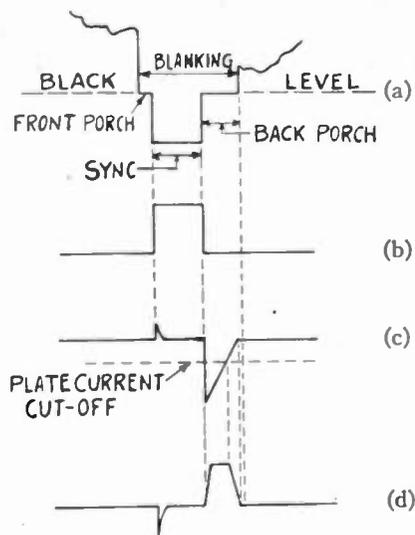
Fig. 18—Derivation of keying pulses for back-porch clamping.
