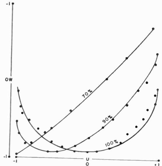
Fig. 11—Experimental  $U$ - $W$  curves taken from auxiliary resonant circuit. (Percentages refer to resonant voltage on auxiliary circuit.)
