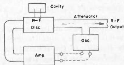
Fig. 1—Block diagram of electronic frequency-stabilization system.
