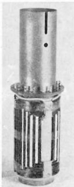
Fig. 8—Deflecting-coil assembly for the image orthicon (outer tube removed).
