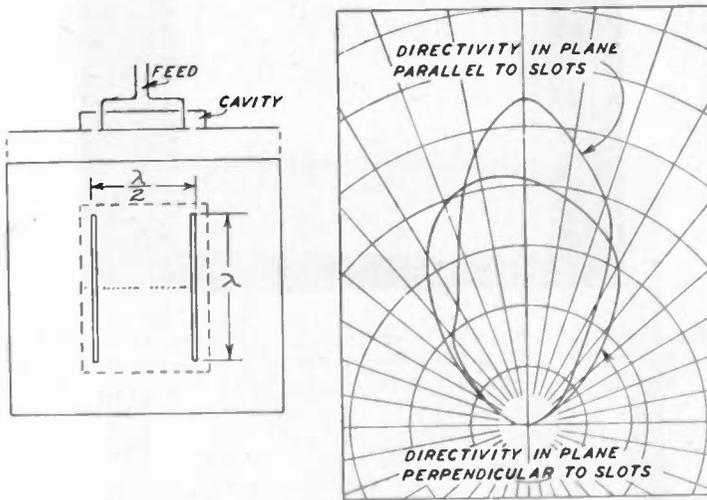
Fig. 3—Simple double-slot antenna.
