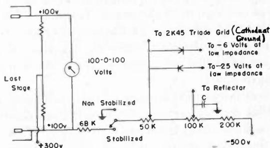
Fig. 10—Supplementary circuit for wide-band single-knob tuning.
