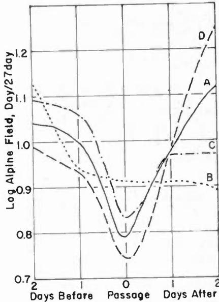
Fig. 9—(A) Alpine fields in log microvolts versus passage of cold fronts. (B) Alpine fields versus passage of cold fronts parallel to transmission path. (C) Alpine fields versus passage of cold fronts making angle with transmission path between 0 and 30 degrees. (D) Alpine fields versus passage of cold fronts making angle with transmission path greater than 30 degrees.
