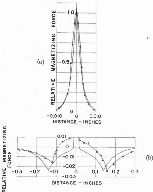
Fig. 5—Measured and empirical field-distribution curves plotted with expanded scales to show comparison. Dots are measured points. (a) Expanded horizontally. (b) Expanded vertically.
