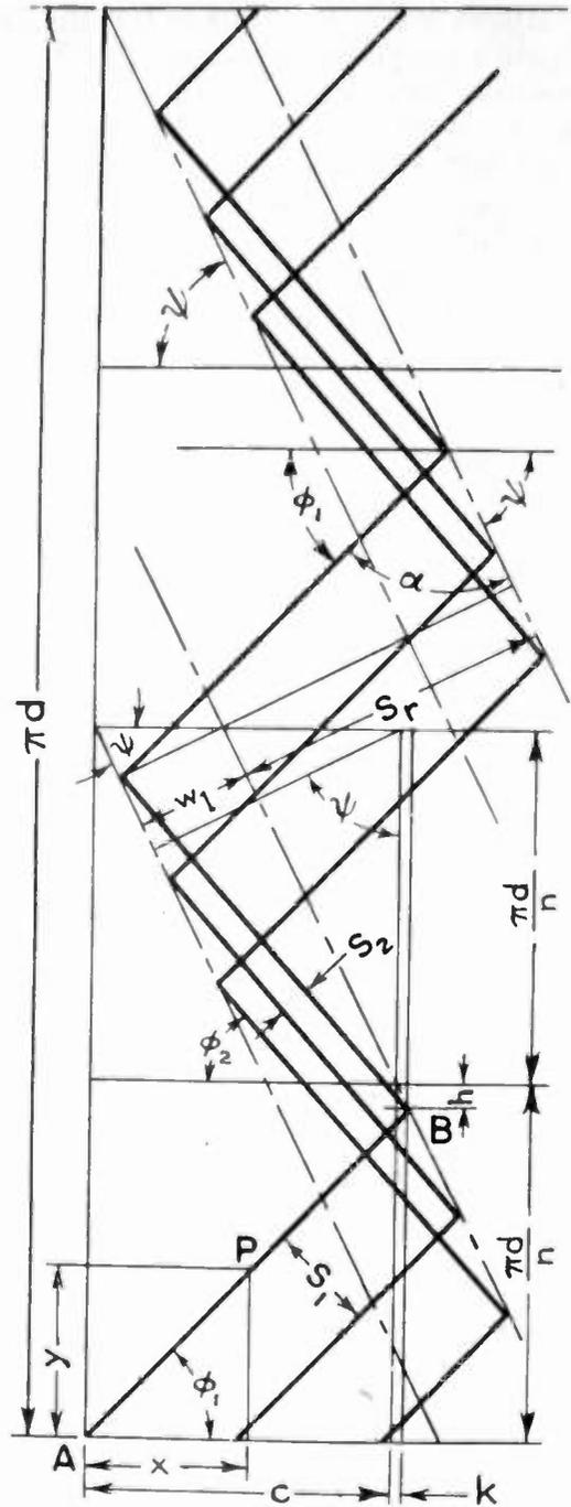
Fig. 2—Developed plane diagram of a progressive universal coil with retrogressive layering.
