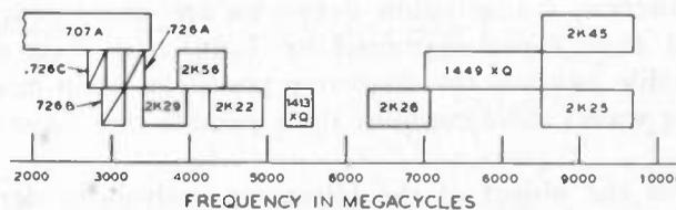
Fig. 15—Frequency coverage of a number of beating oscillators developed in the frequency spectrum of 2000 to 10,000 Mc.
