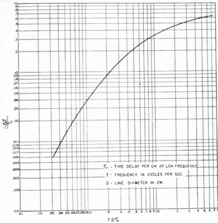
Fig. 4—Delay error as a function of frequency, low-frequency delay, and line diameter.
