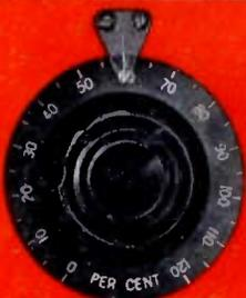
Modulation Indicator Level is set by this dial; lamp flashes when modulation level exceeds that to which dial has been set. Dial range 0 to 120% modulation.
