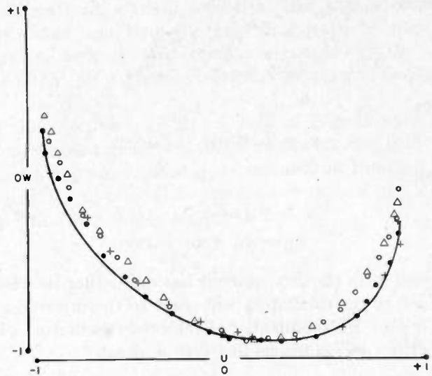
Fig. 8—Experimental and theoretical  $U-W$  curves for the test oscillator. Solid line: theoretical curve for  $\rho = -106.5^\circ$ .
