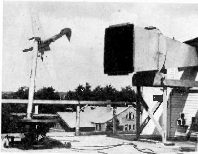
Fig. 4—The electromagnetic horn and the model supporting structure. When measuring patterns, the separation between the model and the horn aperture is usually greater than shown.
