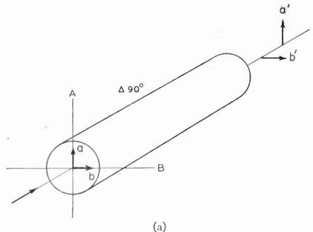
Fig. 2(a)—Conversion from linear to circular polarization by  $\Delta 90$ -degree section.
