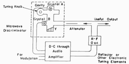
Fig. 8—Block diagram of a d.c. stabilizer
