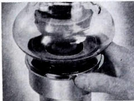
**AUTOMATIC SEAL WATER JACKET.** No tools needed to open and close the new Machlett water jacket. No worry about tube breakage or water leakage. Jacket cannot be opened unless water pressure is off, nor closed unless tube is properly seated. Your hand opens and closes a perfectly safe seal with just a single twist.
