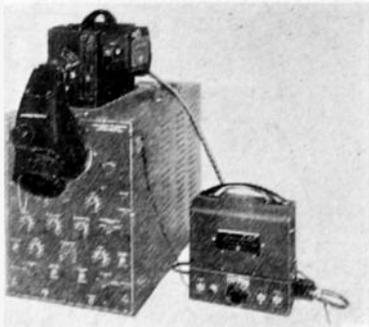
Equipped for mounting atop standard laboratory oscilloscopes, this 35-mm. camera, which makes still or continuously moving film records, photographs high-speed phenomena as well as very low-speed phenomena (too low for visual continuity). It may also be used for quantitative studies—of oscilloscope traces, for record purposes, and for tests using new multiple-beam tubes.
