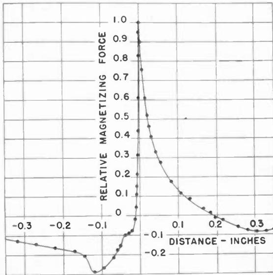
Fig. 7—Relative magnetizing force as a function of distance along the path of the recording medium for an experimental recording head.
