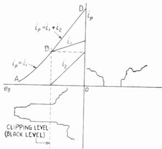
Fig. 21—Characteristic curve of linear clipper.
