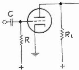
Fig. 19—Schematic diagram of differentiating circuit.
