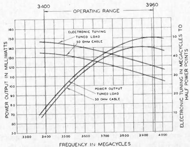
Fig. 4—Power-output and electronic-tuning characteristics for the 2K29 tube. Curves for the tuned-load conditions have been obtained by adjusting a variable load for maximum power output at each measurement. The curves for a 50-ohm-load condition have been obtained by coupling a 50-ohm cable to the tube through a suitable adapter.
