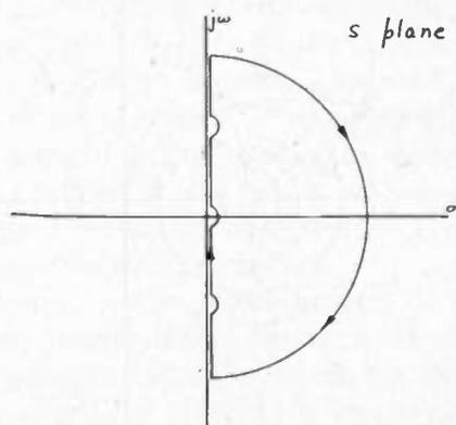
Fig. 2—Contour in  $s$  plane equivalent to  $kL$  contour.
