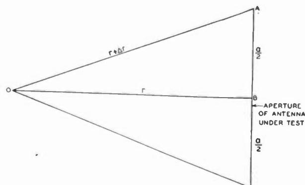
Fig. 11—Calculation of phase deviation due to path length.
