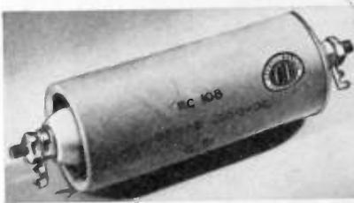
The Type RC-108 capacitor is built in a cylindrical metal container  $1\frac{1}{2}$  inches in diameter, 3 inches long, with screw-type terminals mounted on ceramic insulators protruding  $\frac{3}{4}$  inch from each end of the case. A wax-impregnated cardboard sleeve provides insulation.
