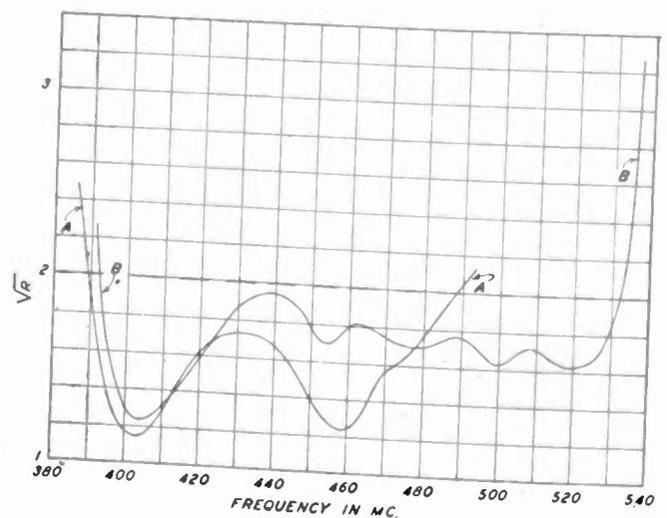
Fig. 14—Standing-wave-ratio curve of the antenna of Fig. 12 as compared with the standing-wave-ratio of the antenna without subdivided cavity.
