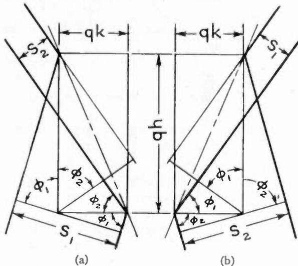
Fig. 3—Detailed view of the spacing of adjacent turns of wire. (a) Retrogressive layering. (b) Progressive layering.
