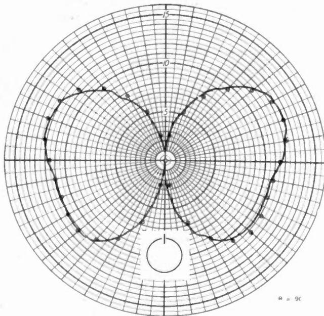
Fig. 10—Pattern of short radial antenna on a cylinder one-half wavelength in diameter. Points computed. Curve measured at 1000 Mc.
