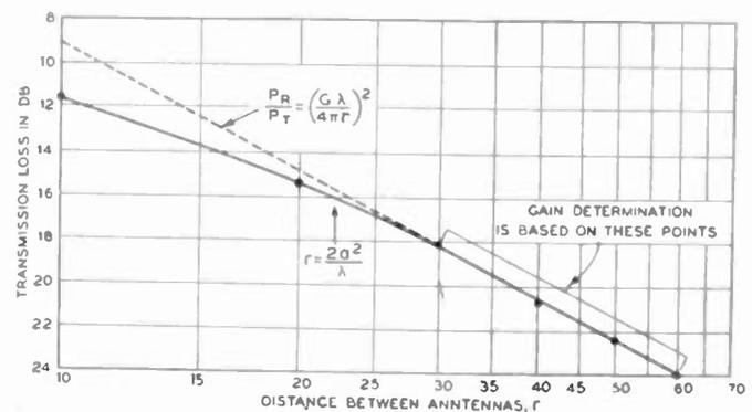
Fig. 3—Absolute-gain determination of two identical optimum horns having square apertures with sides of length  $\alpha$ .
