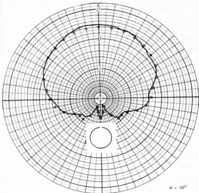
Fig. 13—Pattern of a narrow axial slot three-quarters wavelength long, in a cylinder one and one-quarter wavelength in diameter. Points computed. Curve measured at 3000 Mc.
