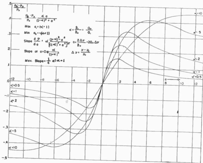
Fig. 7—Output voltage versus frequency for various cavity-coupling factors of the balanced magic-tee discriminator.
