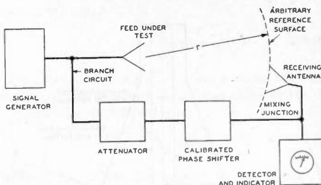
Fig. 9—Basic phase-measuring circuit.
