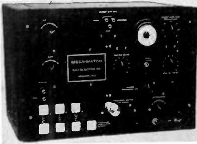
This instrument measures reflected energy over a wide frequency band, 10 to 250 Mc. and up. It presents a visual display of reflected energy over any band up to 30 Mc. This visual display eliminates tedious tabulation work, saving hours of engineering time.
