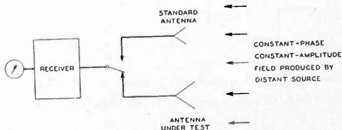
Fig. 1—Gain measurement by the substitution method.
