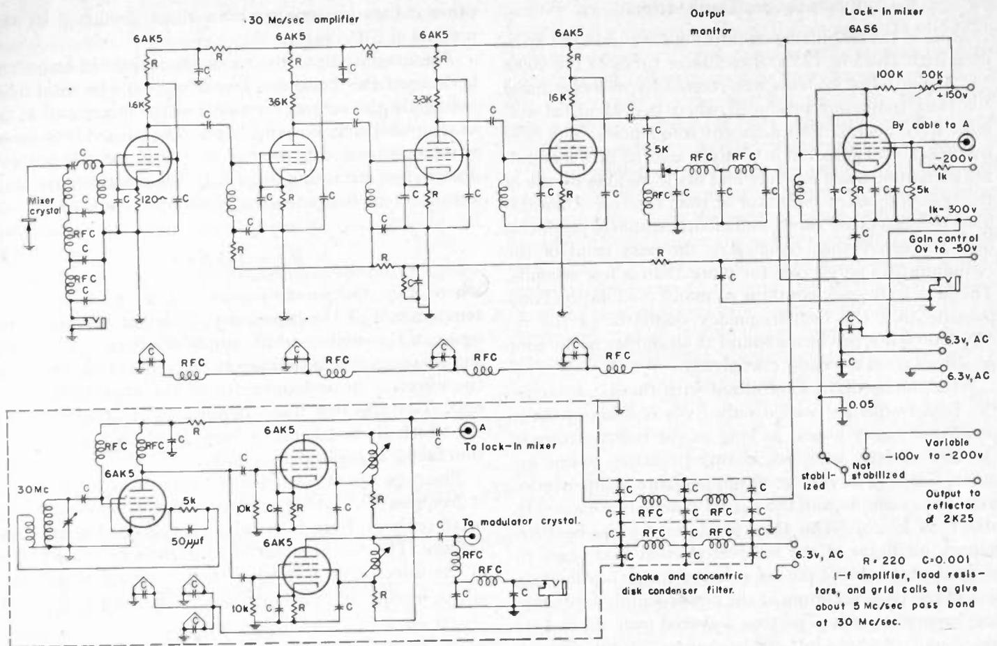
Fig. 12—I.f. amplifier, oscillator, buffers, and phase mixer of the stabilization system.
