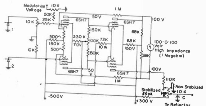
Fig. 9—D.c. amplifier for the electronic frequency stabilizer.
