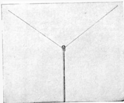
Where the FM reception band is the only object of the antenna design, the well-engineered, simple Premax Adjustable "V" Dipole Type is very effective.
