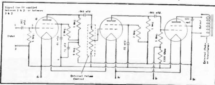
SCHEMATIC DIAGRAM of typical "Ampec" illustrated shows what components can be used. "Ampecs" can be designed to meet a wide range of gain or frequency response requirements.
