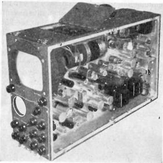
Fig. 10—Field-camera control.
