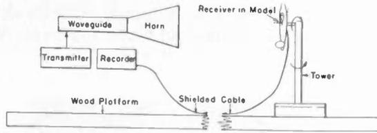
Fig. 3—Diagram showing equipment used for measuring model antenna patterns at high frequencies.
