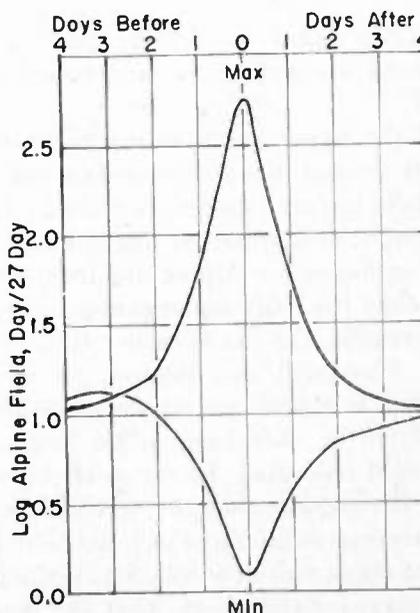
Fig. 5—W2XMN field intensity grouped about epoch of maxima and minima fields in log microvolts. Maxima = 2.0; minima = 0.2,
