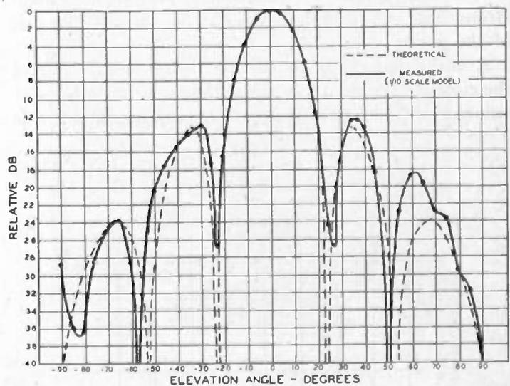
Fig. 7—Calculated and measured free-space vertical-plane field-strength pattern of a five-unit cloverleaf antenna.
