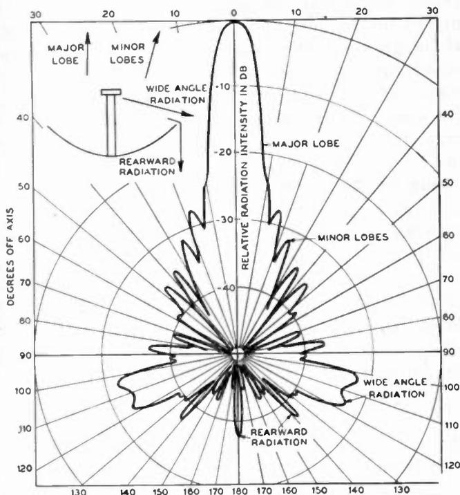
Fig. 4—Representative polar diagram for a microwave antenna.
