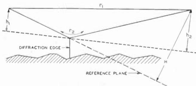
Fig. 13—Use of a diffraction edge.
