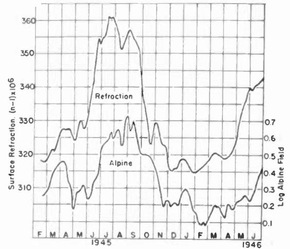
Fig. 2—Field reception of W2XMN on 42.8 Mc. at Needham, Mass., 1945-1946.
