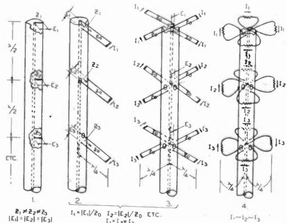
Fig. 5—Proceeding from left to right, steps 1 to 4 illustrate how approximately equal currents are supplied to all radiating units of the cloverleaf antenna.
