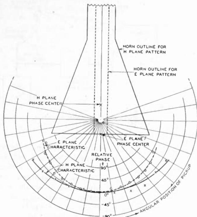
Fig. 10—Typical phase pattern.
