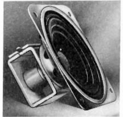
These speakers use 1.47-oz. Alnico V magnets, an unusually sturdy frame, and a preformed speaker cone and curves verify the fine response characteristics. The standard speakers are of RMA 3.2-ohm impedance. Special impedances are available.
