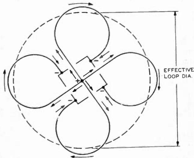
Fig. 1—Arrangement of four radiating elements constituting a radiating unit of the cloverleaf antenna. Arrows indicate assumed instantaneous directions of current.
