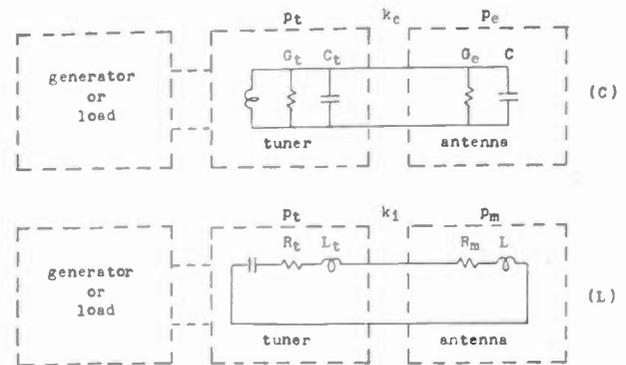
Fig. 2—Tuned coupling of antenna with generator or load.
