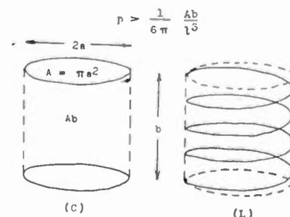
Fig. 1—Capacitor (C) and inductor (L) occupying equal cylindrical volumes.
