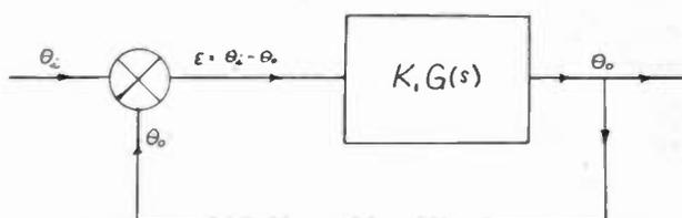
Fig. 1—Block diagram of single-loop servomechanism.
