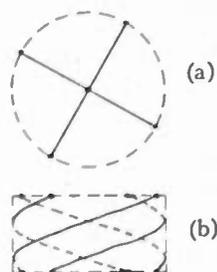
Fig. 2—The multifilar helical antenna of fractional turns.
