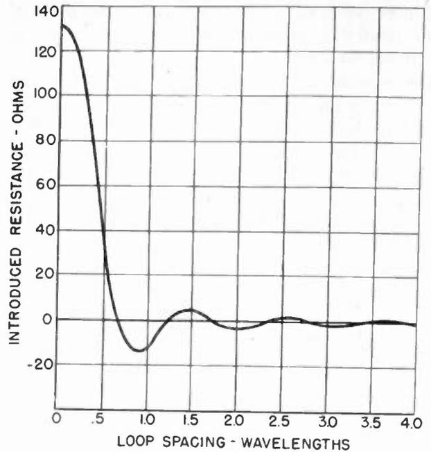
Fig. 4—Introduced resistance in a hypothetical uniform-current loop 0.3 wavelength in diameter, due to the presence of a similar adjacent loop.
