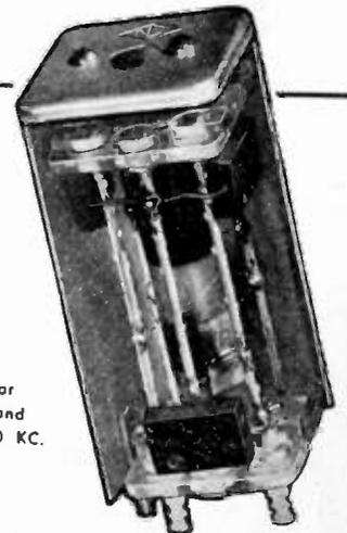
● The IFO is an FM discriminator transformer of the ratio type and is linear over a band of  $\pm 100$  KC.
