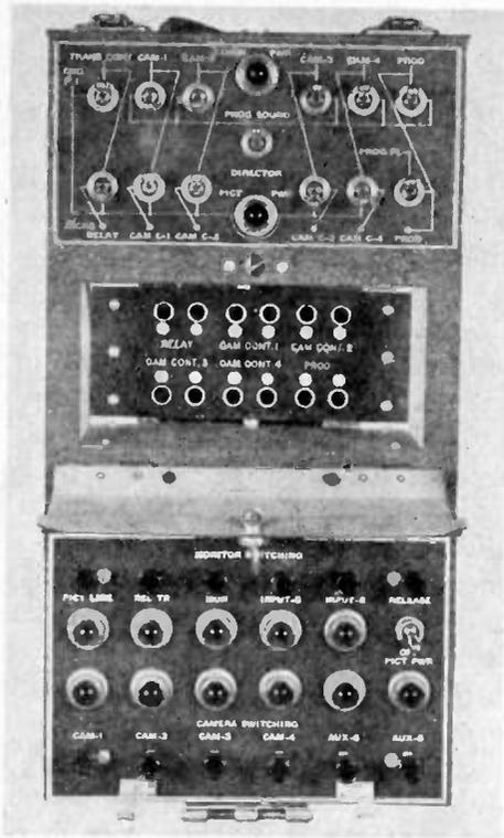
Fig. 14—Field switching system, front side.
