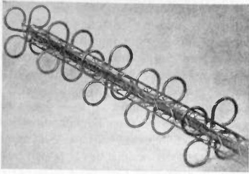
Fig. 3—Stacked array of five radiating units of a scale-model cloverleaf antenna.
