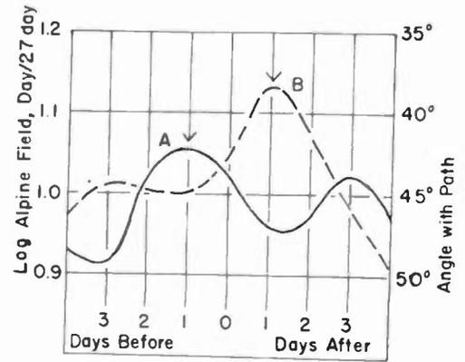
Fig. 15—Alpine fields versus angle of wind direction with respect to transmission path. (A) epoch (0) is for wind parallel with path; (B) shows angle of wind direction with path before and after day of minimum field.
