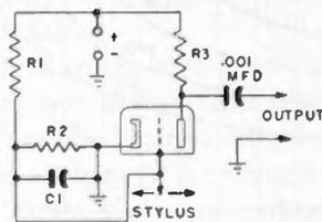
Fig. 8—A simple form of RC coupling which proved satisfactory in the experimental work with the tube.
