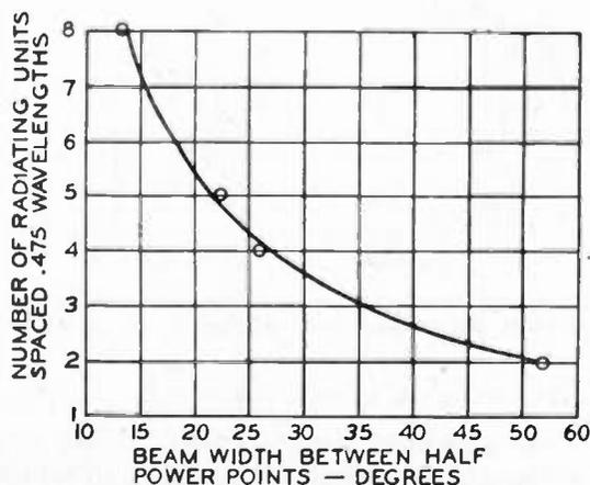
Fig. 9—Calculated and measured vertical-plane beam width between half-power points versus number of radiating units of a cloverleaf antenna.
