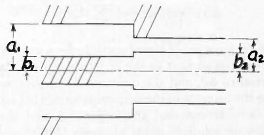
Fig. 1—Coaxial line discontinuity.
