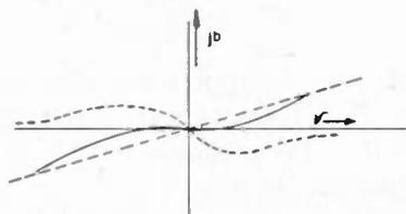
Fig. 3—Susceptance versus frequency at critical coupling.
