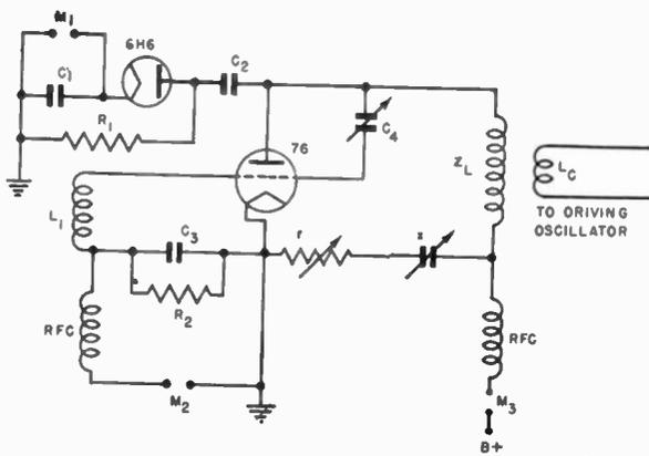
Fig. 3—Circuit diagram of the test oscillator.
