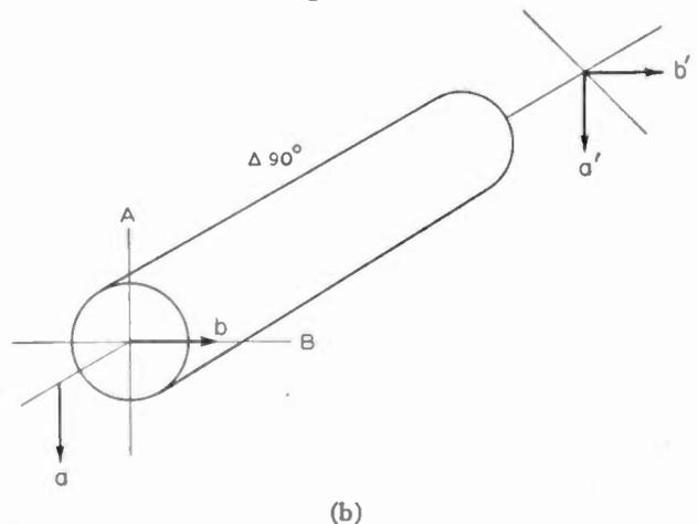
Fig. 2(b)—Conversion from circular to linear polarization by  $\Delta 90$ -degree section.
