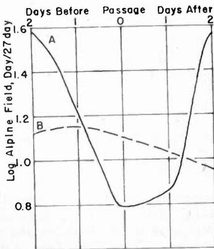
Fig. 10—(A) Alpine fields in log microvolts versus passage of warm fronts. Note that maximum transmission occurs two days before and after day of front passage. (B) Alpine fields versus passage of occluded fronts. Note small effect of such fronts on field strengths.
