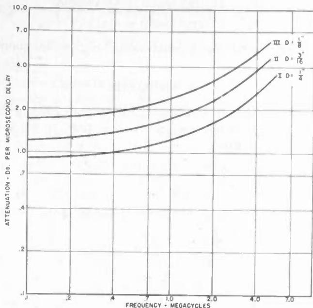
Fig. 5—Attenuation as a function of frequency of curves I, II, and III on the design chart, Fig. 7.
