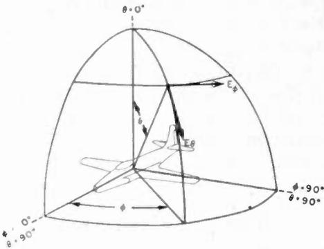
Fig. 1—Spherical co-ordinate system showing orientation of field components relative to aircraft.
