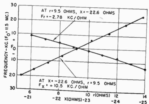
Fig. 5—Experimental curves for evaluation of  $F_r$  and  $F_x$ .
