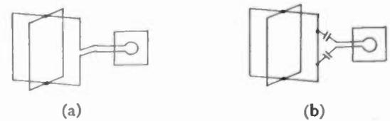
Fig. 5—Connections with a multifilar helical antenna.
