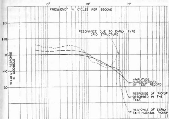
Fig. 6—Frequency response of an early type of pickup, along with that of the tube described in the text, compared with the amplitude characteristic of the test record used.
