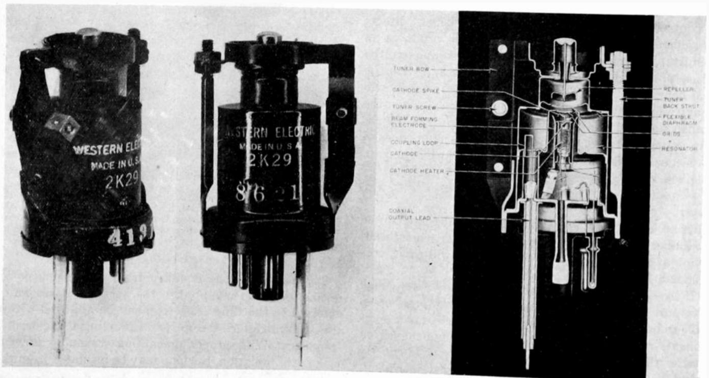
Fig. 3—External and cut-away views of all-metal mechanically tuned beating oscillators. The left-hand views are for a 2K29 showing the bow construction for mechanical tuning. The frequency range of this oscillator is 3400 to 3960 Mc. The right-hand view shows a cut-away section of the 726B beating oscillator. The frequency range of this oscillator is from 2880 to 3170 Mc.
