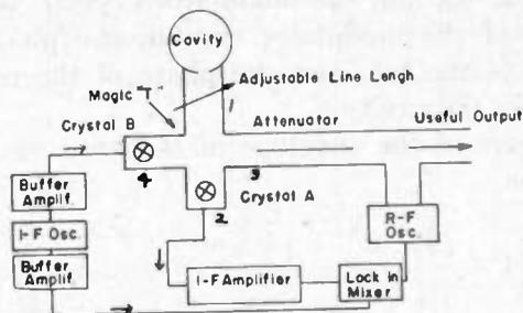
Fig. 11—Block diagram of the i.f. stabilizer.
