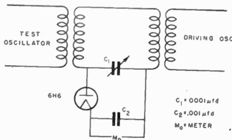
Fig. 10—Auxiliary resonant circuit to obtain behavior characteristic of  $\rho = 0$ .
