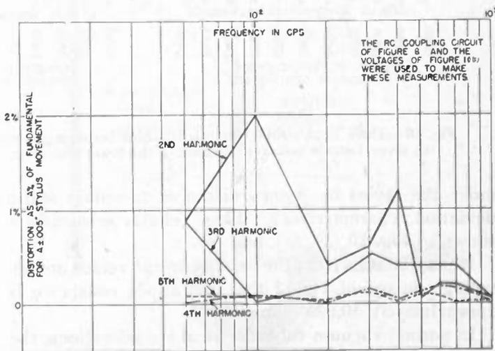
Fig. 9—Curves showing measured harmonic distortion where the stylus was driven by a voice-coil arrangement. In actual practice the stylus deviation does not reach ±0.001 inch with the result that the actual measured distortion is comparable to or less than that on the record itself.
