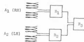
Fig. 6—Diversity receiver using helical antennas of opposite circular polarization.
