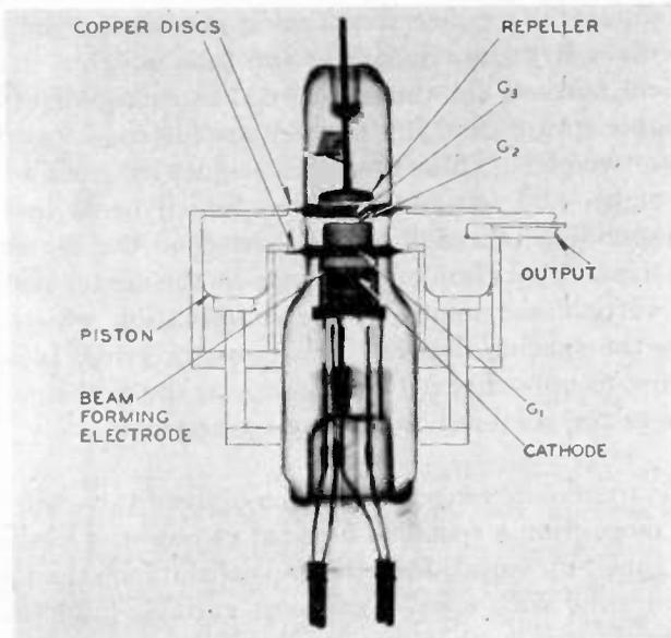
Fig. 1—X-ray view of a W.E. 707A tube. A method of mounting an external resonator on this tube is indicated.
