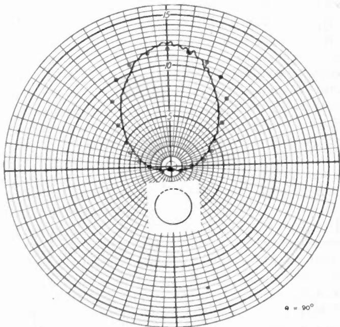
Fig. 14—Pattern of a narrow transverse slot three-quarters wavelength long, in a cylinder one and one-quarter wavelengths in diameter. Points computed. Curve measured at 3000 Mc.
