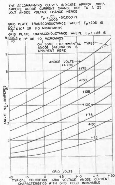
Fig. 2—By maintaining the grid in a fixed position at its neutral point, the static grid-voltage versus anode-current characteristics may be taken in a normal manner.
