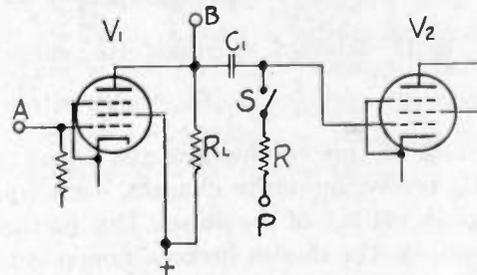
Fig. 16—Simplified schematic diagram of clamp circuit.
