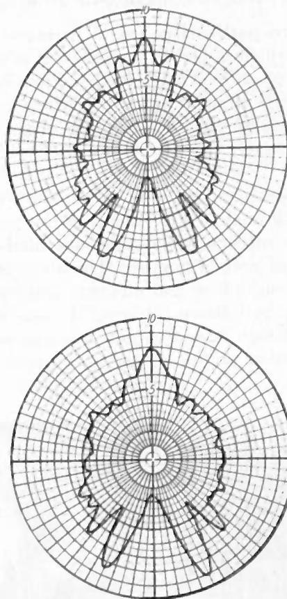
Fig. 15—Patterns of the  $E_{\theta}$  component in the horizontal plane ( $\theta=90^{\circ}$ ) for a vertical stub antenna mounted in a B-17. Full scale frequency, 150 Mc. Above: 1/20-scale model. Below: 1/40-scale model.
