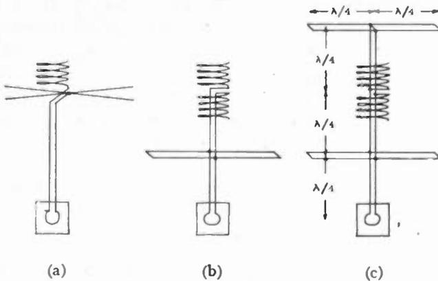
Fig. 4—Connections through a transmission line.
