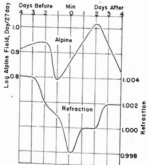
Fig. 8—Upper curve: W2XMN field intensities grouped about epoch of minimum surface refraction. Lower curve: surface refraction grouped about epoch of minimum W2XMN reception.
