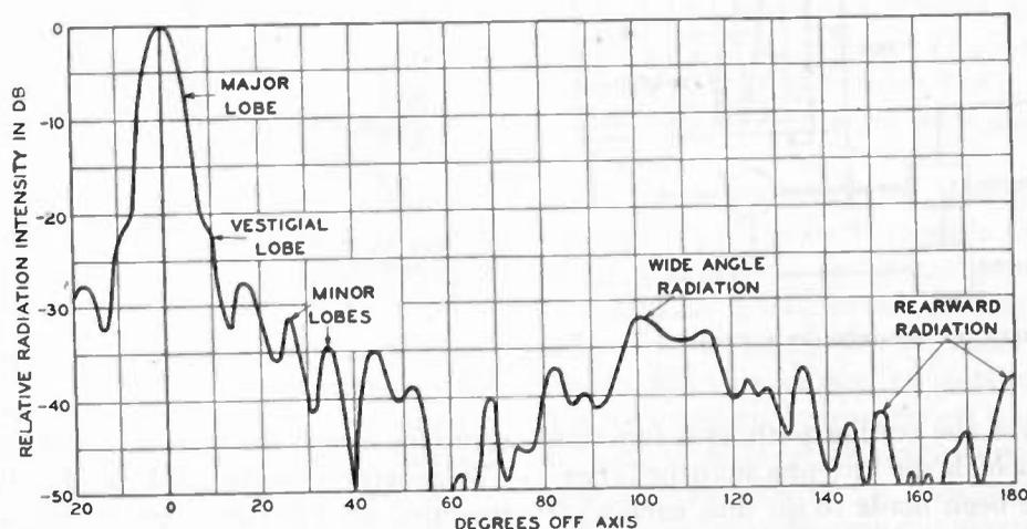
Fig. 5—Directional pattern of Fig. 6, plotted on rectangular co-ordinates.
