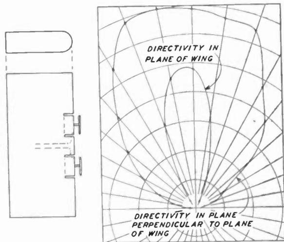
Fig. 2(b)—Same combination as in Fig. 2(a) with parasitic radiators added approximately one-quarter wave in front of each slot pair.
