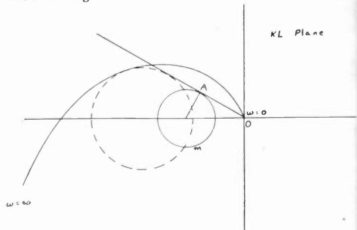
Fig. 4—Graphical construction to determine gain coefficient for desired damping ratio.
