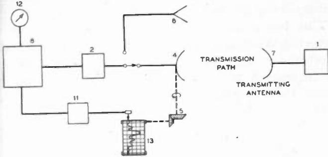
Fig. 15—Simple system for gain and pattern measurement.
