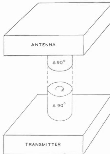
Fig. 6—Rotary joint using circular polarization.
