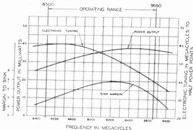
Fig. 11—Power output, electronic tuning, and sink margin for a typical 2K25 tube when coupled to the characteristic impedance of the wave guide through a suitable coupling.
