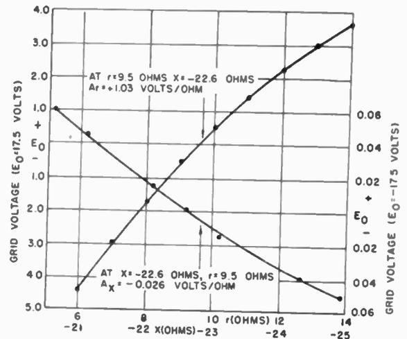
Fig. 4—Experimental curves for evaluation of  $A_r$  and  $A_x$ . (Use left ordinates for  $A_r$ , right ordinates for  $A_x$ .)
