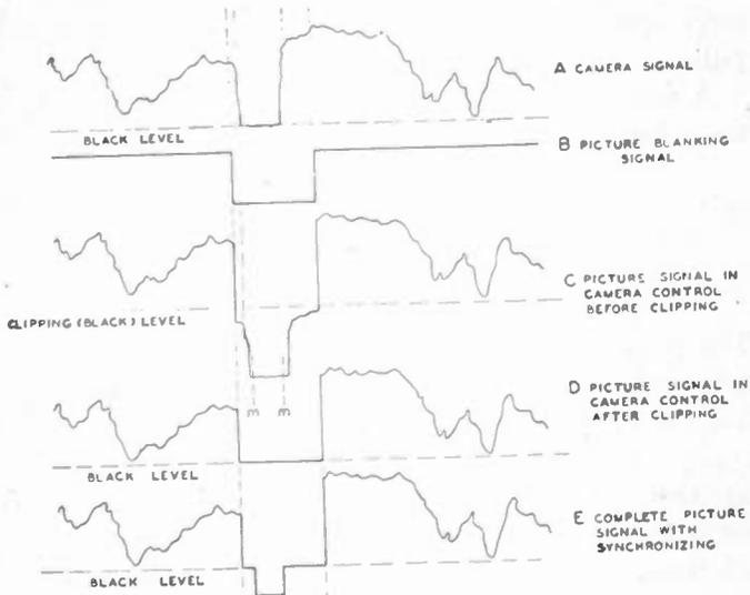
Fig. 15—Television signal waveforms.
