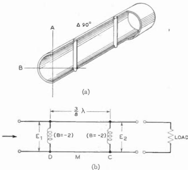
Fig. 10—Rod-type  $\Delta 90$ -degree section. (a) Cut-away view. (b) Equivalent circuit.
