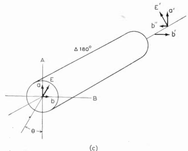
Fig. 2(c)—Rotation of polarization by means of  $\Delta 180$ -degree section.
