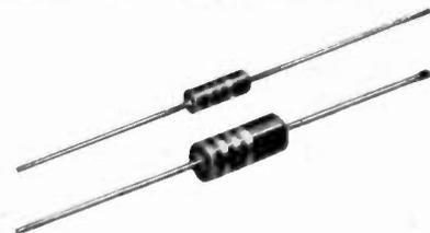
The size of the  $\frac{1}{2}$ -watt resistor is only  $\frac{3}{16}$ -inch long and  $9/64$ -inch diameter; the 1-watt unit is  $9/16$ -inch long and  $7/32$ -inch diameter. They are claimed to meet all test requirements for the best quality characteristics of joint Army-Navy specification JAN-R-11, including salt-water immersion cycling and high-humidity tests.
