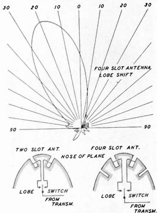
Fig. 9—Shiftable, single-slot feed for lobe switching. Note the application of this slot antenna to the curved contour of the model of the nose of an airplane.
