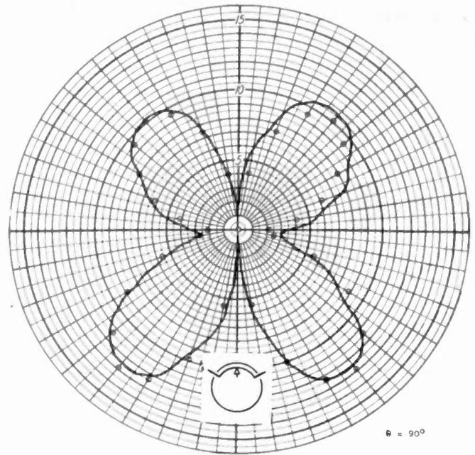
Fig. 11—Patterns of array of two radial antennas on cylinder one-half wavelength in diameter. The antennas were mounted  $120^\circ$  apart on the circumference and fed in phase. Points computed. Curve measured at 1000 Mc.
