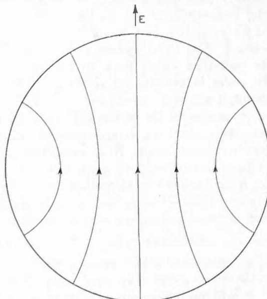
Fig. 1—Field pattern and polarization of dominant wave in circular guide.
