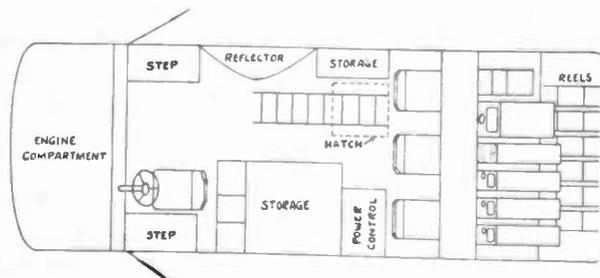
Fig. 5—Plan diagram of the mobile unit.
