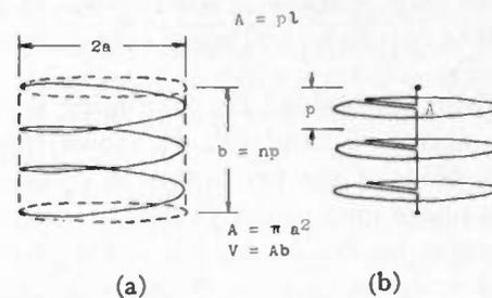
Fig. 1—The helical antenna (a) and the components of a single turn (b).
