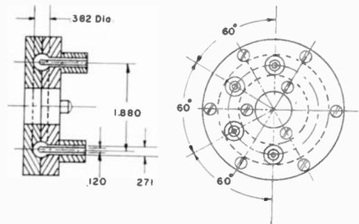
Fig. 5—10-centimeter coaxial line equivalent to a "magic tee."
