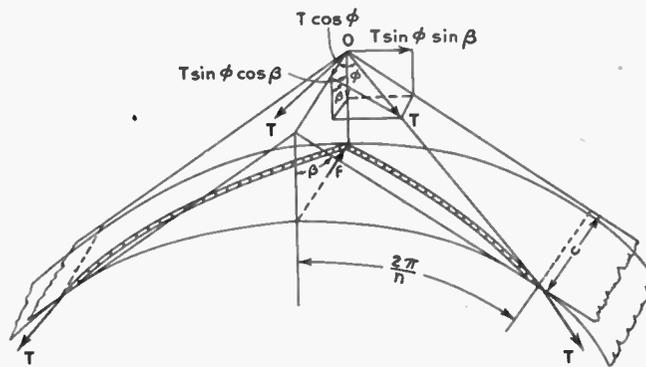
Fig. 4—Spatial view of a portion of an ordinary universal coil, showing all the mechanical forces acting on two throws of wire.
