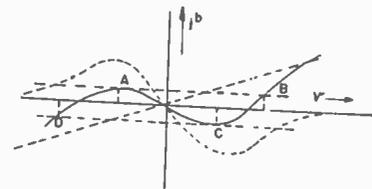
Fig. 2—Susceptance versus frequency in an oscillator with a high- $Q$  load circuit.
