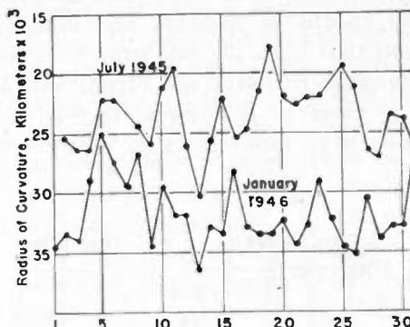
Fig. 4—Calculated radius of curvature of bending by atmosphere from RAOB observations above Albany, N. Y., for July, 1945, and for January, 1946.
