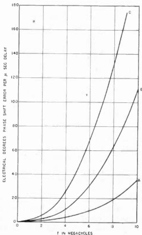
Fig. 6—Delay error as a function of frequency. Phase distortion of curves A, B, and C on the design chart, Fig. 7.
