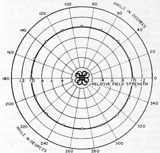
Fig. 2—Azimuth-plane-radiation pattern of a four-unit scale-model cloverleaf antenna. Measured points show variation from a circle to be within the limits of experimental accuracy.
