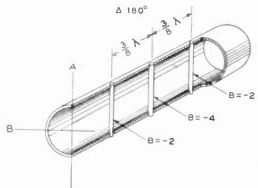
Fig. 11—Rod-type  $\Delta 180$ -degree section.
