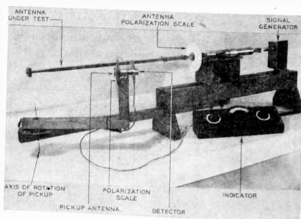
Fig. 7—Primary-pattern-measuring equipment.
