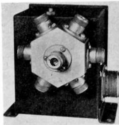
Pictured here is the type D, a six-position switch for use with RG-8/U r.f. cable. Voltage-standing-wave ratio is less than 1.5 to 1; adjacent-channel attenuation is better than 50 db.
