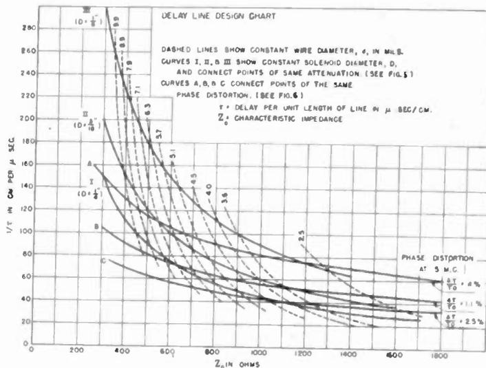
Fig. 7—Delay-line design chart.
