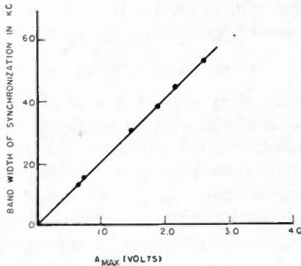
Fig. 6—Experimental determination of bandwidth of synchronization in terms of injected voltage as measured by  $a_{\max}$ . The slope of the curve is 20.6 kc./volt.
