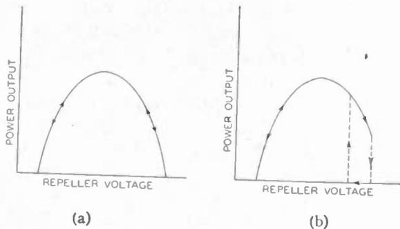
Fig. 5—Power output as a function of repeller voltage. The repeller-voltage range covered is sufficient to show only one operating mode. (a) Ideal curve, showing no discontinuities. The return sweep presents a trace which is completely identical with the forward trace. (b) A type of trace which may be obtained when electronic hysteresis is present.
