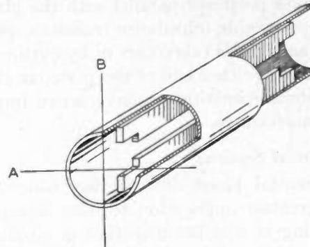
Fig. 8—Fin-type phase-shift section.
