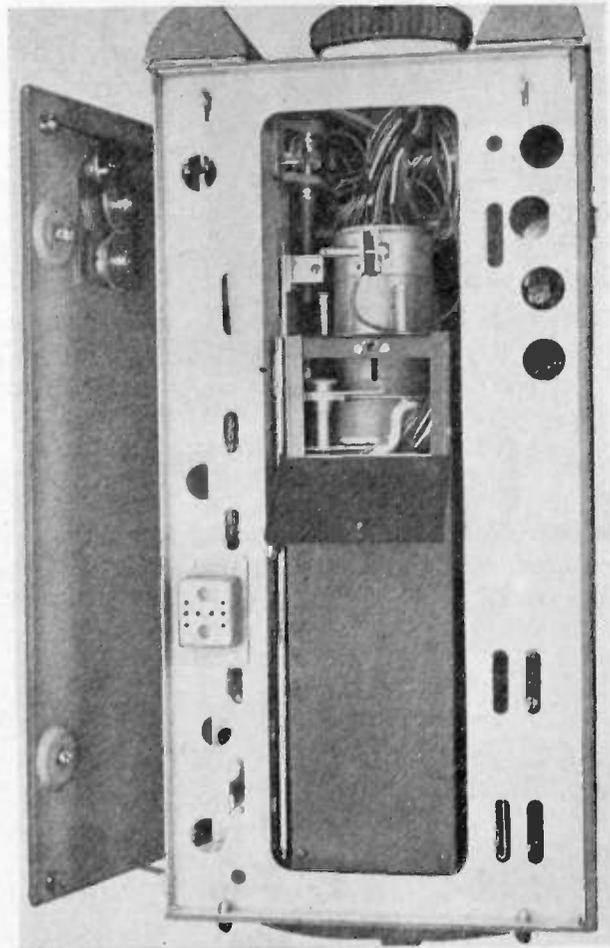
Fig. 6—Top view of camera, showing coil assembly.
