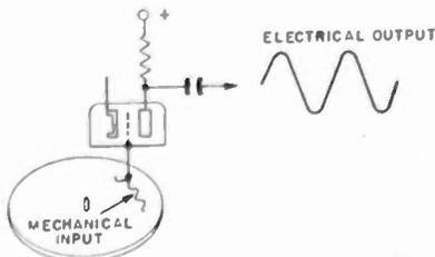
Fig. 1—Diagram of a simple triode phonotube arrangement.
