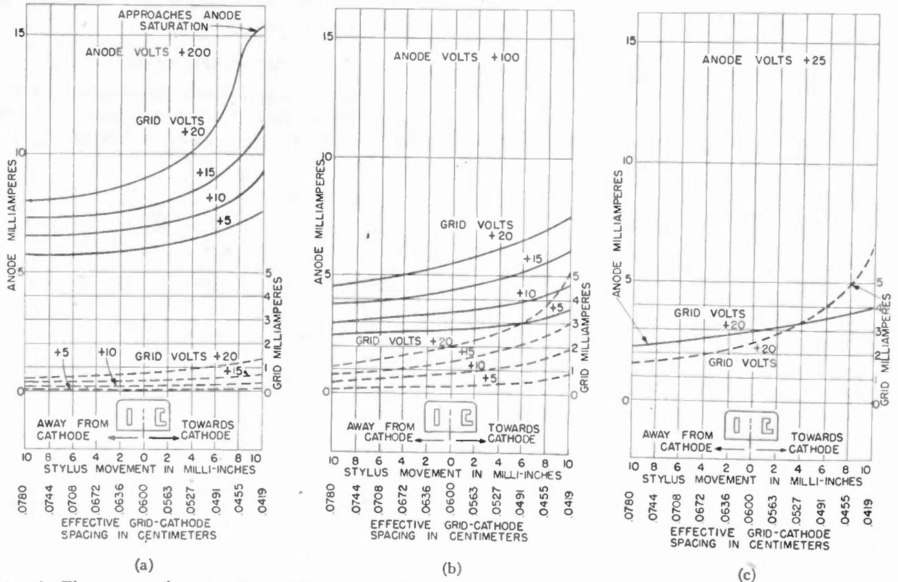
Fig. 10—These curves show the relationships between grid current, anode current, grid deviation, and linearity, with respect to several anode voltages. Because of the lower distortion, the curves shown in (c) are typical operating characteristics.
