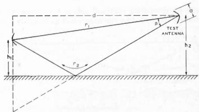
Fig. 12—Path-length determination.
