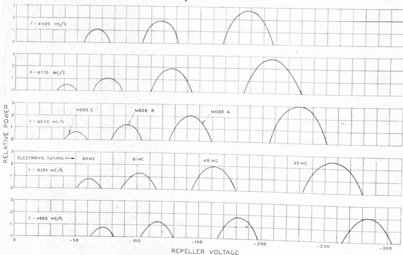
Fig. 12—Power-output performance for a typical 2K25 tube for five different nominal operating frequencies. The performance in the various modes is shown, and the electronic tuning, between half-power points, is indicated for the 9390-Mc. condition. The resonator voltage is 300 volts.
