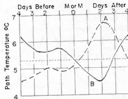
Fig. 11—Correlation of temperature in degrees centigrade with Alpine fields before and after days of maximum reception (A), and of minimum reception (B).
