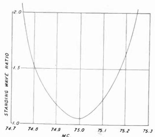
Fig. 19—Standing-wave-ratio curve for marker-beacon antenna.
