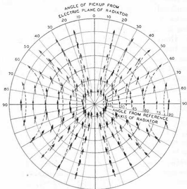
Fig. 8—Polarization characteristic of a typical antenna feed.
