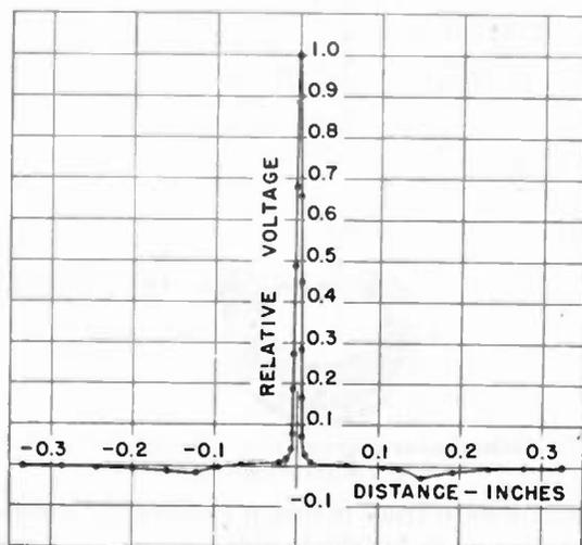
Fig. 4—Relative voltage induced in the exploring coil as a function of distance along the path of the recording wire.
