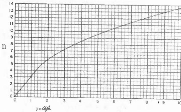
Fig. 5—A plot of the curve which determines the maximum number of throws per coil revolution as a function of the coefficient of friction, coil-form diameter, and cam throw.
