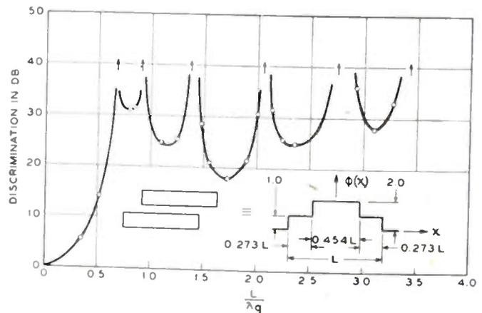
Fig. 4—Computed directivity for two constant-amplitude couplings superposed.
