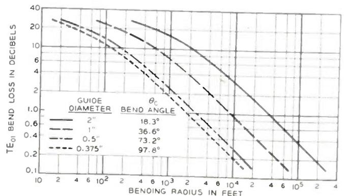
Fig. 23— $TE_{01}$  bend loss versus bending radius for a  $\theta_c$ -angle bend in several round guides operated at 50,000 mc.
