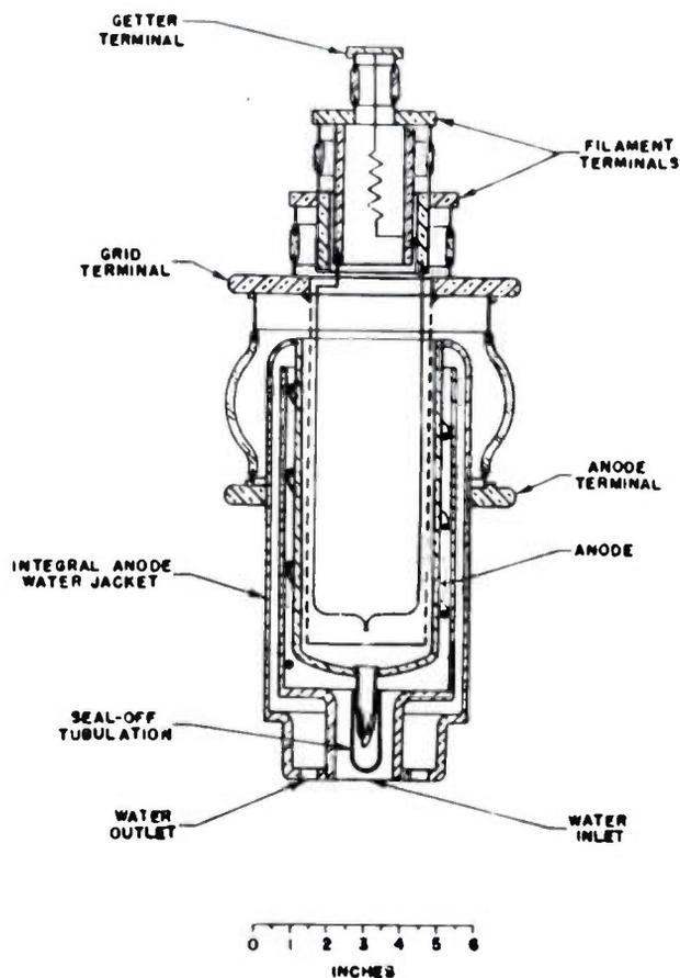
Fig. 1—Section view along the principal axis of the ML-5681 power triode.
