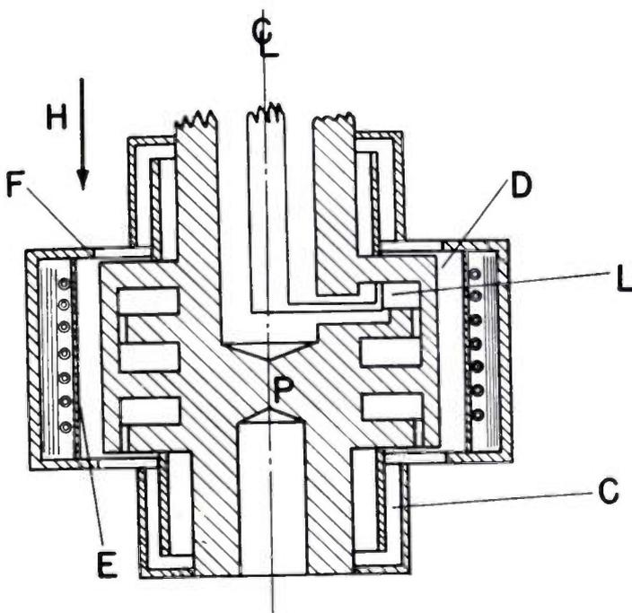
Fig. 2—Cross-sectional view of a stacked inverted interdigital magnetron.
