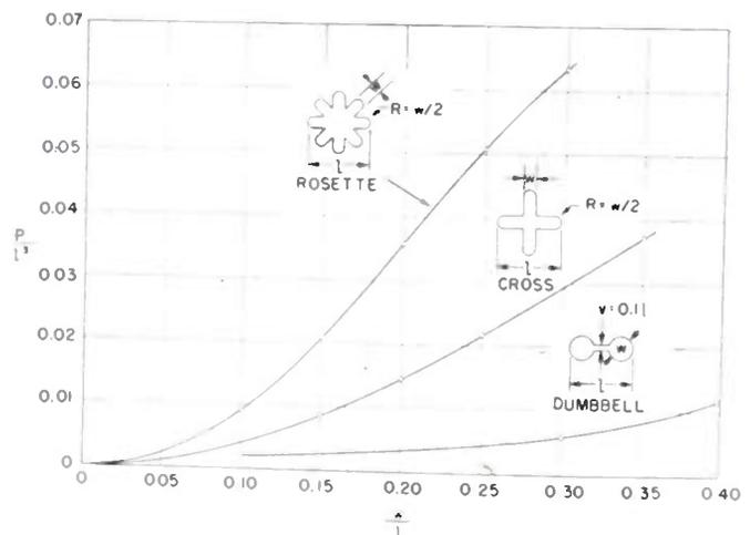
Fig. 4—Measured electric polarizability of cross, rosette, and dumbbell apertures.
