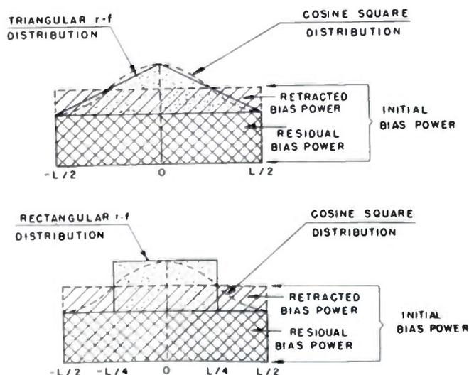
Fig. 5—Bias and assumed RF power distributions in bolometer used to compute the error due to resistance-power nonlinearity.
