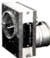
**TYPE V** For precision in sampling speed plus long life. Synchronous drive motor permits selection of single pole sampling of 60 fixed contacts at many rates from 1 rps. to 1 rev. per day. Adaptable, through variety of mountings and terminals, for use as a component of industrial instrumentation systems.
