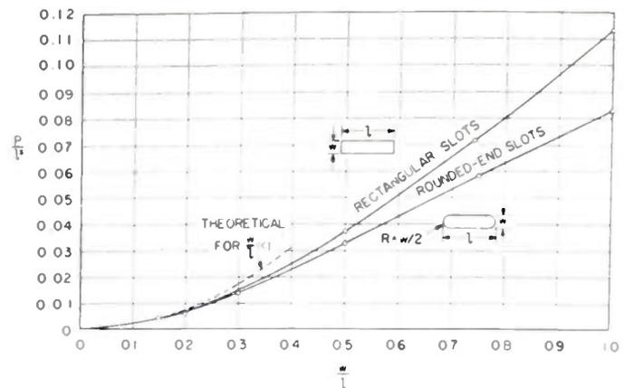
Fig. 3—Measured electric polarizability of rectangular and rounded slots.
