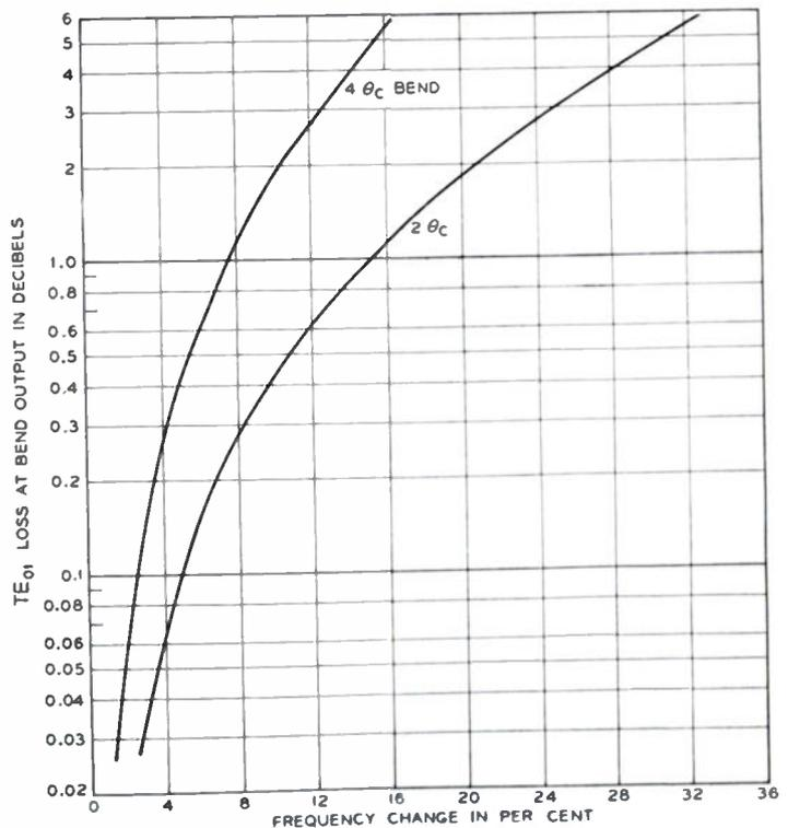
Fig. 5—Theoretical bandwidth of discrete angle bends.
