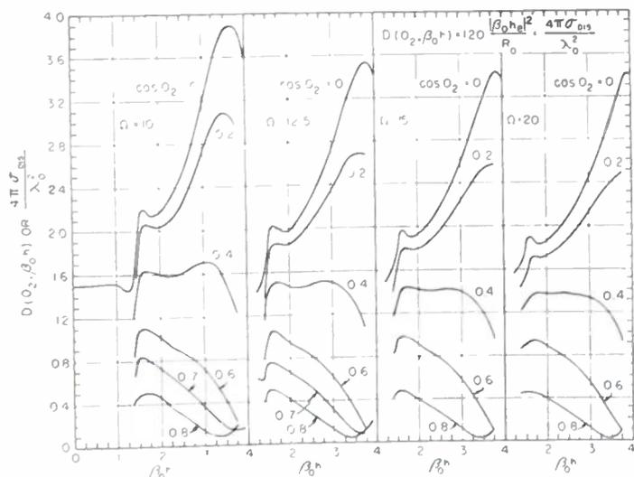
Fig. 11—Gain or directivity of receiving antenna with its orientation angle  $\theta_2$  (Fig. 1) as parameter.
