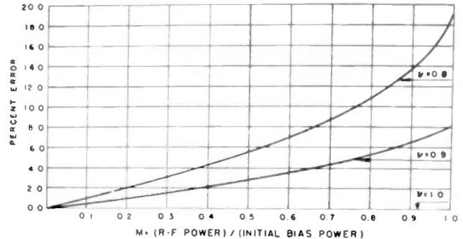
Fig. 7—Calculated resistance-power nonlinearity error as a function of ratio of RF power to initial bias power for rectangular distribution of Fig. 5.
