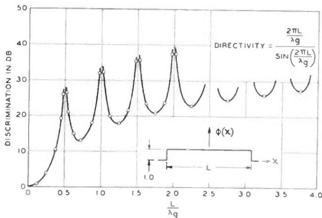
Fig. 2—Computed directivity for constant amplitude and phase of coupling.
