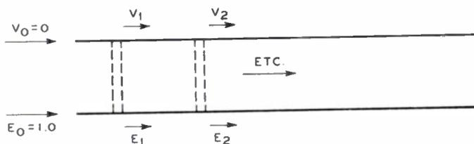
Fig. 20—Diagram for illustrating discrete coupling relations in tightly coupled directional couplers.
