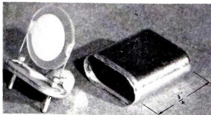
Fig. 1—A typical overtone crystal unit for frequency standard use, with the cover removed to show the simplicity of design.
