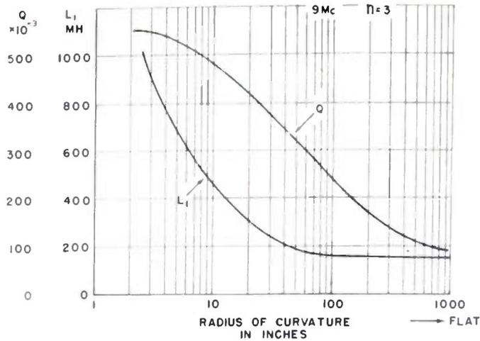
Fig. 5—Variation in  $Q$  and inductance with the degree of contour on a 9-mc, third overtone crystal unit.
