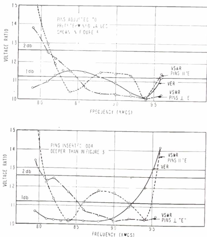
Fig. 4(a) and (b)—Voltage ellipticity and voltage standing-wave ratios versus frequency.
