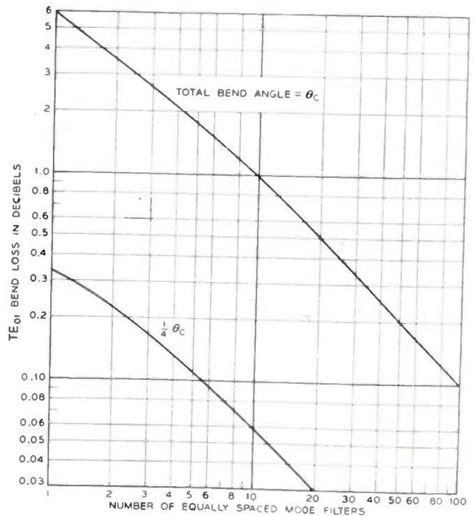
Fig. 19—The effect on  $TE_{01}$  bend loss due to mode filters in the configuration of Fig. 18.
