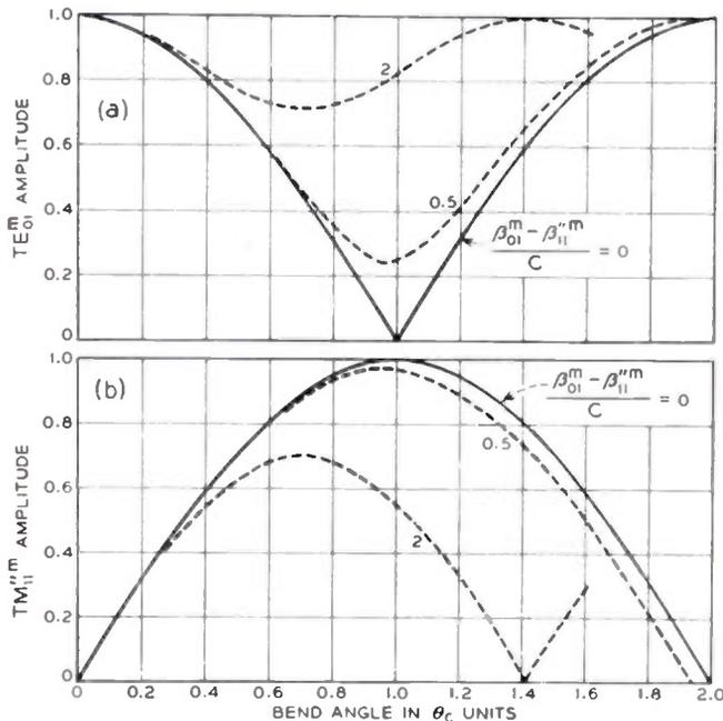
Fig. 6—The effects of degeneracy removal on transmission through bends. (a)  $TE_{01}^m$  bend output. (b)  $TM_{11}''^m$  bend output.
