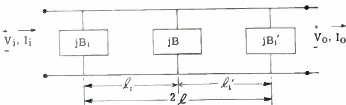
Fig. 1—Susceptance-loaded transmission line.
