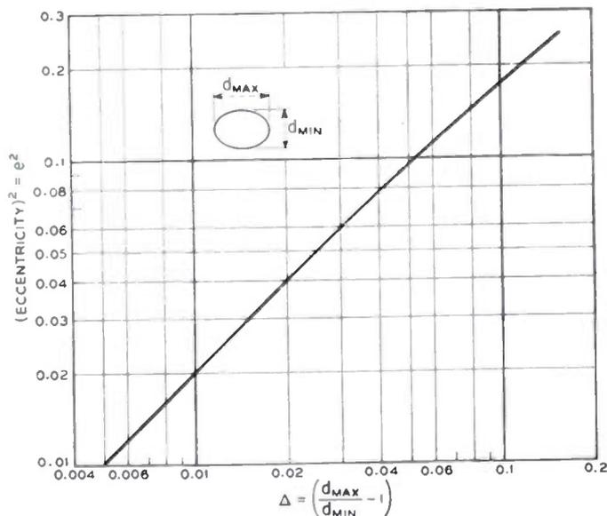
Fig. 9—Elliptic waveguide eccentricity versus the major-to-minor axis ratio.
