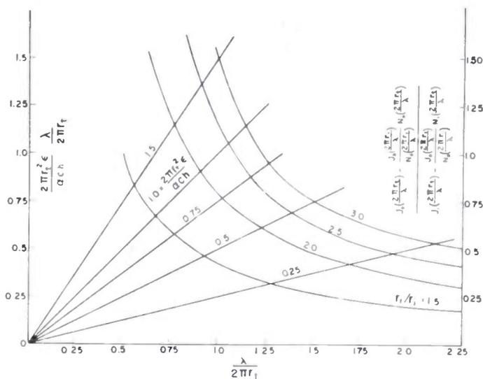
Fig. 4—Resonant wavelength equation plot for inverted interdigital magnetrons in the mode of no angular variation.
