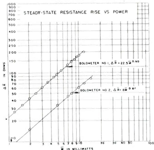
Fig. 4—Steady-state resistance-power characteristics for two different Wollaston wire bolometers.
