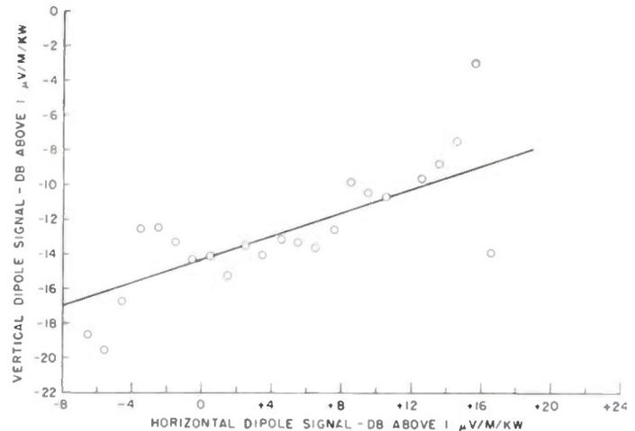
Fig. 4—Vertical dipole component of scattered wave.
