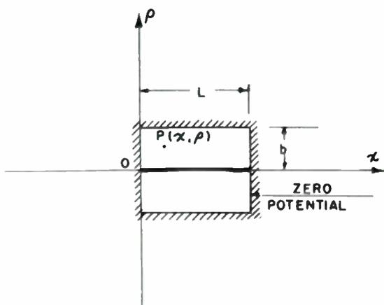
Fig. 1—Electrostatic analogue for an infinitesimally thin heated wire surrounded by a stagnant air sheath. Finite line charge on axis of closed cylinder.
