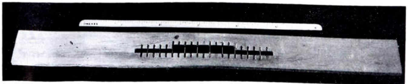
Fig. 10—Insert with two constant amplitude coupling functions superposed.
