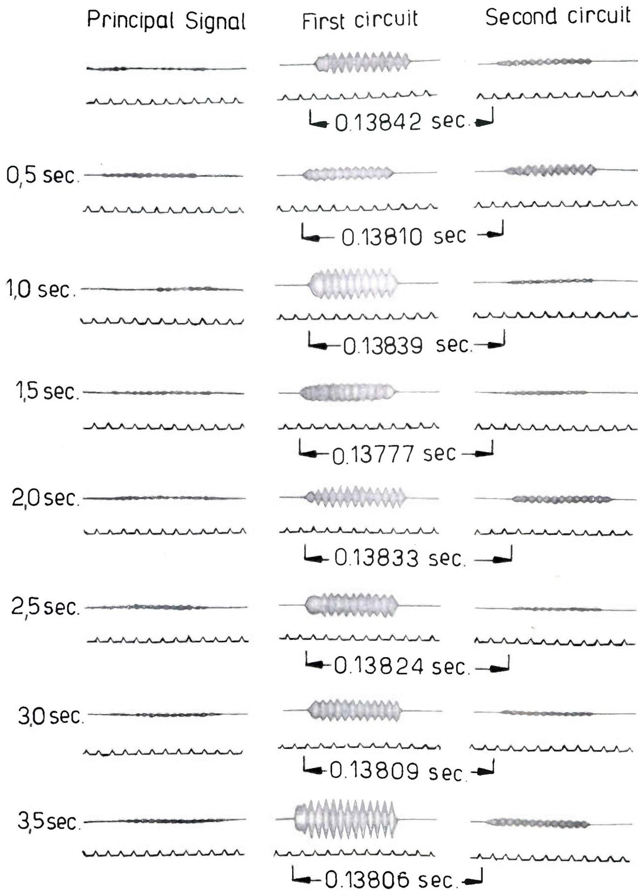
Fig. 1—Recordings made at 0.5-second intervals on DLO, 19,947 kc on November 19, 1944, 0855 GMT, showing detour signals and first and second circuits.
