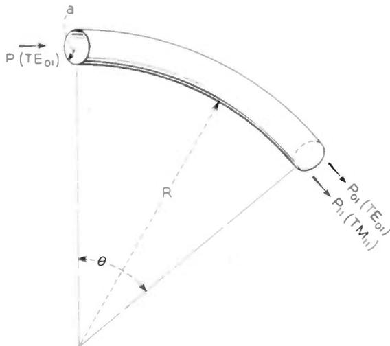
Fig. 1—Round waveguide bent in one plane.
