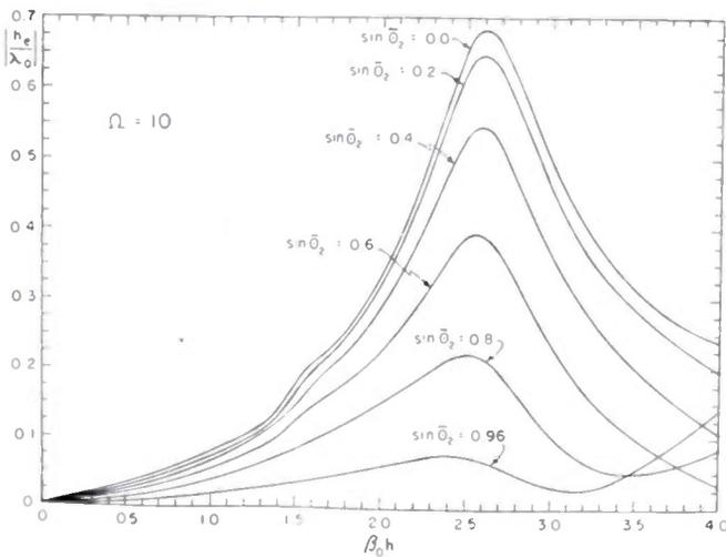
Fig. 4(c)—Magnitude of complex effective length per wavelength;  $\Omega = 10$ .
