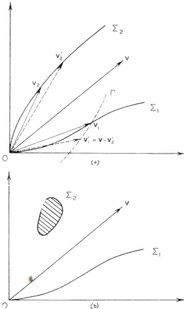
Fig. 3—(a) Case where  $v_1$  can be extracted from  $v_1+v_2$ . (b) Case where  $v_1$  cannot be extracted from  $v_1+v_2$ .
