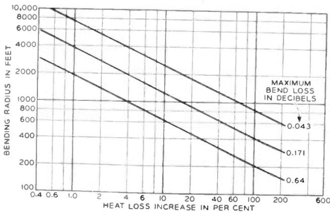
Fig. 11—The allowable bending radius versus the associated increase in  $TE_{01}$  heat loss in elliptic guide, with maximum bend loss as a parameter, for a 2-inch diameter guide at 50,000 mc.
