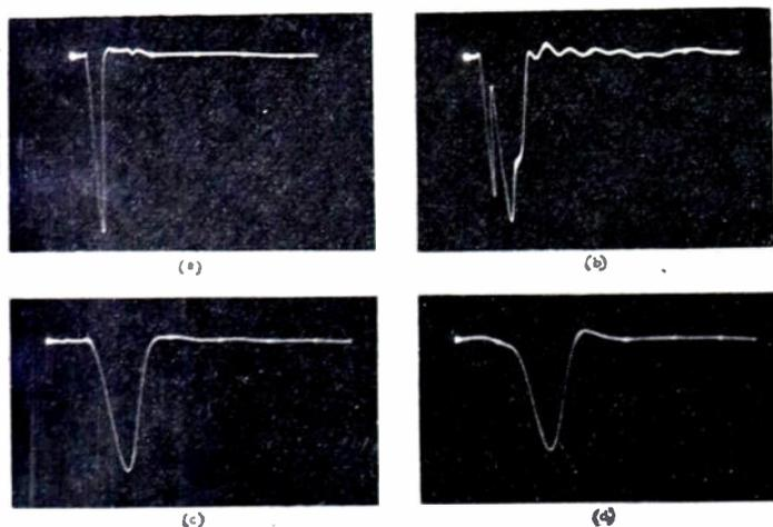
Fig. 5—Transmitter wave shapes— $1 \mu\text{sec}$  timing dots. (a) Plate of modulator tube. (b) Output of filter. (c) Delay-line terminal 4. (d) Delay-line terminal 40.
