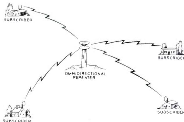
Fig. 9—Use of nonsynchronous system in rural telephony.
