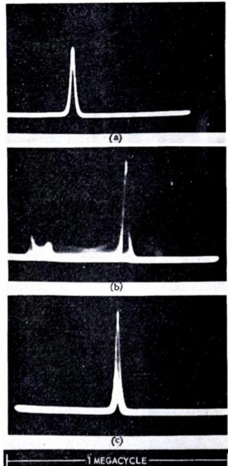
Fig. 1—Spectrograms showing the reduction of frequency pulling of a klystron 723/AB by use of a Pound stabilizer. (a) No crystal modulation; no stabilization. (b) 1,000-cps crystal modulation; no stabilization. (c) 1,000-cps crystal modulation; Pound stabilizer.
