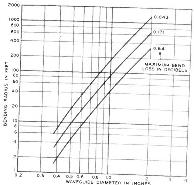
Fig. 13—The allowable bending radius versus guide diameter, with maximum bend loss as a parameter, for elliptic guides of eccentricity  $e=0.3$  and a frequency of 50,000 mc.
