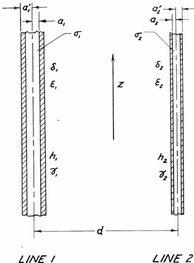
Fig. 1—Two parallel surface-wave transmission lines.
