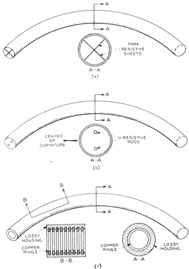
Fig. 20—Structures for negotiating bends using dissipation to prevent  $TE_{01}$  loss. (a) Longitudinal diametral resistive sheets. (b) Longitudinal resistive rods. (c) Closely spaced copper rings in a lossy housing.
