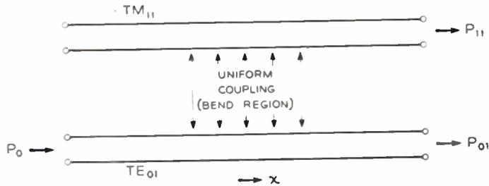
Fig. 4—Coupled transmission-line equivalent of the bent round waveguide.
