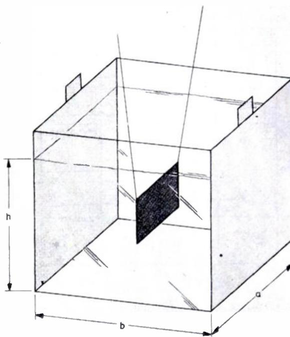
Fig. 1—Electrolytic cell containing a thin nonconducting obstacle.
