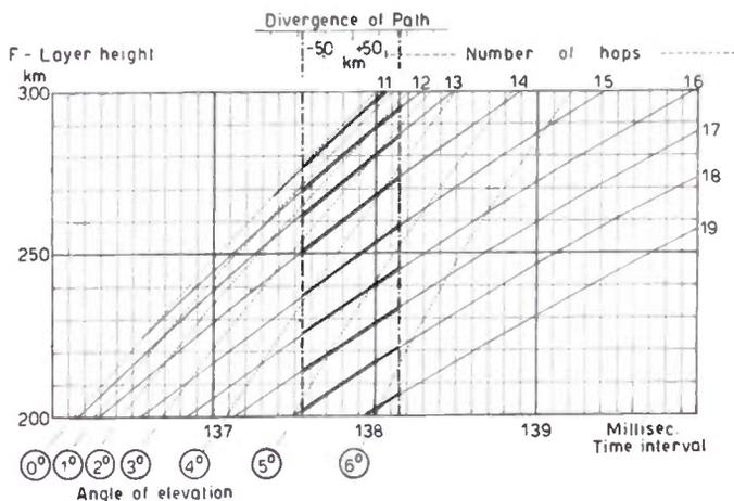
Fig. 4—Time intervals of circuits at 11 to 19 hops between the  $F_2$ -layer and earth's surface, layer-heights 200 to 300 km, and angles of arrival between  $0^\circ$  and  $6^\circ$ .
