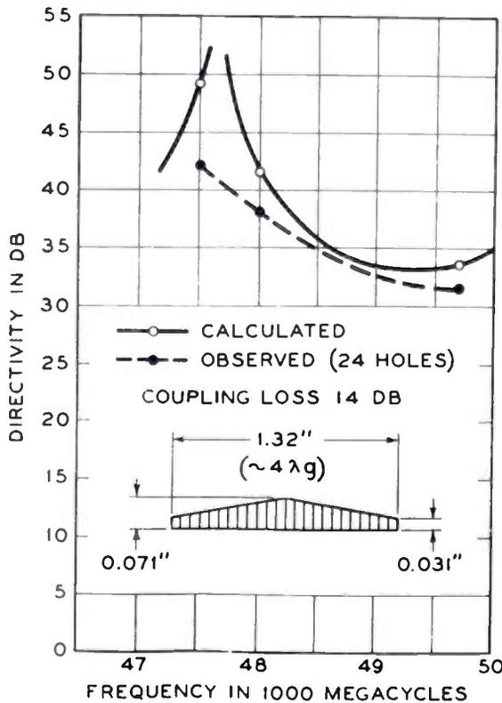
Fig. 16—Observed versus computed directivity for directional coupler of Fig. 15.
