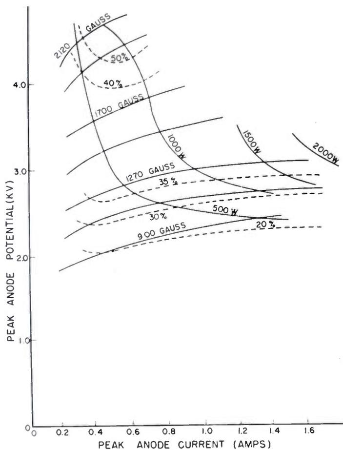
Fig. 5—Performance plot of a single-cavity inverted interdigital magnetron.  $\lambda = 12$  cm. Duty cycle 5 per cent.
