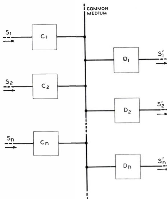
Fig. 1—System in which channels are assigned approximately orthogonal functions of time.
