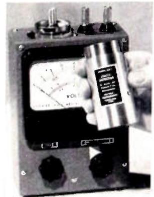
The new electrometer accessory consists primarily of two concentric tubes and an aluminum rod. When clipped over the HI terminal electrode of the electrometer, the tubes provide shielding which gives greater effectiveness to charges along the cylinder axis.
