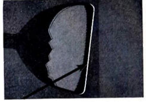
**FOCUS AND DETAIL MAINTAINED!** Tube's outer face is smooth and polished. Consequently, there are no glass-surface irregularities to refract and magnify... as can be the case with etched-face tubes. Viewers see the image in sharpest focus.
