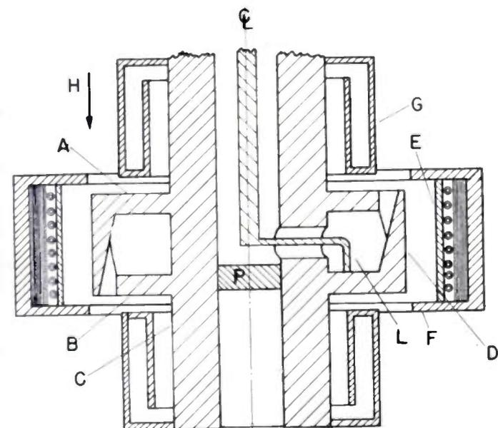
Fig. 1—Cross-sectional view of essential elements of a single-cavity inverted interdigital magnetron. The main vacuum envelope and coaxial output seal are external to all the parts shown.
