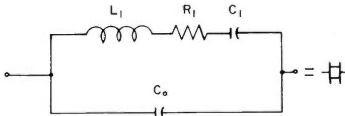
f<sub>r</sub> = series resonant frequency, f<sub>a</sub> = antiresonant frequency
