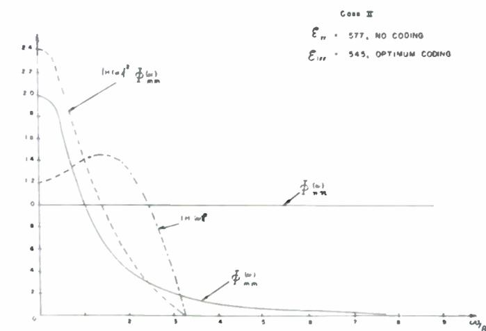
Fig. 3—Power spectra and coding network transfer function; Case II.
