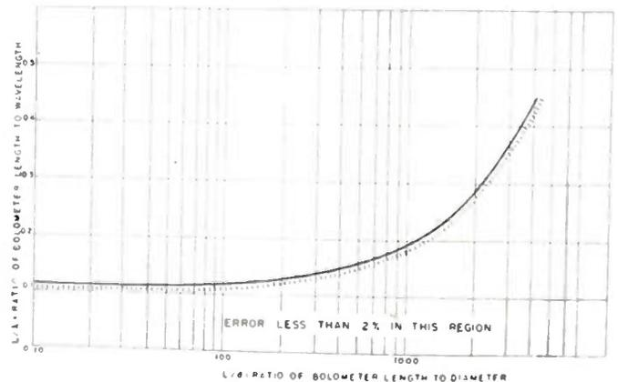
Fig. 8—Maximum permissible  $L/\lambda$  for varying  $L/d$  to limit error arising from metallic conduction and radial convection to no more than 2 per cent. Computed for Wollaston wires, 1 to 3 microns in diameter.
