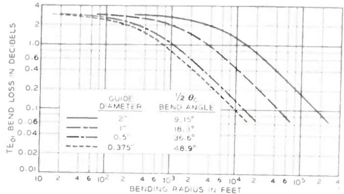
Fig. 22— $TE_{01}$  bend loss versus bending radius for a  $\frac{1}{2} \theta_c$  bend in several round guides operated at 50,000 mc. The reduction in bend loss for large bending radii is due to dissipation in the walls.
