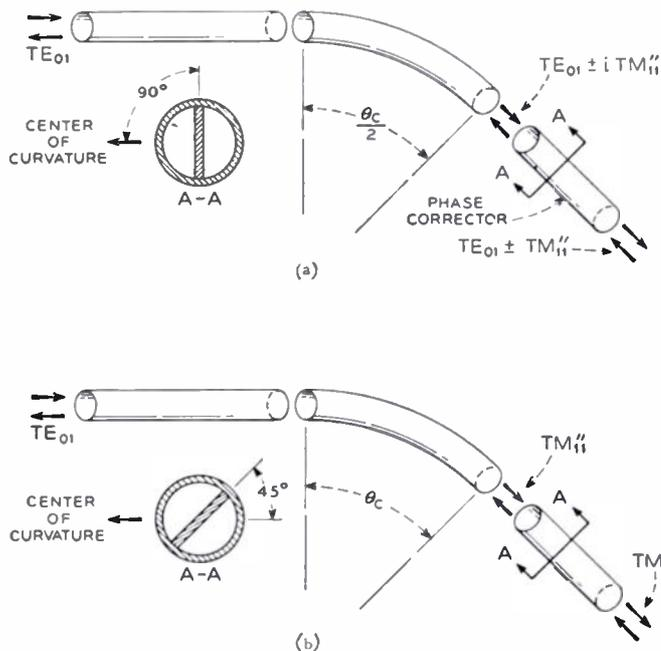
Fig. 16—Mode transducers applicable in the configuration of Fig. 15. (a)  $TE_{01}$  to  $(TE_{01} \pm TM_{11}'')$  mode transducer. (b)  $TE_{01}$  to  $TM_{11}'$  mode transducer.
