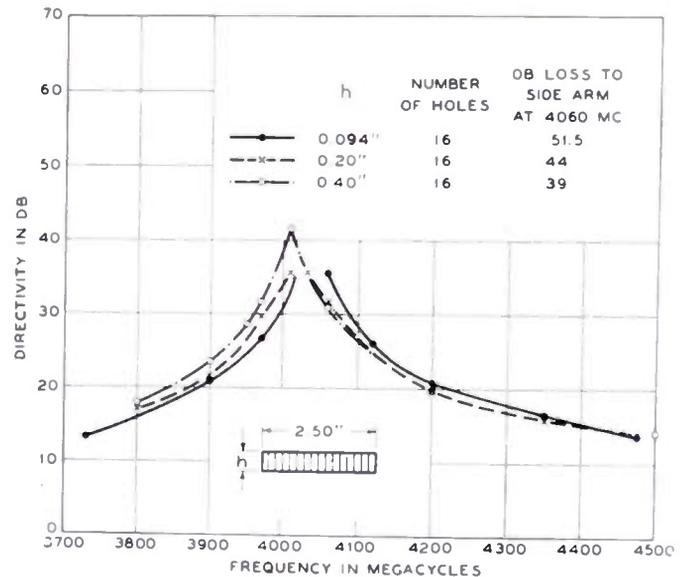
Fig. 9—Observed directivity for constant amplitude coupling when height of slot is changed.
