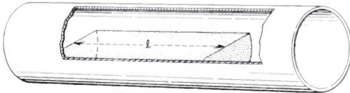
Fig. 17—A  $TE_{01}$  to  $TM_{11}$  mode transducer (due to Morgan).
