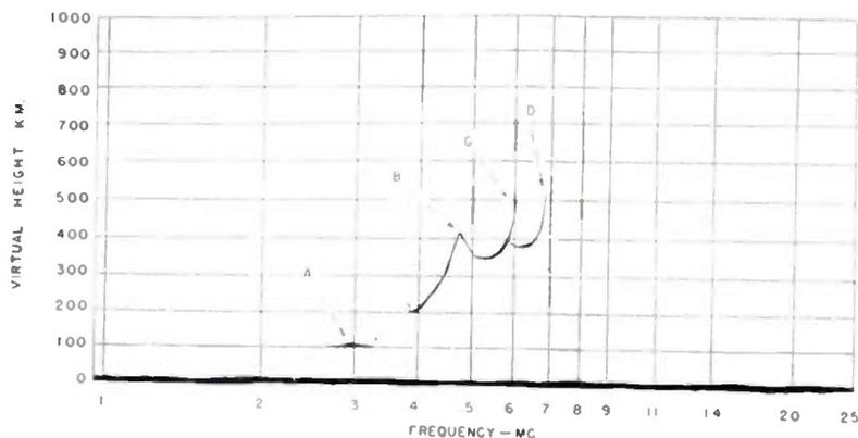
Fig. 2—Corresponding vertical-incidence recordings made at Batavia, Ohio. Both records made on September 4, 1951 at 11:30 A.M.
