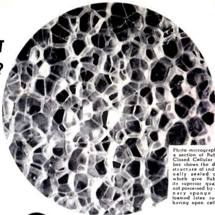
Photo-micrograph of a section of Rubatex Closed Cellular Rubber shows the dense structure of individually sealed cells which give Rubatex its superior qualities not possessed by ordinary sponge and foamed latex rubber having open cells.
