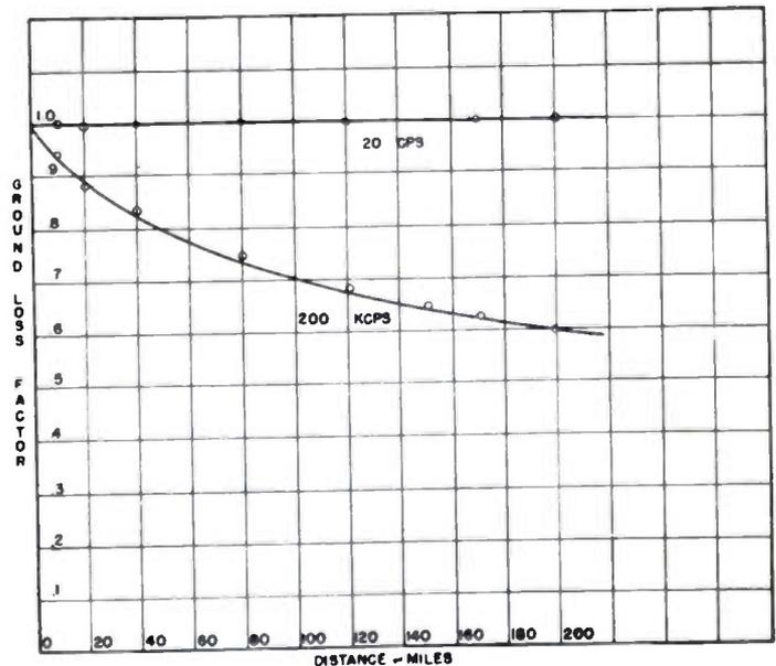
Fig. 1—Ground loss factor versus distance.
