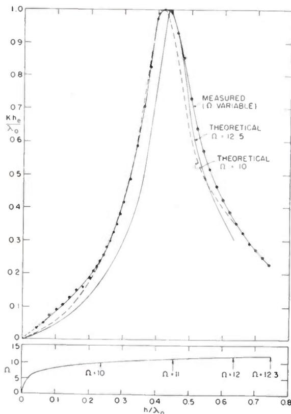
Fig. 9—Normalized effective length of receiving antenna as measured by Morita and Taylor as a function of  $h/\lambda_0$ . Corresponding values of  $\Omega = 2\ln(2h/a)$  are shown together with theoretical curves for the normalized effective length for two values of  $\Omega$ .
