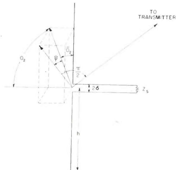
Fig. 1—Center-loaded receiving antenna in linearly polarized field.
