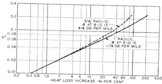
Fig. 10—The increase in  $TE_{01}$  heat loss due to waveguide ellipticity for 1 inch or  $\frac{3}{16}$  inch guide radius and a frequency of 50,000 mc.
