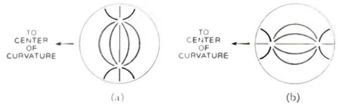
Fig. 2—Electric field directions for the  $TM_{11}''$  and  $TM_{11}'$  modes.
