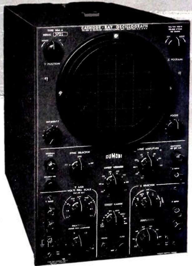
to a minimum. Thus by the inclusion of this new tube and its auxiliary circuitry, an unusually fine, bright trace is achieved, enabling a degree of resolution—and hence a degree of accuracy—heretofore impossible in instruments employing medium accelerating potentials.
