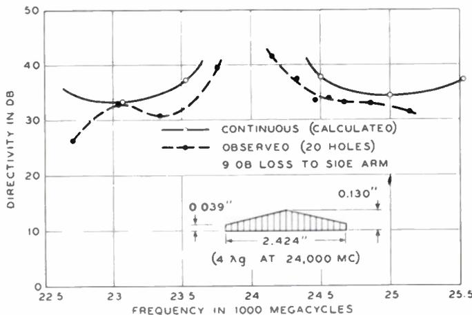
Fig. 14—Observed versus computed directivity for a 24,000-mc directional coupler.
