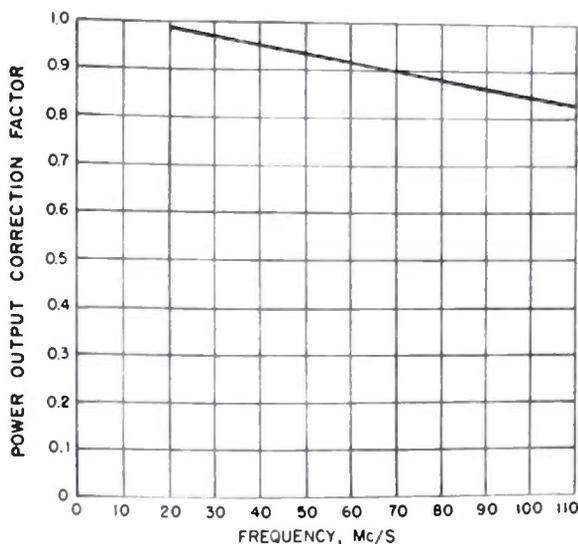
Fig. 3—ML-5681 correction of power output with frequency (transit-time effect).
