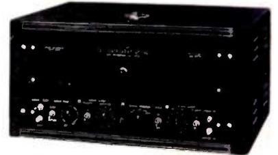
Type 2010 offers: crystal-controlled pulse rates of 200 to 2,000 pps, derived from a 327.80 kc marker crystal by the use of a binary divider system, "Master"- "Slave" operation permitting the use of a number of calibrators for multi-position test systems, narrow and stable 500 yard marker pulses, and a completely regulated power supply for operation from 105-125 v, 100 w 50-60 cps.
