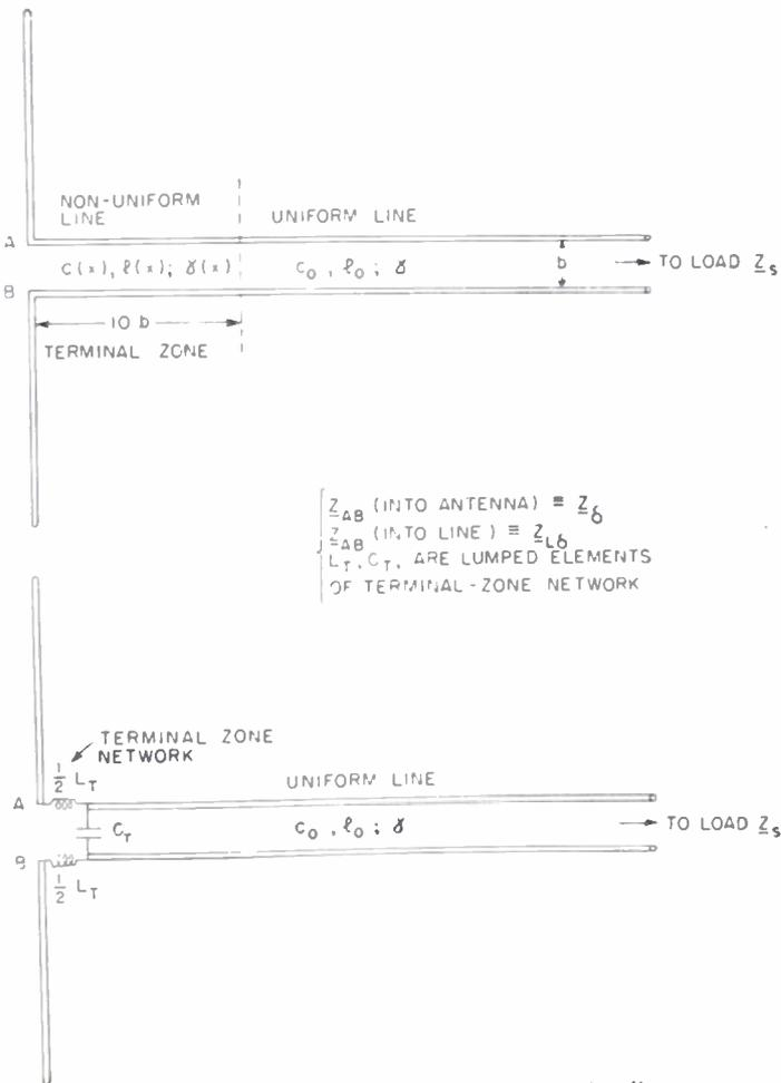
Fig. 2—Actual and equivalent transmission line.
