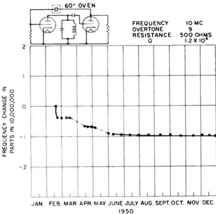
Fig. 2—Aging data taken on a crystal unit, oven, and simple oscillator with reference to the Bell Telephone Laboratories primary frequency standard. An accuracy of 1 part in 10<sup>8</sup> was held for 7 months.
