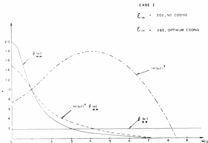
Fig. 2—Power spectra and coding network transfer function; Case I.
