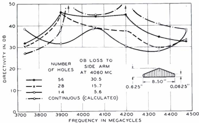
Fig. 13—Observed versus computed directivity for insert of Fig. 12.
