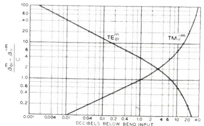
Fig. 7—Bend-output wave amplitudes at the bend angle of maximum conversion versus  $\beta_{01}^m - \beta_{11}''^m/c$ .
