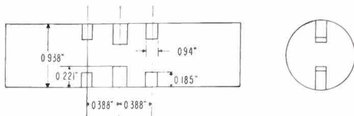
Fig. 3—Waveguide section; schematic, showing calculated dimensions.
