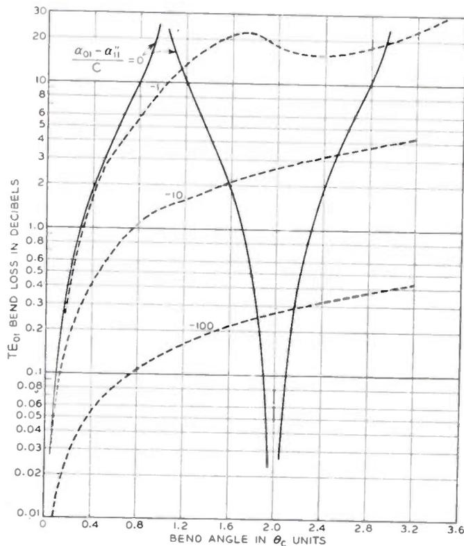
Fig. 21— $TE_{01}$  bend loss versus bend angle, with  $\alpha_{01} - \alpha_{11}$  as a parameter.
