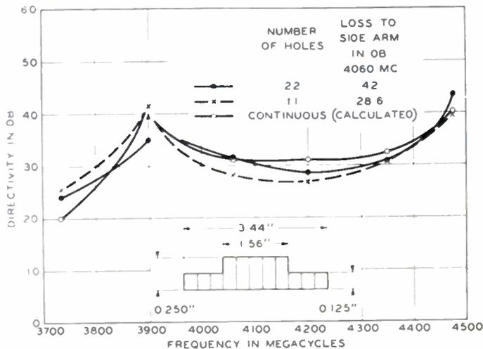
Fig. 11—Observed versus computed directivity for insert of Fig. 10.
