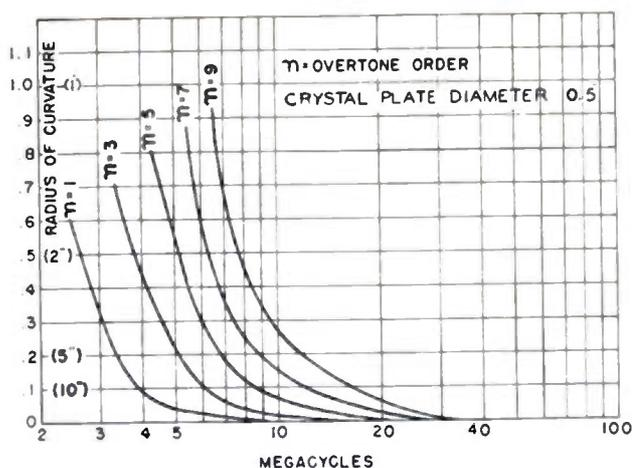
Fig. 7—Typical design chart of the degree contour to obtain minimum series resonant resistance for crystal units 3 to 20 mc and overtones 1 to 9.
