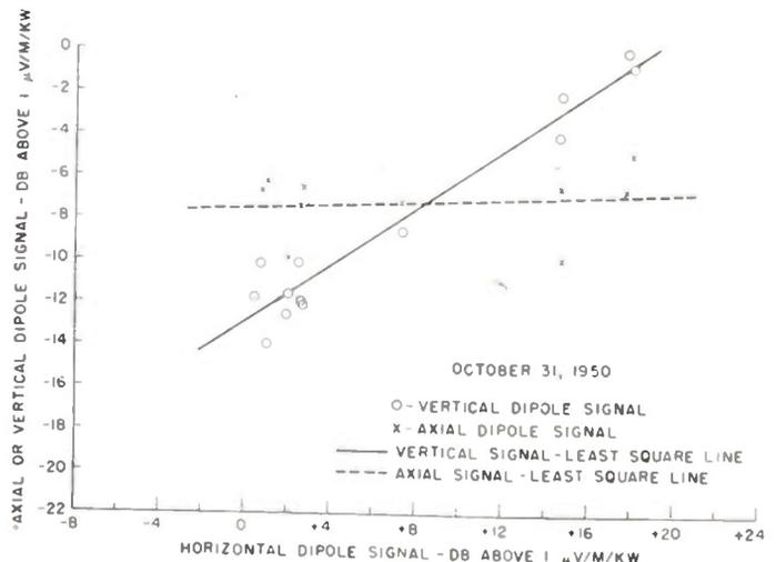
Fig. 5—Axial and vertical dipole components of scattered wave.
