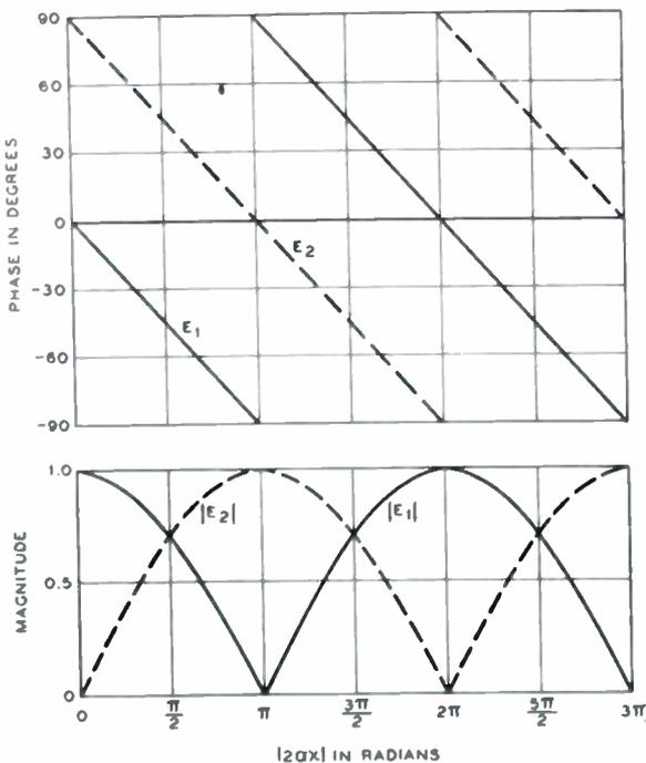
Fig. 19—Amplitude and phase of waves in a tightly coupled directional coupler.
