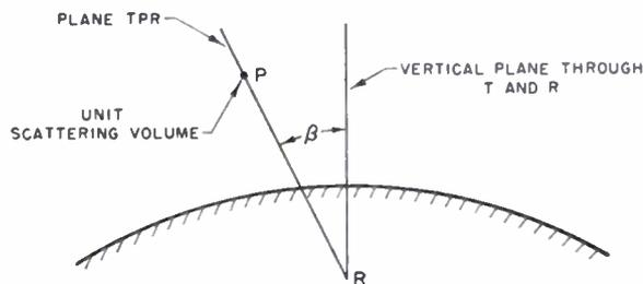
Fig. 2—Scattering geometry with unit scattering volume in plane  $TPR$  tilted at the angle  $\beta$  with respect to the vertical plane passing through transmitter and receiver.
