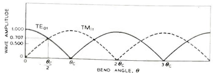
Fig. 3— $TE_{01}$  and  $TM_{11}''$  wave amplitudes versus bend angle.
