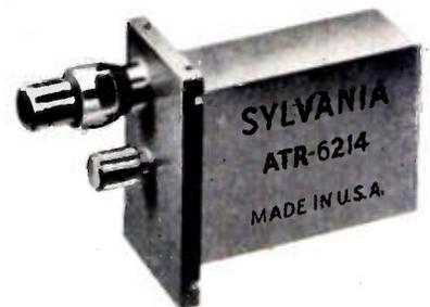
This model, type 6214, developed to meet the special requirements of beacon radar, is capable of instantaneous operation of the first pulse of a coded system of pulses. Conventional ATR tubes often fail to operate immediately when the transmitter starts, thus preventing proper transmission for this period of time, possibly as long as several seconds.
