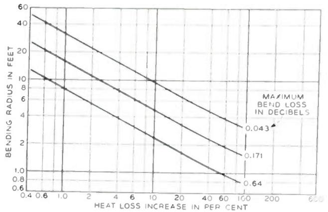
Fig. 12—The allowable bending radius versus the associated increase in  $TE_{01}$  heat loss in elliptic guide, with maximum bend loss as a parameter, for a  $\frac{3}{8}$ -inch diameter guide at 50,000 mc.
