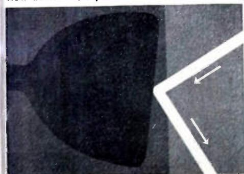
**ROOM LIGHTING IS DEFLECTED DOWN!** Light from ceiling lamps, table lamps, or windows is bent to the floor. Here a G-E Cylindrical is shown from the side in normal tilted mounting position. No light beams reach the viewer's eyes.
