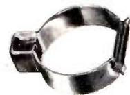
Each trap is stabilized and tested on special equipment designed by Heppner for this specific purpose. Installation time is 2 or 3 seconds. The smooth metal-to-glass contact permits easy adjustment. Model T-312 stays put without wobble or shift during shipment of the completed TV set. It is also light in weight, ¾ ounce, so the tube's neck cannot be harmed. Gauss readings range from 25 to 60.
