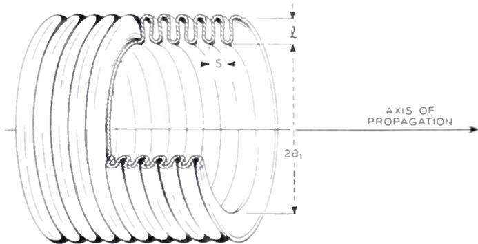
Fig. 14—Flexible waveguide for transmitting  $TE_{01}$  around bends (due to King).
