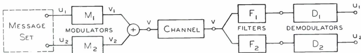
Fig. 1—Functional diagram of a typical two-channel multiplex system.
