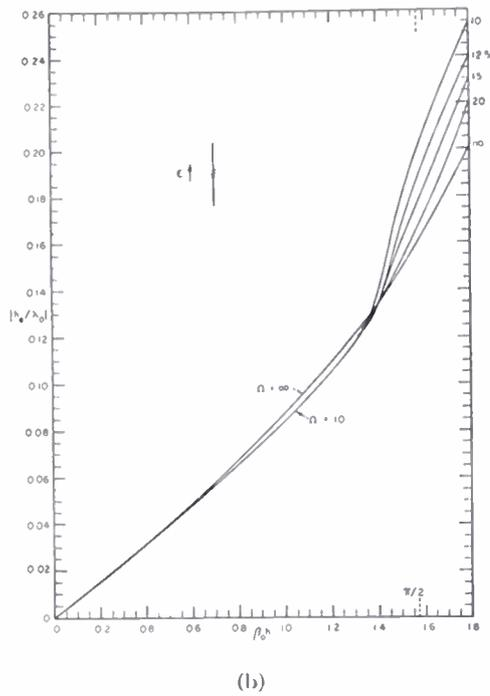
Fig. 6 (a) and (b)—Magnitude of effective length per wavelength for several values of  $\Omega$ .
