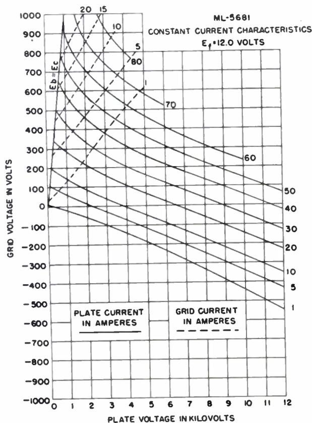
Fig. 6—ML-5681 constant current characteristics.
