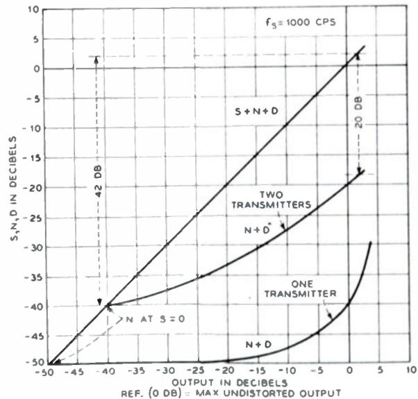
Fig. 8—Signal, noise, and distortion relative to maximum undistorted output. Output in decibels. Ref (0 db) = max undistorted output.
