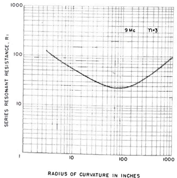
Fig. 6—Variation in series resonant resistance with the degree of contour on a 9-mc, third overtone crystal unit.
