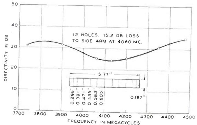
Fig. 17—Observed directivity for tapered amplitude and spacing of coupling elements.
