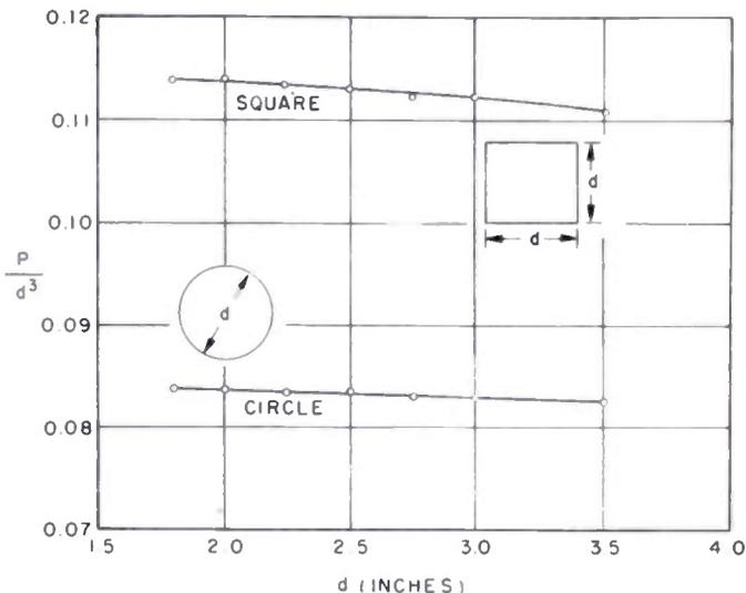
Fig. 2—Measured electric polarizability as a function of size for circular and square obstacles in a 6-inch cubical cell.
