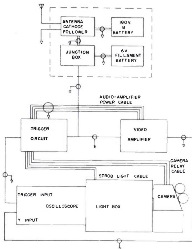
Fig. 2—Cabling diagram for atmospheric detector.
