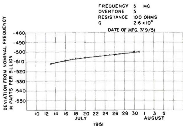
Fig. 3—Aging data taken on a crystal unit alone, showing a change in frequency of about 5 parts in 10<sup>10</sup> per day, 2 weeks after manufacture.
