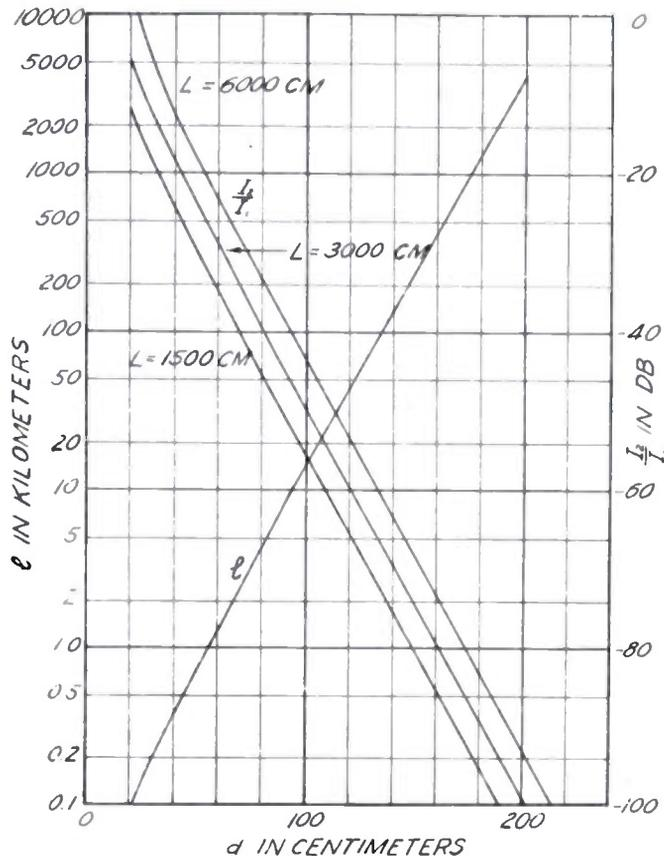
Fig. 3—The propagation distance  $l$  required for complete energy transfer versus separation  $d$ , and the total current ratio versus  $d$  for three line lengths  $L$ .
