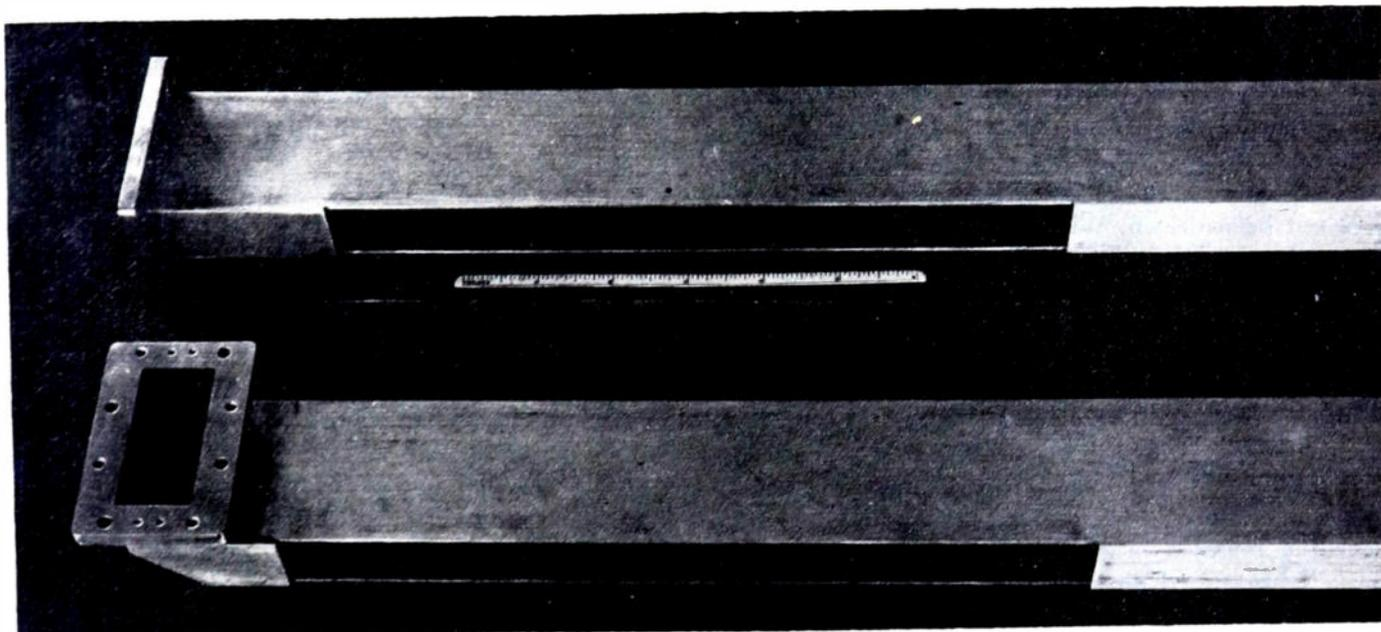
Fig. 5—4,000-mc directional coupler test jig.
