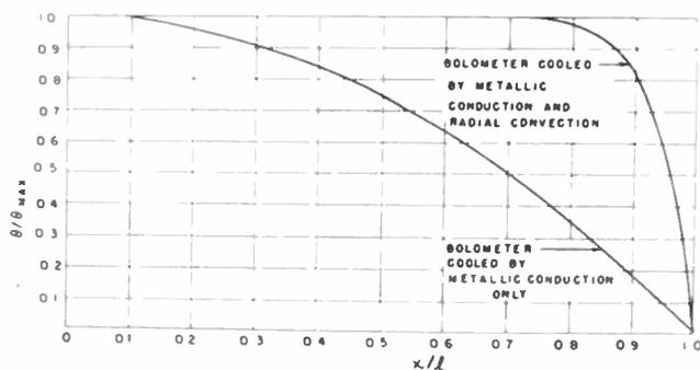
Fig. 3—Calculated temperature distributions for uniformly heated bolometer wires. Fraction of maximum temperature rise above ambient plotted against length co-ordinate expressed as a fraction of half-length  $l$ . Upper curve computed for a Wollaston wire, 1 micron in diameter and 1.5 mm long, in air,  $cl=17$ .
