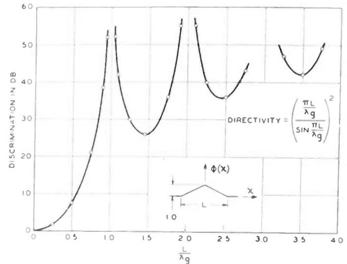
Fig. 3—Computed directivity for linear taper form of coupling.
