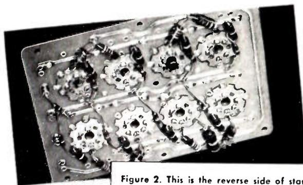
Figure 2. This is the reverse side of stamped circuit shown in figure 1. Both sides of the circuit were stamped in one operation.
