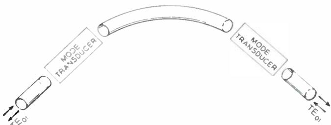
Fig. 15—The normal-mode bend solution.
