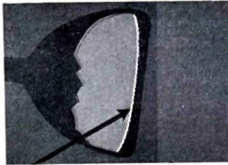
**INTERNAL REFLECTIONS ARE REDUCED!** The inner, or screen face of a G-E Cylindrical is stippled. Stippling wards off reflections, yet permits a picture surface which is fine-grained and uniform. The image has highest quality and rich contrast.
