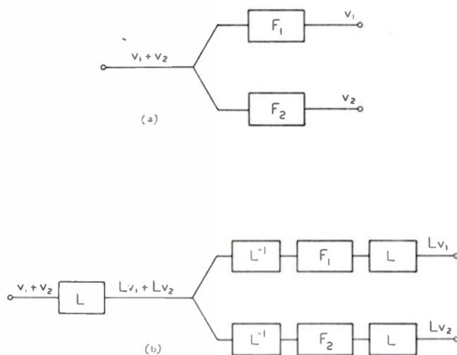
Fig. 4—Linear transformation of a multiplex system.
