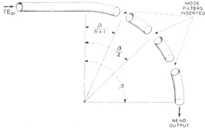
Fig. 18—Sketch for illustrating the effects of mode filters in a bend.
