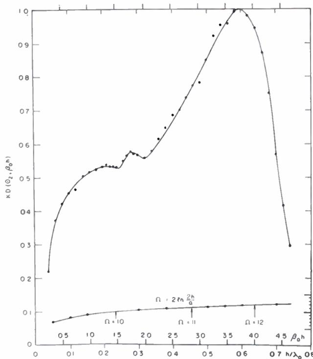
Fig. 12—Measured normalized gain of receiving antenna. Data of Morita and Taylor.
