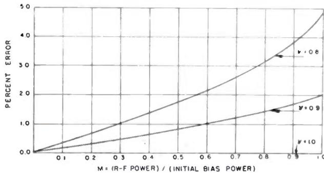
Fig. 6—Calculated resistance-power nonlinearity error as a function of ratio of RF power to initial bias power for triangular distribution of Fig. 5.
