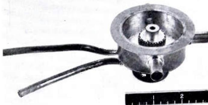
Fig. 3—A partially assembled single-cavity inverted magnetron used for basic study of magnetron space-charge behavior.
