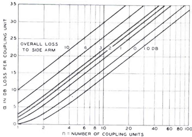
Fig. 21—Chart showing the relation between number of coupling units, loss per coupling unit, and over-all net loss to the side arm in directional couplers.
