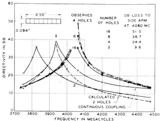
Fig. 8—Observed versus computed directivity for constant amplitude coupling. Number of holes varied from 2 to 16.
