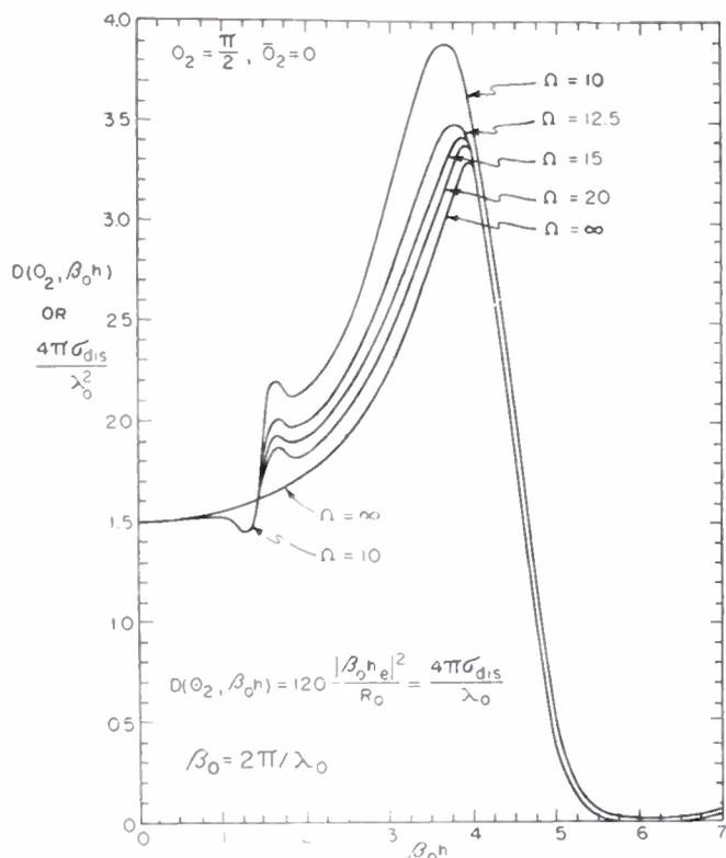
Fig. 10—Gain or directivity of receiving antenna parallel to the incident electric field.
