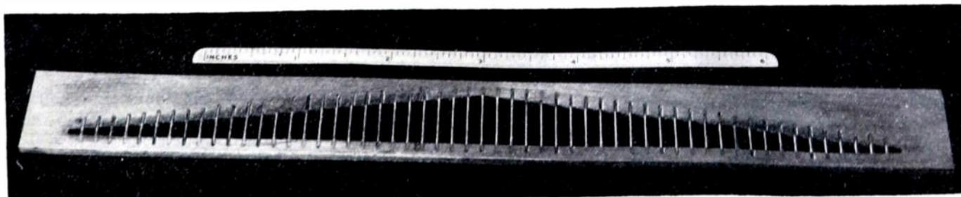
Fig. 12—Insert with linear taper plus constant amplitude coupling.
