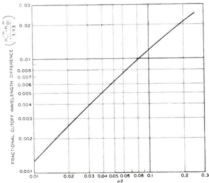
Fig. 8—The effect of eccentricity on the difference between the cutoff wavelengths of  $TE_{01}$  and  $TM_{11}$  in elliptic waveguide.
