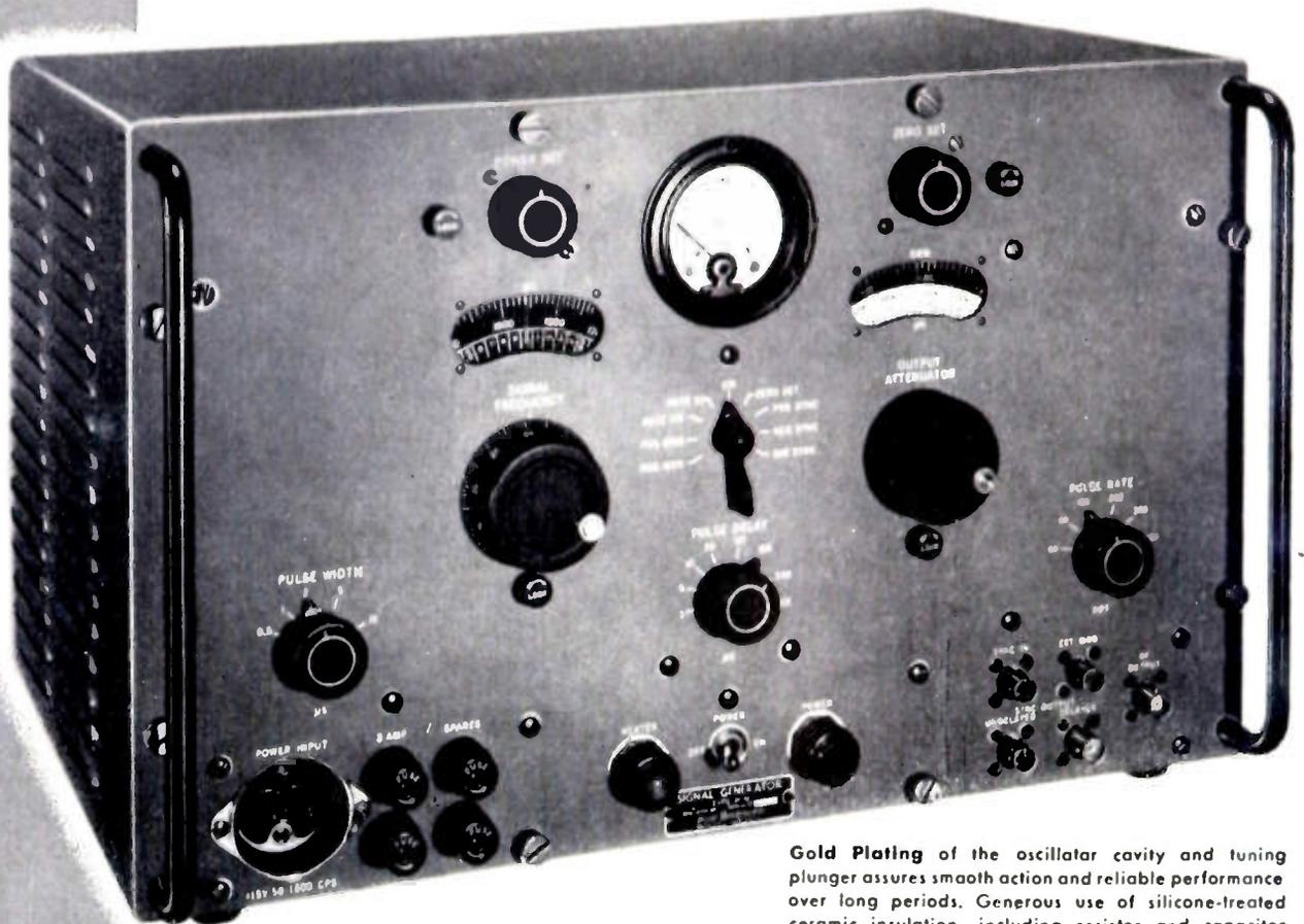
Gold Plating of the oscillator cavity and tuning plunger assures smooth action and reliable performance over long periods. Generous use of silicone-treated ceramic insulation, including resistor and capacitor terminal boards, and the use of sealed capacitors, transformers, and chokes, insures operation under conditions of high humidity for long periods.
