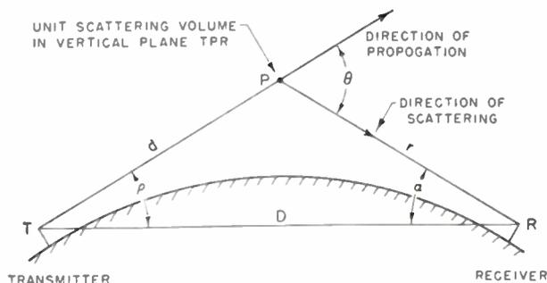
Fig. 1—Scattering geometry with unit scattering volume in a vertical plane passing through the transmitter and receiver.
