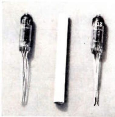
Both of these tubes are suitable for use at frequencies ranging up into the uhf region.
