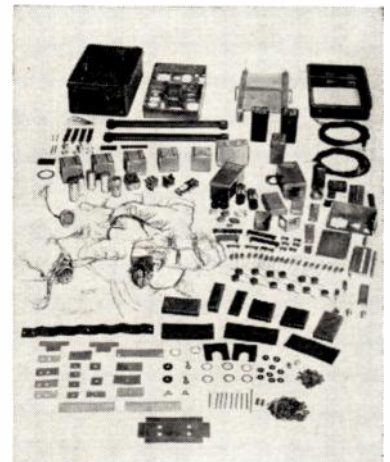
Exploded view of formerly used Vibrator Power Supply PE-237 with its components.
