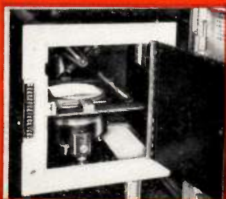
Light source is a special cathode-ray tube designed and built only by Du Mont. Face plate is optically corrected, of medium density and is non-browning. Tube is operated at 45,000 volts on accelerating ring.
