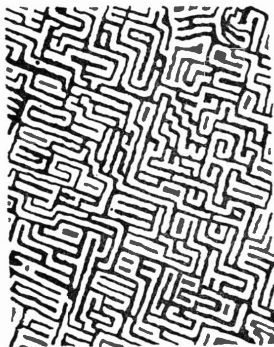
Fig. 2—"Bitter" pattern on the face of a polished single crystal of iron-silicon.
