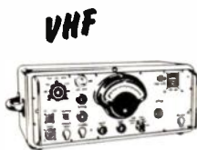
NM-30A, 15mc to 400mc Commercial Equivalent of AN/URM-47. Frequency range includes FM and TV bands.
