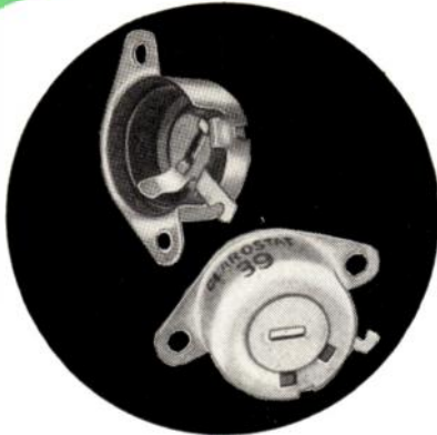
Latest "Humdinger" Series 39. Metal-case mounted with rivets or screws. Mounting surface serves as cover. Semi-fixed setting by screwdriver slipped into rotor slot — no shaft 2-watt 4 to 5000 ohms.
