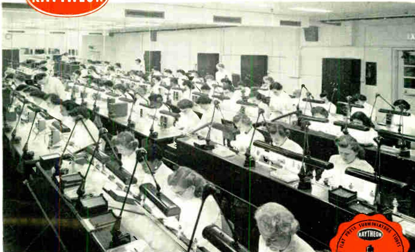
**HOSPITAL-CLEAN** conditions minimize danger of contamination from air borne lint or dust particles that might lead to catastrophic tube failures.
