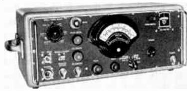
Radio signals or interference, either radiated or conducted, may be measured through the use of accessories which are available for the equipment. Sine wave, pulsed rf, impulsive and random noise may be readily measured. Average, quasi-peak or peak values of complex waveforms can be selected. The NM-30A may also be used as a two-terminal frequency selective voltmeter.
