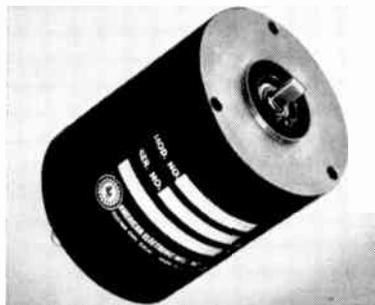
The motor operates on 400 cps. It is excited with 115 v on the fixed phase and 24 v on the control phase. Torque at stall is 2.9 inch/ounces with a power factor at stall torque of 50 per cent. No load speed is 5,100 rpm. Temperature range: -55°C to 90°C. Weight is 13.7 ounces. Additional data is available from the manufacturer.
