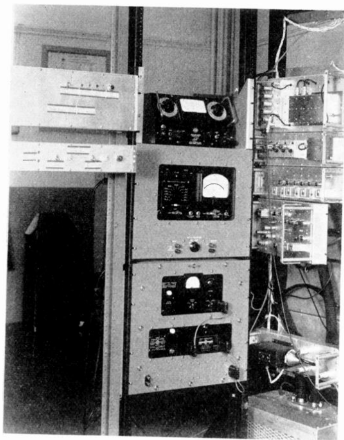
Fig. 7—Fixed frequency noise-loaded intermodulation distortion test set.
