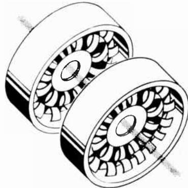
Fig. 22—Schematic of "interlaced" negative mutual structure.
