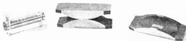
Fig. 2—Details of magnetic structure. Left—Field straightener assembly consists of permalloy disks separated by aluminum spacers. The permalloy disks must be held accurately perpendicular to the axis. Middle—This pair of magnets weighs three pounds. It produces a field of 500 oersteds along the common axis in the 5 3/4-inch gap between polepieces. Right—Single magnet, showing inner contours.
