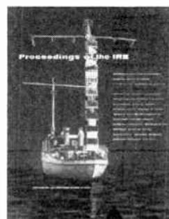
THE COVER—The Natalia, an experimental boat operated by the Hammond Laboratory, was used in 1914-1915 for developing some of the earliest forms of automatic pilot, radio control and target seeking devices. These and other important developments during the early days of radio, which remained undisclosed for many years because of military security, are disclosed for the first time in a paper of unusual historical significance on page 1191 of this issue.
