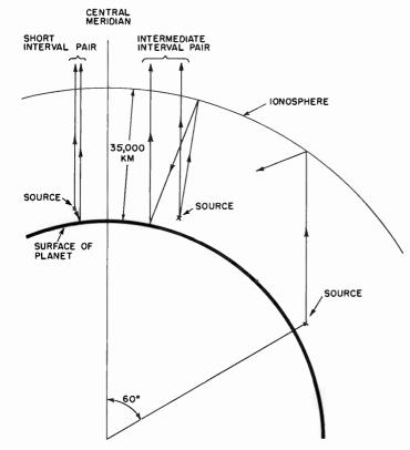
Fig. 10—Diagram illustrating possible wave paths for explaining multiple Jupiter pulses separated by short and intermediate intervals by means of an echo mechanism.
