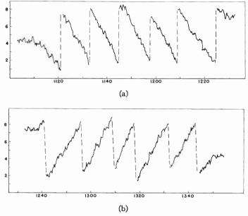
Fig. 2—Recorded output of radiometer during eclipse of June 30, 1954; (a) ordinates—relative power received, (b) abscissas—universal time.
