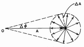
Fig. 17—Vector diagram showing addition of scattered waves to wave from source.
