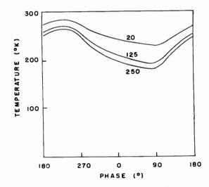
Fig. 9—Calculated microwave temperatures for a solid with a surface skin, for which  $D = C = \sqrt{2\pi}$ . The numbers on the curves are the values of  $(K\rho c)^{-1/2}$  for the substratum. (Jaeger, Aust. J. Phys.)
