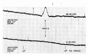
Fig. 3-Record of radio source Virgo A taken with 12 helices (lower trace) and with 96 helices (upper trace) showing improvement resulting from 8-fold increase in antenna aperture.
