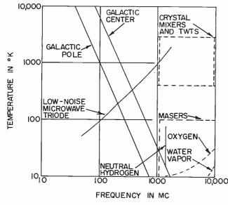
Fig. 5-Background and receiver noise vs frequency.
