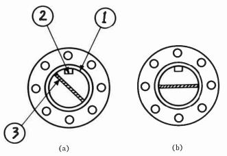
Fig. 6-Radiation source for the calibration of sensitivity-1) Circular waveguide, 2) phase shifter, and 3) lossy plate.
