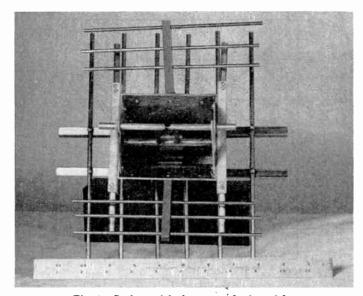
Fig. 1—Scale model of antenna feed used for primary pattern measurements.
