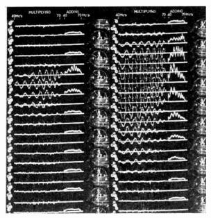
Fig. 5—Two typical records of Type III bursts obtained on July 3, 1957. As indicated by the clock, time advances vertically downwards. Patterns of the multiplying interferometer are displayed at one-second intervals, and those from the adding interferometer at two-second intervals.
