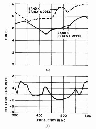
Fig. 4(a)—Noise figure of two Band C receivers. (b)—Relative gain of Band C receiver as a function of frequency.
