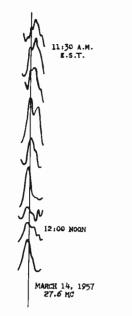
Fig. 12—Three-helix lobe-sweeping array patterns obtained during transit of source on March 14, 1957. Horizontal chart width corresponds to lobe displacement of 20° either side of meridian (vertical line). East of the meridian is to the right and west to the left.
