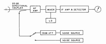
Fig. 2-The block diagram of the 440-mc receiver.
