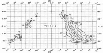
Fig. 11—Map of the radio sky background at 600 mc (after Piddington and Trent<sup>20</sup>). The contours give the absolute brightness temperature of the radio sky in degrees Kelvin.
