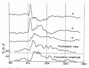
Fig. 14—Lerwick magnetogram April 1-2, 1955. Cassiopeia fluctuations. The fluctuation rate is the number of maxima per minute. The fluctuation amplitude is expressed as a percentage of mean source intensity.
