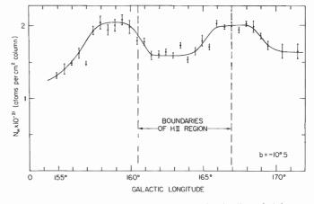
Fig. 3—Number of neutral hydrogen atoms in the line of sight per square centimeter column as a function of galactic longitude at  $b = -10.^{\circ}5$ .
