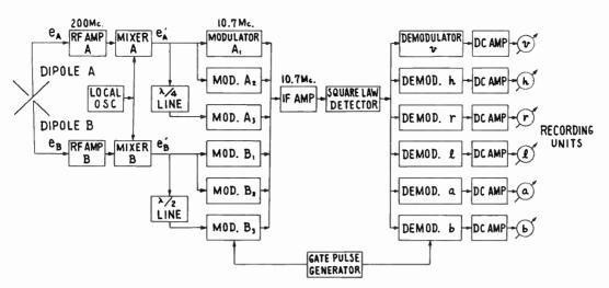
Fig. 1—Block diagram of the circuit.
