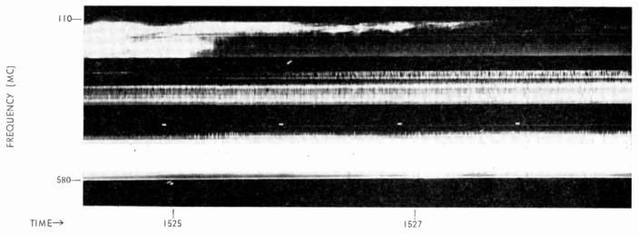
Fig. 8—Continuum: September 12, 1957. This is a small section from the record of a great solar radio outburst, which was associated with a class-2+ flare (beginning 1510, maximum 1517.5, end 1550 U.T.; intensity 35, which is the maximum; 20° W, 12° N). The continuum started at 1517 U.T., two minutes after the outburst commenced. Here it covers the range 180-580 mc and is gradually drifting downward in frequency. The end of a slow-drift burst can be seen on the low-frequency receiver, 100-180 mc.
