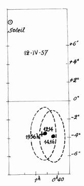
Fig. 5—Relative positions of the sun and the comet on April 12, 1957. The contours of antenna lobes are given. The cross indicates the position of the comet, after Candy's ephemeris. The black circles are the lobe centers for observations recorded in Fig. 4.
