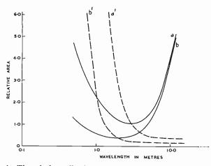
Fig. 4-The relative collecting area required for a constant snr on a typical source at different wavelengths. The solid curves refer to an unresolved source, the dotted curves to an extended source. (a) Curves based on the use of a 6AK6 cascode preamplifier and 50 per cent efficiency. (b) Curves based on the best available modern techniques.
