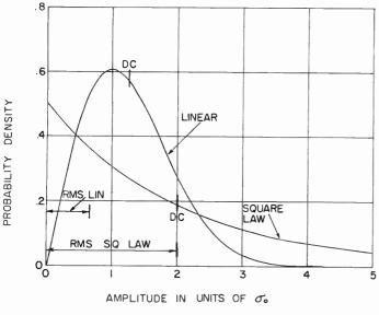
Fig. 8—Probability densities of detected output voltage for linear and square-law detectors.
