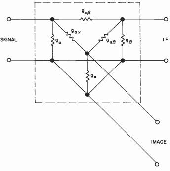
Fig. 3—Equivalent circuit of a crystal mixer.
