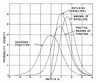
Fig. 7—Probability densities of several features of random noise that has been passed through a narrow band-pass filter.
