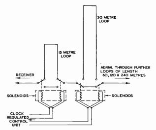
Fig. 7—Diagrammatic plan view of two sections of the variable line, in which only one of the two wires of each radio frequency line is seen. The complete line can be varied from 0 to 480 m in steps of 15 m.
