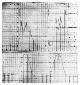
Fig. 3—Drift curves of the sun; above: moderately active; below: quiet.
