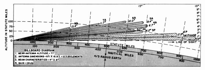
Fig. 2-Sea interferometer lobe pattern produced by reflections from the sea.
