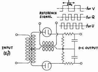
Fig. 5-Mixer for coherent detection.
