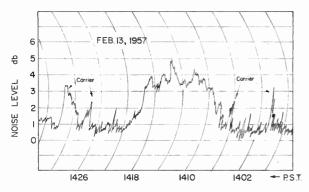
Fig. 3—Penmotor recording of the radio noise source Cassiopeia as it transists the 13-meter array beam, taken February 13, 1957. Each four-minute division represents one-half degree.
