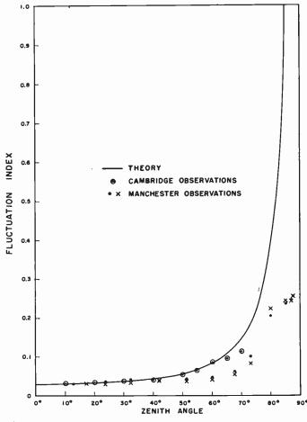
Fig. 19—Comparison between a theoretical curve for the zenith angle dependence of fluctuation index and observations made at Cambridge and at Manchester.
