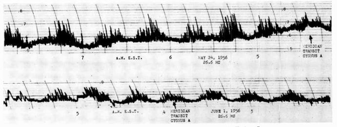
Fig. 4-Interferometer lobe patterns of Cygnus A showing large scintillation effect.
