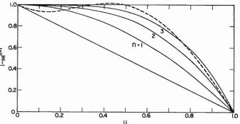
. 2—Spectral factors corresponding to different stages of restora-tion by successive substitutions. The broken line refers to the Fig. 2chord construction.
