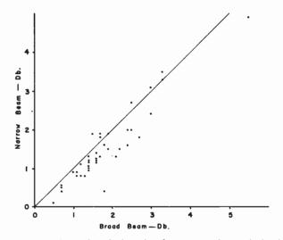
Fig. 6—Peak absorption during singular events observed simultaneously on broad- and narrow-beam antennas at College. The straight line is that of equal absorption on the two antennas.
