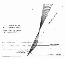
Fig. 4-Ray tracing for the narrow-beam case.
