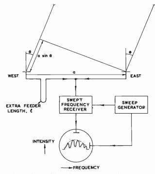
Fig. 1—The principle of the swept-frequency interferometer.
