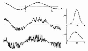
Fig. 4—Observations of the intensity fluctuations of source 23.01 made with a phase-switching receiver on 6.7 m. The probability distribution of amplitude p(A) deduced from the records is shown on the right.
