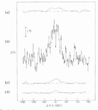
Fig. 5—Summary of the measurements of planetary radiation. (a) Average of eleven drift scans through Venus made at a wavelength of 9.4 cm. (b) A reproduction of the output trace of the 3.15-cm radiometer as Venus drifted through the beam on June 17, 1956. (c) Average of forty-five drift scans through Jupiter made at 3.15-cm wavelength. (d) Average of seventy-one drift scans through Mars made at 3.15-cm wavelength.
