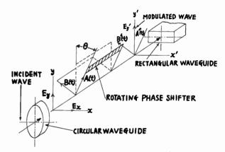
Fig. 1-Principle of phase modulation.
