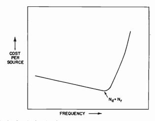
Fig. 2-Graph of radio telescope cost per observable radio source as a function of frequency. The minimum cost occurs at or close to the frequency for which the number of sources which can be detected  $(N_d)$  is equal to the number which can be resolved  $(N_r)$ .
