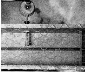
tions, 10 in all, are joined through manually-operated variable phase shifters and relay-operated stepped phase shifters. The former are used to correct phase errors which might occur along each line section, the latter for changing the declination in small discrete steps.
