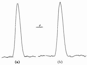
Fig. 3—A comparison between (a) the computed E-W response curve of the instrument and (b) the response to the transit of the radio source Hydra A (IAU 09S1A).
