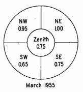
Fig. 3—Median values of the ratio of absorption to that in the NE direction for the zenith, and NW, SE, and SW directions, based on twenty-two events in March, 1955.
