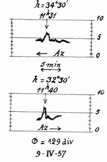
Fig. 2—Deviation obtained on the comet's region on April 9, 1957. In the upper figure the antenna beam has the same direction as the diurnal motion; in the lower figure, the opposite.
