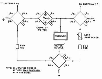
Fig. 1—Interferometer details. (Same as Fig. 1, J. Geophys. Res., vol. 61; September, 1956.)
