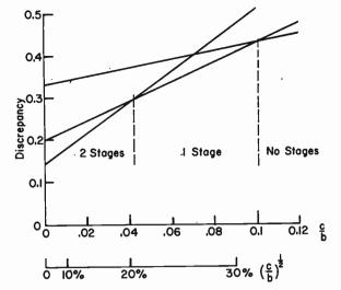
Fig. 3—How the discrepancy depends on the error level for different stages of restoration by successive substitutions.
