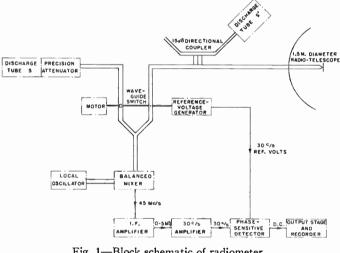
Fig. 1-Block schematic of radiometer.
