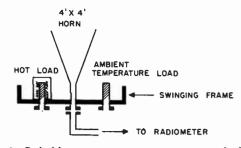
Fig. 3—Switching arrangement at antenna terminals for measurement of sky temperature.
