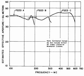
Fig. 7-Estimated effective aperture of antenna system.
