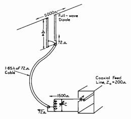
Fig. 6—The schematic feed arrangement for the full-wave dipoles in the N-S array.
