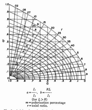
Fig. 2—Axial ratio and polarization percentage vs ratios of circular components.
