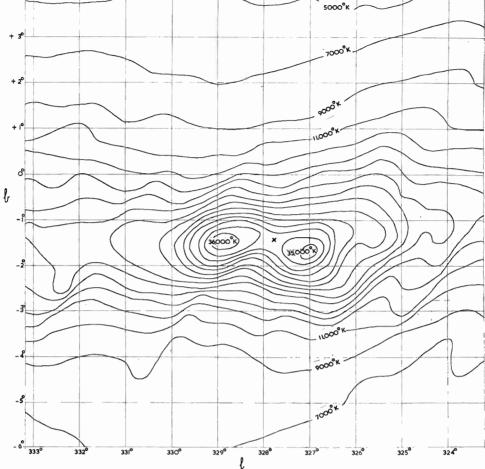
Fig. 17—An example of a brightness temperature contour diagram near the galactic center. The cross near the middle of the diagram indicates the position of a strong source observed at short wavelengths in the direction of the galactic center. At 3.5 m the source corresponds with an area of absorption, suggesting that it is a region of ionized hydrogen.
