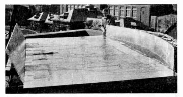
5-Scale model operating at one-cm wavelength built to test performance of standing parabolic reflector type antenna.
