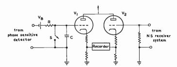
Fig. 15—A simplified circuit illustrating the recording method used when scanning the pencil beam.
