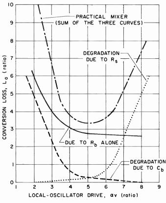
Fig. 4-Conversion loss vs local oscillator drive.
