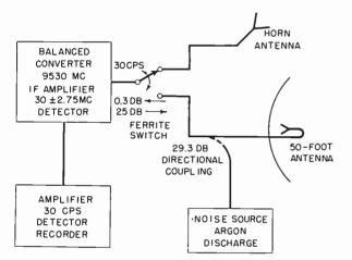
Fig. 1-Block diagram of 3.15-cm radiometer.
