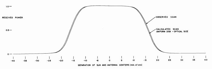
Fig. 7.-The observed 4.3-mm sun scan compared to a calculated scan for a uniform sun equal in diameter to the optical disk.
