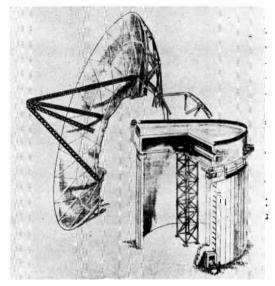
Fig. 3—General side elevation of 140-foot altazimuth telescope proposed by D. S. Kennedy Company of Cohasset, Mass.
