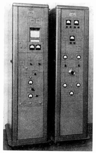
Fig. 3—Photograph of phase tracking interferometer receiver showing front panel engraving, meters, controls, and test points.
