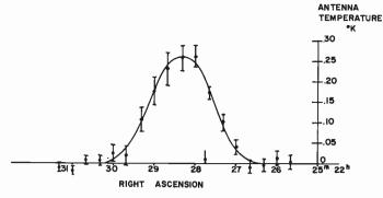
Fig. 9-Mean of 5 observations of NGC 7293, with probable errors of the observed points indicated. The mean probable error is 0.022°K; the arrow indicates the optical center of the nebula.
