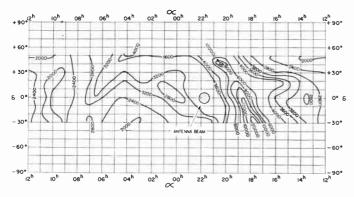
Fig. 5—Map of the radio sky background at 64 mc (after Hey, Parsons, and Phillips<sup>12</sup>). The contours give the absolute brightness temperature of the radio sky in degrees Kelvin.
