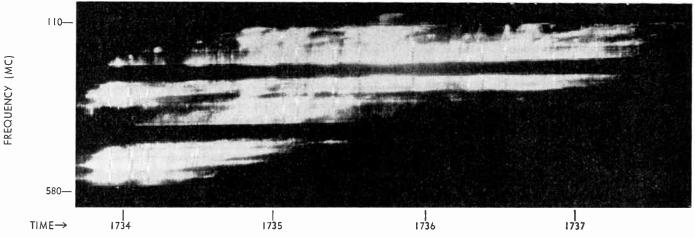
Fig. 4—High intensity slow-drift burst: January 7, 1957, commencing 1733.7 U.T. This burst, which is shown in its entirety, was completely isolated in time from any other activity. Unfortunately, there were no visual observations of the sun at that time.
