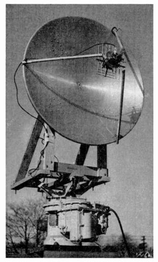
Fig. 3—Scale model of reflector and feed used for secondary pattern measurements.
