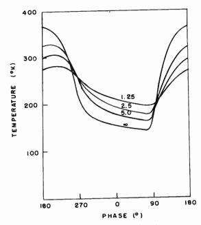
Fig. 8—Calculated microwave temperatures for a homogeneous lunar surface for which  $(K\rho c)^{-1/2} = 125$ . The numbers on the curves are the values of  $C = \alpha_m (KP/\rho c)^{1/2}$ . (Jaeger, Aust. J. Phys.)
