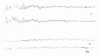
Fig. 7—Simultaneous record of solar scintillations with two antennas at distance D: a) D=60 m; good correlation ( $\rho=0.88$ ), b) D=460 m; no correlation ( $\rho=0.05$ ).
