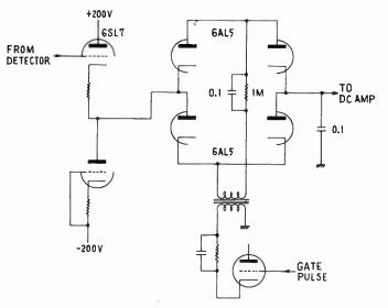
Fig. 4-Construction of the time demodulator.
