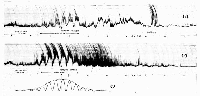
Fig. 2—(a) Record of 11-meter solar radiation on August 31, 1956, at and following a large solar flare. The large deflection labeled "outburst" occurred close to the time of the flare. (b) Record of solar noise on August 30, 1956. (c) Interferometer antenna lobe pattern with envelope (dashed).
