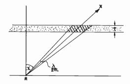
Fig. 18-Illustrating calculation of amplitude fluctuations.
