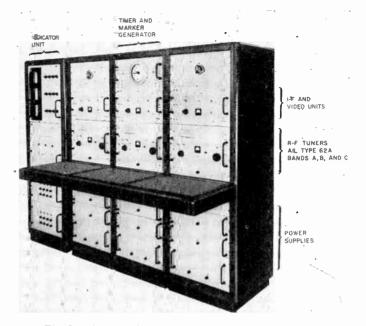
Fig. 2-Photograph of the dynamic spectrum analyzer.
