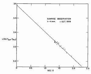
Fig. 4—Plot of log  $(T_{sun} - T_{sky})$  vs sec z for October 1, 1956.
