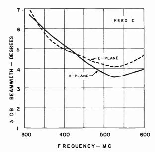
Fig. 6-Secondary pattern beamwidths for Feed C.
