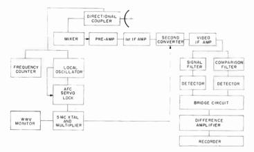
Fig. 1—Block diagram of NRL hydrogen radiometer. The receiver is an L band radiometer employing a crystal mixer and double conversion. Signal and comparison bands provide a comparison of the spectral intensity received by the antenna in two regions of the spectrum. A stable local oscillator is tuned in frequency, translating the signal and comparison bands through the spectrum. The difference in energy received in the two bands is presented at the recorder.
