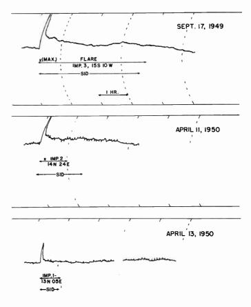
Fig. 9—Examples of 2800-mc radiation at the time of flares for which there was no distinctive event at 200 mc. Cross indicates time of flare maximum.
