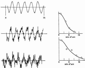
Fig. 1—Cassiopeia fluctuation records taken simultanoeusly by two receivers 11 km apart on a north-south base line. Records A: Correlation 0.9 (effective base line 4.1 km). Records B: No correlation (effective base line 7.7 km).
