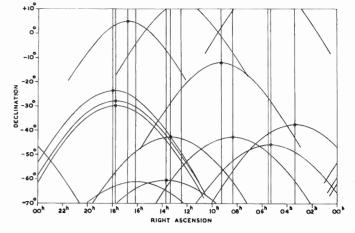
Fig. 16-The disposition of the "lines of interference;" the strong sources indicated by dots on the diagrams may produce spurious responses along these lines.
