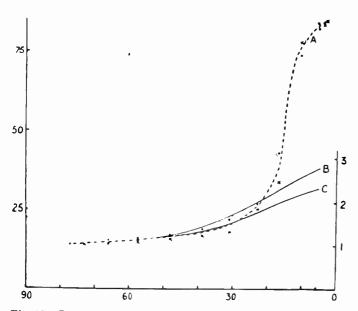
Fig. 12—Curve A: Amplitude of Cygnus fluctuations with elevation Xsource setting, ·source rising (averages over 12 months). Curves B and C: Ratio of effective thickness of disturbing region in line of sight to zenith thickness—(Curve B for a disturbing region of assumed minimum height 300 km and maximum height 500 km; Curve C for assumed minimum height 250 km and maximum height 1000 km).
