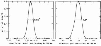
Fig. 6-Measured patterns of model standing parabolic reflector an-tenna. The half-power beamwidth is 0.26° (16 minutes of arc) in the horizontal plane and 1.9° in the vertical plane.
