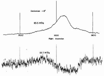
Fig. 4—Variation of brightness during a sweep across the Milky Way at declination  $-12^{\circ}$ . The upper record is at 85.5 mc and shows the sharp ridge characteristic of such records at this frequency. The lower record shows the trough observed at 19.7 mc due to interstellar absorption.
