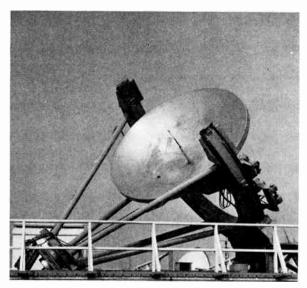
Fig. 1-Receiving system for cosmic radiation at 35 kmc.
