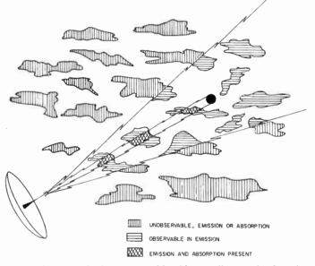
Fig. 4—Antenna viewing an assembly of interstellar gas clouds and a radio star included within the beam. Two beams are evident: the cone subtended by the radio star, and the cone defined by the beam of the antenna. Emission and absorption effects are indicated in the figure.
