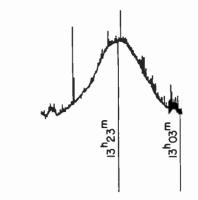
Fig. 4—A drift curve of the source, Centaurus A. The long vertical lines are time markers. The right ascensions to which the antenna was pointed at the times are indicated.
