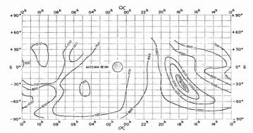
Fig. 7—Map of the radio sky background at 100 mc (after Bolton and Westfold<sup>16</sup>). The contours give the absolute brightness temperature of the radio sky in degrees Kelvin.
