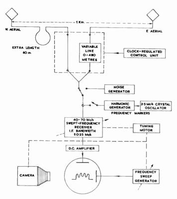
Fig. 3-The adding interferometer.
