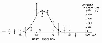
Fig. 11-Mean of 4 observations of NGC 6853, with probable errors of the observed points indicated. The mean probable error is 0.017°K; the arrow indicates the optical center of the nebula.
