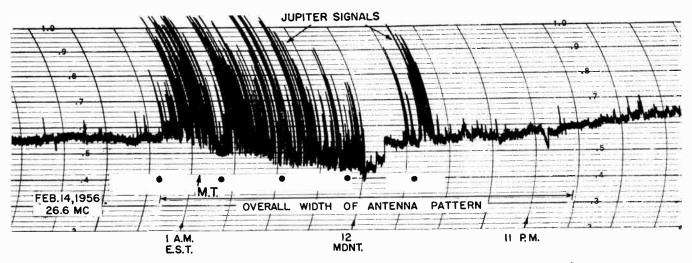
Fig. 5-11-meter Jupiter noise recorded February 14, 1956, at a tape speed of three inches per hour.
