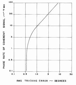
Fig. 6—Curve of rms tracking error angle as a function of rate of change of coherent signal phase at the two receiver inputs. Predetection bandwidth of 500 kc, a postdetection integration time constant of 0.2 second, a unity ratio of power gain in the two receiver channels and a ratio of input signal temperature to background plus excess receiver noise temperature of 0.05.
