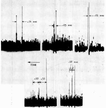
Fig. 8—Cathode-ray oscillograms of 11-meter Jupiter multiple pulses or cracks showing three pulse pairs and two triplets. The pulse separation is given in seconds. Photograph partly retouched for clarity.
