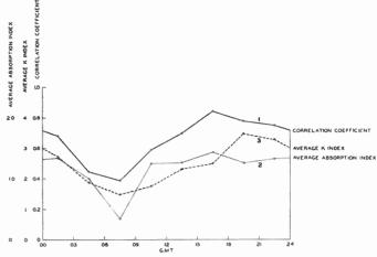
Fig. 20—Diurnal variation of the absorption at College and K index at Sodankylä. Curve 1 shows the diurnal variation of correlation between K(Sodankylä) and absorption(College). Curves 2 and 3 show the mean diurnal variations of K(Sodankylä) and absorption(College).
