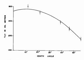
Fig. 13—The effective total area of the arrays (including ohmic losses) as a function of zenith angle. The solid curve is theoretically derived and fitted to the measured areas indicated by dots; the vertical "wings" indicate the probable errors of the measured points.
