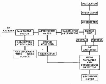
Fig. 2-Diagram of 4.3-mm radiometer.
