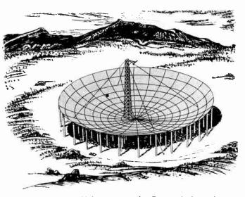
Fig. 9—Proposed 500-foot antenna for Cygnus A absorption measurements. This antenna is discussed in the text.
