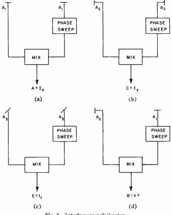
Fig. 5—Interference polarimeter.
