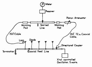
Fig. 8—The phase and amplitude comparator used in adjusting the dipole currents.
