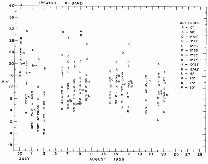
Fig. 12-Daily range of refractive errors 9375 mc.
