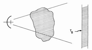
Fig. 3—Antenna viewing an interstellar cloud illuminated by a continuum source. The spectrally-emitting cloud fills the antenna beam and the cloud is illuminated from behind by a continuum source of uniform brightness temperature  $T_B$ .
