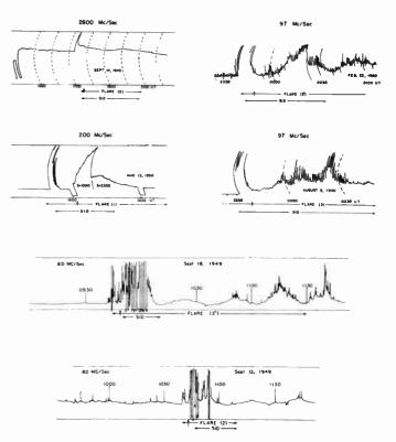
Fig. 1—Examples of 2800, 200, 97, and 80-mc radiation at the time of solar flares. Vertical arrows indicate times of flare maxima. The 80-mc records were made with an interferometer and show maxima and minima in the interference pattern as well as changes in solar emission.
