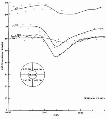
Fig. 2—Absorption of cosmic noise recorded as a function of direction. The circular insert shows the maximum absorption observed during the event for each quadrant and for the zenith.
