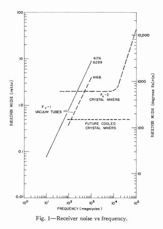
ceptionally close-grid cathode spacing achieves excess noise  $(F_v - 1)$ , as shown by the dotted straight line, but has not been suitable for the low vhf because of its internal construction.
