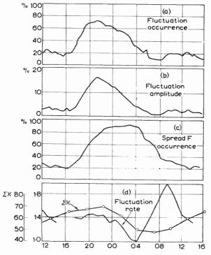
Fig. 8—Yearly average diurnal variations of radio star scintillations (August, 1954 to July, 1955): (a) fluctuation occurrence, (b) fluctuation amplitude, (c) occurrence of spread F at Inverness, and (d) fluctuation rate compared with summation of magnetic K indexes (K).
