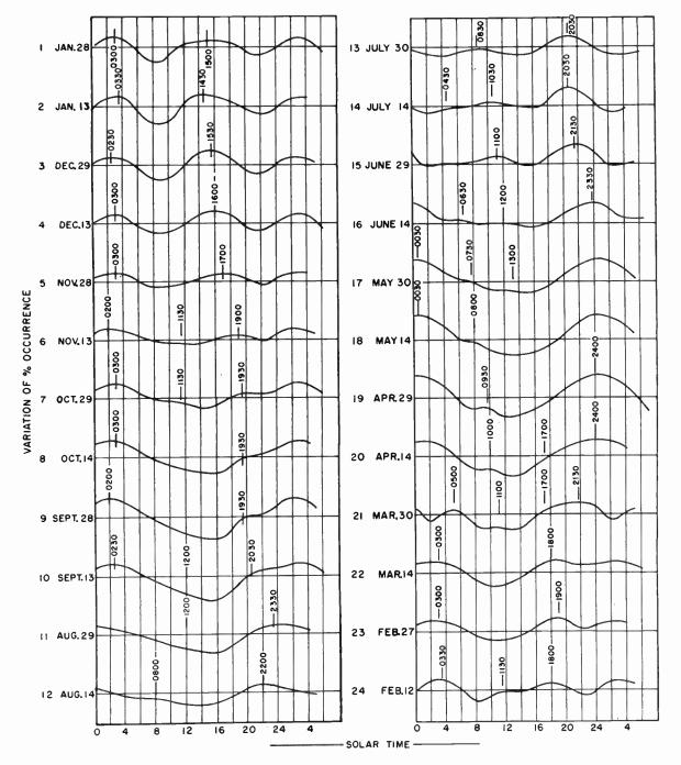
Fig. 10—Each of the 24 graphs shows variation of the percentage occurrence of scintillations plotted against local mean solar time for a given 15-day interval centered about the date written beside the graph. The numbers from 1 to 24 are used to identify 24 positions of the earth on its orbit around the sun in the course of one year. The hours marked along the curves indicate the times during the day at which the occurrence of scintillations passed through a maximum.
