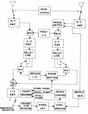
Fig. 2-Phase tracking interferometer block diagram.
