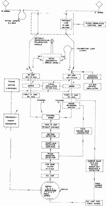
Fig. 4—The multiplying interferometer.
