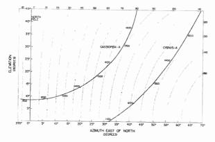
Fig. 2—108-mc lobe pattern from Table Mesa. Small numbers along starpath are local sidereal time. Every tenth lobe, numbered from the plane of symmetry, is shown as a dotted line.
