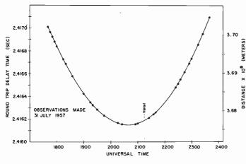
Fig. 2-Distance to the moon as measured by radar for a single six-hour observation period.
