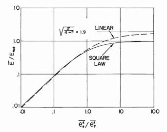
Fig. 6—Ratio of average output voltage to rms deviation from the average vs input snr for linear and square-law detectors.
