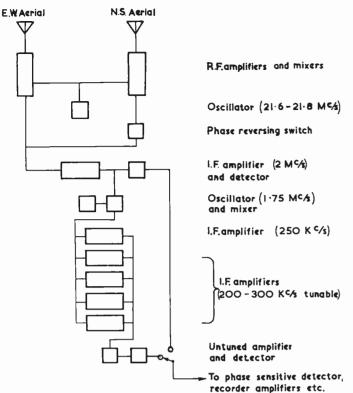
Fig. 2—Block diagram of the receiving equipment. Only the main units are shown. Among the units omitted are the square wave generator for the phase switch, the beat frequency oscillator, and a separate IF channel for recording the output from the N-S antenna separately.
