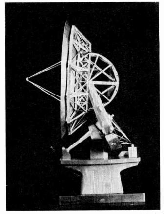
Fig. 7—Another photograph of the model; note the tilted (side view) polar shaft, which will be adjusted to be parallel to the axis of the earth.
