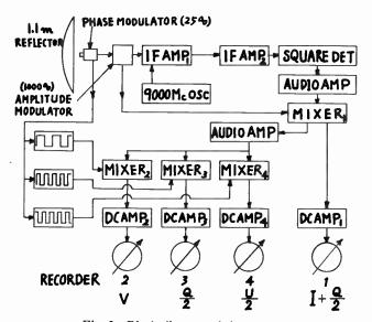
Fig. 2—Block diagram of the system.
