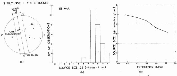
Fig. 15—Observations of Type III bursts. (a) An instantaneous position measurement, averaged over frequency, (b) histogram showing the distribution of source size in the 26 bursts (55 mc), (c) the average spectrum of source size during the bursts referred to in (b).
