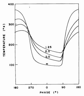
Fig. 7—Calculated microwave temperatures for a homogeneous lunar surface for which  $(K\rho c)^{-1/2} = 1000$ . The numbers on the curves are the values of  $C = \alpha_m (KP/\rho c)^{1/2}$ . (Jaeger, Aust. J. Phys.)
