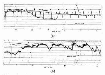
Fig. 1—Ionospheric absorption of 30-mc cosmic noise, (a) recorded by a total power system and (b) recorded by a servo-controlled self-balancing system. In both cases the signal level expected under ionospherically quiet conditions is shown by the dashed line.
