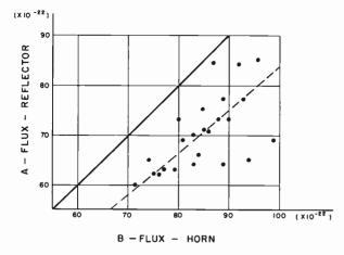
Fig. 5-Flux, as measured with the four-foot parabolic reflector. vs flux, as measured on corresponding days with the 3-foot  $\times$  4-foot aperture horn.
