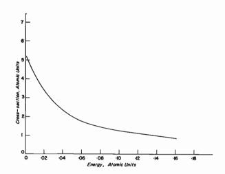
Fig. 1—Cross section for de-excitation of the hyperfine triplet by electrons. Energies are in Rydbergs (13.6 ev) and cross sections in units  $\pi a_0^2 = 8.8 \times 10^{-17}$  cm<sup>2</sup>.
