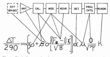
Fig. 1-Block diagram of typical system and the threshold equation showing the influence of the components on the factors in the equation.
