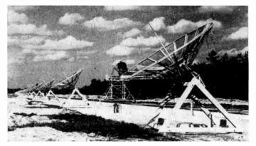
Fig. 2—General view of the 32-antenna interferometer; one of the 3-cm radio telescopes is seen on the rail track.
