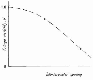
Fig. 2—Fringe visibility diagram for the source of Fig. 1(b) and 1(c).
