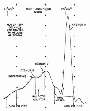
Fig. 2—Sample profile taken with the Ohio State University 96-helix radio telescope in the Cygnus region. The deflections due to the transit of radio stars Cygnus A, Cygnus X, and Cygnus B are shown superposed on the gradual rise due to the general background radiation.
