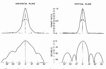
Fig. 3—Radiation patterns of the 50-foot reflector measured at 3.15-cm wavelength.
