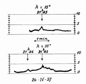
Fig. 6—Deviation obtained on the comet's region on April 26, 1957. In the upper figure the antenna beam has the same direction as the diurnal motion; in the lower figure, the opposite.
