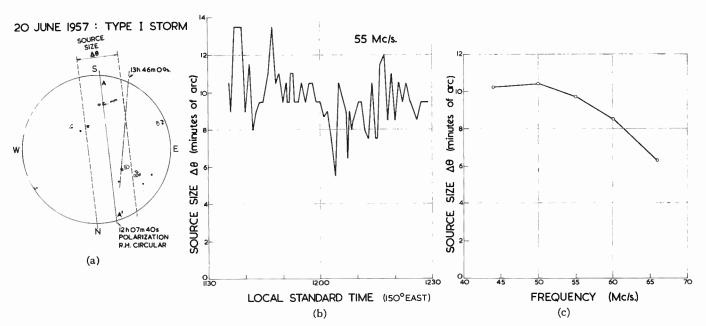
Fig. 14—Observations of a Type I storm. (a) A pair of instantaneous position measurements, averaged over frequency, (b) the variation with time of the apparent source size at 55 mc, (c) the average spectrum of source size over the period in (b).
