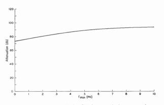
Fig. 14—Sensitivity curve of the C-3 ionosonde in terms of attenuation in db required to produce an observed minimum frequency of the E layer,  $f_{\min}E$ .
