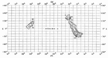
Fig. 10—Map of the radio sky background at 480 mc (after Reber<sup>24</sup>). The contours give the absolute brightness temperature of the radio sky in degrees Kelvin.
