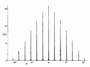
Fig. 2—Directivity of 32-element interferometer at Potts Hill  $\Phi(\theta)$  is power flux compared with that from one element of the array.  $\theta$  is the azimuth angle.
