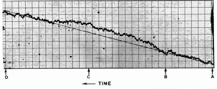
Fig. 7-Radiometer measure of radio emission from Saturn. Maximum antenna temperature 0.04°K. Time' constant = 320 seconds. Between A and B, the antenna pointed  $\frac{1}{2}^{\circ}$  east of Saturn; between B and C, the antenna pointed at the planet; between C and D, the antenna pointed  $\frac{1}{2}^{\circ}$  west of Saturn.
