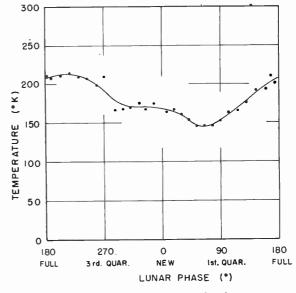
Fig. 5-The maximum antenna temperature for the moon, corrected for atmospheric attenuation, with a pencil-beam antenna radia-tion pattern 0.2° in width between half-power points.
