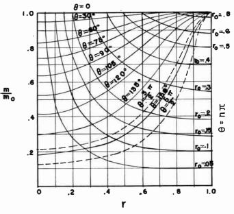
Fig. 7—Polarization parameters as functions of Faraday dispersion angle and initial polarization parameters.
