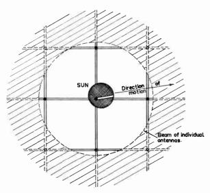
Fig. 4—Sketch showing the multiple lobes of the crossed multielement interferometer and the way in which the sun is scanned by one of these. The path of the scanning lobe across the solar disk is indicated.
