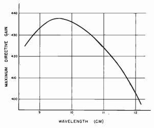
Fig. 2-Calculated maximum directive antenna gain of 3-foot×4foot aperture horn as a function of wavelength.
