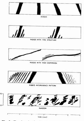
Fig. 5—Sketches showing idealized examples of the principal types of dynamic spectra observed.
