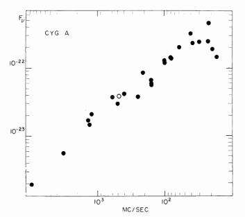
Fig. 7—The spectrum of Cygnus A. The points measured in the present survey are indicated by open circles in Fig. 7-Fig. 11, [2], [3], [8]-[21].
