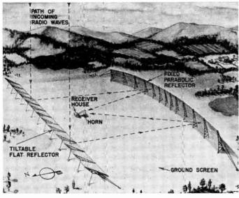
Fig. 4—Sketch showing arrangement of fixed standing paraboloid tiltable flat reflector radio telescope antenna with path indicated for incoming radio waves. An antenna of this design with parabolic reflector 360 feet long by 70 feet high is now under construction at the Ohio State-Ohio Wesleyan Radio Observatory near Delaware, Ohio.
