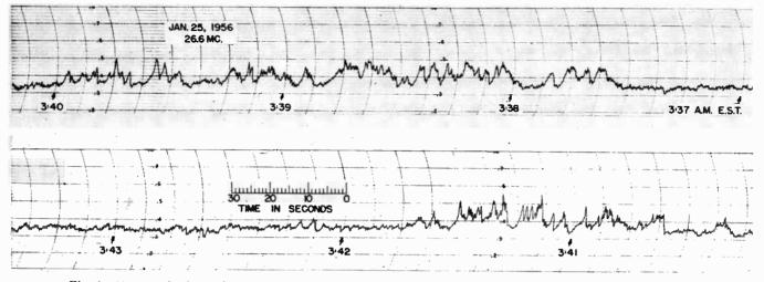
Fig. 6—11-meter Jupiter noise on January 25, 1956, recorded at a tape speed of six inches per minute. The noise corresponds to the peaks beginning about 3:37.5 A.M. and extending to about 3:41.5 A.M.
