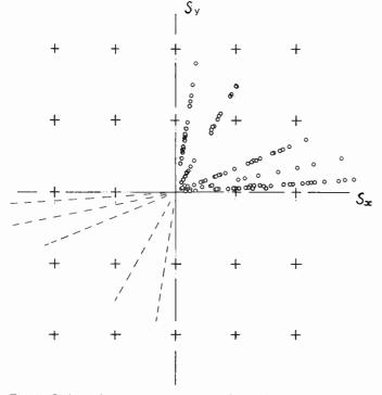
Fig. 4—Independent measurements may be made at the crosses. The circles show the amount of redundancy in an example drawn from current practice.
