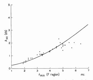
Fig. 16—Absorption at 30 mc using the cosmic noise technique, vs  $f_{\min}F$  (F layer). The solid curve is the theoretically predicted curve, assuming all absorption occurs below the point of reflection from the F layer. The dots are experimental points.
