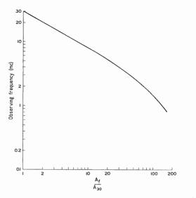
Fig. 13—Ratio,  $A_I/A_{30}$  of the absorption at any frequency f (less than 30 mc) to the absorption at 30 mc, as a function of frequency f. The curve is calculated for the ordinary wave assuming a constant collision frequency  $\nu$  of 10<sup>6</sup> per second, and gyromagnetic frequency  $\omega_L$  of 10<sup>7</sup> radians per second.
