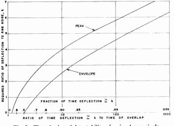
Fig. 2—The criterion of detectability of a signal on a single analog trace.
