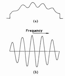
Fig. 2—Characteristic patterns of intensity (vertical) vs frequency obtained with (a) an adding interferometer and (b) a multiplying interferometer.
