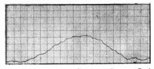
Fig. 4—Radiometer response as the strong radio source Cassiopeia A drifted through the antenna beam. Maximum antenna temperature = 2°K. Receiver time constant = 80 seconds.
