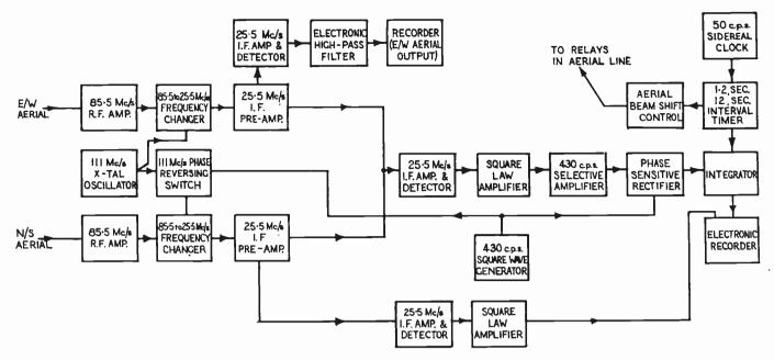
Fig. 14-A simplified block diagram illustrating the essential functional elements of the system.
