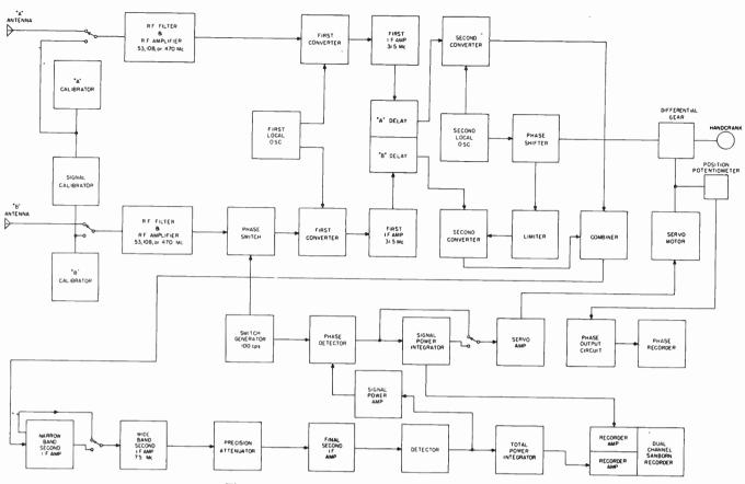
Fig. 1-Block diagram of phase scintillation receiver.
