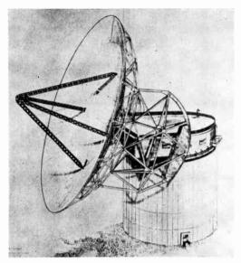
Fig. 4—Rear elevation of Kennedy design, showing truss structure of the reflector.
