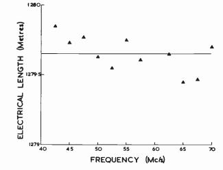
Fig. 9—A typical measurement of electrical length  $(l_L+l_T)$  as a function of frequency. (This example refers to the west feeder with the variable line set to 450 m.)
