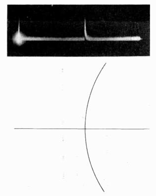
Fig. 11-Lunar echo compared in scale to curvature of the moon.
