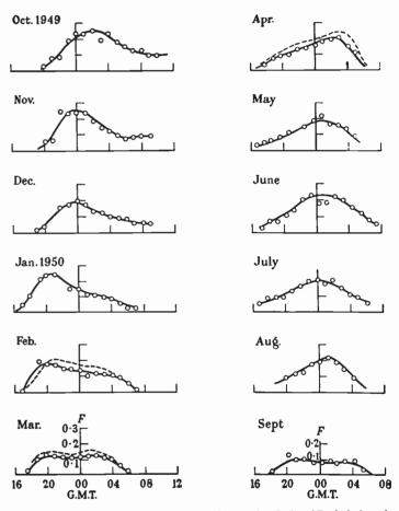
Fig. 7—The diurnal variation of the fluctuation index  $(F_{rms})$  deduced from observations of source 23.01 on 6.7 m. The dotted curves were obtained during the following year on 8 m.
