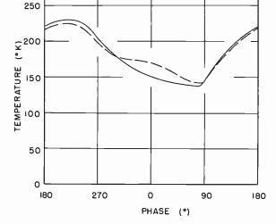
Fig. 6-Comparison of the brightness temperature for the center of the lunar disk (dashed) with a calculated curve (solid) for a lunar surface of deep dust.
