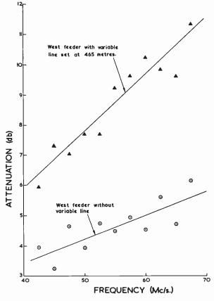
Fig. 10—Two sample measurements of attenuation  $(\alpha_T + \alpha_L)$  as a function of frequency.
