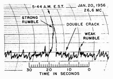
Fig. 7-11-meter Jupiter noise of January 20, 1956, recorded at six inches per minute showing small peak due to very short double crack or click followed about five seconds later by a strong rumble.
