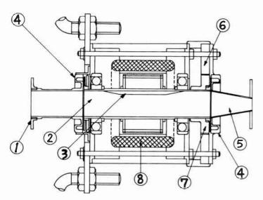
Fig. 4—Phase modulator—1) Feeder waveguide, 2) circular waveguide for modulation, 3) phase shifter, 4) choke coupling for transmission, 5) tapered waveguide, 6) magnet, 7) rotor for reference signal, and 8) coil for induction motor.
