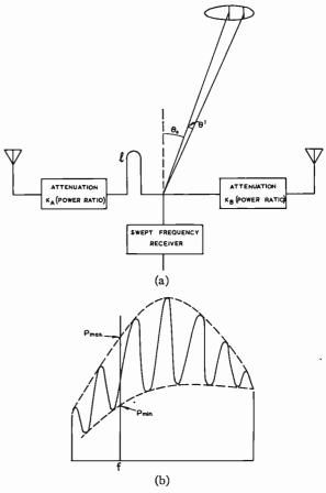
Fig. 12—Defining the symbols required for source-size measurements.
