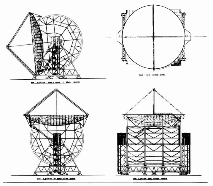
Fig. 1—Drawing by Husband & Company of Sheffield, Eng. for the proposed 140-foot altazimuth telescope design. The two end elevations show the reflector pointed to the zenith and horizon. The front elevation again shows the reflector pointing to the zenith. The plan view shows the quadraple support for the antenna feed.
