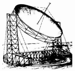
Fig. 5—General view of the 140-foot altazimuth radio telescope design proposed by Dr. Jacob Feld of New York, N. Y.
