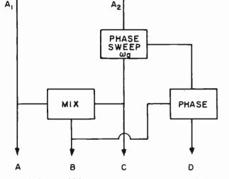
Fig. 2-Polarimeter which measures two components of polarization.
