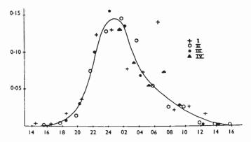
Fig. 6-Variation of the "fluctuation index" for the four sources plotted as a function of the time of observation. Ordinates: Fluctuation index. Abscissae: Local time.
