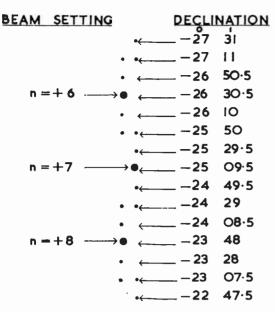
Fig. 10—Examples of some of the standard beam positions available by manual setting (large dots) and automatic switching (small dots). The angles given refer to the declinations to which the beam is directed.
