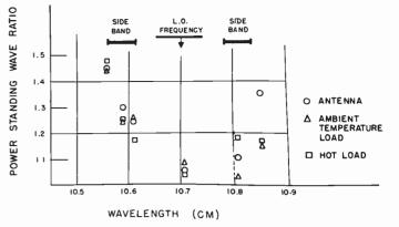
Fig. 4—Power standing-wave ratios of the 4-foot $\times$ 4-foot horn antenna, ambient temperature load, and hot load vs wavelength.
