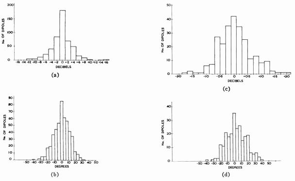
Fig. 9—Histograms of the errors in amplitude and phase of the dipole currents measured five months after setting up. (a) Amplitude errors, E-W array. (b) Phase errors, E-W array. (c) Amplitude errors, N-S array. (d) Phase errors, N-S array.
