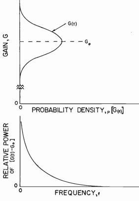
Fig. 4—Approximate probability density and spectrum of random gain fluctuations.
