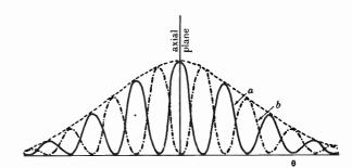
Fig. 2—Reception pattern of two spaced antennas: (a) connected in phase and (b) connected in antiphase.
