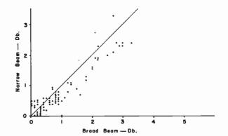
Fig. 5—Hourly values of absorption observed simultaneously on broad- and narrow-beam antennas at College. The straight line is that of equal absorption on the two antennas.
