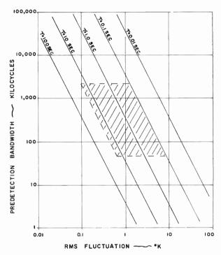
Fig. 5—Plot of rms fluctuation at the synchronous detector output as a function of predetection bandwidth for postdetection integration time constants of 0.01, 0.1, 1, 10, and 100 seconds. The rms fluctuation is given in degrees Kelvin for a background radiation plus excess receiver noise level of 1000° Kelvin.
