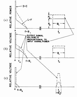
Fig. 9-Approximate power and voltage spectra.
