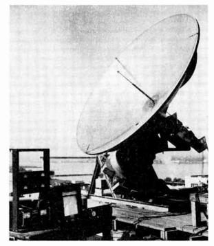
Fig. 1-10-foot radio telescope for 4.3-mm wavelength.
