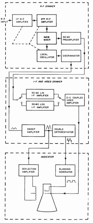
Fig. 1-Block diagram of a typical receiver and indicator.
