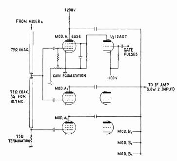
Fig. 3-Construction of the time modulators.
