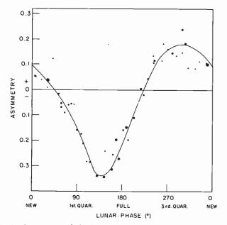
Fig. 3—Asymmetry of the lunar scan curve as a function of phase.
