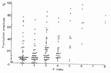
Fig. 13—Comparison of radio star scintillation amplitude with the magnetic K index.
