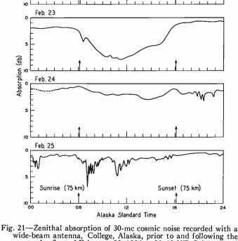
Fig. 21—Zenithal absorption of 30-mc cosmic noise recorded with a wide-beam antenna, College, Alaska, prior to and following the great solar flare of February 23, 1956 at 03:40 UT. Solar control of the absorption is particularly marked during the daylight hours of February 23, 150°. First indications of aurorally associated absorption are on the night of February 24-25.
