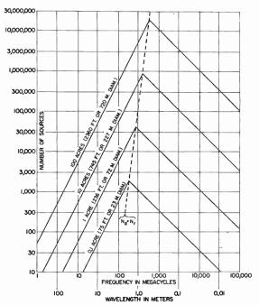
Fig. 1—Number of sources which a radio telescope can both detect and resolve as a function of frequency (and wavelength) and size of antenna aperture. The antenna aperture is given in acres (1 acre=43,560 square feet). Although the aperture may be of any shape, the diameter in feet and meters is given for the case of a circular aperture. To the left of the dashed line  $(N_r = N_d)$  the telescope is resolution limited and to the right it is detection limited.
