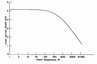
Fig. 2—Cross section for de-excitation, averaged over electron speeds at temperature  $T_{K}$ .
