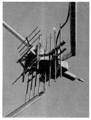
Fig. 2-Close-up view of scale model feed mounted in reflector.
