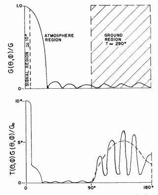
Fig. 3—A typical two-dimensional antenna pattern showing the effects of the source, the atmosphere, and the ground on antenna temperature.
