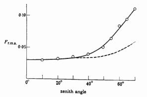
Fig. 11—The dependence of the fluctuation index  $(F_{\rm rms})$  upon the zenith angle of the source. The secant of the angle of incidence on the ionosphere at a height of 400 km is shown by the dotted curve.
