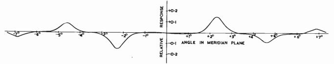
Fig. 12—The error response in the meridian plane near the zenith produced by switching the beam by -20 minutes of arc from a manual position; when switched by a +20 minutes of arc the signs of the responses are reversed.
