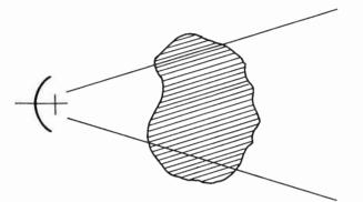
Fig. 2—Antenna viewing an interstellar cloud of hydrogen gas. This is a schematic representation of an antenna viewing a spectrally emitting gas cloud which completely fills the antenna beam.
