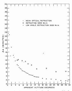
Fig. 11--Refractive error as a function of apparent altitude of source: 9375 mc and optical.
