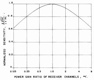
Fig. 4—Curve of reduction in receiver sensitivity as a function of power gain ratio in the two receiver channels.
