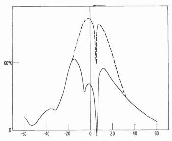
Fig. 6—Expected and observed profiles for Sagittarius A. In this diagram the ordinate is in °K and the abscissa is in kilometers per second. The upper curve is the emission profile expected in the absence of the source while the lower curve is the observed curve.
