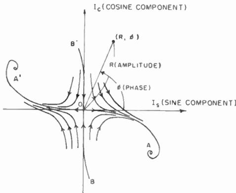
Fig. 5—The amplitude-to-phase ( $R, \phi$ ) locus of an oscillating parametron.
