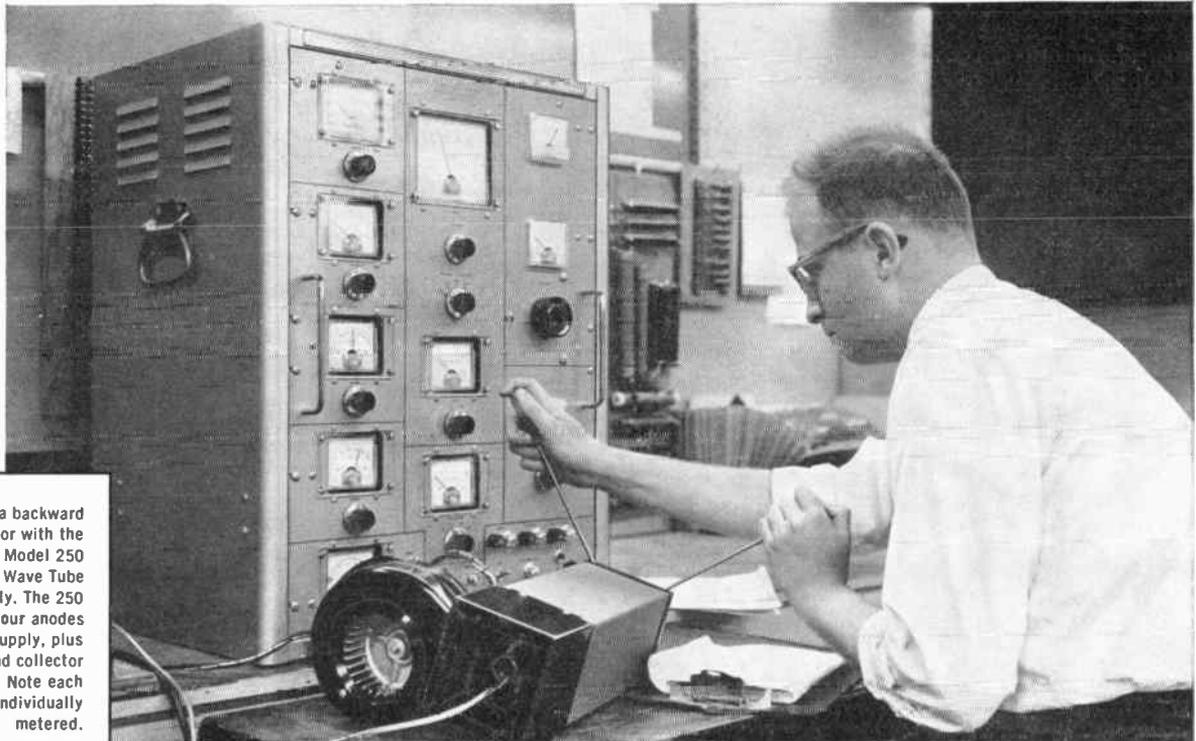
Aligning a backward wave oscillator with the Alfred Model 250 Traveling Wave Tube Power Supply. The 250 features four anodes and grid supply, plus helix and collector supply. Note each supply is individually metered.
