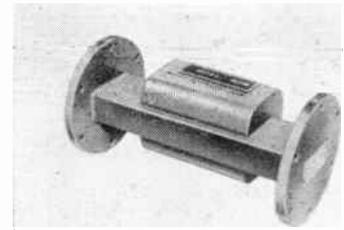
Covering the frequency range from 3.95 to 12.4 kmc in three broadband models, these isolators have an insertion loss of 1.0 db and a vswr of 1.2. Each covers an entire waveguide band.
