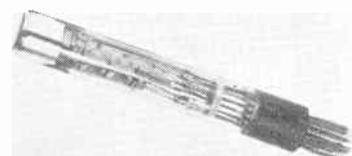
Applications include deep-down geological exploration, aircraft and space vehicle installations, medical probing, scintillation probes, spectroscopy, and various low level light source analysis. The two tubes that are announced are identical in design and performance except in secondary emission characteristics. Type 6362 with silver magnesium dynodes features maximum stability at high voltages, while Type 6934 with cesium antimony dynodes features high gain at low operating voltages.
