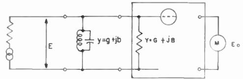
Fig. 13—Susceptance neutralization.
