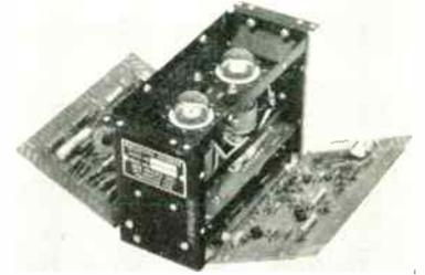
The Model 2202TL Timer is the first in a line of JANized miniature transistorized counters. It provides an accuracy of  $\pm 1$  count  $\pm 0.05$  per cent and a service life of over 5000 hours. It weighs less than two pounds and occupies 160 cubic inches. Performance exceeds the shock, vibration, high and low temperature, pressure salt spray, sand and dust requirements of MIL-T 945A.
