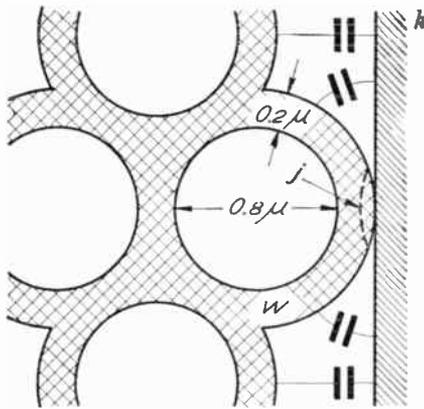
Fig. 3—An embankment whisker  $w$  in contact with the cathode  $k$ . A junction at  $j$  is suggested. At reverse bias this junction gives rise to a capacitance between the whisker and the cathode. Other capacitances between whiskers and cathode in the vicinity of the junction are shown.
