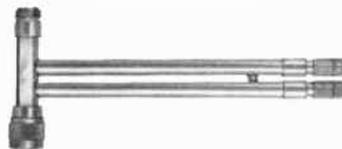
Used to optimize the power output of microwave oscillators by matching the impedance of the source and the load; to tune out reflections in a coaxial transmission system; to maintain a low VSWR on a transmission line for maximum power transfer within a system; as an impedance transformer; to provide a DC return for crystal holders or other devices where DC returns are needed.
