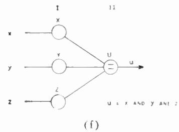
Fig. 8—A three-input majority operation circuit. (a) Circuit diagram. (b) The schematic diagram of (a). (c) An "or" circuit for two inputs. (d) An "and" circuit for two inputs. (e) An "or" circuit for three inputs. (f) An "and" circuit for three inputs.
