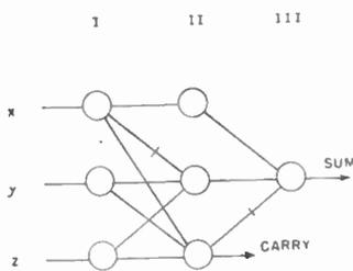
Fig. 12—A binary full-adder circuit.
