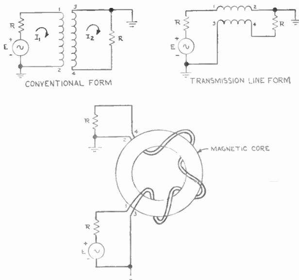
Fig. 1—Reversing transformer.
