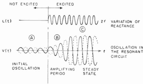
Fig. 4—Oscillation of parametrons.
