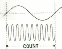
Frequency ratio measurements
