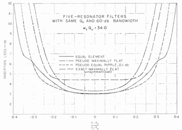
Fig. 5—Pass-band insertion-loss curves for four different five-resonator filter designs.
