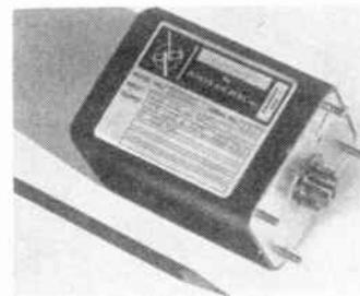
In the past, 30-35 volts dc was the maximum input that could be reliably handled by transistors. This, of course, limited the applications of transistorized inverters because higher voltages, or transients, would blow out the transistors.
