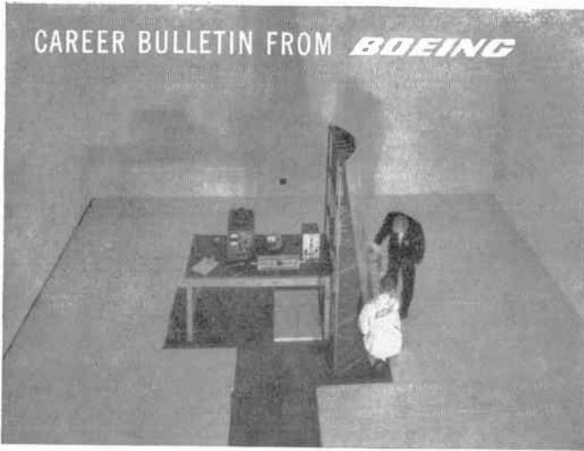
**FREE-SPACE ROOM** in Boeing antenna and radar laboratory, built for advanced antenna and radome development and testing. Expanding missile and advanced jet aircraft projects at Boeing provide outstanding career opportunities for engineers in virtually every area of electronics.
