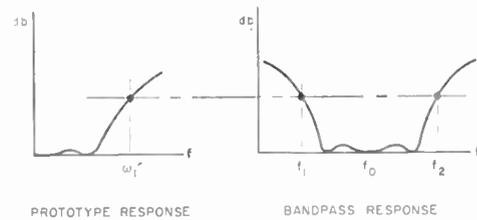
Fig. 1—Correspondence between low-pass prototype response and equivalent band-pass response.
