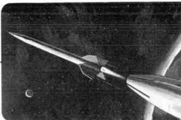
**THE WAC-CORPORAL...** fired in flight from a V-2 rocket, established a world's altitude record of 250 miles in 1949. The combination was known as the Bumper-Wac.
