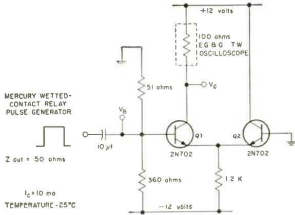
TYPICAL NON-SATURATED LOGIC SWITCHING CIRCUIT
