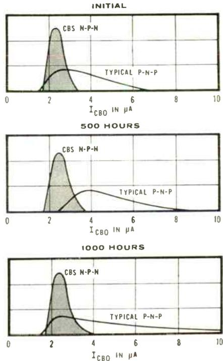
The superiority of CBS NPN transistors is achieved by special processing: For example, advanced surface chemistry techniques seal out moisture and contamination. Precise control of alloying produces high back voltages. Thorough bake-out stabilizes gain. The result is reliable NPN computer-type switching transistors featuring fast switching . . . high voltage . . . low cutoff current . . . and low saturation resistance . . . in a welded JETEC TO-9 package
