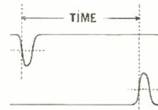
2-channel time interval measurements
