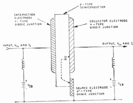
FIG. 1 Structure and circuit arrangement of amplifier.
