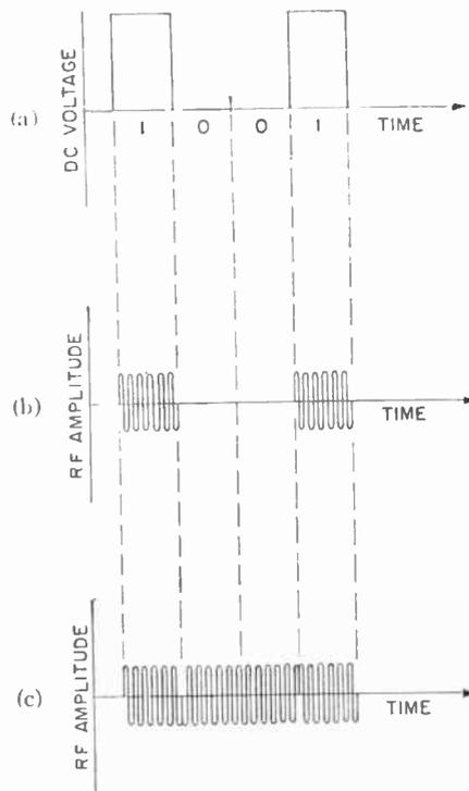
Fig. 5—Three types of script to represent binary information. (a) DC pulse script, (b) RF pulse script, (c) RF phase script.
