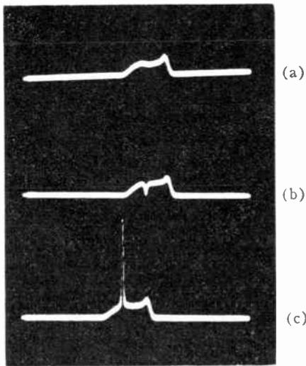
Fig. 1—Oscilloscope display of power reflected from maser cavity as a function of frequency. (a) No pump power. (b) Pump power sufficient to overcome cavity losses. (c) Maser gain with high pump power.
