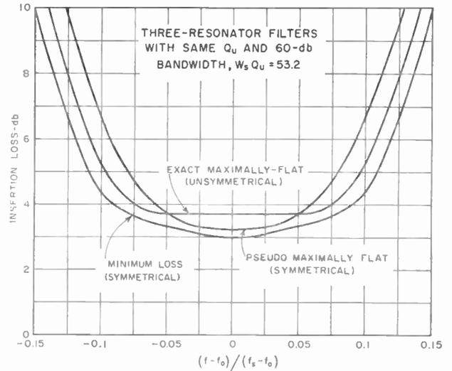
Fig. 4—Pass-band insertion-loss curves for three different three-resonator filter designs.
