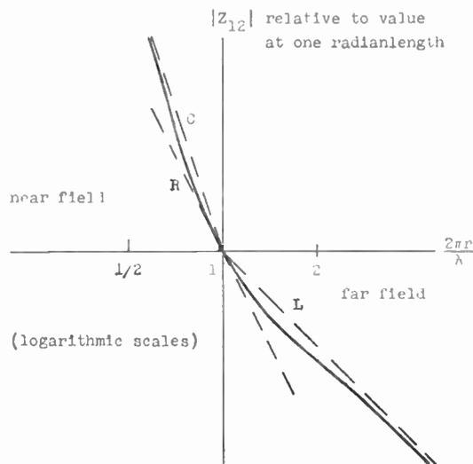
Fig. 6—Variation of components of mutual impedance.
