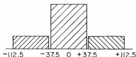
Fig. 1—Audio sweep range of carrier and first-order sidebands for subcarrier at maximum value (75 kc).
