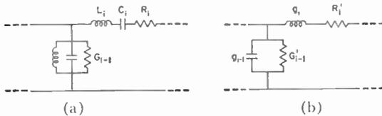
Fig. 8—(a) Dissipative lumped-constant band-pass filter, and (b) equivalent low-pass prototype filter.
