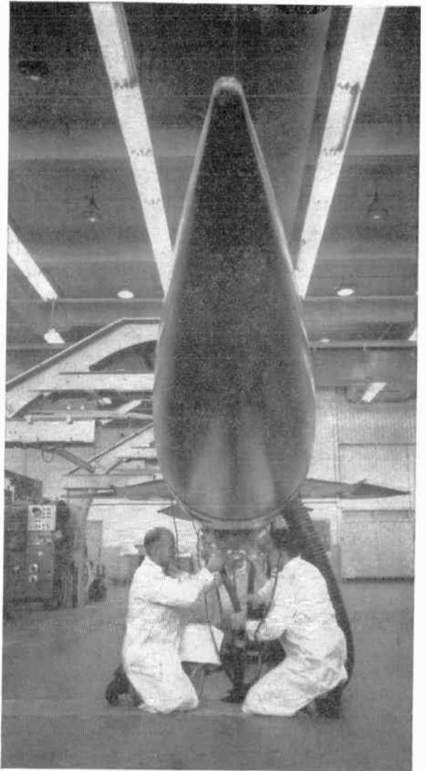
**BOEING ENGINEERS** attaching missile monitor plug for dynamic compatibility test of BOMARC interceptor. In addition to wide variety of simulated tests, BOMARC test firings are conducted at Cape Canaveral, Florida. Expanding Boeing projects offer engineers and scientists outstanding career openings, all with plenty of opportunities for advancement.
