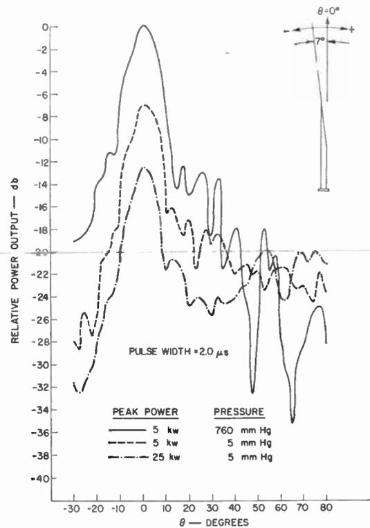
Fig. 6— $E$ -plane radiation pattern of 20-db traveling-wave antenna under breakdown conditions.
