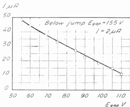
Fig. 4—Relationship between the current  $I$  and the gap voltage  $E_{gap}$  above a current jump.
