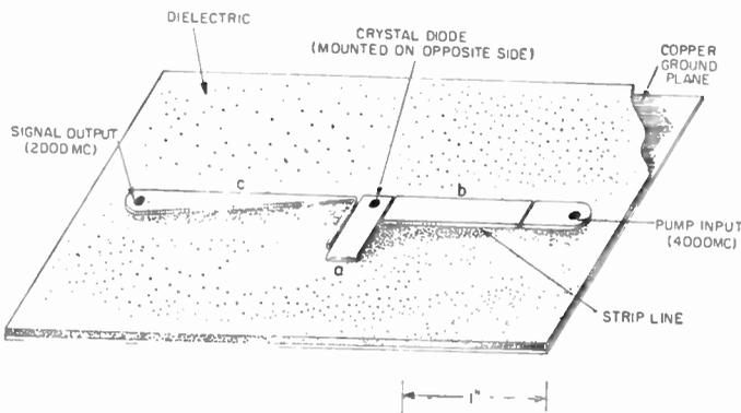
Fig. 1—A strip line subharmonic oscillator with 2000 mc output frequency.
