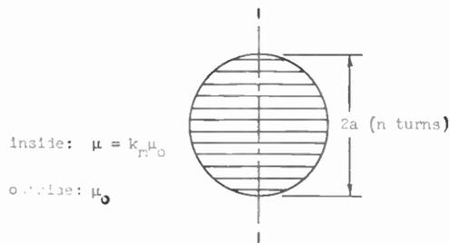
Fig. 7—Spherical inductor.
