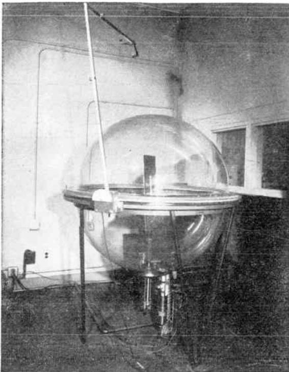
Fig. 2—Photograph of Plexiglas vacuum chamber.
