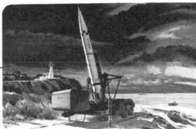
**THE SERGEANT...** A second-generation solid propellant missile developed by JPL for the U.S. Army. The SERGEANT is now being readied for production.
