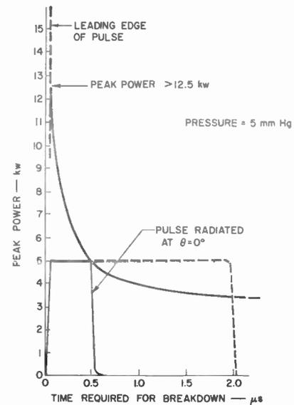
Fig. 12—Time required for breakdown as a function of peak power for 5 mm Hg pressure.
