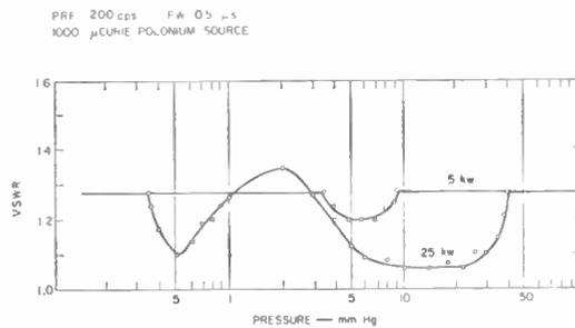
Fig. 4—VSWR as a function of pressure for 5 and 25 kw peak power.
