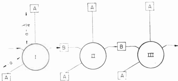
Fig. 10—Shift register. A = subharmonic oscillator, B = delay line.
