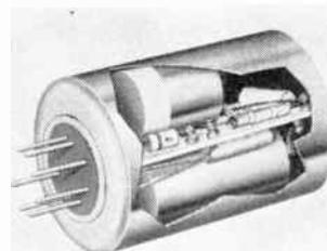
Unit has a 1-volt output operating into 1000 ohms. It holds this output to within  $\pm 1.2$  millivolts over input conditions from 100 to 130 volts, at frequencies from 25 cps to 10,000 cps. The 1-volt output is maintained over an operating temperature range of  $-55^{\circ}\text{C}$  to  $+100^{\circ}\text{C}$ , and any combination of specified variations in tem-
