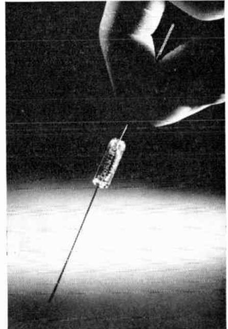
**Fusion-sealed resistors** For *ultra* specs. Glass-enclosed, tin oxide resistance element. Impervious to moisture because of fusion seal. 10 ohms to 360 K at 70°C., derating to 160°C. Well in excess of MIL-R-10509C, Char. B.
