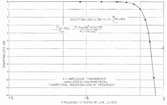
Fig. 16—Theoretical insertion loss vs frequency.
