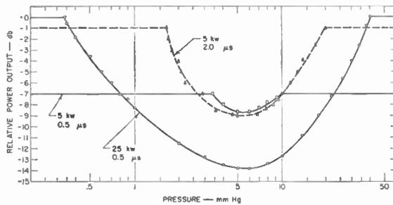
Fig. 5—Power transmitted on main lobe as a function of pressure with 5 and 25 kw peak power applied.
