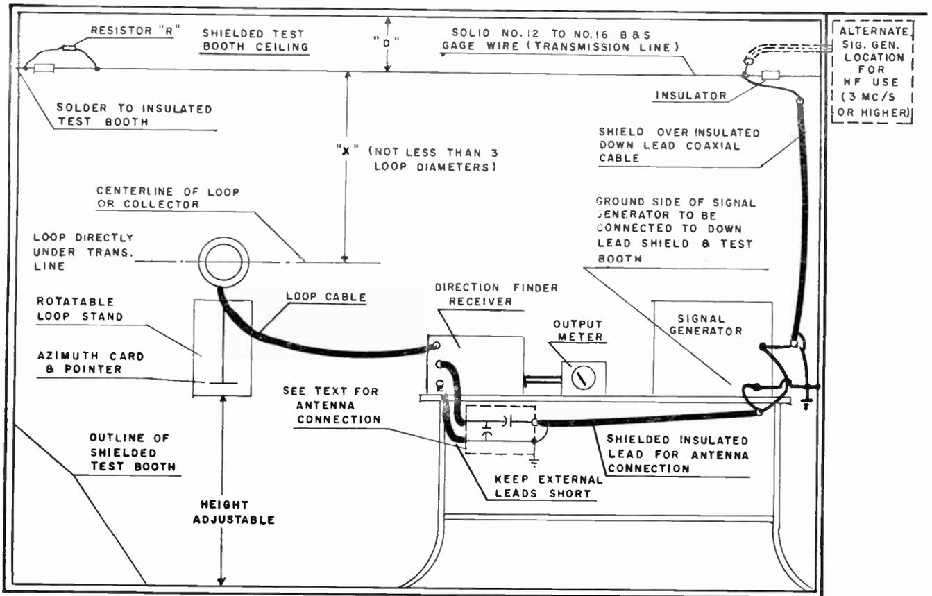
Fig. 1—Shielded transmission line.
