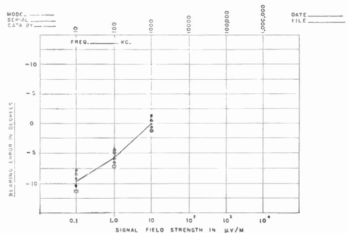
Fig. 6—Bearing sensitivity (average bearings of five observers).
