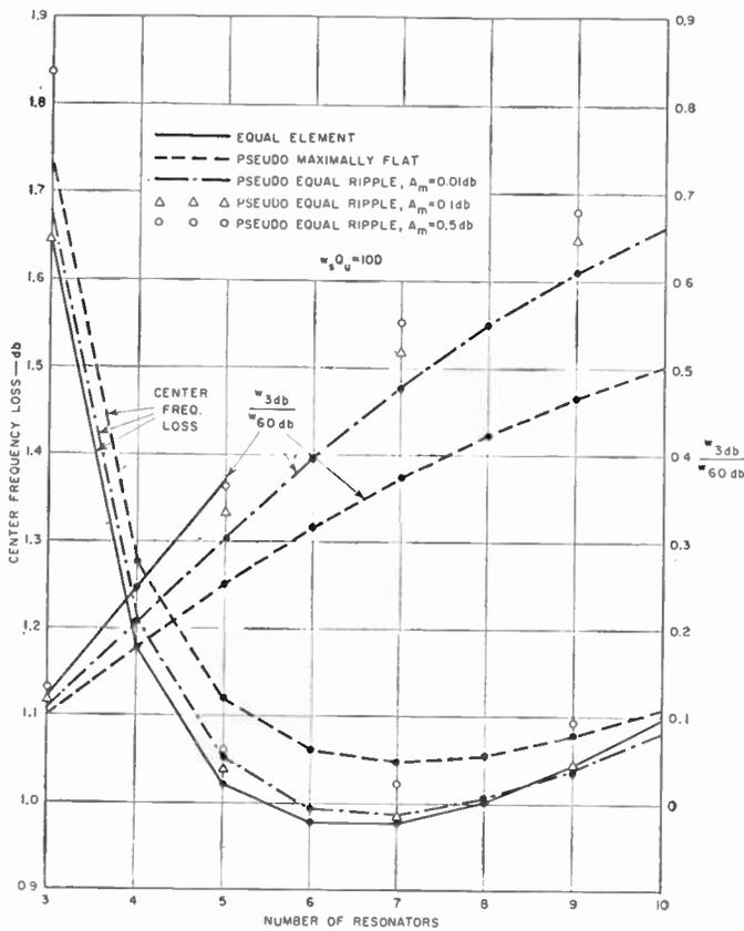
Fig. 6—Center-frequency dissipation loss and relative bandwidth for various symmetrical multiple-resonator filters.
