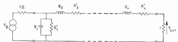
Fig. 3—Dissipative low-pass prototype filter.
