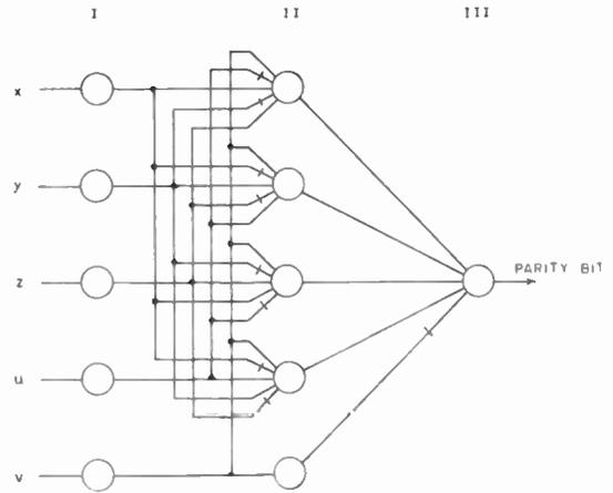
Fig. 13—A parity-check circuit for five input signals.
