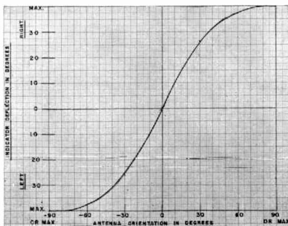
Fig. 10—Indicator deflection vs antenna orientation.
