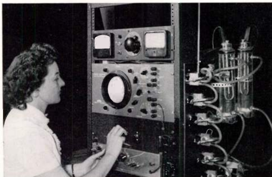
Thermal resistance measurement equipment, another Clevite development, is used to check temperature drop between the junction and mounting base of power transistors under actual operating conditions. It's one of many specialized testing procedures to control quality and improve performance.
