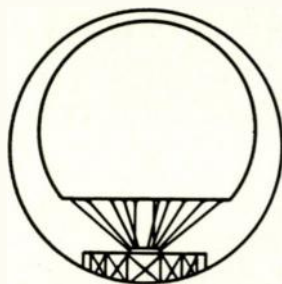
The Original Paraballoon was mounted on a metal support. Only the antenna and balloon protector were air supported.
