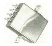
The new model utilizes the standard BR-7 header with an additional set of single pole, normally open contacts which ground one coil terminal to the case when the relay is energized. The 1A set of contacts is rated at 1 ampere inductive and is
