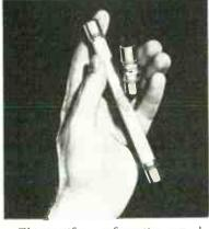
This rectifier configuration was developed and introduced to industry by International Rectifier. The recent addition of high current types makes this the widest selection available. The current range is from 45 to 440ma. PIV voltages range from 1500 to 16,000 volts in standard types. With modification, the PIV can be increased to 20,000. On special order, 72,000 PIV units can be supplied. For complete technical data on these units ...
