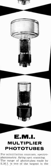
photometry, flying spot scanning. The range of phototubes made by E.M.I. is one of the largest in the world. It includes end-window types of 1" to 15" diameter, with S10, S11, S13 and S20 cathodes, with 10 to 14 dynodes of venetian blind type or of box and grid or focused construction. Tubes for C<sup>14</sup> and H<sup>3</sup> Scintillation counting, also very low dark-current types, are an E.M.I. speciality. Tubes can also be produced to special order.
