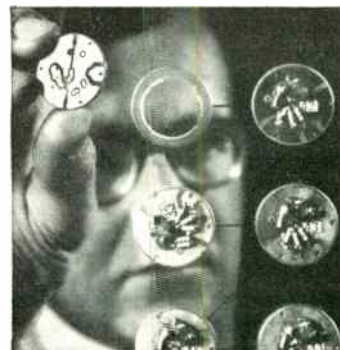
500 MEGACYCLE LOGIC SYSTEM , the first to take full advantage of the ultra high speed capabilities of the tunnel-diode, operates 50 times faster than present circuitry.
