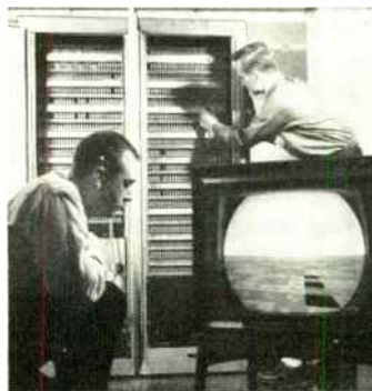
CONTACT ANALOG DISPLAY for blind flying or flight simulation uses a digital computer to "paint" a moving TV picture of the ground analogous to the obscured real ground.
