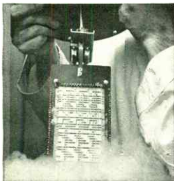
CRYOGENIC ASSOCIATIVE MEMORY enables computers to function like a human brain by instantaneously comparing and associating a new fact with all data in its memory.
