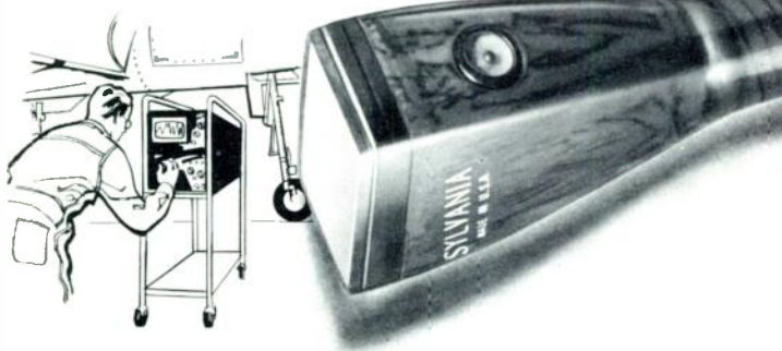
Sylvania 3BGP1, 3BGP2, 3BGP7, 3BGP11 . . . feature direct-view rectangular faces, electrostatic deflection and focus, high deflection sensitivity.
