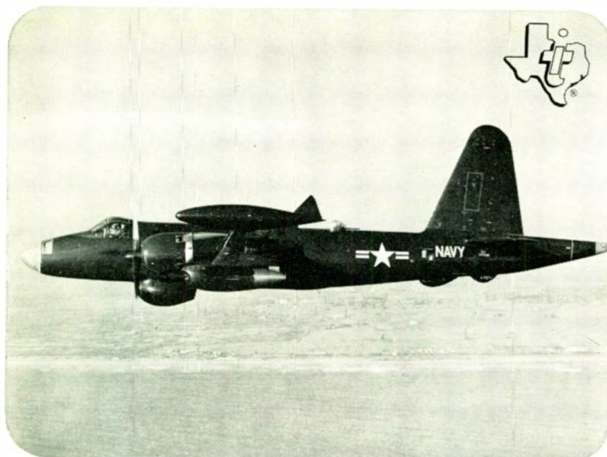
U. S. Navy P2V NEPTUNE antisubmarine aircraft, produced by Lockheed—equipped with TI-built AN/ASQ-8 magnetic anomaly detector, AN/AIC-15 intercommunications system and TD-239A intervalometer.
