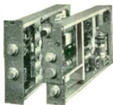
Type 492 Amplifier (left) provides 2 channels of precision amplification per unit. The Type 491 (right) is a single channel unit, with input coupler for added versatility.
