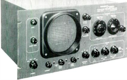
Panoramic's advanced Model SB-15a automatically and repetitively scans spectrum segments from 1 kc to 200 kc wide through the entire range (0.1 kc to 600 kc) . . . plots frequency and amplitude along the calibrated X and Y axes of a long persistence CRT, or on a 12 x  $4^{1}/_{2}$ " chart (optional RC-3a/15). Sweep rates are adjustable from 1 to 60 cps.
