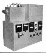
Precision Gas Diffusion Furnace with multiple controls for quality transistor and semiconductor bodies.
