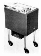
The recording mechanism, with low impedance, enclosed galvanometers, uses the heated stylus method to produce traces on 50 mm rectangular coordinate charts moving at a choice of four pushbuttonselected speeds. The system includes two transistorized current-feedback power amplifiers, their power supply, and the preamplifier power supply. System cooling is provided by forced filtered air from an integral blower.
