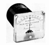
The integrator features an input sensitivity as low as 10 my rms. Standard models are available to indicate 57 to 63 cps and 380 to 400 cps. Variations are also available with center frequencies from 50 cps to 50 kc. Resolution is 0.1%. The Pulse integrator features an integrally mounted panel-type meter. Standard meter sizes are  $3\frac{1}{2}$  wide or  $4\frac{1}{2}$  inches wide. Special meters are available.
