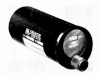
They are contained in 2" diameter MS33639 sealed cases and the assemblies qualify to MIL spees. The counters are new designs and are available in special configurations and calibrations, and with red or white integral lighting. Backlash is reduced to approximately 2 minutes through use of AGMA precision 2 gears and ABEC-7 ball bearings.
