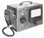
The noise-generating head is a separate assembly which connects to the main housing by a flexible cable. This arrangement allows the head to be attached directly to the receiver under test; this eliminates stray signal pickup from long connecting leads. The type 5722 noise diode and associated circuitry are located within this external head which fits into a clamp on the side of the housing when not in use.
