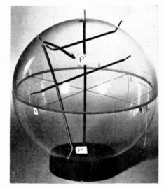
Fig. 1—Model of the Cayley-Klein representation of three-dimensional hyperbolic space showing the transformation of an impedance or a reflection co-efficient through an ideal transformer.
