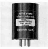
The unit incorporates the addition of a transformer-coupled isolating drive network and clipping diodes so that it can, for example, be driven from a 60 or 400 cps sine wave power line or from a drive source that is common to the dc voltage being chopped.
