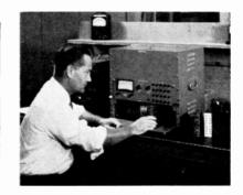
The introduction of the TR-5 Mounting Unit makes it possible for special purpose analog computers to be assembled without the problems usually associated with such a project. The PACE solid state analog computing components plug into the TR-5 mounting unit where they may be interconnected according to the computing function to be performed.
