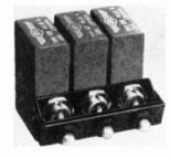
Characteristics are as follows: Continuous duty ratings from 50 milliamperes to 15 amperes. Contacts are rated for 50 dc volts or 120 rms volts at 60 or 400 cps. Operational life is at least 10,000 operations, at rated current.
