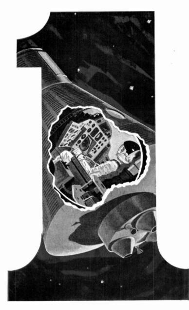
America's FIRST man into space will rely on a Honeywell designed and developed Attitude Stabilization and Control System for controlling his space capsule. This system automatically damps out initial launch rates, orients and maintains the capsule in proper orbital plane, and provides for the correct descent trajectory and re-entry angle. This device is just one of the many contributions being made by Honeywell scientists and engineers to our nation's space programs.
