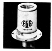
The new thyratron is capable of switching 350 kw peak power after a 30-second filament warm-up time. Operation at 125° ambient temperature is possible without forced cooling when the tube is operated at its maximum plate dissipation factor  $(P_b)$  of 2.7×10°. A hydrogen reservoir, connected internally across the cathode filament, increases tube life.
