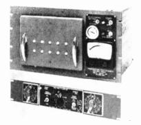
Individual high and low temperature timer adjustments allow independent time durations of up to 3 hours each for any pair of pre-selected high and low temperatures. A selector switch permits timed intervals to include only the constanttemperature time or to include the transition times as well. A master timer either will permit cycling indefinitely or will stop the cycling after any period up to 24 hours.
