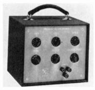
**Electronic Development Corp.**, 432 W. Broadway, Boston 27, Mass., has introduced a new Precision Voltage Reference Source which features an increased voltage range of -111.11 to +111.11 volts dc, selectable in 10 millivolt increments. The new Model VS-111 is a 4-decade directreading instrument available in portable or standard rack-mounting models. Absolute accuracy is 0.025 percent and resolution is 1 part in 10,000 plus vernier resolution.
