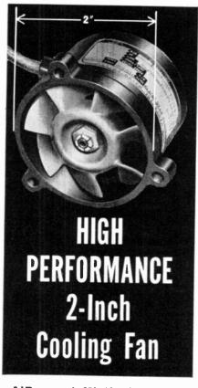
AiResearch Minifan\* is an extremely high performance 400-cycle AC motor-driven fan used for cooling airborne or ground electronic and electrical equipment. Model shown has a flow capacity of 53.5 cfm at a pressure rise of  $3.44 \text{ H}_2\text{O}$ , and requires only 69 watts.
