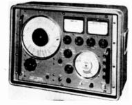
Additional features include a calibrated fine frequency control for bandwidth measurements, a modulation compression circuit for constant FM deviation and mutual inductance piston attenuator of very low VSWR for RF level control.
