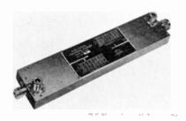
A directional coupler used as a reflectometer must exhibit extremely high directivity, since the error in VSWR introduced in the measurement is equal to the VSWR associated with the directivity of the reflected wave coupler. The directivity
