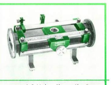
conveniently interchangeable waveguide sections no slope adjustment required vernier position scale readable to 0.1 mm. dial gauge holder and movable stop tapered slots to minimize residual VSWR
