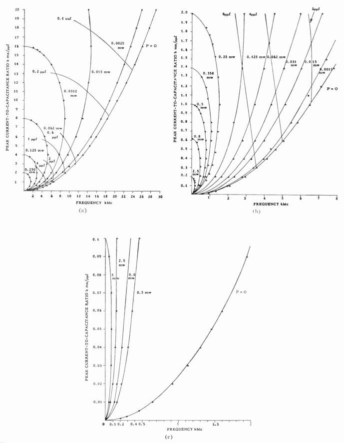
Fig. 4—(a), (b) and (c). Germanium constant power-inductance product, *PL* curves for L=0.25 mµh, V=0.1 volt, and  $R_*C=6$  ohm-µµf. *V* is the voltage swing over the linear range of negative resistance;  $R_*C$  is the diode series resistance junction-capacitance product. Constant capacitance-inductance *CL* curves for L=0.25 mµh, and V=0.1 volt have been included in (a) and (b).
