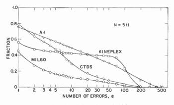
Fig. 5—Fraction of the code words with errors which have more than *e* errors.
