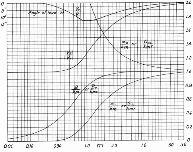
Fig. 3-Normalized parameters of a tapered line.
