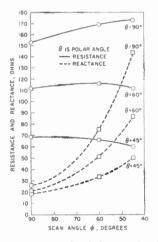
Fig. 11-Impedance vs scan angle of element 31 of half-wave, dipole array with reflector (after Carter).
