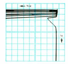
**Dynaquad** is a three-terminal device featuring regenerative switching characteristics. One terminal —the base—serves as the control gate for initiation of the regenerative action. It permits turn-on and turn-off by bursts of drive power. In this way, a small signal controls large amounts of energy in a ratio not approached by conventional '3-layer junction transistors. Trace shows Dynaquad collector characteristics with base current turn-on.
