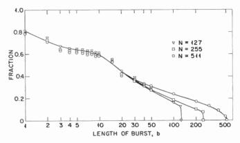
Fig. 2—Fraction of the N symbol code words with errors for which the burst length of errors is greater than b (CTDS data).
