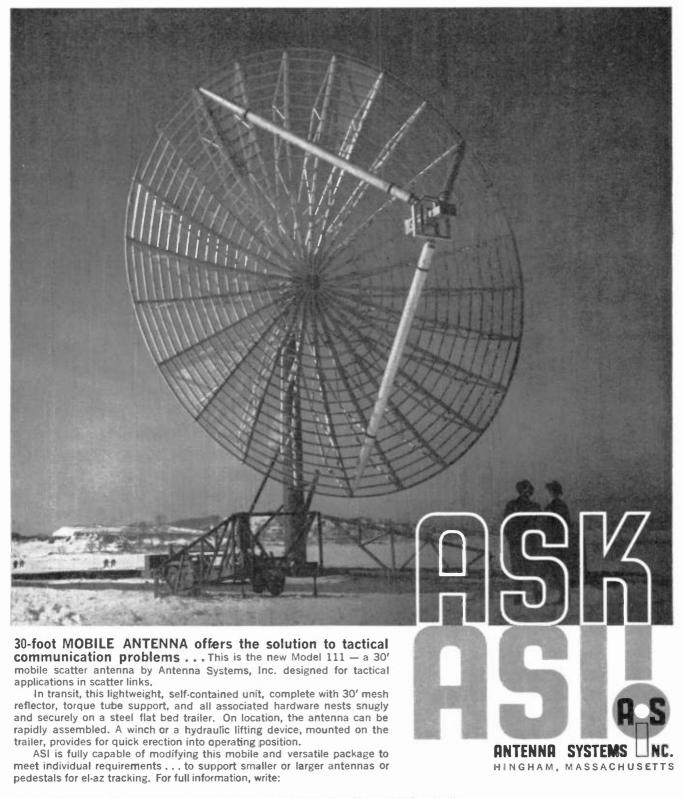
FOR ANSWERS TO PROBLEMS IN THE DESIGN, FABRICATION AND INSTALLATION OF ANTENNA SYSTEMS, ASK ASI!
