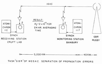
FROM ERRORS INTRODUCED BY TRANSMITTER FACILITIES
