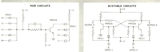
Typical Propagation Delay 20 nanosec.
