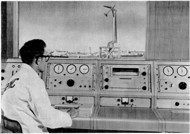
Scientific-Atlanta antenna pattern recording console at Boelng Airplane Company, Wichita, Kansas. with Scientific-Atlanta model range tower in background.
