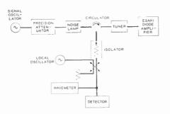
Fig. 2—Block diagram of the 55-kMc test circuit used for noise and gain measurements of the amplifier.
