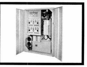
Transmitters for the Air Force Search Radar AN/ FPS-20, built by Bendix Radio Division of the Bendix Corporation for the Rome Air Development Center, Air Research and Development Command.
