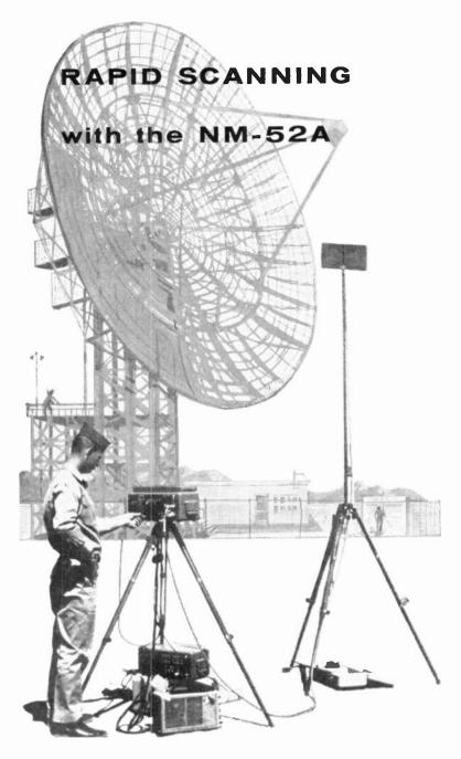
. ensures r-f compatibility of new and existing electronic equipment over the frequency range 375 to 1000 mc.
