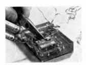
Defective part is removed and its replacement soldered into the cir-cuit without damaging encapsulant.
