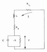
Fig. 2—Equivalent network for tunnel diode. The junction parameters are  $C_{i} = R_{i}$  and  $R_{i}$ . The inductance of the cavity and the load are L and  $R_{L}$ .
