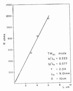
Fig. 2- Experimental variation of the radiation sistance vs length of a dielectric tube waveguide
