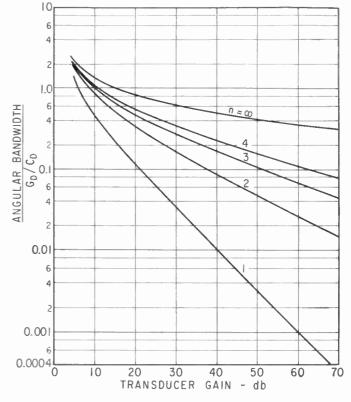
Fig. 14—Gain-bandwidth performance of the optimum transmission-type amplifier.
