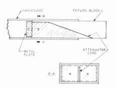
Fig. 1—Teflon plunger for rectangular cross-section waveguide.
