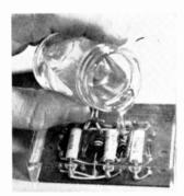
After circuit repair, additional resin is poured over replacement part. Replaced material honds to original encapsulant.
