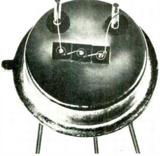
FSP-60 Triple Darlington High Gain Low Noise Amplifier T0-5 size header  $3 \cdot 2N1613$  Planar Transistors hFF typical = 100,000
