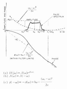
Fig. 1-Filter transfer characteristic
