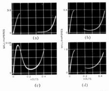
Fig. 1. Oscilloscope tracings of forward 60-cps V-I characteristics of high-frequency GaSb Esaki di-odes: (a)-(c) diodes of p-type GaSb with formed point contacts of a Sn-Te alloy; (d) diode of ntype GaSb with formed point contact of zinc.
