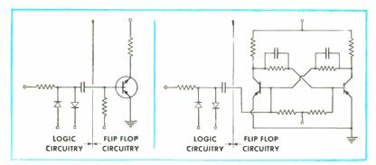
7 components replace 14. Comparison of a single stage of the 10-bit shift register designed with Dynaquad transistors (left) and conventional components (right) shows the circuit simplicity and component reduction obtained with Tung-Sol's new germanium multilayer alloyed junction transistor.
