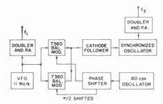
Fig. 2-Circuit for the generation of the signals of frequency f1 and f2
