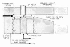
, 1—Cross section of a millimeter-wave Esaki-diode amplifier circuit. The waveguide was RG 99 U reduced in height to 0.01 inch. Fig.
