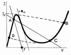
Fig. 2—Operating conditions for single tunnel-diode flip-flop and the monostable circuit.
