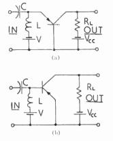
Fig. 1—Transistor frequency divider. (a) Common base. (b) Common emitter.
