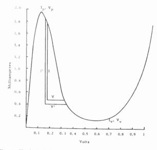
Fig. 1—Typical GaAs tunnel-diode current-voltage characteristic with forward bias.  $V_p$  = peak voltage;  $V_V$ , valley voltage; V and L, voltage and current swings over linear range of negative resistance, respectively.
