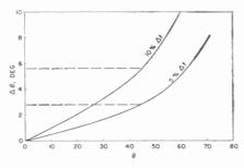
Fig. 8-Beam shift due to frequency offset.
