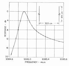
Fig. 2—Response curve of a resonator formed by two plain circular plates.
