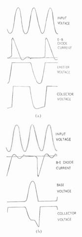
—(a) Common base circuit waveforms. (b) Common emitter circuit waveforms. Fig. 2
