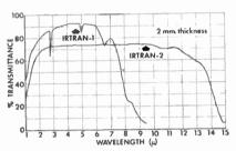
Irtran-1 material seems to provide the best present answer to the "dual-mode" problem. Infrared and microwave guidance can look through the same window. At 9.4 kmc its dielectric constant is around 5 and its loss tangent 10<sup>-4</sup>. One untuned sample .012" thick we tested in the X-band introduced an attenuation of less than 0.3db, with a maximum standing wave ratio of 1.5. In the infrared at 1 $\mu$  its refractive index is only 1.38. No need for anti-reflection coatings, you see.
