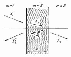
Fig. 1—Schematic representation of a plane electro-magnetic wave incident on a plane boundary and transmitted into medium 3.
