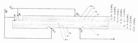
Fig. 3-Sketch showing features of epitaxial slab.
