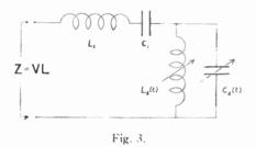
Suppose the network contains angular frequencies  $v_i$ . These are then the elements of the diagonal matrix V. The inductance matrices for each component are, for  $L_1$ ,  $(jL_1)$  U; for  $C_1$ ,  $[-j(1/C_1)]V^{-2}$ ; for  $L_2(t)$ ,  $L_2$ ; and for  $C_2(t)$ ,  $(VC_2V)^{-1}$ , where all are skew Hermitian. Assuming that the indicated inverses exist then, the over-all matrix is
