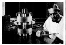
RCA Super Power Tubes have made operation with conventional circuit tuning techniques a practical reality in high-power UHF.
