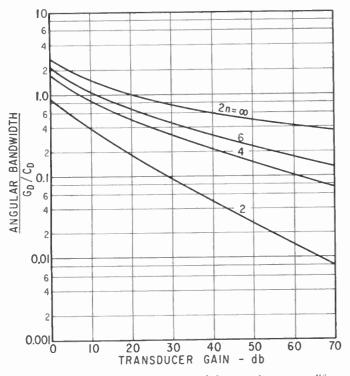
Fig. 17-Gain-bandwidth performance of the cascade-type amplifier.
