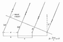
Fig. 1-Linear Van Atta reflector.
