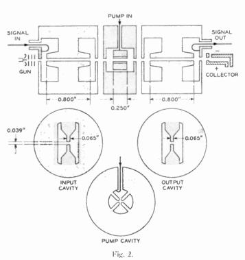
a sketch of its components. The tube differs from previous microwave quadrupole amplifiers<sup>5,6</sup> in the design of its signal and pump cavities, and also in several other features to be described.
