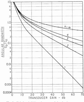
Fig. 9—Gain-bandwidth performance of the circulator-type and hybrid-type amplifiers.
