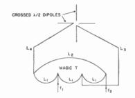
Fig. 1-Arrangement of the magic T and dipoles.
