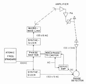
Fig. 2—Block diagram of the A5NA transmitter facilities and its frequency and phase control circuit.
