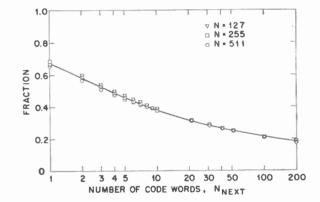
Fig. 4—Fraction of the time for which the number of code words from one code word with errors to the next code word with errors is greater than  $N_{next}$  (CTDS data).
