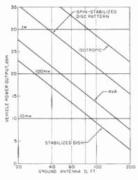
Fig. 9-Vehicle power per Mc bandwidth.
