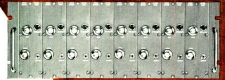
Model 658-3400 - drives high frequency optical galvanometers to 5 KC
