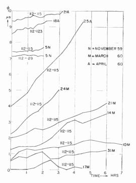
Fig. 3—Some typical phase recordings for A5XA transmission signals.
