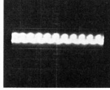
Fig. 1—Output waveforms: (a) sinusoidal, horizontal (30 µsec/cm), vertical (5 volts/cm); (b) gated, horizontal (30 µsec/cm), vertical (1 volt/cm).
