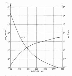
, 1– Electron density  $n(x_s)$  and sheath thickness  $(x_s)$  as a function of altitude. Assume  $\gamma = 10^{-2}$  and Fig. 1constant.
