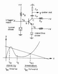
Fig. 2- Base-triggered avalanche stage with tunnel diode.
