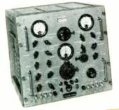
In 1946, we introduced the highpower signal generator, providing 10,000 times more power than any previous generator. Today, we manufacture a complete line of R-F test instruments (from 85 KC up to microwave) that are in wide use by government agencies (including the National Bureau of Standards), by the Armed Forces and by major industries.
