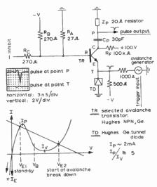
Fig. 3—Emitter-triggered avalanche stage with tunnel diode.
