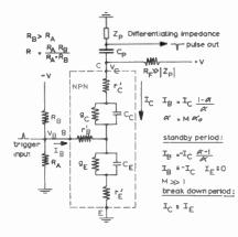
Fig. 1—Base-triggered avalanche stage.
