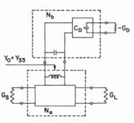
Fig. 3—Insertion of a tuned circuit between  $N_a$  and  $N_b$ .
