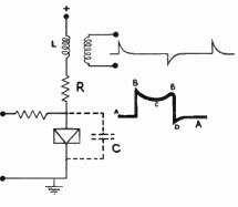
Fig. 1—Single tunnel-diode flip-flop.
