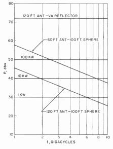
Fig. 7-Ground power per kc bandwidth.
