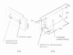
Fig. 2—Sketch illustrating slab external geometry. (a) Resistive region. (b) Capacitive and switchingnegative resistance regions.
