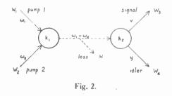
powers  $W_1$  and  $W_2$  at the frequencies  $\omega_1$  and  $\omega_2$ , respectively. The sum of these powers is delivered to the reactance changes at the frequency  $(\omega_1 + \omega_2)$ . The second transformation  $k_2$  is a Mode 4. It delivers power to both the signal circuit and the idler circuit at the respective frequencies v and y. The various powers in terms of the energy coefficients are:  $[Note: y = (\omega_1 + \omega_2 - v)]$
