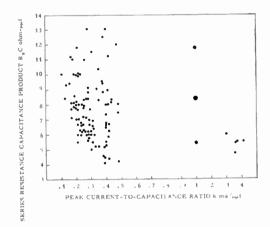
Fig. 3—Series resistance-capacitance product  $R_kC$  for various Ge diodes vs peak current-to-capacitance ratios k.
