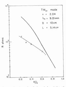
Fig. 3—Experimental and theoretical variation of radiation resistance vs.  $a, \lambda$  for a dielectric tube waveguide. (A different glass seal from the one in the results of Fig. 2 was used.)
