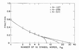
Fig. 3—Fraction of the N symbol code words with errors for which the number of 16 symbol words with errors is greater than  $n_{16}$ (CTDS data).
