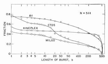
Fig. 6—Fraction of the code words with errors for which the burst length of errors is greater than *b*.
