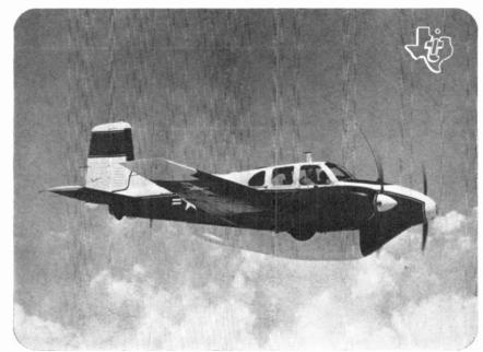
U. S. Army L23D produced by Beech Aircraft—equipped with AN/UPD-1 highresolution, ground-mapping radar developed and built by TI in cooperation with the University of Michigan and the U. S. Army Signal Corps.
