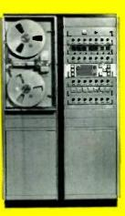
Ampex's Advanced Recorder / Reproducer. the FR-600 used for missile check-out work.
