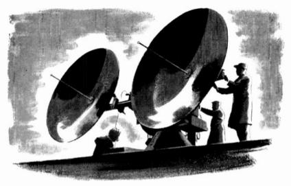
The quest for accurate tornado "signatures" by scientists at CAL may one day permit tornado path prediction at great savings in life and property. Here, CAL engineers conduct meteorological radar echo studies applying Doppler radar techniques to weather observation. The heart of this program is a Doppler Velocity Measuring Tornado Warning System which has been developed for the United States Weather Bureau.
