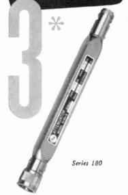
FREQUENCY RANGE: 0.6 KMc to 12.4 KMc ATTENUATION VALUES: 3, 6, 10, 20 db CONNECTORS: Type N — male one end, female the opposite end
