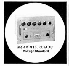
The KIN TEL Model 601A AC Voltage Standard is an exceptionally stable and accurate AC calibration source. It produces AC at 60, 400, or 1000 cps, from 1 to 501 volts. Voltage accuracy is within 0.1% or 5 millivolts; short-term stability, 0.01%. The frequency is stable within 1.0%, and harmonic distortion is less than 0.3%. Output capability is 5 amps up to 5 volts, 25 watts above 5 volts. The output is floating and guarded. Price: \$4500.
