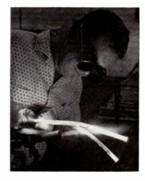
Flame from torch causes tube of imported materials to sag sharply. Domestic tube is affected considerably less.
