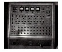
The electrical outputs of any card may be analyzed using simulated inputs while the card is subjected to temperatures ranging from -50 to +185°F, and acceleration loads of 2g and 5g. Minor modification will allow this unit to simulate the pressure and humidity environments as required by card application. Input and output voltages may be monitored and variable input-output loading conditions may be accomplished at the control panel.
