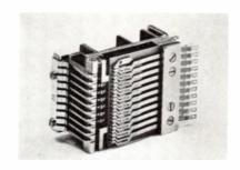
The nominal minimum pulse duration for operation of the device is 20 milliseconds and the minimum interval between pulses is also nominally 20 milliseconds. The actuating winding of the counter is available in both 24- and 60-volt designs with corresponding current ratings of 650 and 324 milliamperes. At the conclusion of each counting sequence, the device is returned to zero by application of a 40-millisecond pulse to a release winding.
