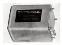
Using all silicon semiconductors and tantalum capacitors, these modules have a temperature rating of -40 to  $+100^{\circ}$ C. Over 90 models are available ranging from 2.8 to 52 volts at powers of 1.0 to 20 watts. Other specifications are as follows: input voltage range -105 to 125 volts, 50–400 CPS.
