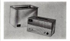
The generator has 150W average power and 600W peak. High efficiency, half wave self rectifying circuit scans transducer producing even cavitation throughout complete cleaning tank. Generator dimensions are 13"×10"×8½".
