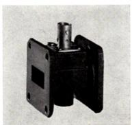
CMC Model X110 operates in the frequency range of 8.2 to 12.4 Gc with typical isolation of 20 db at 9 Gc and insertion loss of 1.3 db. Its switching speed is less than 10 nanoseconds. RF power handling capacity is 4 watts CW and 150 watts
