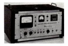
ments, it will continuously indicate the progress and extent to which a reaction has progressed by providing a digital reading of the accumulated charge. With a calibrated ionization chamber the A309B will measure X-ray and gamma radiation intensity and measure the accumulated exposure or dossage over a wide range and for extended periods of time.
