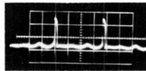
Fig. 4—The voltage waveform across the tunnel diode where N=3 .
