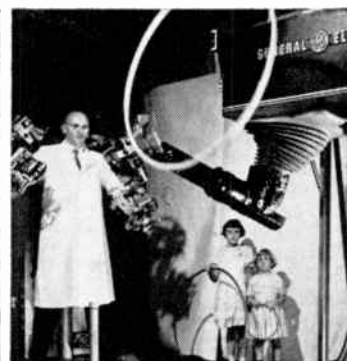
ELECTRO-HYDRAULIC HANDYMAN is an example of remotely operated servo systems being produced to manipulate radioactive materials for routine tasks as well as highly specialized nuclear research projects.
