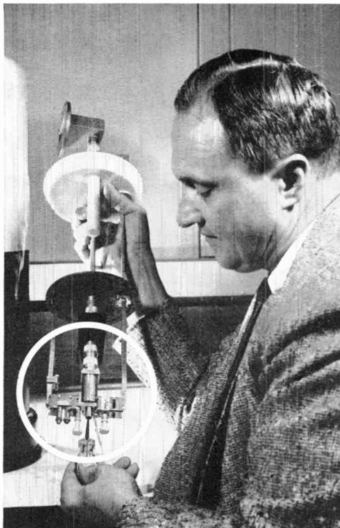
Bell Laboratories' Michael Chroney adjusts waveguide assembly (in circle) housing the diode. After adjustment the entire parametric amplifier will be immersed in liquid nitrogen in dewar at left. The new amplifier operates at 4170 megacycles (center of band) and provides an almost flat gain of 38 db over a 50-megacycle band with a noise figure of approximately 0.6 db.
