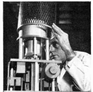
RADIATION EFFECTS OPERATION will use equipment such as this pulsed nuclear test reactor to solve radiation problems. Capabilities exist for both simulation and basic research in radiation effects.
