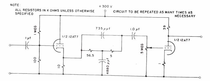
Fig. 7 Schematic Diagram of a One Stage "V" Filter.
