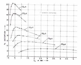
Fig. 9 G. B. Third harmonic distortion vs peak collector current swing, at different values of emitter bias (indicated by DC collector current in AL).
