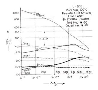
Fig. 5 Incremental Permeability vs. Normalized Air Gap for Class W-01 and W-03 Ferrites. Constant d.c. Bias as Parameters. T = 100° C.
