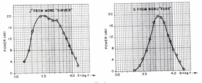
Fig. 1 Power Spectra for Turbulent Sounds
