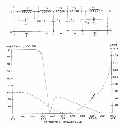
Fig. 9 Theoretical Filter, Channels 7 and 13
