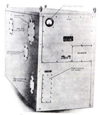
Fig. 12 - Automatic Dehumidifier for Magnetic-Tape-Storage Vault
