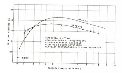
Fig. 4 Wavelength Response Ferrite Heads
