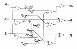
Fig. 1 Block diagram of color television studio masking circuit in which the six independent controls are suitable for ganging to simplify the relationship between manual adjustments and visual effects.
