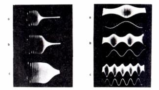
ll.A.(left)  $f_s = 100 - 1500 \text{ cps}$ ,  $e_c$  adjusted for  $f_c = 200 \text{ cps}$  (a), 500 cps (b), 1000 cps (c). ll.B. (right)  $f_s = 500 \text{ cps}$ , sinusoidal control voltage,  $f_{cv} = 5 \text{ cps}$  (a), 10 cps (b), 20 cps (c).
