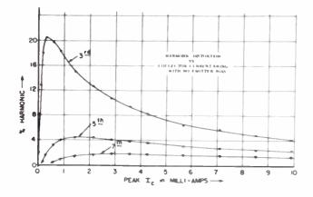
Fig. 7 G. B. 3rd, 5th, and 7th harmonic distortion vs peak collector current swing. No emitter bias.
