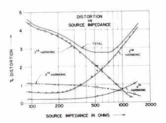
Fig. 13 G. E. Distortion vs source impedance, with emitter bias.
