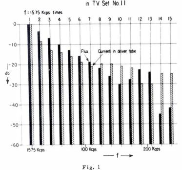
Frequency Spectrum Measured on a Flyback Transformer.
