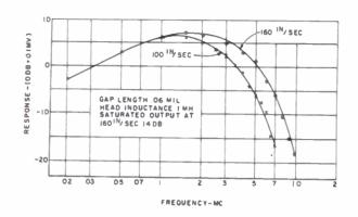
Fig. 5 Frequency Response Head No. 15
