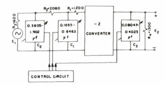
Fig. 3. Simplified Circuit Diagram of Electronically Controllable LP Filter.
