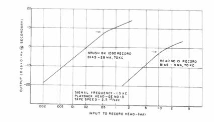
Fig. 6 INPUT-OUTPUT Curves
