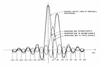
Fig. 3 Response of Ideal Channel to Several Sample Pulses
