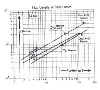
Fig. 4 Hysteresis Losses as Function of Flux Density for Class W-01 and W-02 Ferrites.
