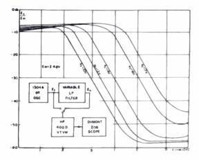
Fig. 13. Response of Electronically Controlled LP Filter for Various Values of Control Voltage ec
