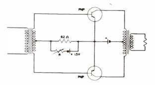
Fig. 12 Class B grounded emitter circuit.
