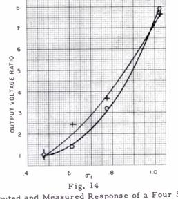
Computed and Measured Response of a Four Stage "V" Filter to Artificially Generated Power Spectra.
