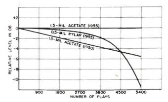
Fig. 8 - Reduction in Level of a 15-kc Signal as a Result of Continuous Replay
