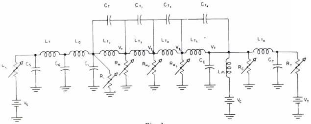
Fig. 2 Electrical equivalent of typical tape transport.
