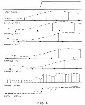
Effect of Skew on System Output Signal
