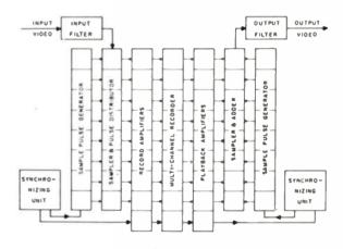
Fig. 1 Block Diagram of 8-Channel Time-Division Multiplex System
