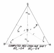
Fig. 8 Trilinear plot showing calculated visual effects from a 0.4 clockwise rotation of the red hue knob of Fig. 6. In this and the succeeding figures, the numbers associated with some of the arrows represent relative luminance values. In this and the succeeding figures, the initial positions of the upper row of control knobs of Fig. 6 are given by equations 4.
