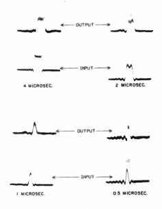
Fig. 16 Pulse Response of a 1.1 mc Magnetic Recording System
