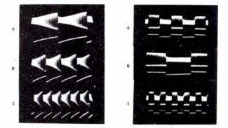
15A.(left)  $f_s = 500$  cps, saw-tooth control voltage,  $f_{cv} = 5$  cps (a). 10 cps (b). 17 cps (c). 15B. (right)  $f_s = 500$  cps, square-wave control voltage,  $f_{cv} = 10$  cps (a), 5 cps (b), 20 cps (c).
