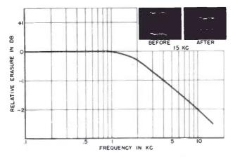
Fig. 7 - Erasure of Recorded Energy as a Result of Contact with Paper Timing Tape
