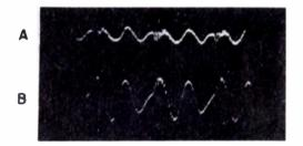
Fig. 21. Filtered (A) and Unfiltered (B) Samples of the Sound "i".
