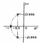
Fig. 2. Pole Pattern for Butterworth LP Filter.
