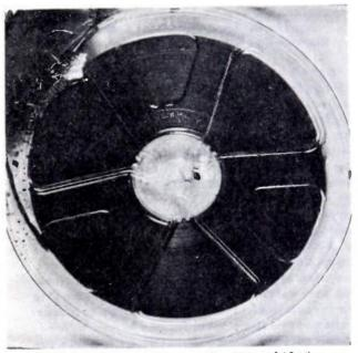
Fig. 10 - Effect on Boxed Recording Tape of 15-Minute Exposure to Direct Flame, Cover Removed
