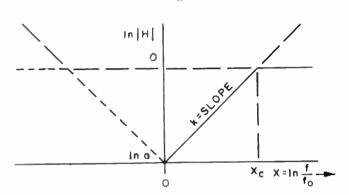
Fig. 3. Network Characteristic of the "V" Filter.
