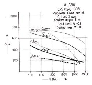
Fig. 6 Incremental Permeability vs. Flux Density for Class W-01 amd W-03 Ferrites. Constant d.c. Bias as Parameters at T = 100° C.
