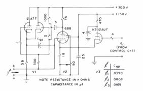
Fig. 7. Gircuit Diagram of Electronically Controllable Capacitors.
