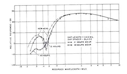
Fig. 10 Effect of Wear Resolution, Ferrite Head No. 10, Wear at 100 in/sec
