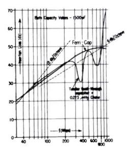
Fig. 11 Insertion Loss Vs. Frequency for a "Ferri-Cap" and a "Standard" UHF Filter.
