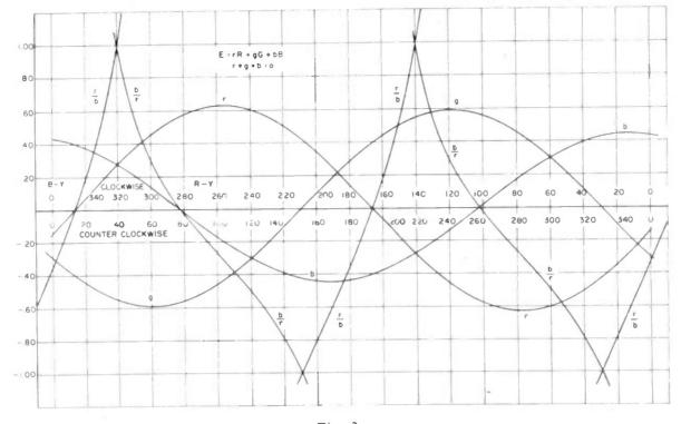
Fig. 2 Graphical Representation of the Chrominance Demodulator Output
