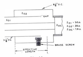
Fig. 10 Coaxial Shunt m-derived Terminating Half-Section
