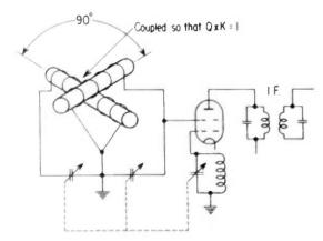
Fig. 8 Semischematic Diagram of an Omnidirectional Ferrite Antenna.
