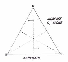
Trilinear plot showing qualitatively the Fig. 2 visual hue and saturation effects associated with a change in a single masking coefficient, a12.
