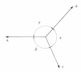
Fig. 1 Vector Diagram of the Output of a Synchronous Demodulator at Different Angles
