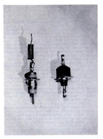
Fig. 10 Photograph Contrasting a "Ferri-Cap" and a "Standard" UHF Filter.
