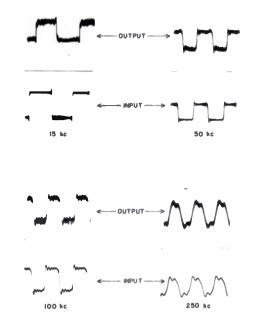
Fig. 15 Square-Wave Response of a 1.1 mc Magnetic Recording System
