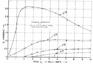
Fig. 10 G. B. Odd harmonic distortion vs peak collector current swing, with 95 A DC flowing in each collector as a result of emitter bias.
