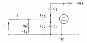
Fig. 6. Principle of Operation of Electronically Variable Capacitor.
