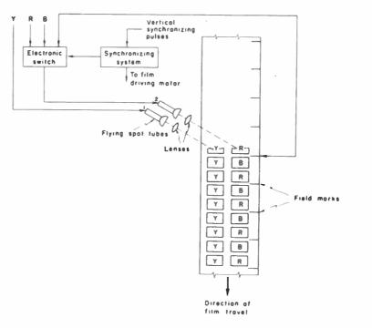
Fig. 12 Continuous motion kinescope recorder for color television
