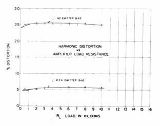
Fig. 11 G. B. Harmonic distortion vs amplifier load resistance.
