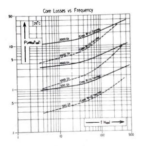
Fig. 3 Frequency Dependency of Hysteresis Losses for Class W-01 and W-02 Ferrites.
