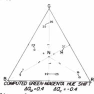
Fig. 10 Trilinear plot showing calculated visual effects from a 0.4 counterclockwise rotation of the green hue knob of Fig. 6
