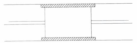
Fig. 2 Overlapping of the Dielectric in the Low Impedance Section to Provide Longer Voltage Breakdown Path
