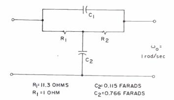
Fig. 6. Bridged "T" Form of "V" Filter for k = 1.
