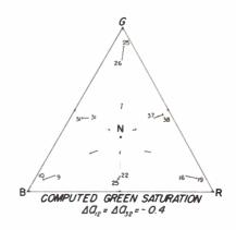
Fig. 11 Trilinear plot showing calculated visual effects from a 0.4 counterclockwise rotation of the green saturation knob of Fig. 6.
