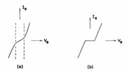
Fig. 8 (a) Input characteristic: emitter current vs emitter voltage, with no emitter bias.
