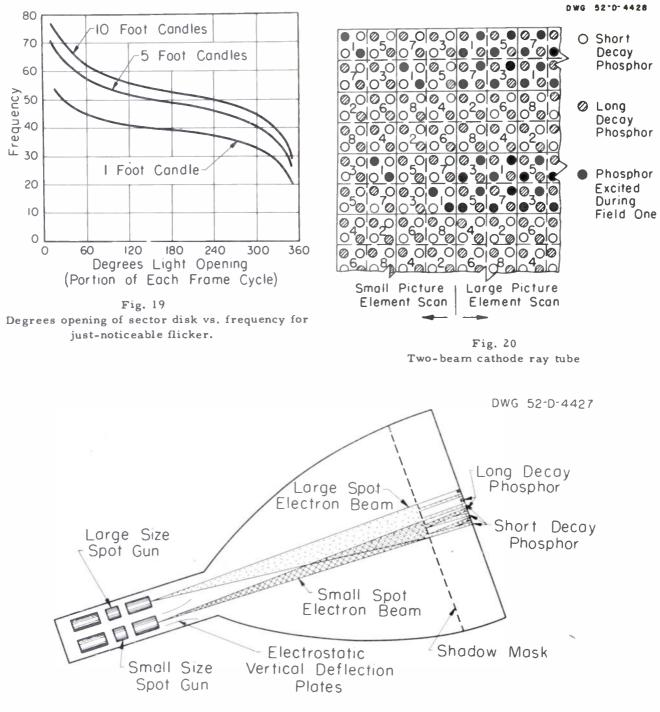
Fig. 21 Portion of faceplate of display device
