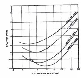
Fig. 4 Minimum perceptible per cent flutter for oscillator tones in small auditorium.
