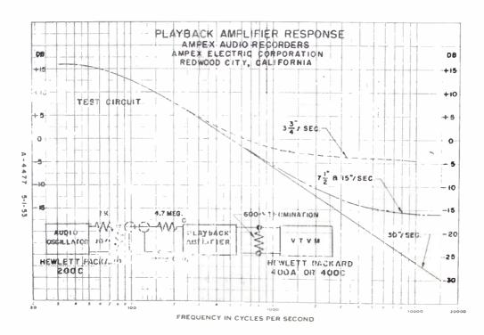
Fig. 6 Playback Amplifier Response.
