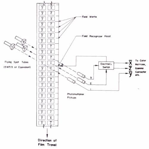
Fig. 1 Continuous film scanner for color television
