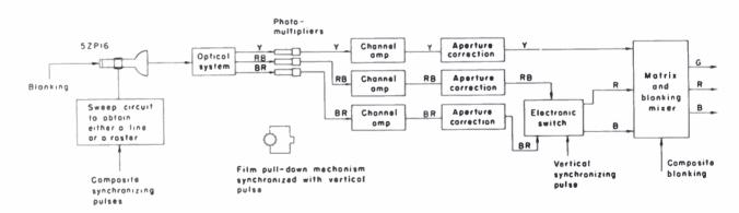
Fig. 3 Basic electronic system.
