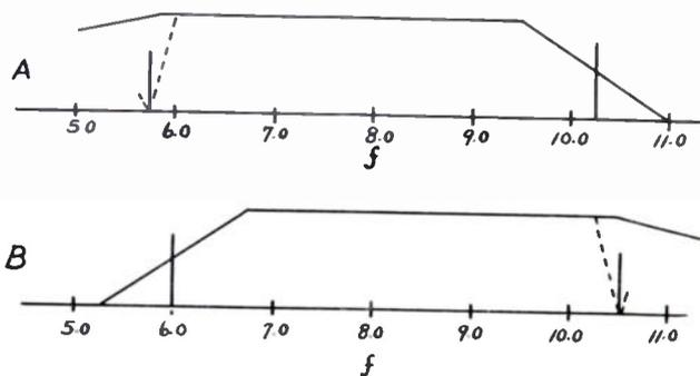
Fig. 4. I.F. Response, ideal amplitude curve.
