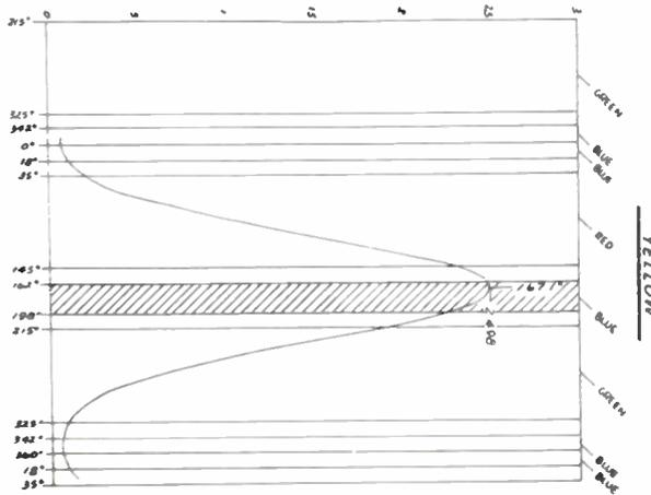
Fig. 10. Quadramatic decoding beam current waveforms.
