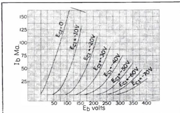
**FIG. 5** Plate family characteristic curves for the Type 10DE7
