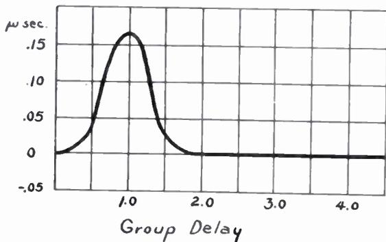
Fig. 3. Group delay of filter having response of Fig. 2.
