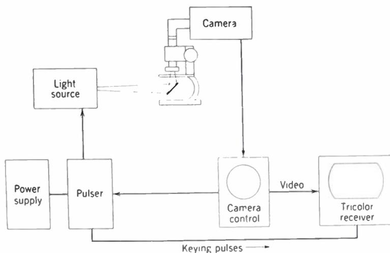
Fig. 1 General Block Diagram of Television Color Translating Microscope.
