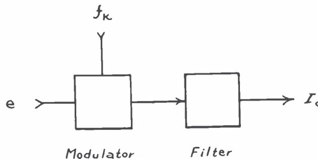
Fig. 1. Block diagram of product detector.
