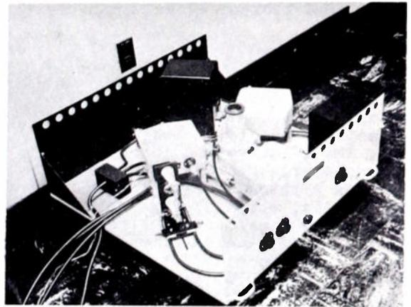
Fig. 4 Illuminating System of Television Color Translating Microscope with Three Sources
