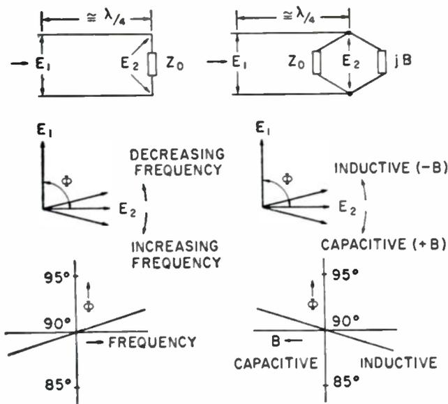
Fig. 12—Phase delay as a function of freq.  $\lambda/4$  shunt loading in  $\lambda/4$  transmission line.
