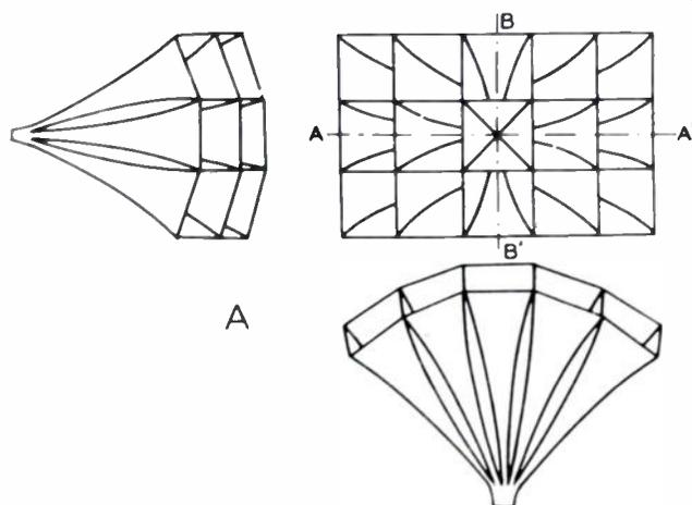
Fig. 1. A spherical radiating surface consisting of 15 individual exponential horns. The mouth of each horn is 8 inches square. Each horn subtends an angle of 17 degrees, both horizontally and vertically.
