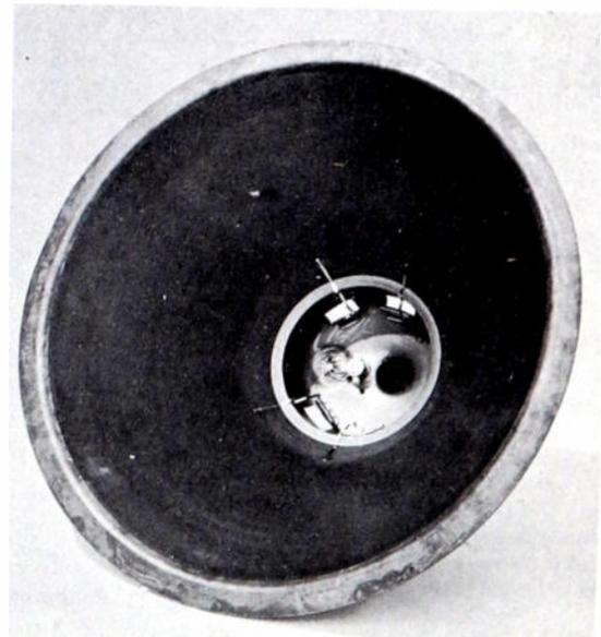
Fig. 5. Flood gun mounted in the funnel section.
