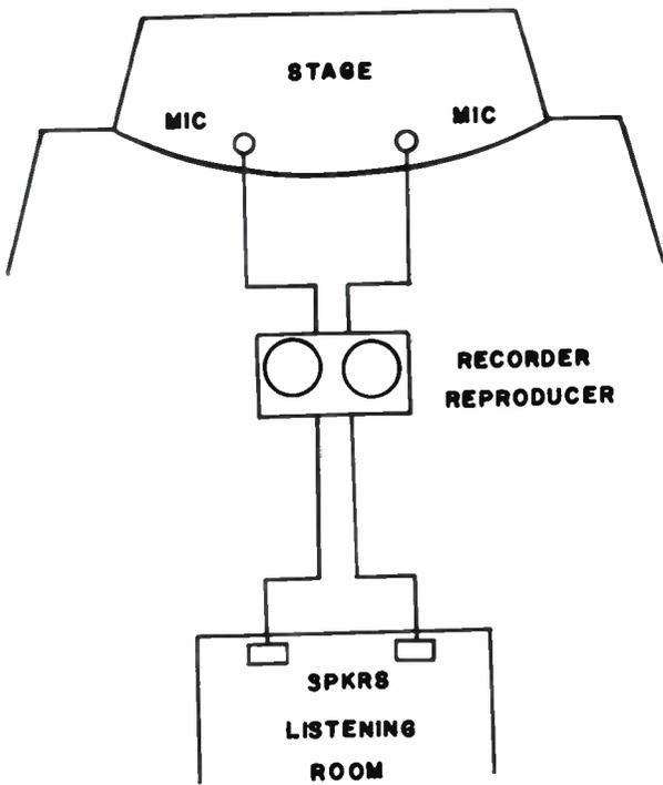
Fig. 3. Two-channel stereophonic system.
