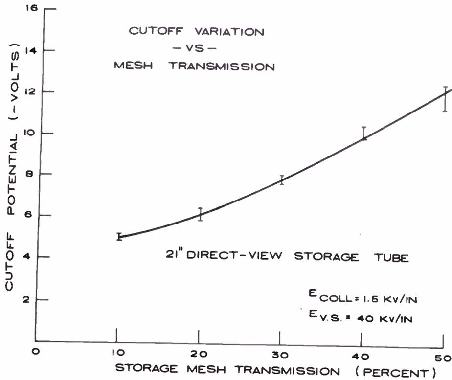
Fig. 8. Cutoff variation with storage mesh transmission.
