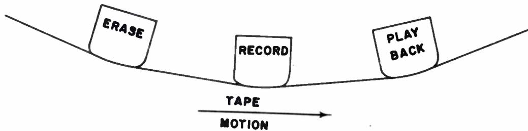
Fig. 1. Normal head arrangement.
