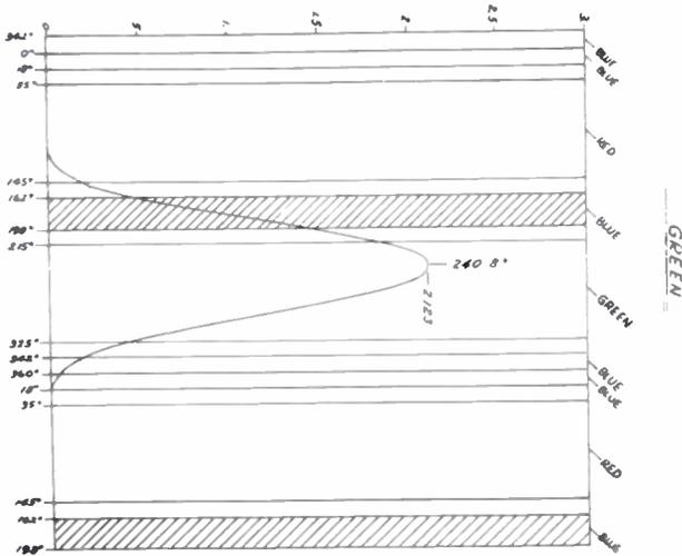
Fig. 9. Quadramatic decoding beam current waveforms.
