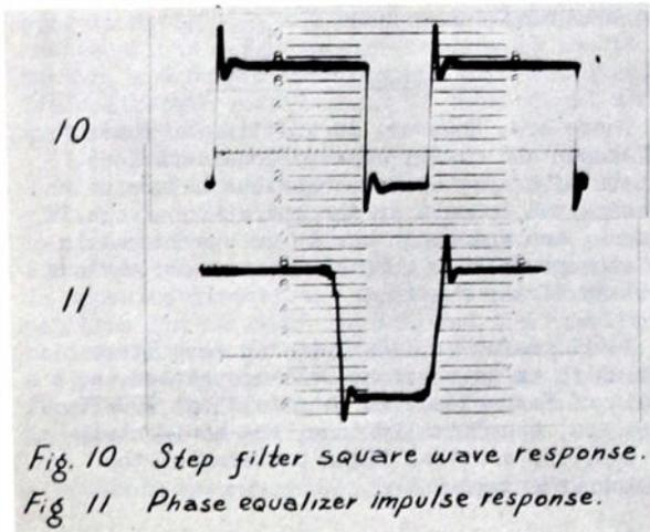
Fig. 10 Step filter square wave response.
