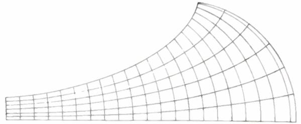
Fig. 5. Revised version of horns showing construction lines used in drafting. The horns are identical to those in Figure 4.
