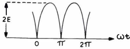
$$e = \frac{4}{\pi} E \left( 1 + \frac{2}{3} \cos \omega t - \frac{2}{15} \cos 2\omega t + \frac{2}{35} \cos 3\omega t \dots \right)$$
