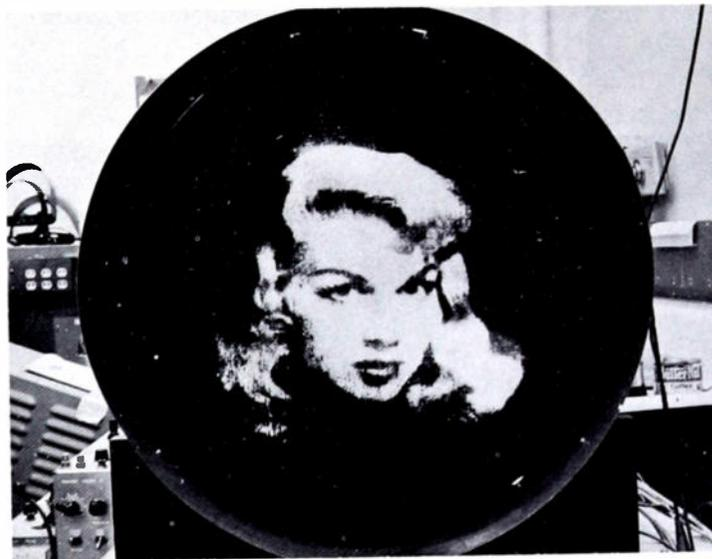
Fig. 12. Slow-scan TV picture on 21-inch Tonotron tube.
