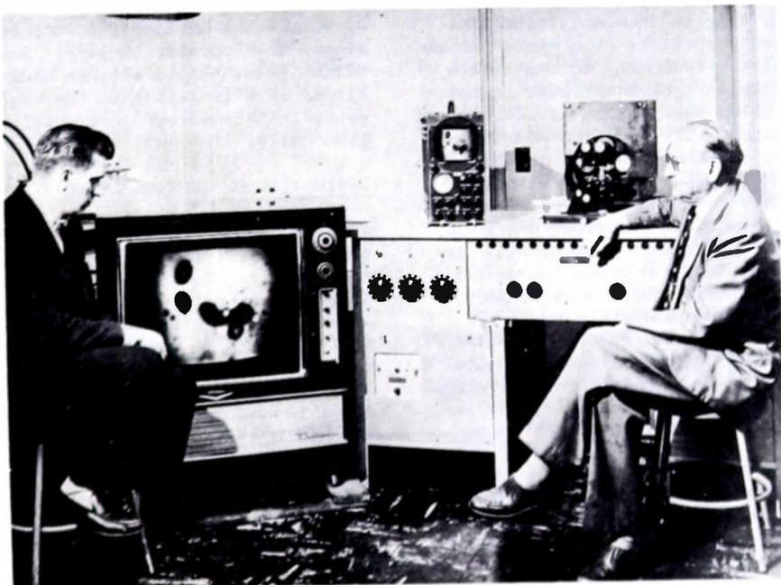
Fig. 7 The Complete Television Color Translating Microscope with Image Orthicon Camera.
