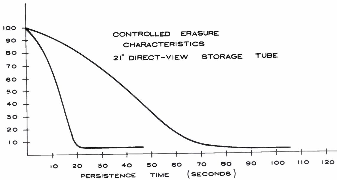
Fig. 11. Controlled erasure curves.
