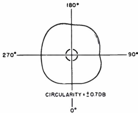
Fig. 8—Measured horizontal pattern of bottom quarter of gain of 18 antenna. 18-inch diameter, 30-foot length, channel-10.
