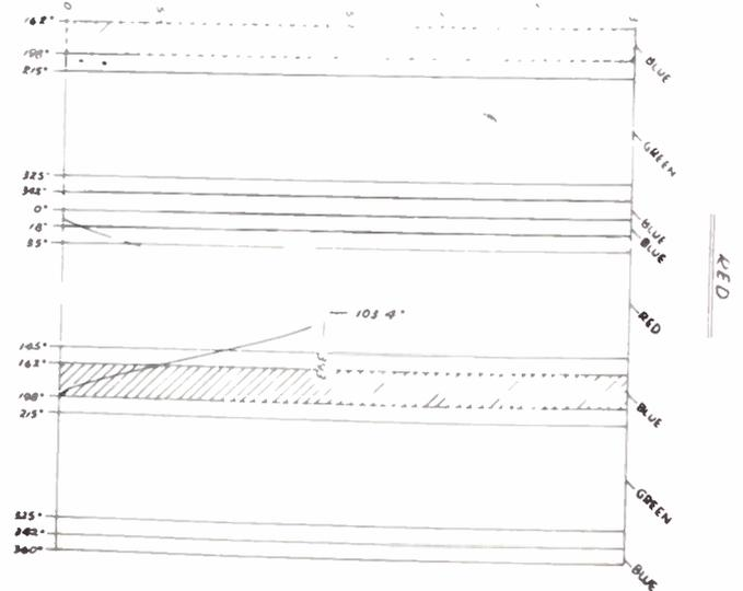
Fig. 7. Quadramatic decoding beam current waveforms.
