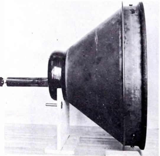
Fig. 9. 21-inch Tonotron tube.
