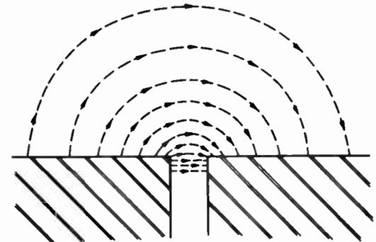
A. MAGNETIC FIELD PRODUCED BY GAP
