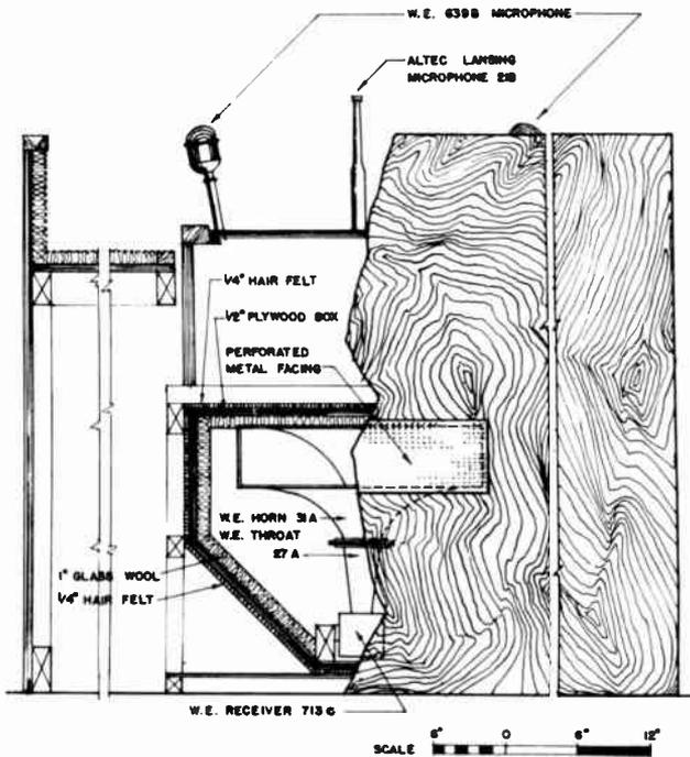
FRONT ELEVATION WITH PORTION OF FACING REMOVED TO SHOW CONSTRUCTION
