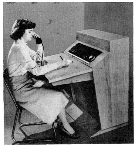
Figure 11-Operator's position handling up to 16 trunks and 2 operator's lines.
