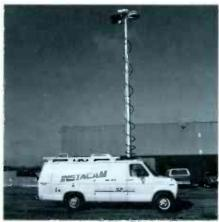
Will-Burt's Model 6-25-357/367 pneumatic telescoping mast.
