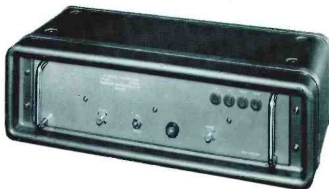
Fig. 4. A.F. Signal Compressor, Type TM 6629, used for limiting external a.f. modulating signals
