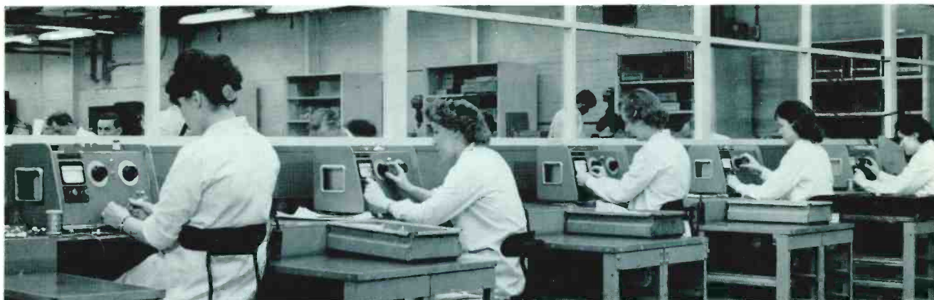
Operators adjusting resistors for the \frac{1}{4}\% Universal Bridge, TF 1313, using the special bridges made for the purpose
