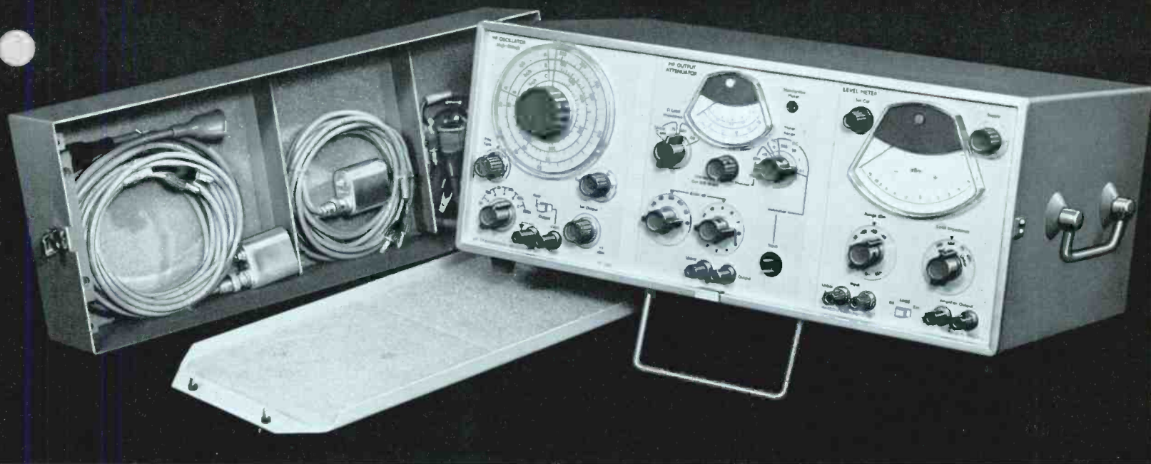
TF 2333 Transmission Measuring Set comprises (from left to right) an oscillator, a monitored attenuator and a level meter. It is supplied with a splash-proof front-panel lid which also provides neat stowage for a comprehensive set of measuring leads
