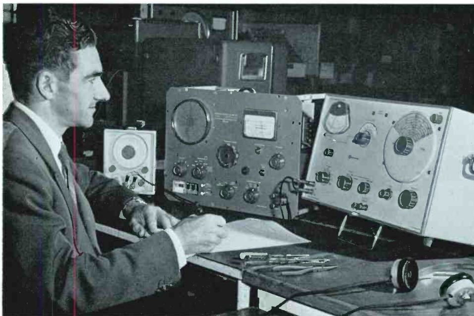
Utilizing the low distortion output of the A.F. Oscillator to test the l.f. amplifier of Carrier Deviation Meter TF 791D
