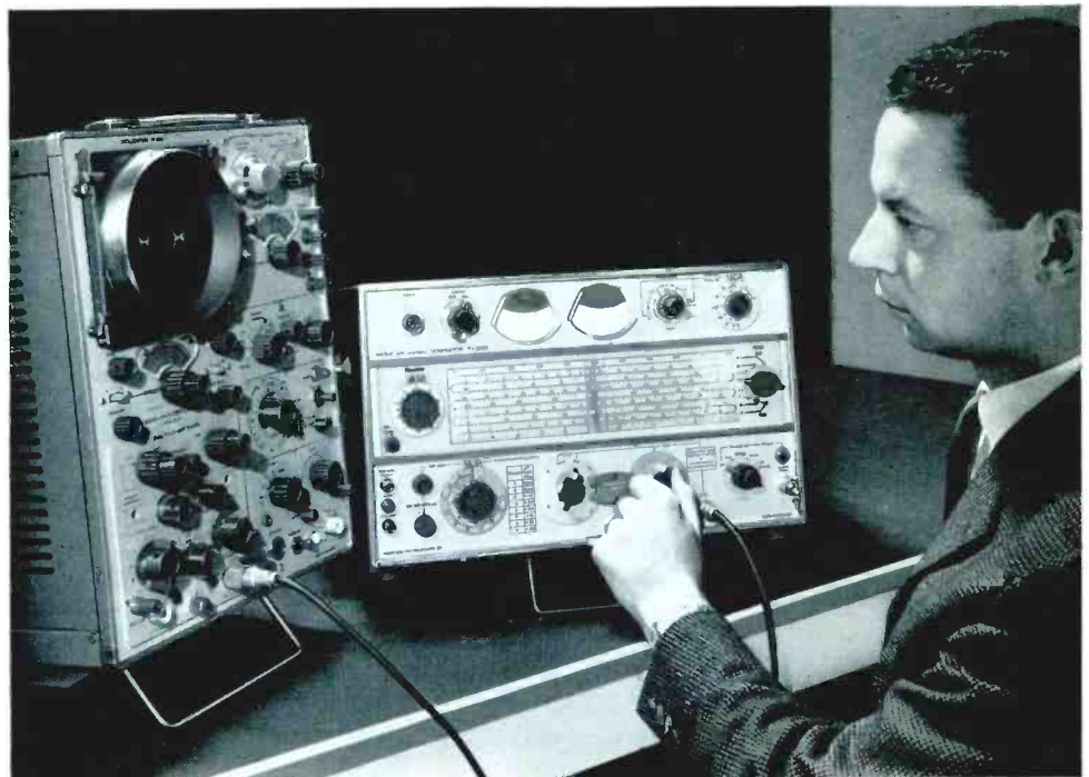
A 100% modulated r.f. output signal from the generator being viewed on the Oscilloscope type TF 2200
