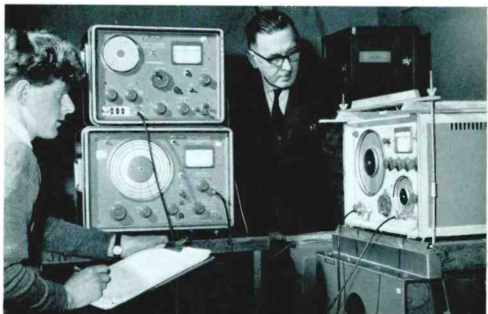
Prototype model of TF 1060/3 being subjected to the mechanical bump test. Here the frequency deviation of the output signal is being monitored with a Carrier Deviation Meter type TF 791 D
