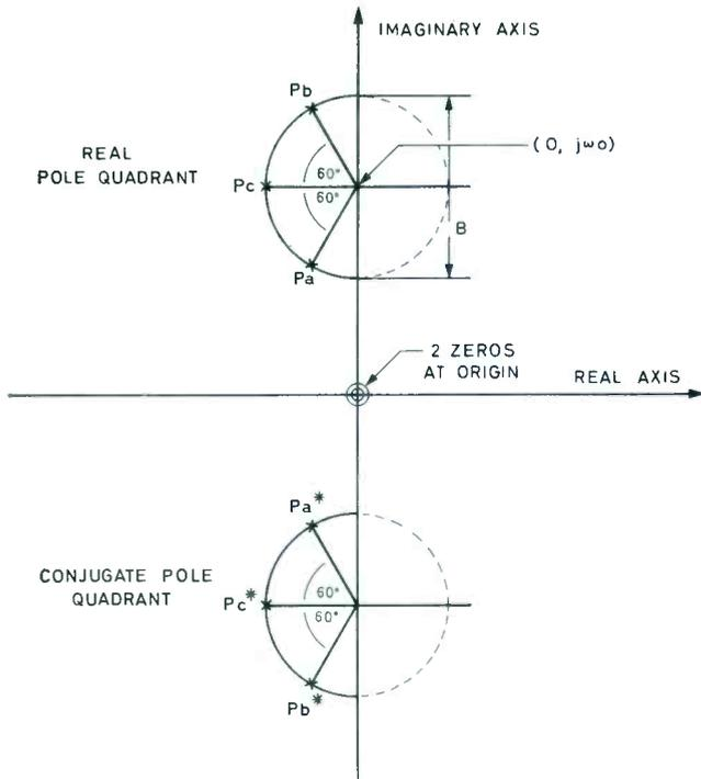
Fig. 5. Complex frequency plane representation of maximally flat response
