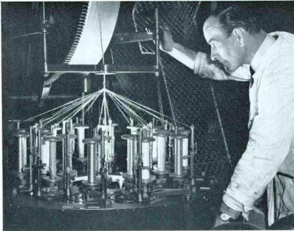
In the manufacture of coaxial cables complex machines are required, such as this one which forms the outer screen
