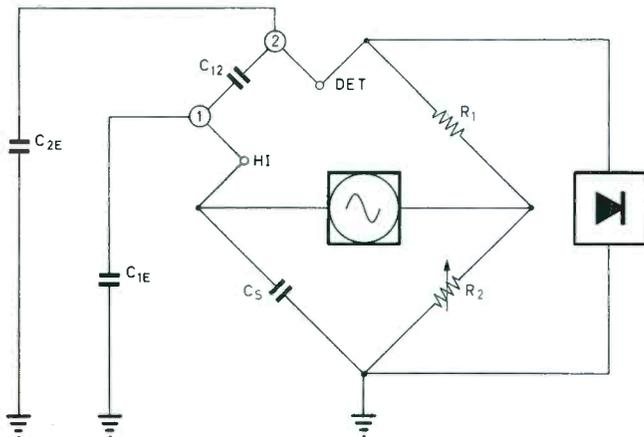
Fig. 2. Network connected to bridge terminals
