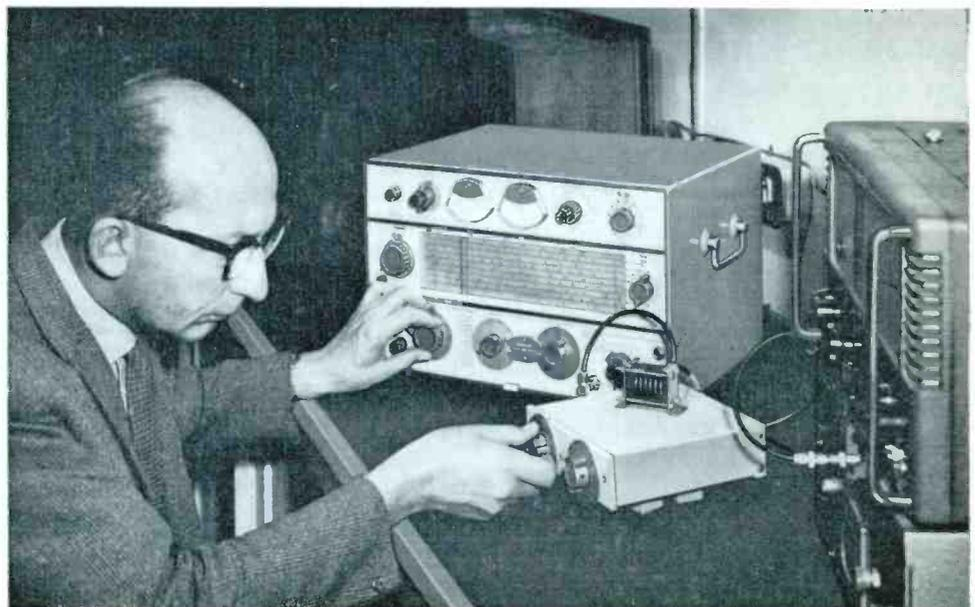
*This coaxial transformer is used in our Standards Laboratory when testing the attenuator of the new TF 2002 Signal Generator*
