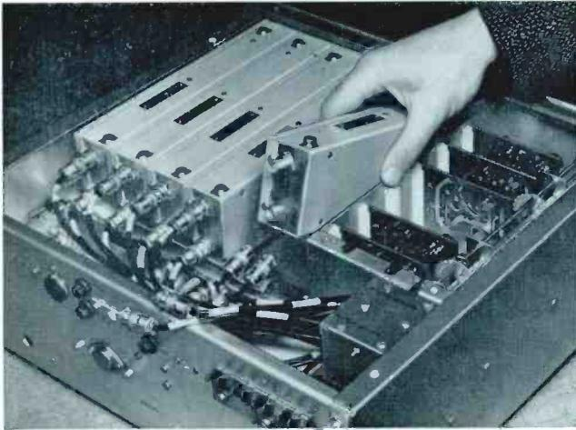
The receiver accommodates up to six band-pass filters which are switch-selected at the front panel. New filters can be readily fitted as shown above
