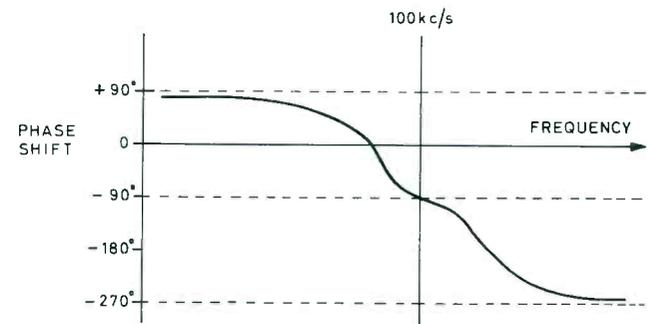
Fig. 9. Phase response of double crystal filter of Fig. 4 (a)
