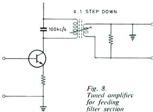
Fig. 8. Tuned amplifier for feeding filter section
