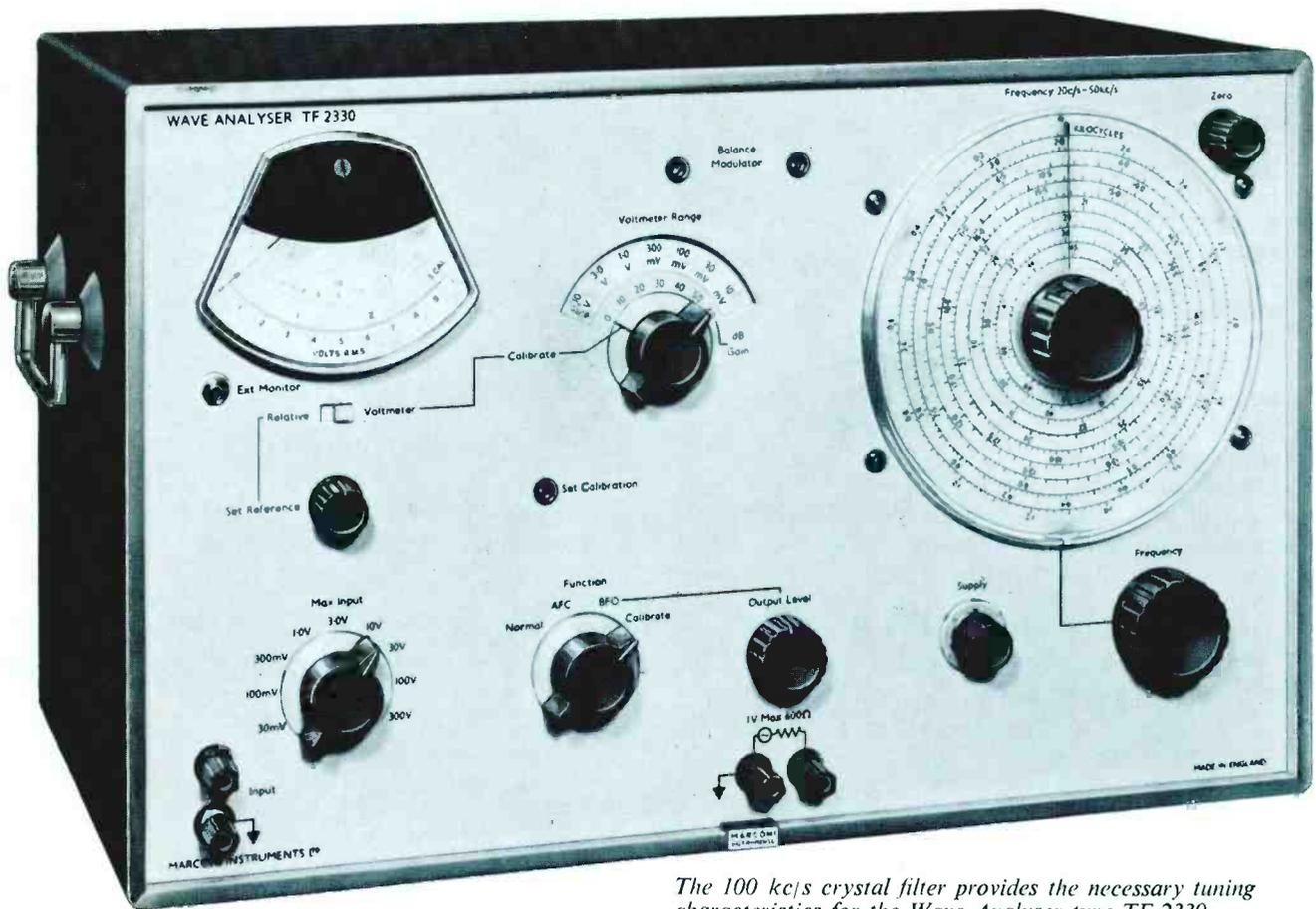
The 100 kc/s crystal filter provides the necessary tuning characteristics for the Wave Analyser type TF 2330
