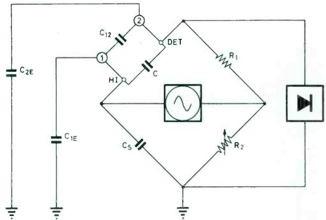
Fig. 3. Network plus auxiliary capacitor across bridge terminals
