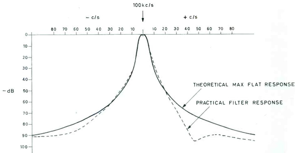
trimmer capacitor of the single crystal filter is adjusted to obtain maximum flatness of response.
