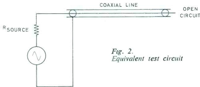
Fig. 2. Equivalent test circuit
