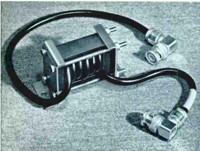
Fig. 1 (above). The coaxial transformer consists of six turns of cable on a ferrite core
