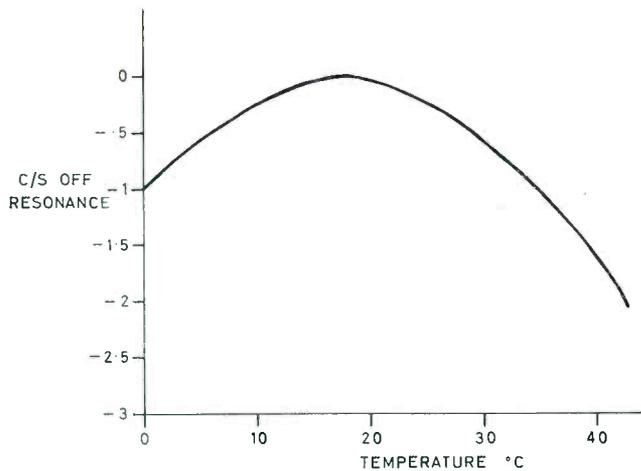
Fig. 3. Resonant frequency variations of crystal 0°X cut bar with temperature
