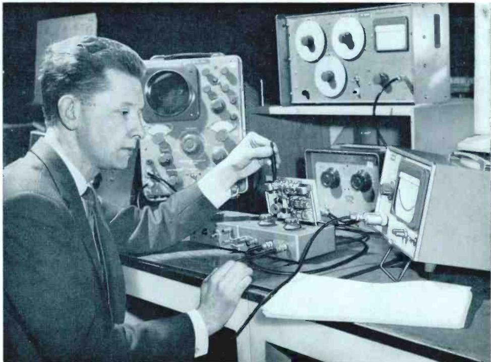
Setting up a 100 kc/s crystal filter with the aid of a high-discrimination oscillator, oscilloscope and voltmeter
