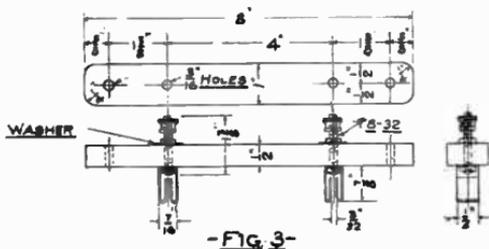
make two brass rods with 8-32 threads on each end. the rods to be  $1\ 3/8$  inches long. Provide two nuts and a washer and also a battery knurl for each and set together in the inside holes of the 8 inch piece of rubber, as shown in Fig. 3.
