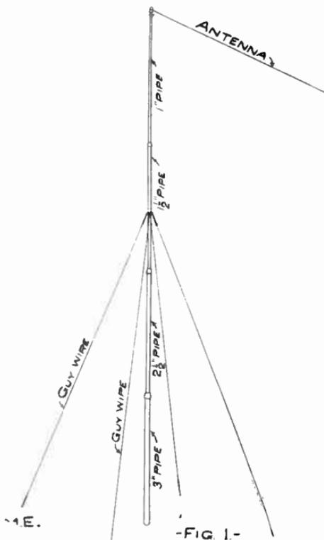
wires (Fig. No. 1), but if it is to be raised 80 or 100 feet, it will of course need two sets, one near the top, the other approximately half way down (Fig. No. 2).
