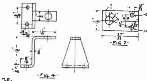
care must be taken in the making of this part, and twice out of every three times it will be necessary to make it over again, for the reason that silicon differs, one piece not being as sensitive as another in the detection of the waves.
