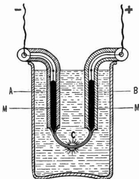
put into a vessel containing water, which serves to constantly cool C, which part would soon break in the open air. Connect the two wires with two small storage cells, and the interrupter will start instantly. In the middle of C there will be a bright bluish-green spark, and a high-pitched tone will emanate from the interrupter, indicating that the interruptions are of high frequency.
