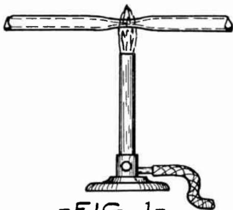
The material needed is a piece of thermometer tubing about three inches long, having a bore of not more than  $1/64$  inch diameter, two pieces of platinum wire, one  $1/2$  inch long and  $.001$  inch diameter, the other  $3/8$  inch long, of No. 20 or 24, a piece of glass tubing
