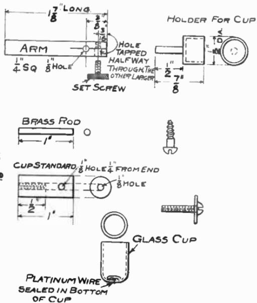
In the standard 1 3/4 inches from the bottom drill a 1/16 inch hole 1/8 inch deep, and drive into it a short pin, allowing about 1/16 inch to stick out. This piece fits in the slot of the brass tubing.
