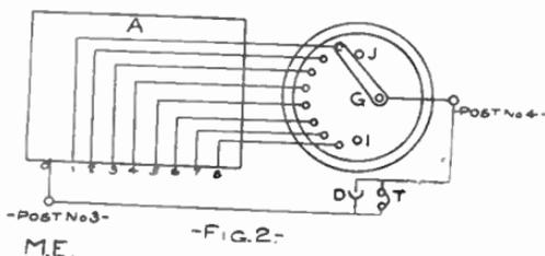
detector if desired. The wiring diagram is for so-called thermo-electric detectors. If an electrolytic is used, a battery and potentiometer must be used and connected as shown in diagrams of previous issues of "M. E."
