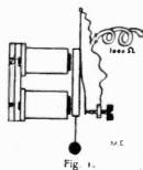
You have now a double wire, which you can wind on a small spool. The two ends are connected to the contact points of the decoherer (Fig. 1), The idea of winding a double wire on one spool, or as commonly called bifilar winding (Fig. 2), is to destroy all inductance and all electro-magnetism. Each wire tries to destroy the effects of the other, which is necessary for the work this resistance is intended to perform.
