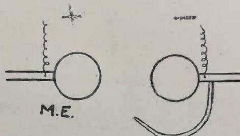
If the distance is well selected, the intensity and general appearance of the spark is not changed; the regularity of the discharge, however, is increased over 100%.
