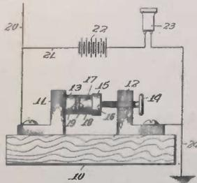
1. A coherer for a receiving instrument of the class described, comprising a loose, dry mechanical mixture of fine particles of zinc and carbon.
