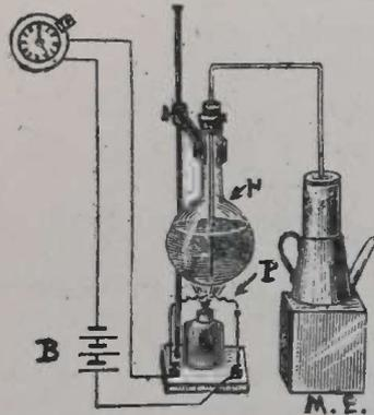
Let us suppose you have to be up by 5 o'clock in the morning. In that case the contact brass strip is glued to the dial at that point, which is reached by the hour hand at 10 minutes *before* five. The alarm itself is set for 5 A. M.
