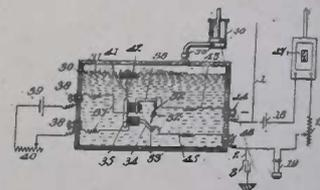
1. Receiving apparatus for space signaling by Hertzian oscillations, comprising a conductor arranged to be excited by said oscillations, relatively movable conducting surfaces in close proximity to each other, means normally separating said contacts but permitting contact when said oscillations are received on said conductor, said means re-establishing said separation after the passage of each oscillation, and means to damp the movement of said surfaces.
