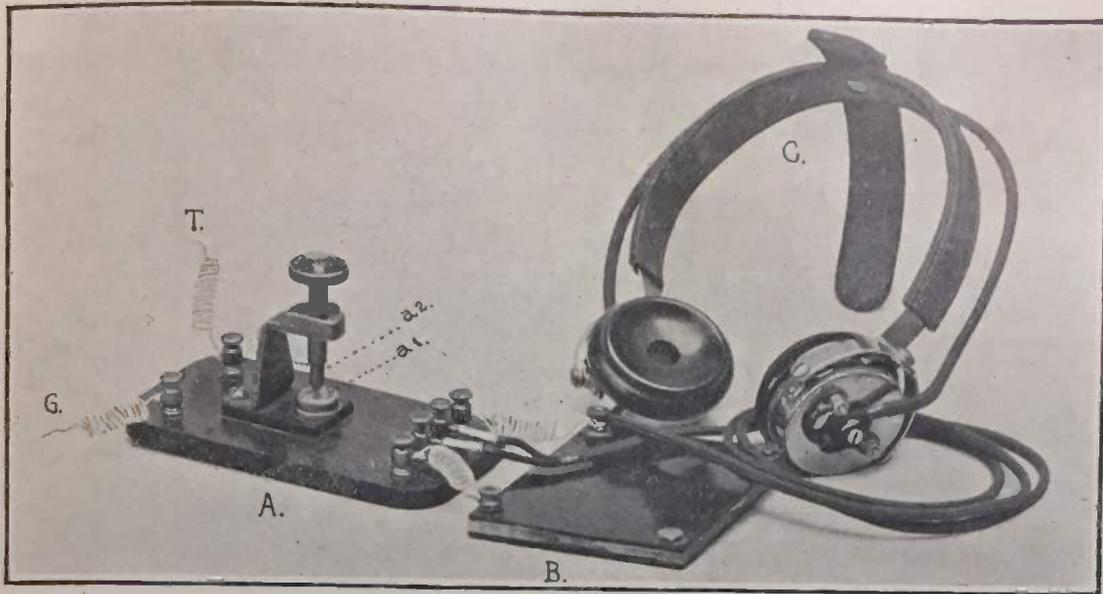
About a year ago the writer had the opportunity of examining a Pickhardt Silicon Detector, and after listening to it in operation, decided to build one himself. The operator, a friend, explained the action of the detector in detail, saying in part there were no batteries to run down, that the adjustment was very easy, and when once adjusted it could be depended upon not to get out of order, and that the connections were very simple.
