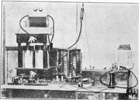
The receiving instruments consist of a receiver which has tuning coils, two detectors, one electro-lytic and one carborundum type, variable condenser and rheostat, all made by myself and mounted on and in this box which makes it portable. The phones and batteries
