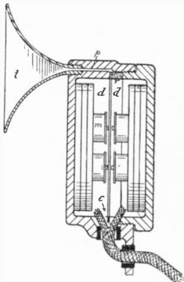
formed between the two diaphragms. At the upper part of the pasteboard ring a small piece is cut out. At this point a small channel p ends, which is in communication with the funnel t.
