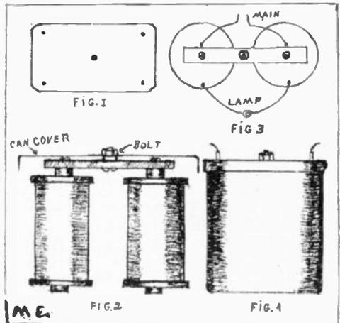
one inch in diameter with a quarter of an inch round hole in the center; these are fitted on the magnet cores at each end.
