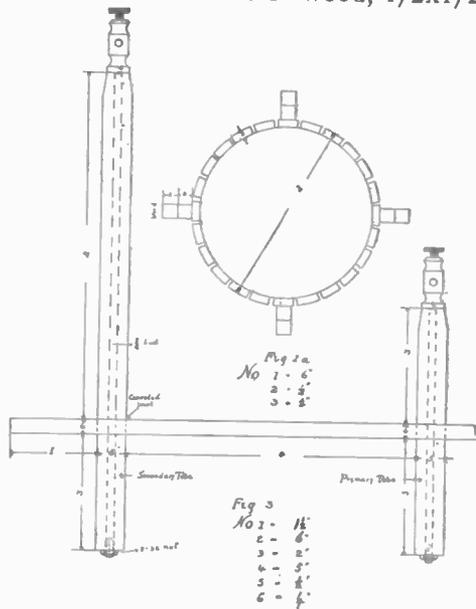
1 inch at equal distances from each other, on each end of the coil, so as to form supports for four sticks, 1/2x 1/2x17 inches, running lengthwise on the coil, and separated from the secondary wire, on which to wind the primary coil.
