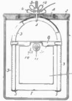
1. In a voltaic battery, the combination with an inverted U shaped hanger of a copper oxid plate supported in said hanger, a cross piece secured to the sides of said hanger and zinc plates secured to said cross-piece but in insulated therefrom.
