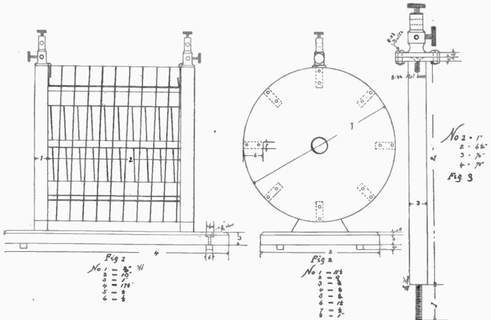
Some few months ago the writer constructed an inductance, or tuning coil for the transmitting circuit, which has proved very efficient, making possible the use of many different wave lengths in transmitting, either with open or closed circuits, and opening up a wide field of experimentation in tuned transmission in which many interesting phenomena have been noted.
