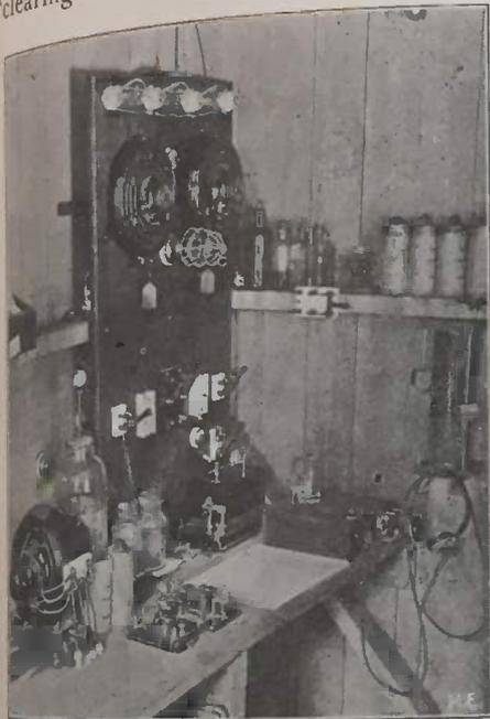
On the front side of the box is a pole changing switch to throw in my coherer and relay outfit, seen in front of the dynamo. I only use this set for calling purposes, as I find the electrolytic much more sensitive, and capable of receiving messages with greater speed.
