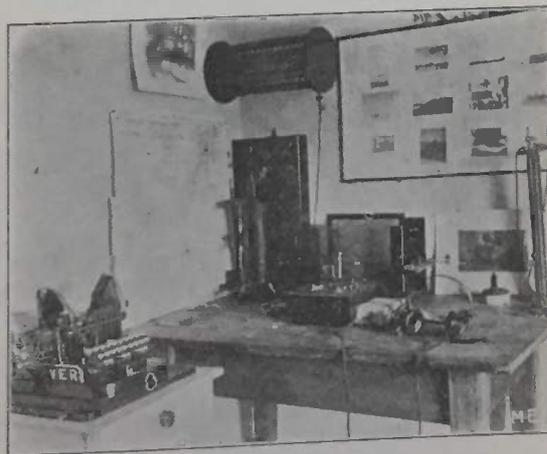
On the extreme right is a small tuning coil, used in connection with the detector.
