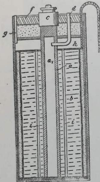
sistance of only 10 ohms. At the beginning of test the voltage was 1.60. The test was started February 29, 1908. The cell was never disconnected from its resistance and consequently never had a chance to recuperate. Despite this when a reading was taken on July 6, 1908, the voltage was still 1.18. The total capacity of the battery, consequently, was 163 ampere hours, which is a remarkable showing for a dry cell.
