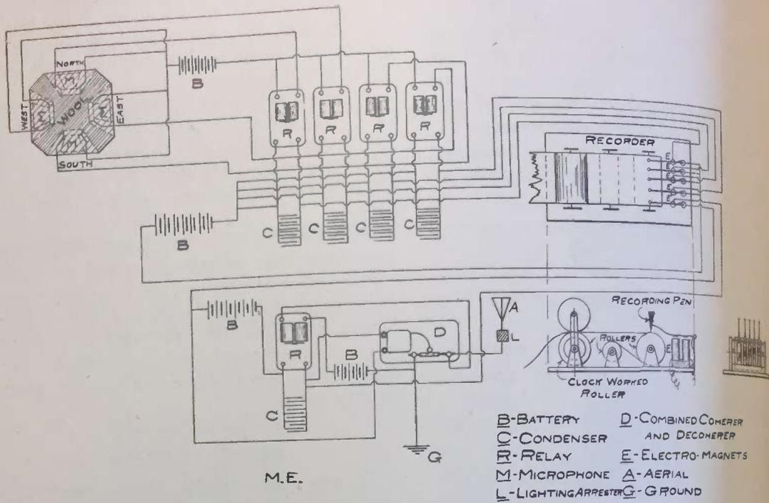
This apparatus is designed to show in what direction and approximately how far off lightning takes place.
