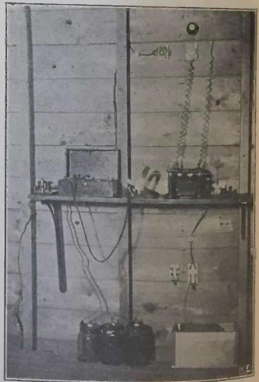
power for the induction coil, and a set of spark balls on hard rubber stands. These stands I made out of the shells from two old telephone receivers, and two binding posts. They can be seen in the picture directly in front of the induction coil.
