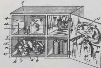
1. A machine of the character described comprising a normally open electric circuit, a camera adapted to use photographic plates, means for operating the shutter mechanism of said camera, an arc in the aforesaid electric circuit, fusible means adapted to hold said shutter operating mechanism in inoperative position and extending in the path of said arc, and means for closing said circuit to complete the arc therein.
