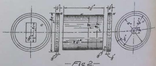
Fig. 2 shows the details of the muffer. The ends, G and H, are both made of hard rubber, and have annular grooves 1/8 inch deep, turned in their faces, which set the ends of the glass cylinder, F. The end, G, has an aperture of the size given, cut out of its centre, enabling it to pass over the brass cylinder, J, and fit tight up against the piece, C.
