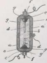
1. In a device for use as a resistance in an electric circuit, in combination, a closed conducting metal envelop, particles of a resisting material filling said envelop and two terminals extending through and insulated from opposite ends of the said envelop and embedded in the said particles.
