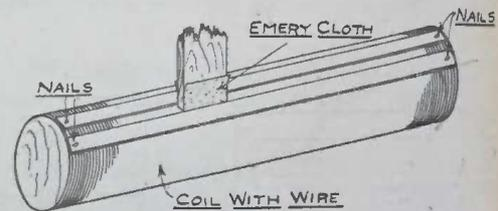
was rubbed up and down the groove made by the laths until the insulation had been scraped away by the emery paper. The laths were then removed and the result was very satisfactory.
