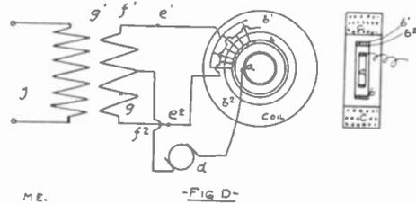
field. The effect is extremely rapid and comes to some thousands of turns per second if the arc is a strong one. The arc thus passes from b1 to b2 in a very short time, and on account of the connection of these segments with the transformer we have an alternating current in f1 f2 and a succession of current inversions which is extremely rapid, so that we take off a high frequency current from the secondary j.
