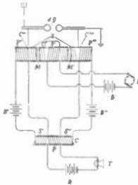
1. In a system for the transmission of sound-modulated electric radiant energy a pair of secondaries of a sound-controlled primary, a pair of primaries connected with the said secondaries, a primary generator of high frequency currents, a secondary connected with the conductors of electrical oscillations all substantially as set forth.
