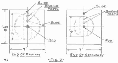
probably be made clear. With two sliders on the primary very fine tuning can be accomplished, and the slider on the secondary will also be of help.
