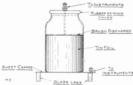
Upon assembling the condenser plates, tinfoil and lead ins, it should be treated with the greatest care, for in the "casting" lies the efficiency of a condenser. A plate glass condenser to produce maximum results should be boiled in a non-hydroscopic solution till all moisture is
