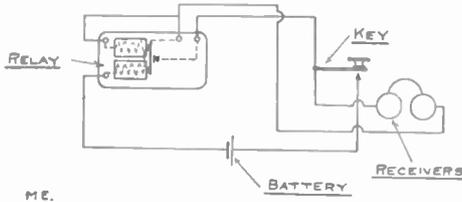
upon the ordinary buzzer. With the relay buzzer students can send and receive in the same room without "interference" to one another.
