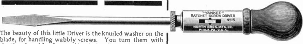
The beauty of this little Driver is the knurled washer on the blade, for handling wabby screws. You turn them with the thumb and forefinger while the handle steadies the blade until they are well set then using the Ratchet movement. A fine Driver for small wood screws, but especially useful for electrical work and work on small machinery, like sewing machines, typewriters, adding machines, etc. A nice tool for the pocket.
