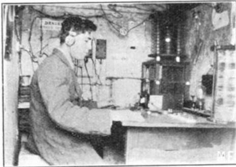
on top is the helix of twelve turns of No. 8 brass wire, inside is the zinc spark gap with muffler. My hand is on key operating transformer, spark can be seen through hole in muffler.
