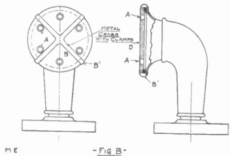
practice shows that the contrary effect takes place, and that the action of the voice on the diaphragm is increased in a marked degree. The exact reason for this effect is not clear, but we may suppose that it is due to some extent to resonance which occurs in the chamber in front of the diaphragm, as this is now practically closed. The disc A can be made of various materials such as wood, ebonite, or celluloid. A good method is
