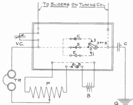
TRICS. All the binding posts, switches, etc., are mounted on a board of convenient size (about 12 x 15 inches). The dotted lines show how binding posts are wired on under side of board. In center of board is shown a three-point switch with which either of the three detectors, electro-lytic, silicon or carbon-dum, may be thrown in circuit.
