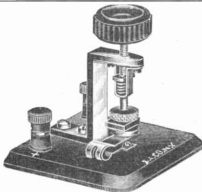
**The Famous Peroxide of Lead DETECTOR.** A dry electrolytic. More sensitive than silicon or carborundum. Postage of 12 cents must be added. Detector sells for \$1.00.
