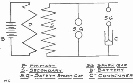
connected across the same terminals with the spark gap "S' G," as shown in diagram, with another spark gap "S' G'" a trifle smaller than "S' G," so that the spark will jump here instead of the other.
