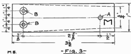
base K, Fig. 1. For an upright L, Fig. 1, take a piece of wood and cut it into a piece 3 1/2 inches by 1 inch by 3/4 inch, as Fig 3. To relieve the stolid looking
