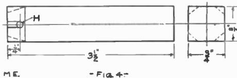
3/4 inch by 3/4 inch. If a turning lathe is not handy, they may be made round by first changing the square into an octagon by planing, then a 16-sided polygon, etc., till finally a very good circular piece is obtained. A hole is bored, H, Fig. 4.
