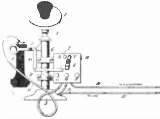
1. In a combined telephone and telegraphone system, the combination of a telephone line adapted for inter-communication, a telegraphone, means for connecting the telegraphone with the telephone line for recording the telephone conversation, a telephone receiver and a switch whereby said receiver may be used at will for ordinary telephonic communication or for listening to a record of the telephone conversation.
