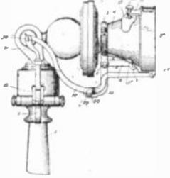
1. The combination with the mouthpiece and receiver arm of a telephone, of a disinfectant holder movably supported in front of said mouthpiece and adapted to open and close by gravity, and a pivoted lever in connection with said telephone and actuated by said receiver arm to give said holder sufficient impetus to move.
