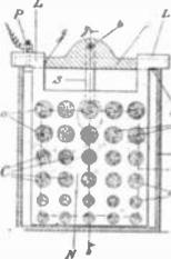
1. A battery element, composed of a malleable iron plate having apertures disposed generally therein, and extending therethrough, and a series of compressed oxid of copper plugs forced under intense pressure into said apertures.
