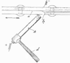
1. The herein described method of welding, brazing or soldering with an electrode containing soldering material consisting in passing a current to form an arc between the electrode and the parts to be welded and then moving the electrode in a line parallel to the part where the solder is to be applied while held at a sharp angle to the line of movement, so that the soldering material will pass from the electrode in a continuous stream and be applied in rows and layers to the parts to be welded.
