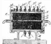
1. The combination with an induction coil having a suitable core, of a primary and secondary coil one over the other, both the primary and secondary coils being divided into separate sections, a casing for such coils, two removable end pieces connected with said casing, a telephone receiver opposed to each end of said core, said telephone receivers forming the end of the casing.
