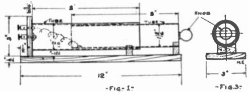
x 1/2 x 3 1/2 inches, and the other 3 x 3/8 x 2 1/2 inches. Secure two (2) 2/32 brass tubes, one being 8 x 2 inches and the other 8 x 15/16 inches. The 1/16 inch difference is allowed so that one tube can be inserted into the other. Fig. 2 will explain fully the method of fastening the larger tube to the board that
