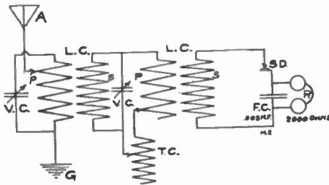
impossible to tune in the desired station. Having an extra loose coupler I connected them, as in diagram, and found that I could hear the messages louder as well as tune a great deal easier. Static also diminished a great deal. By putting a single slide tuner in, it made quicker tuning possible.
