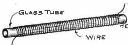
heated the tubing which would then bend very nice and evenly, as quite a long space was heated at the same time. I would recommend this method above all others I have tried. Use about No. 30 iron wire and wind closely and evenly. Connect to the lighting circuit in series with a water rheostat, as then you need not use so much wire, which will save time and trouble in winding it on.
