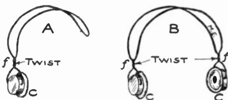
it to fit the head snugly, besides being very light and cheap. A double head-band may be made as at B. If made of nickel-plated brass, or phosphor-bronze wire, it will be found very neat as well as useful.
