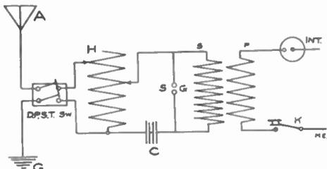
2.—Receiving set consists of one loose coupler, 2-slide on primary, one 2-slide tuner with 570 turns of 28 enameled wire on a core 12 1-2 inches long and 3 inches in di-
