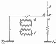
A system of wireless telegraph in which a closed oscillating circuit is used to accumulate energy which is emitted periodically by an antenna, the duration of the emission of the energy by the antenna being continued until the emission reaches the steady condition.
