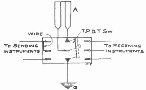
and connect the two aerial lead-in wires to two of the levers and the ground to the third. To one side connect the receiving instruments as in any other switch. On the other side run a wire (about No. 14 for average use) from one post to the other, which makes contact with the aerial, thus bridging across. Now connect as with a straight aerial switch.
