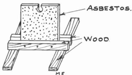
lumber nailed to some cross-pieces (Fig. 1.) with a small groove in the top to hold the wire will answer the purpose. A square of hard rubber or shellacked wood with the groove lined with asbestos is also good. About one inch below
