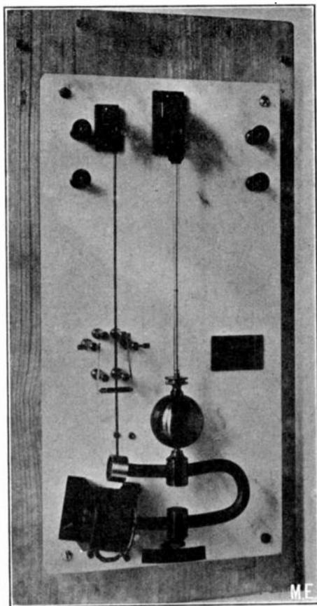
the clock is to work very accurately, and it always causes more or less disturbance, hence it is recognized that it would be much preferable to do away with the contact were this possible. M. Fery now succeeds in doing this in a very ingenious manner. The pendulum ball is suspended as usual from an upper point (see photo) and it carries below a U-shaped permanent magnet. A solenoid mounted on one side serves to attract the
