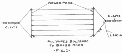
An easily insulated aerial (straight away) may be made by using a couple of brass rods for spreaders. The lead-in may be connected wherever it is handiest and the number of cleats must be governed by the tension you are handling.
