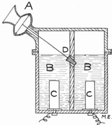
which allows the liquid to communicate. The current is passed in the two wires, and the resistance of the circuit depends upon the size of the hole D. A conical stopper is placed in the hole, and it is connected by a wire or rod to the diaphragm in such way that any movement of the diaphragm will give a corresponding movement of the stopper so as to change the size of the orifice. Speaking into the mouthpiece will thus cause variations of resistance due to this cause,
