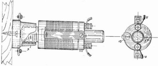
Near the end of part 2 a round hole is made with a groove running up to screw, part 7. A brass spring wire, about No. 22 B. & S. gauge is run in groove and the little coil is dropped in the hole—see illustration—so that it makes good sliding contact on the brass rod, part 4. The other end of wire is connected to screw part (7). A little wood plug is put over spring to keep it in place.
