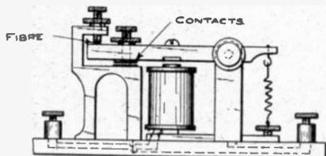
justment screw and the other on the anvil where this screw hits. This will probably be better understood by referring to sketch. The filed surfaces should come together perfectly flat. On the back click screw, glue a little piece of fibre. Then run wires to anvil and lever and key is complete.
