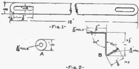
Get two pieces of 1/2-inch ribbon brass each 12 inches long, and slot them as in Fig. 1. To do this, first drill several 3/16-inch holes and finish with a file.
