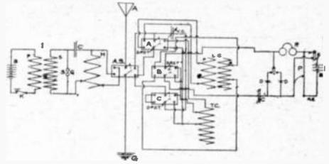
2.—My sending set consists of a 2-inch coil, key, helix made of 30 feet of No. 8 copper wire, wound one inch apart, leyden jar condenser, six Edison primary batteries, and same aerial, water pipe ground, and zinc spark gap. Are my instruments well proportioned?
