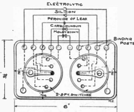
Having screwed them to the base, get 12 binding posts off of dead dry batteries, put 2 at the bottom with one on each side. These are to lead to the instruments. Then put the other 10 at the top. Starting in the middle, space them according to the number to be used. The dotted lines shown in the drawing show where the wires run under the base. The wires are led to the detectors as shown.
