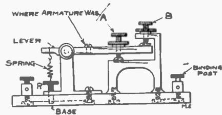
adjustment can be accomplished by the thumb screw and spring, R, and the other two points A and B. Of course only one detector should be used at a time.
