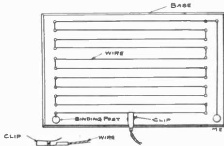
inches and tack on about 20 small nails about half way in. Now procure some German silver wire about the size of a thread and wind it on the nails, as per sketch, about 10 or 15 feet is sufficient, which can be purchased for 5 cents.
