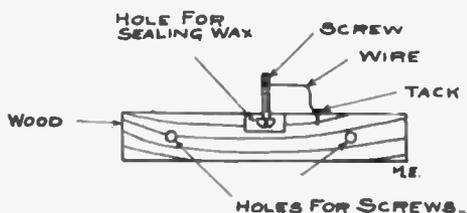
the wax is hard take out the screws, carefully pull the mould apart and trim the head with a knife and file.
