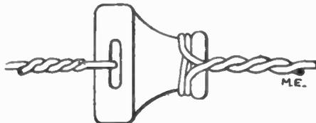
top, then put through the hole a piece of wire and fasten to your spreader where the rubber washer was formerly and your aerial wire after the manner shown which makes a very fine small insulator.
