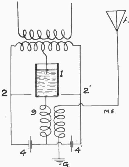
disturbances. The second figure shows a double valve connection. The cooled electrode (1) is connected at the middle point of the transformer secondary, with the other electrodes (2) (2<sup>1</sup>) in separate circuit with the condensers (4) (4<sup>1</sup>) and a common induction coil (9) so that first
