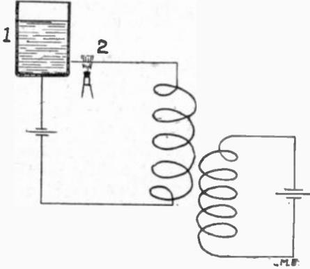
(2) is heated by the flame of a spirit lamp or by a small extra spark gap. When a strong supply current is used, a special means of heating is not needed. When using high tension direct current, we adjust the spark frequency and capacity so that a musical note is produced at the receiver, and this allows of receiving messages in spite of atmospheric
