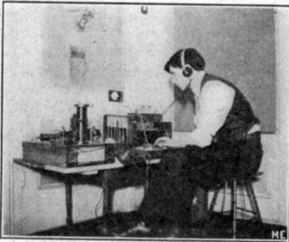
At the right is our sender. In the center of the table is an E. I. Co.'s sending helix, adjustable condenser, key, E. I. Co.'s one inch coil, spark gap, 18 dry cells and D. P. D. T. switch (not seen) in back of the helix to throw in the sending and receiving apparatus.
