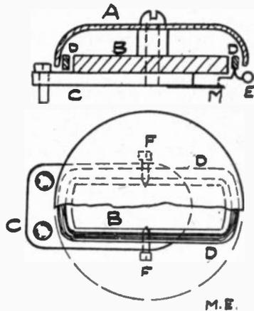
On the base plate, C, is mounted an iron piece, B, which serves as a core for the movable coil and the magnetic circuit is completed by the iron bell A. The coil, D, sur-
