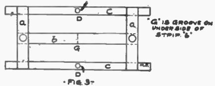
fasten them on the under side of the pieces a a, as shown in Fig. 3, and then solder a short piece of flexible cord to the center of each at D D, Fig. 3, which go to binding posts 1 and 2, Fig. 5, for the aerial and ground. This entire framework sets on the pivot B, Fig. 1. From a piece of No. 26 or No. 28 spring brass cut out four pieces like Fig. 4, and after making the holes, bend at right angles on the dotted lines. Two of these pieces
