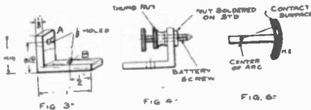
Sharpen the ends of 2 battery screws (see Fig. 4). These are for the key to move on.
