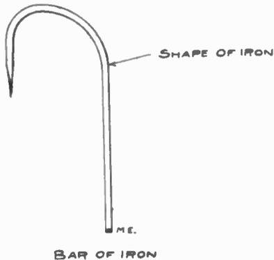
Heat the short pointed end to cherry heat and you can hold the long end in your hand and work all day without burning your hand. Now trace with this iron along the lines made by the file and the glass will break smoothly and evenly. A curious fact about this method of cutting glass is that you can press your finger on glass edges cut in this manner with no harmful result.
