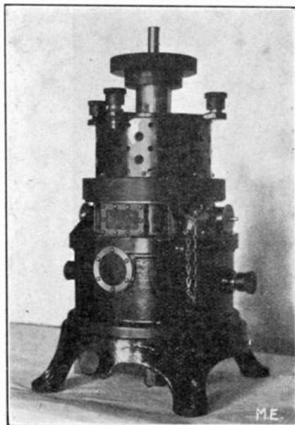
C and an inductance L in series (Fig. 1.) The operation is as follows: When the spark balls are put in contact a current is drawn from the supply and passes through the large inductance K. If the balls are separated, an electric arc is formed and the condenser becomes
