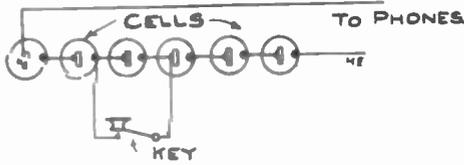
nect the cells in series; connect the complete terminals to a telephone receiver. From three or four of the cells connect the terminals to an ordinary key. The sound in the receivers is the same as in the wireless 'phones. The idea may be easily understood from the following diagram.
