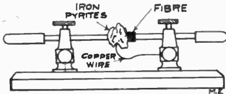
A piece of copper wire was put on binding post that held the latter rod. Other end of wire touched the mineral and detector was found to work as well as high priced detectors.
