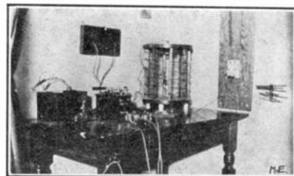
Transmitting, aerial 2 wires, 2 feet apart, 25 feet long, 40 feet high at one end, 30 feet high at the other. Sending helix, glass plate condenser, 1-inch spark coil, spark gap, and key. Receiving, single slide tuner, silicon detector, condenser, and 2 2,000-ohm phones on a headband. With this station I am able to receive 100 to 150 miles and transmit 3 to 6 miles.
