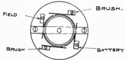
handle and the reverse switch is complete. Make connections as shown and you will have a reverse switch as good as any.
