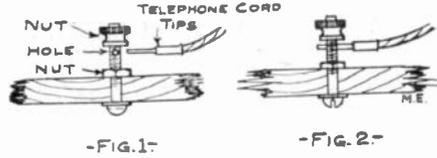
hand for my telephone cords I took a large brass screw and drilled a hole in it as in Figs. 1 and 2, after which I put on a nut to tighten it and found it to work all right.
