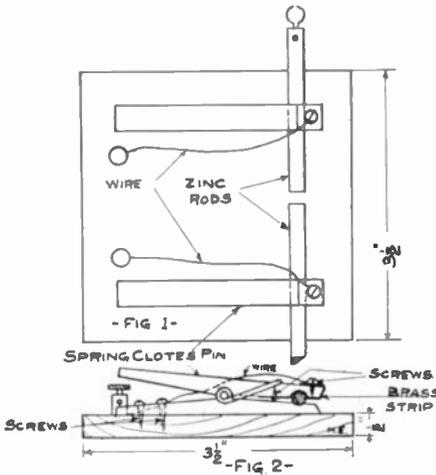
clothes-pins to posts in middle of base. Place zinc rods in the jaws and your spark gap is complete.
