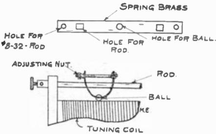
from old dry batteries, and an old ball-bearing of suitable size.
