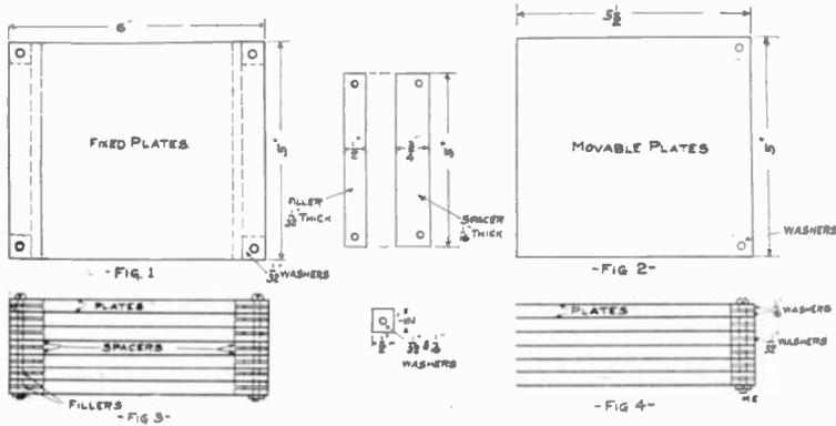
In the up-to-date receiving station a variable condenser is an absolute necessity. Of the various types, those employing sliding plates, with air as a dielectric, are preferred by many. The difficulty, however, of grooving a frame to receive the plates has deterred many amateurs from constructing a condenser of this type.
