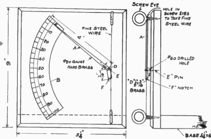
This ammeter, a description of which is given in the following, is the simplest that I have seen or read of, and is quite as efficient as a more complex instrument. The expanding and contracting of the fine wire acting directly on the pointer eliminates all springs and threads. The material required is:
