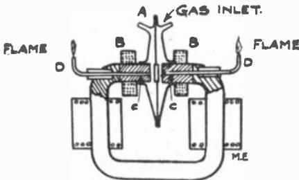
A very sensitive receiver which can be used either for wireless work or for ordinary telegraphy is here represented. The current coming in on the line gives fluctuations in a pair of small flames, corresponding to the signals, so that
