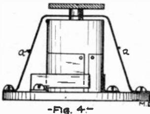
in the center of which a hole has been bored to insert the axle for the spool. Get a steel or brass strip and bend it as shown at a Fig. 4. Make a handle by
