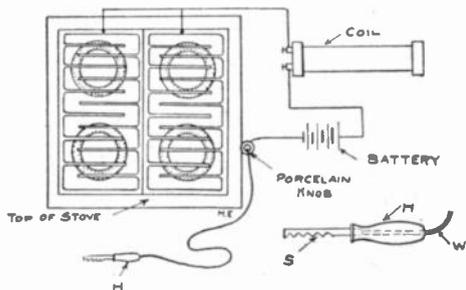
grate over the burner with the notched lighter will be sufficient to ignite the gas when turned on. Where electric gas lights are already used this may be worked from the same coil.
