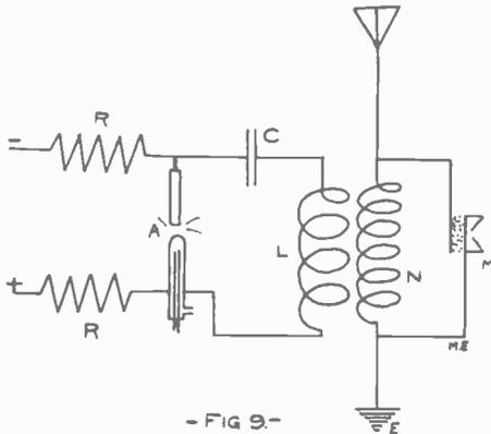
cuit slightly, and also affects the current in the sending aerial. Words spoken into the mouthpiece, therefore, produce an effect upon the amplitude of the emitted electric waves, and these are, so to speak, moulded into speech form, that is to say, made to vary as to the ordinates of a wave curve representing the change of air pressure taking place in the transmitter.
