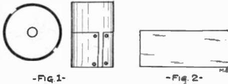
some thin copper, such as used for brushes on small motors. Cut pieces as shown and tack two pieces (No. 2) on the spool, as shown.
