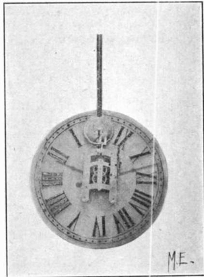
influence of the coil the armature is impelled against the pendulum, driving it forward, after which the circuit is broken, leaving the armature free to be returned to its original position under the momentum of the pendulum in its return swing. The swinging pendulum also operates the escapement lever by which the clock mechanism is advanced so no weights or springs are necessary.
