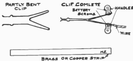
One like that shown in the sketch can be made of a strip of spring brass or copper bent into the shape shown in the drawing. Two battery screws are next
