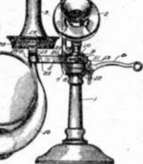
1. The combination with a stand, of a bracket rigidly secured thereto, an amplifier supported by said bracket, and means carried by said bracket to hold a telephone receiver in position to communicate with said amplifier.
