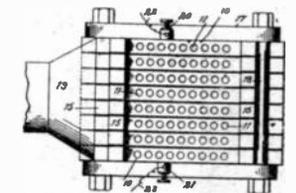
1. An apparatus comprising a plurality of electrodes and dielectrics spaced between them, said dielectrics being twice as thick as the width of the space between them and the electrodes.
