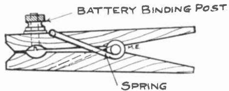
size as a battery binding-post, but with a flat head. This screw should be put through the hole with the flat head inside the jaw and a battery nut and binding post should be screwed on the other side of the jaw. Thus this will serve as a binding post and a contact at the same time. This clip being of wood should be shellacked or taped to prevent the operator being shocked.
