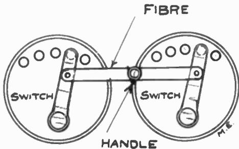
they both rest on the same point. Now unscrew the knobs on the handles and place a strip of fibre a half-inch wide across the handles, fastening it loosely with machine screws where the knobs were.
