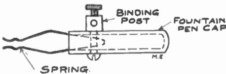
binding post screw to pass through. The rubber handle is a fine insulator so there is no danger of a shock.
