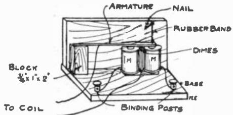
the binding posts. Then connect the wires from your key to the dimes and use your key to work this instrument. It works well on three dry batteries.
