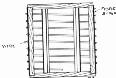
tween the open and closed circuits if less than four are used. The wire used should be no smaller than No. 12. The following table may be used in the construction of helices of various capacities:
