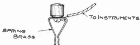
a 3/16 inch hole in the center and then bend into the shape shown. Just back of the place where it is to grip the helix wire a drop of solder may be placed to stiffen the spring. Now insert a short 8/32 machine screw through the hole to hold an electrose knob to serve as binding post and insulating handle.
