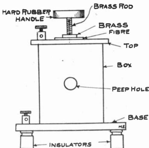
a 3/16 inch hole in the center of the fibre and screw the brass to the fibre, the fibre to one end and that in turn to the cover of the box.
