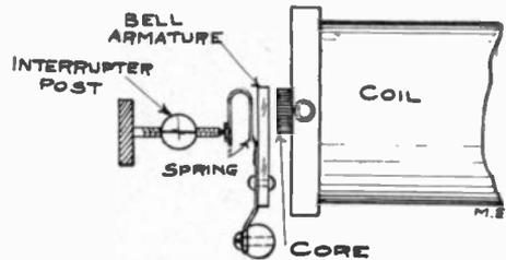
by merely bending the copper contact, which bears the platinum, around to come in contact with the thumb screw bearing the other contact, as per drawing.
