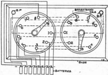
For testing storage batteries, connect a voltmeter or ammeter with the two binding posts. This saves a lot of bother of going around to find the condition of each battery by testing, or it may be used as a control.
