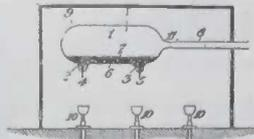
1. In an apparatus for exhausting a hermetically sealed chamber through the action of vaporization and expulsion of a volatilizable liquid, auxiliary expelling means said means consisting of an additional more easily volatilizable liquid introduced in the chamber prior to exhaustion.
