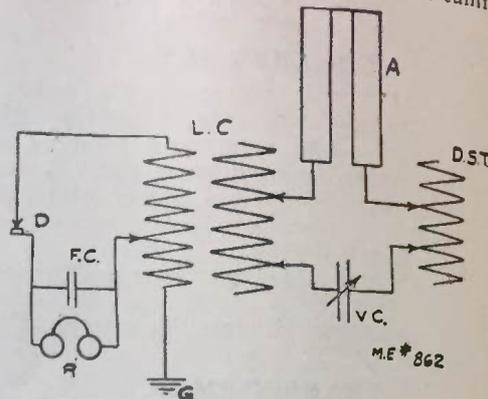
coil, double-slide receiving transformer, rotary plate variable condenser, Murdock improved silicon detector, fixed condenser and phones with a joint resistance of 4000-ohms, aerial composed of four No. 14 aluminum wires 60 feet high and 60 feet long, ground on water pipe and chicken netting in moist ground?
