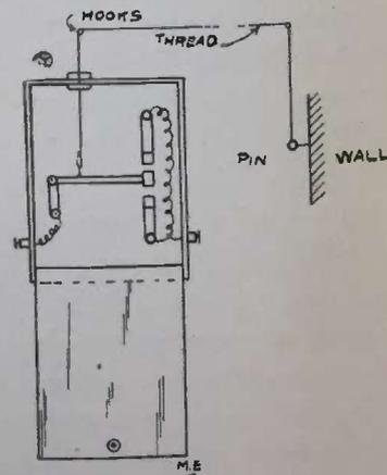
is stretched at the desired place in the room by running it over a pair of ordinary insulating hooks. It then runs into the box containing the alarm device. This consists of an arm which is pivoted at one end and is held in place in the middle position by the stretched
