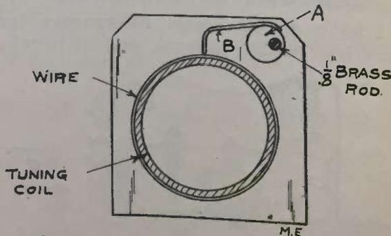
together with the weight of B, is heavy enough to make good contact with the wire.
