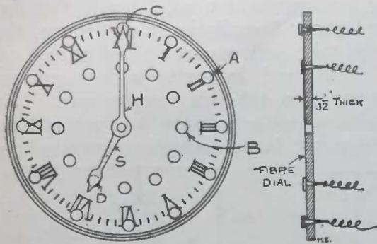
numerals are driven 12 more tacks as shown at B. These tacks are driven as close as possible to the surface of the fibre, and not separated therefrom by washers.
