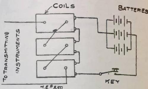
also suggest using about 20 dry cells in series multiple to work the coils. This would in all probability transmit the required distance with the large aerial you have.
