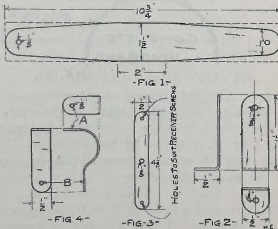
this bend should be regulated after the headband is finished so as to make the phones fit properly. The remaining piece is cut lengthwise into two pieces, each 1/2" by 4 1/8". These strips are rounded on the ends, and each has holes in the ends to fit the screws in the sides of the receivers, and a 1/8" hole in the center.
