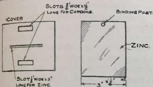
inch from the bottom of the crock. Now take the cover and cut three (3) holes in the top as per sketch, insert the carbons with the binding posts on. Next put the zinc in with a binding post on, which will also serve as a
