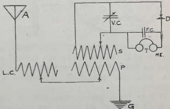
waves properly, was because better selectivity could be secured by having a small primary, and then using a loading coil for taking in long waves.
