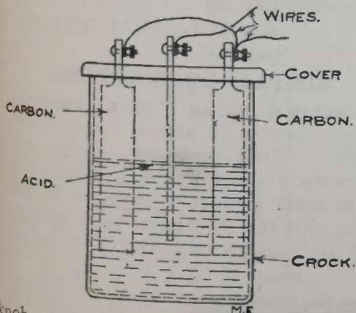
knob as well as a connection. Now make a solution of Potassium Bichromate 8 oz; Sulphuric Acid 17 oz. and Water 56 oz. Connect the carbons together and bring one wire out for connections from both carbons and one from the zinc. When the battery is not in use take out the zinc as the acid eats it very rapidly. This battery will give two volts if properly constructed. If four cells are used will run a one inch coil.
