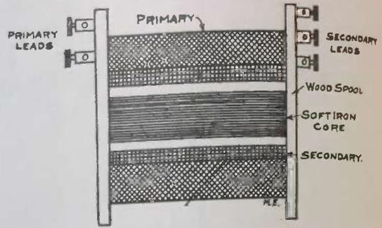
Over the secondary a few layers of paper are wound to serve as insulation tube.
