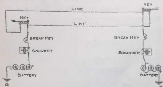
actly as shown; that is, each line wire is to be connected to different posts on opposite ends, and the sounder wire is to be connected to the back contact of key at each end. The break key should be similar to the "Electro" double-circuit "Cinch" key, using the upper contact. Diagram shows battery at each end, although it may be placed at one end if desired. A good ground is absolutely necessary to get good results.
