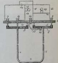
1. A temperature alarm apparatus comprising a pipe in loop form having open ends, diaphragms respectively disposed in front of said ends, terminals in proximity to said diaphragms, and means for electrically indicating a change in the contact relation between each of said diaphragms and its associated terminal.
