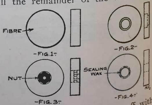
with sealing wax and polish off with a piece of emery cloth. You then have a handsome and serviceable thumb-screw.
