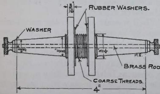
taper the part 1 1/2 inches from the edge of the raised part in the middle to the end, making the end 3/8 inch in diameter. On the raised part cut some rather coarse threads. Now take the hard rubber ends from a large magnet. These ends should be 2 inches in diameter, 3-16 inch thick, and have a hole 5/8 inch in diameter. If the experimenter has no such magnet he can turn them from a piece of hard rubber sheet. In the holes cut threads to cor-
