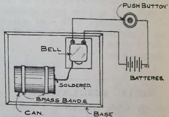
base should be made to suit the size of the can and bell, also the block. Connect as in diagram, using three or four cells of dry battery.
