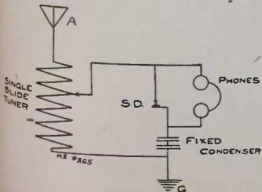
A. 1.—Single-Slide Tuning is never as efficient as a double-slide one, especially when connected as per your diagram, as ground cannot be varied.
