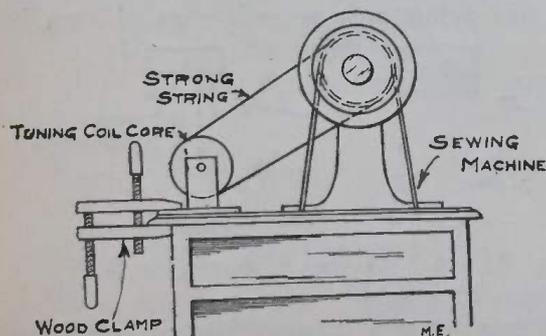
make a frame by taking a piece of board about 2 in. longer than the core, and nail two pieces upright on each
