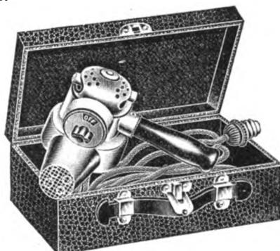
The hair dryer consists of a small motor driving a blower. In the large tube leading from the blower, a heating unit made of many turns of resistance wire is placed, with a rheostat in the circuit for regulating the temperature. The motor is of the very best construction, with the best of materials used, insuring perfect satisfaction under the worst treatment. One of the illustrations shows the apparatus placed in its carrying case, while the other
