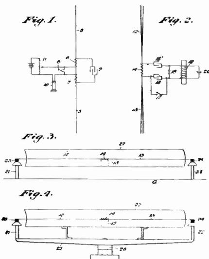
It will be seen that in the apparatus shown the magnetic or horizontal component of the electro-magnetic waves is utilized instead of the vertical or electro-static component.
