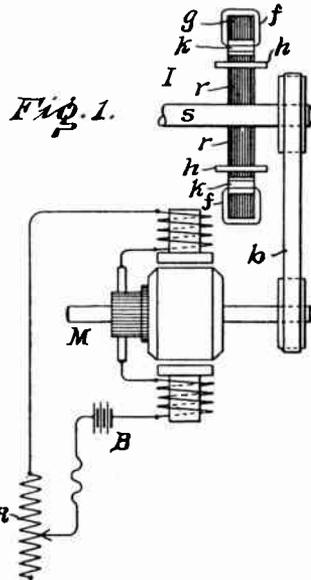
ternating current whose frequency is that of the current passed through the field or primary winding. The induction generator is not self exciting and therefore the alternating current must be produced or furnished by some other means which may be known as a "frequency setter."
