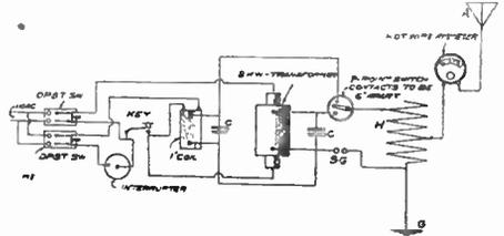
in diagram you can operate either transformer or coil without discharging both at the same time.
