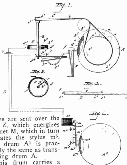
pulses are sent over the line Z, which energizes magnet M, which in turn operates the stylus m<sup>5</sup>. The drum A<sup>1</sup> is practically the same as transmitting drum A.
