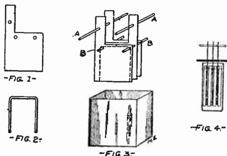
While it is true that some storage battery plates have lugs by which they are supported on the edges of the jar, it adds an inactive weight to the battery and does not provide for the support of proper separators for the plates.
