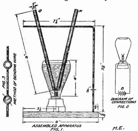
seal each piece at one end. Fill the lamp with water to which has been added a small quantity of salt, or, better, sulphuric acid if it is to be had. Now put the tubes in place one over each platinum wire after filling both of them with water.
