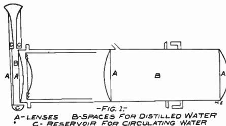
The lamp which concentrates rays into the telescope requires a direct current of 20 amperes at 55 volts. It can revolve around a vertical axis on which it is fastened with a screw. A rheostat is
