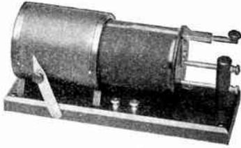
The neatest and most compact tuner on the market. Primary is wound with bare wire, secondary with green silk covered wire. Has all the merits of ALL the \$15.00 tuners. Tubes are hard rubber composition so wire cannot loosen. Notice unique slider construction.
