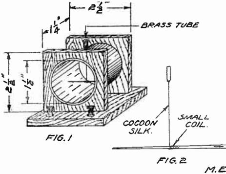
tube at the top. Wind about one-fourth pound of No. 30 D.C.C. wire on the reel. Be sure that the same amount of wire is wound on either side of tube.
