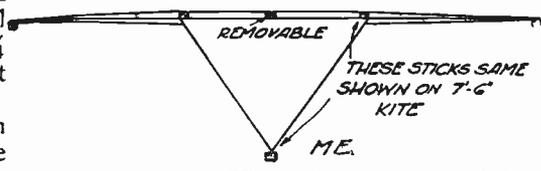
THE BRIDLE OF 6 FT KITE IS 10' LONG AND IS ATTACHED  $8\frac{1}{2}$ " FROM THE TOP OF STICK AND 21" FROM BOTTOM. THE STRING IS ATTACHED ABOUT 4" FROM TOP AND 5" FROM BOTTOM OF THE BRIDLE
