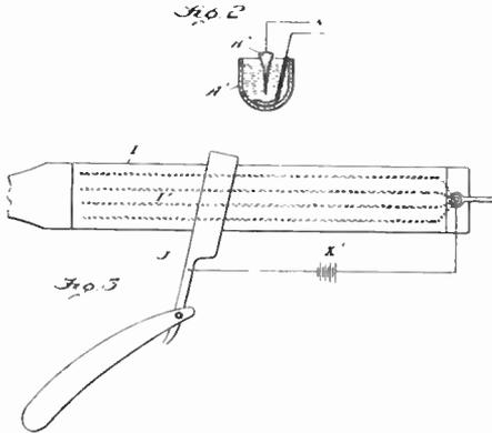
attack steel much more actively than if the current were not employed. The inventor has found that to secure this rapid electrolytic action it is not necessary to immerse the metal in a liquid bath, but that wherever the acidulated liquid is present and completes the circuit through the steel body there is, by reason of the current, more or less increase of effect upon the steel.
