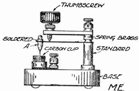
ment for holding the delicate Wollaston wire. Amateurs become disgusted with fingering minute screws and discard a most excellent detector for a more convenient, if not so efficient, type.
