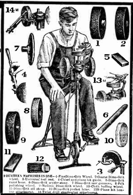
FOURTEEN MACHINES IN ONE—1-Fine Dimo-Grit Wheel. 2-Coarse Dimo-Grit wheel. 3-Universal tool rest. 4-Chisel and plane bit saw guide. 5-Dimo-Grit razor hone. 6-Dimo-Grit scythe stone. 7-Dimo-Grit saw gummer. 8-Felt polishing wheel. 9-Medium Dimo-Grit wheel. 10-Cloth buffing wheel. 11-Dimo-Grit oil stone. 12-Dimo-Grit pocket hone. 13-Plane bit honing attachment. 14-Twist drill sharpening attachment.
