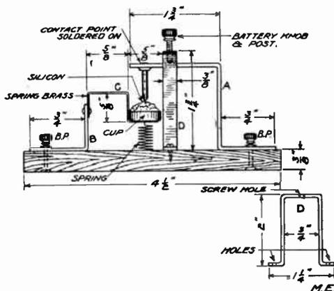
sions and shows how the detector is assembled.
