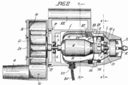
chamber, 16, and the air is thus forced out from the funnel like arrangement, 19. A handle, 22, is provided, to carry the motor; and the motor may be switched on and off by means of switch, 12. An ordinary plug and cord, 23 and 24, are used to make connection.
