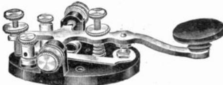
The best low priced wireless key made. Base is polished black composition. Lever is connected to binding post by a phosphor bronze strip. Silver contact points 5/32 in. diameter in removable holders to facilitate renewal. Can be used on sets up to 1/2 K. W.
