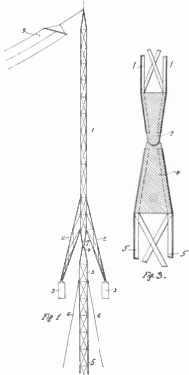
mous, in order to put even a small strain upon the aerial, 9. The inventor also states that four counterweights, instead of two, could be used.
