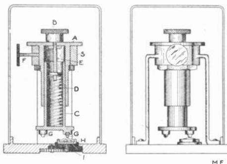
the spring, and so varies the pressure of the points, G, on the crystal.
