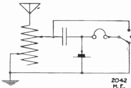
Q. 2.—How far would the above set receive with an aerial about 40 feet high at one end, 25 feet at the other, and 60 feet long?
