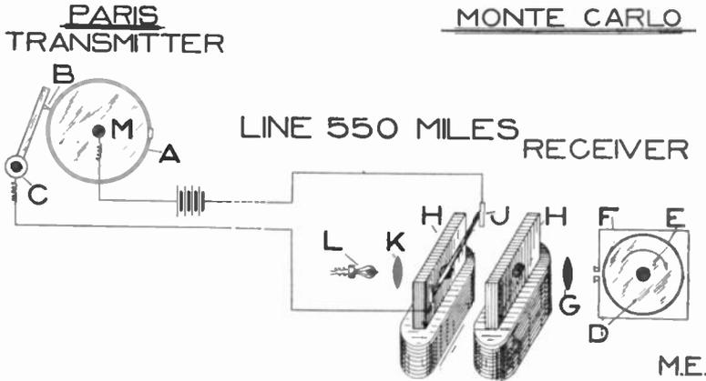
the transmitted picture. The recording is done entirely by the photographic method, utilizing the action of a small beam of light which passes
