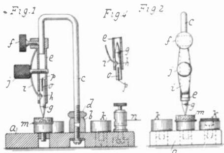
used for an electrolytic detector, and the Wollaston wire, p, is clamped by the spring, o, also a novel arrangement.
