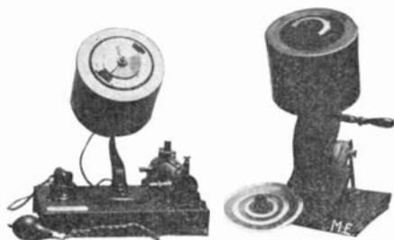
discs are adjustable so that any amount of the three primary colors may be combined to match any given color. A graduated circle shows the exact amount of each color used. An apparatus of this sort is very useful in matching or analyzing colors. The motor operates on the lighting current with a resistance in series. At the right is also shown a hand operated machine.
