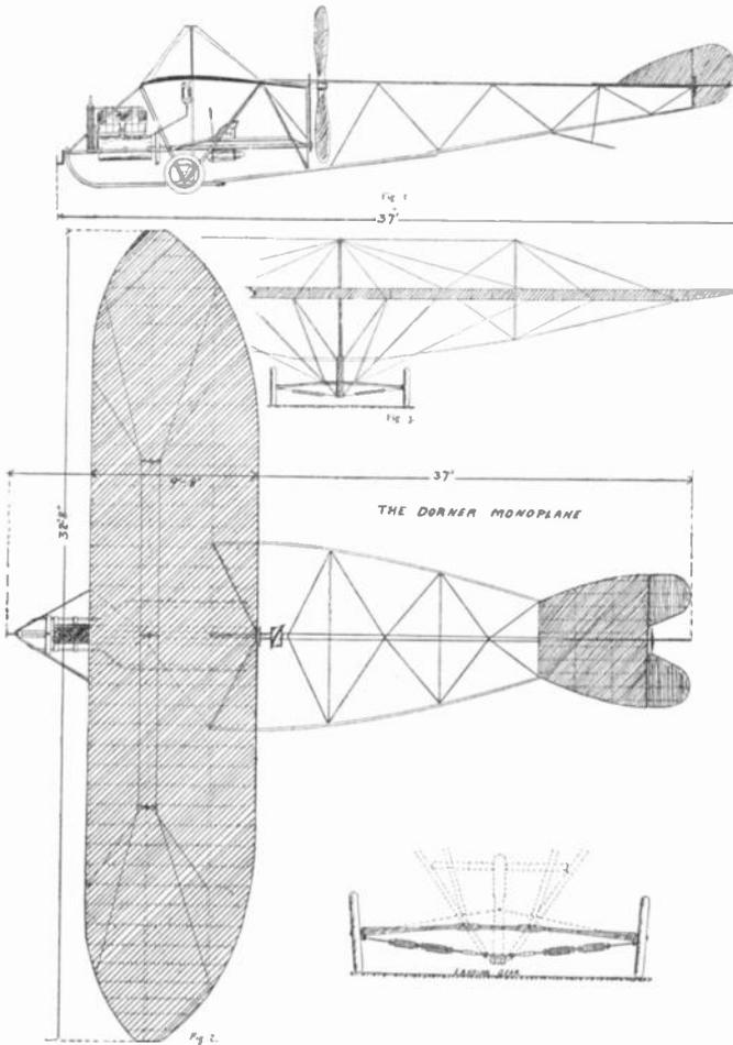
the open triangular type tapering front and rear with the single main spar running along the bottom and acting as a skid. The two upper spars are spread out in the vicinity of the propeller to
