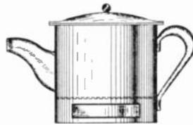
incandescent units having the heating wire sealed into exhausted tubes. This arrangement allows the heat to be freely radiated, with little absorption, and, at the same time protects the wire against oxidation. The heater is adapted to slide into a recess in the bottom of the double bottomed kettle, like a drawer in a cabinet, and is provided with a heat regulating switch.
