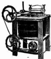
Not a hand power machine with motor attached. Built for electric motor or gasoline engine from the ground up.
