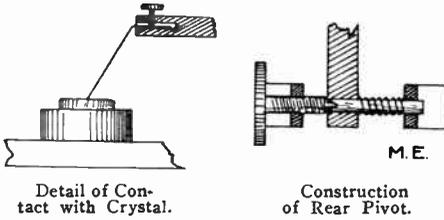
any point on the surface of the crystal to be reached. The cup is fixed in position, but may be revolved.
