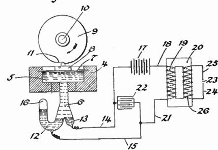
breaker in which effective means are utilized for overcoming the tendency of the contact points to oxidize. This and other objects we attain in an apparatus described and illustrated in the accompanying drawings, throughout the several views of which
