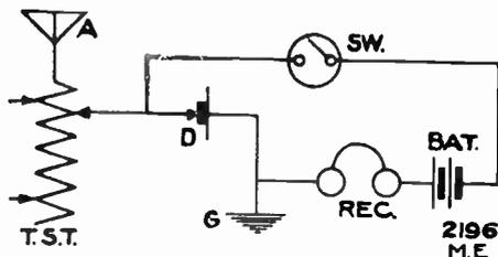
A.—If you are using a silicon detector, cut out the batteries and the switch and hook up the apparatus as per the diagram in answer to No. 2139 in the September issue of *Modern Electrics*, leaving out the variable condenser and putting a small fixed condenser in the position shown in the diagram.
