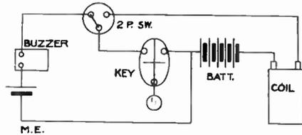
switch is for changing from the buzzer to the spark coil. This connection will permit the use of the key, which will be found to work much easier than a push button.
