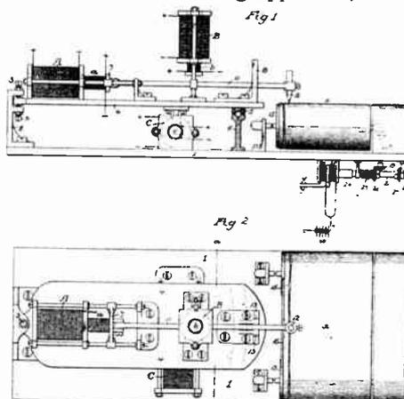
is obvious that any movement of the stylus, 12, will be reproduced on the receiving instrument in the same manner as the stylus, 12, moves in the transmitting apparatus.
