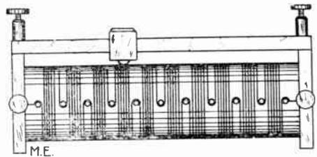
Enclosed you will find a sketch of a non-inductive potentiometer, which I constructed and use.
