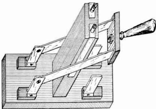
This switch has been in use in my station now for over a year and has proved satisfactory in every respect. It is so simple that any amateur can make one. As will be seen only a throw of 30° is required to change
