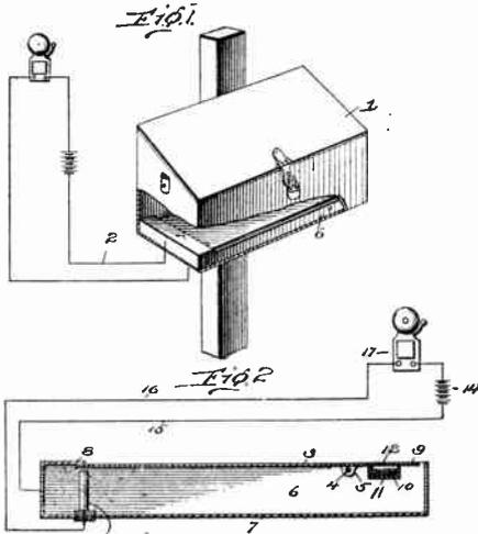
fore curve more or less in cold or hot weather, thereby closing the contact.
