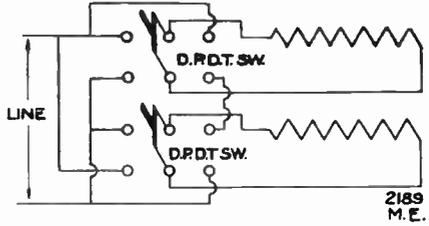
When both switches are to the left the two sections are in multiple. When both are to the right they are in series. With either of the switches to the right and the other to the left, one section is connected in and the other is not.
