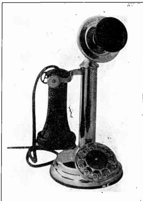
FIG. 1.—THE SUBSCRIBER'S INSTRUMENT
