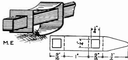
struction that I send it to you. It should be made of fairly substantial spring sheet brass.
