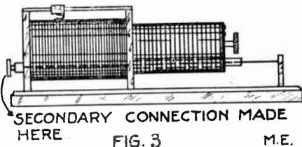
$3\frac{3}{4}$  inches in diameter to allow the primary to set into it. The other end piece must have a circular groove of the same diameter, into
