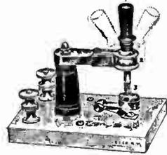
New Commercial Detector Stand. The latest addition to our commercial instruments. Highest grade detector on the market. Has ball joint (2) and tension adjustment (3). Handle (1) can be pulled up vertically, making it the most sensitive detector on the market. **¾" Italian marble base. Nickel finish throughout. Weight 1 lb. Size 4½ x 3 x 5". Price.... \$3.75**
