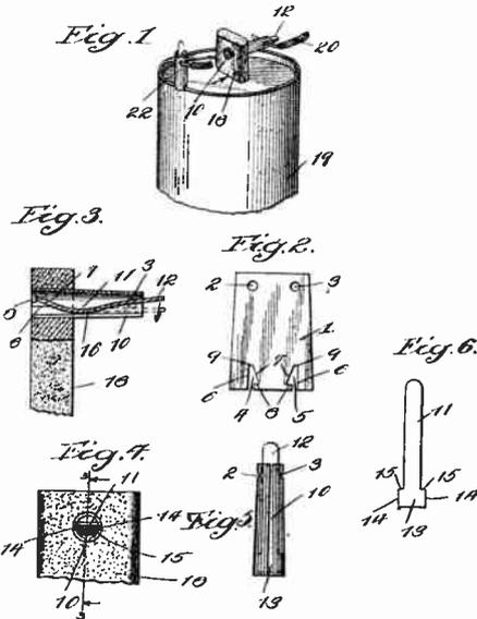
perhaps more. The working of this binding post is identically the same, the spring, 12, being depressed in order to uncover the hole, 3, Fig. 3, which breaks the connecting wire, 20, Fig. 1.
