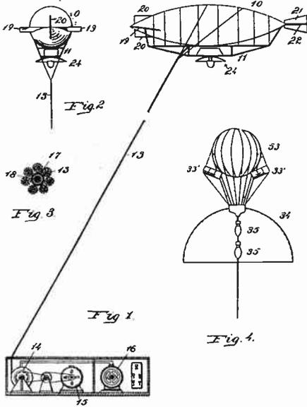
In the accompanying drawing, Fig. 1, is a view of a dirigible type of balloon, moored to suitable mechanism, and carrying a light and reflecting apparatus. Fig. 2 is an end view of the balloon. Fig. 3 is a section of the cable employed. Fig. 4 is a view of a spherical type of balloon, with a modified type of lighting and reflecting apparatus.
