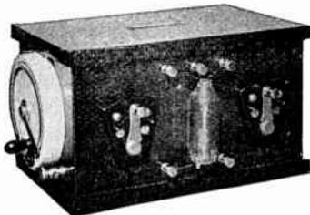
Consists of valve bulb, high and low (storage) voltage battery and necessary appurtenances mounted in a mahogany cabinet. Combines all the advantages of the Audion and Fleming Valve with an absence of their failings. The following are extracts from the logs of two of the ships equipped with our valve detectors:
