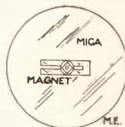
DETAILS OF MAGNET & BOLT
