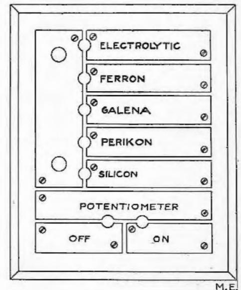
The pieces are now mounted on the base with a space of 1/16 inch between the adjacent parts, connections being made through small holes beneath each plate, the wire being soldered securely before fastening them down.
