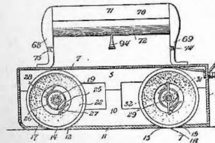
the interior of the casing, 2. 94 is a finger contact lever for reversing the motion in the propelling roll, 15, said lever being shown here in its normal, neutral position, in which both the motor and the heating elements are cut out of circuit. The roll, 14, is hollow in construction and is provided with a cylindrical shaft, 19, whose extremities are journaled in suitable bearings carried by the side walls, 10, respectively, of the lower section of the frame. Suitable
