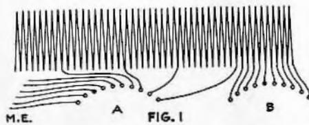
mercial coils of this type. The secondary taps are taken every 20 turns and soldered to the points of a switch on the end of the coil. The diameter of the secondary is three and one-quarter inches.
