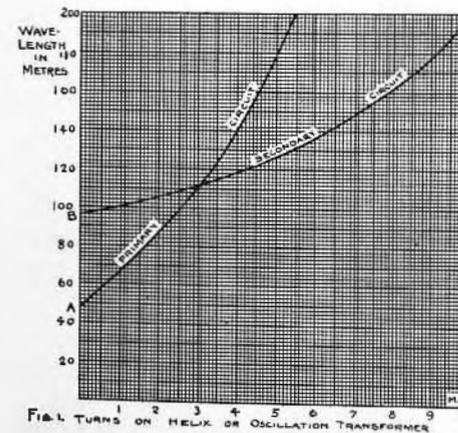
1, must be had, and along the last horizontal line numbers are put corresponding to the turns on the helix or oscillation transformer. In this instance it is assumed that the total number of turns
