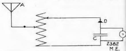
tiometer, which is unnecessary when using galena detector.
