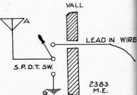
nection running to the ground from this switch should be as straight as possible, with no sharp turns or abrupt bends. A diagram is appended here-
