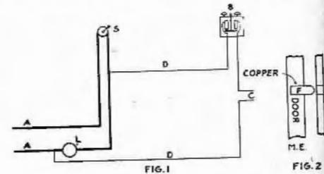
is represented by light lines in the diagram. AA are service lines and S is a snap switch at the head of stairs leading to the cellar. L is a light or many lights. C is the contact made at the door, which is shown in detail in Fig. 2. One wire is connected at F and the other at G. B is an ordinary telephone magneto bell, either of 600 or 1,000 ohms, mounted on a block of wood.
