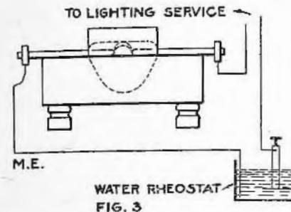
to be slipped through them to form the electrodes. The carbons may be secured from supply houses, or from arc lamps after they have become too short for further use.
