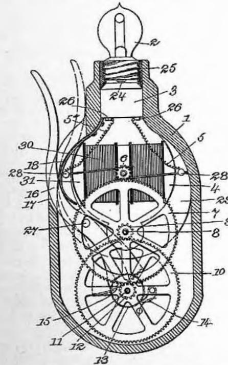
leasing the pressure spring 18 forces the lever back. Each inward movement of the outer projecting end of the lever spins the armature of generator 4, through action of the pawl and ratchet
