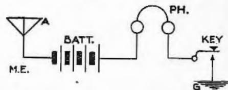
With this arrangement I have detected leakage in my aerial.
