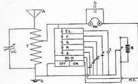
“Electrolytic.” This connects that detector in circuit. Now to connect the potentiometer, place the second plug between the plates “potentiometer” and “on.” When not in use the plugs may be kept in the holes in the blank plate, provided for that purpose.
