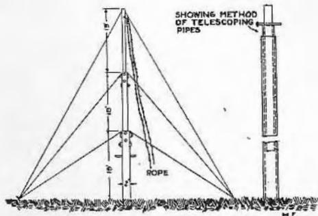
section easily. The third section can be made as long as desired and is small enough so as to slip into the second joint easily. The novel part of the mast is the method by which the sections are fastened at the joints. Two holes are bored at each end of the pipes, one foot apart, and two more bored at right angles to them, as shown in sketch. A step made of strap iron is fastened on the first joint to aid in erecting it.
