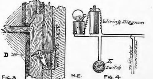
the window frame, close to the window sash. The arrow, D, points to a small L shaped screw hook screwed into the window sash. Notice the hook is hold-
