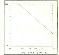
Fig. 4. This is the log-log plot of resistance-versus-force for the Interlink FSR.
