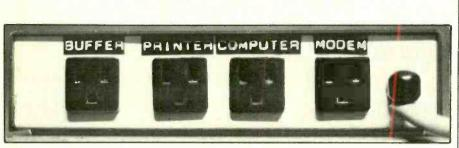
Photo shows details of controller's rear panel. Ac power cord enters through and ac receptacles mount on panel. So, too, does a circuit breaker.
