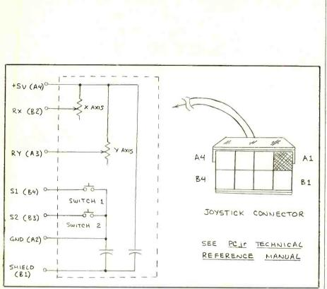
Fig. 9. PCjr joystick circuitry and connector plug schematic diagrams.
