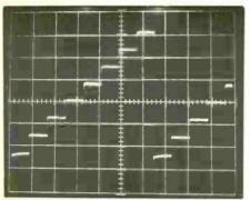
Fig. 1. Multiplexer generated a reasonably linear staircase waveform.
