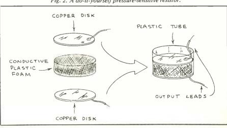
Fig. 2. A do-it-yourself pressure-sensitive resistor.
