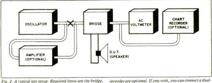
Fig. 2. A typical test setup. Required items are the bridge, oscillator and ac voltmeter. The amplifier and chart
