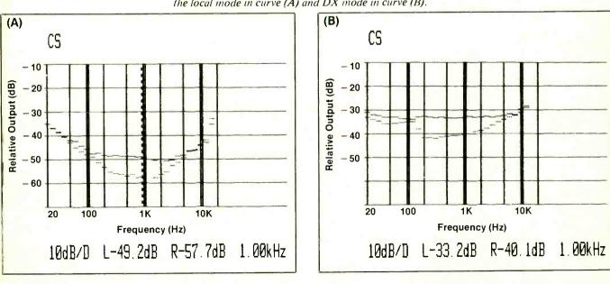
Fig. 1. Separation characteristics for the Model R-9's stereo FM tuner section shown in the local mode in curve (A) and DX mode in curve (B).
