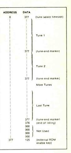
Fig. 2. EPROM allocation map per memory page, data column in octal.
