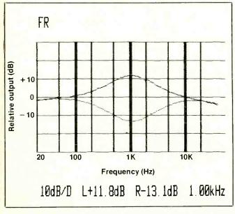
Fig. 4. Curves show range of receiver's midrange tone control.
