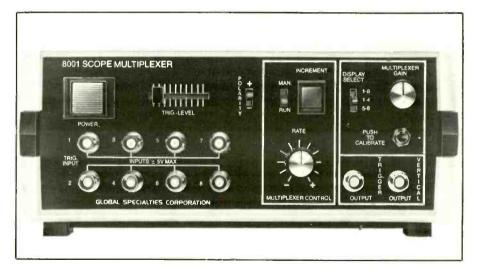
be set up to display a single waveform or, with the flip of a switch, four or eight waveforms simultaneously. Furthermore, an incrementing circuit whose function is activated with the touch of a switch lets you step through all input channels individually for examination of a single waveform at a time.
