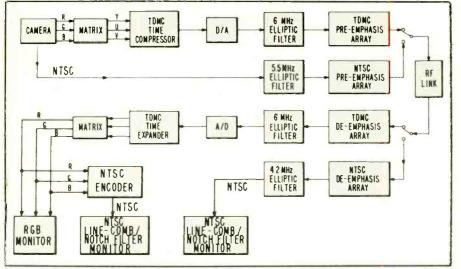
Fig. 1. Block diagram compares B-NTSC system readied by RCA (upper portion) with Britain's B-MAC system (lower portion) currently in operation.
