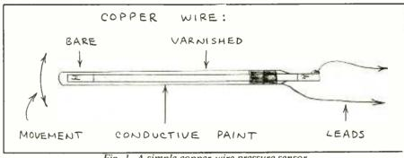
Fig. 1. A simple copper-wire pressure sensor.
