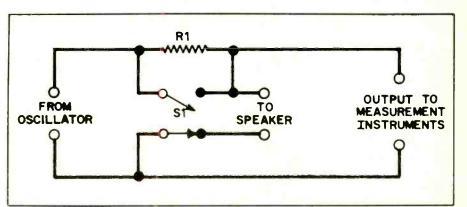
Fig. 1. This is the schematic diagram of the impedance bridge. This two-component circuit must be used with at least an oscillator and an ac voltmeter.
