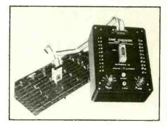
and display IC errors under actual operating conditions. A front-panel zero-insertion-loss socket is used to plug in a known "good" reference IC. The Model TTL-1 Chip Checker tests virtually all 14-, 16-, 18- and 20-pin DIP TTL ICs, including lowpower Schottky TTL. Though some specialized ICs and those devices that depend on external resistors or capacitors, such as the 74121 monostable, cannot be tested, tri-state, bidirectional and open-collector devices can in most cases be checked.
