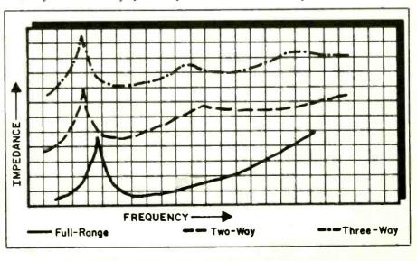
Fig. 3. Shown here are impedance-versus-frequency plots for typical full-range, two-way and three-way speaker systems. Note resonance peaks on each curve.
