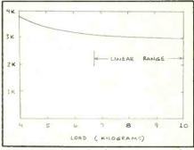
Fig. 5. High-load-value resistance plot for the FSR example in Fig. 4.
