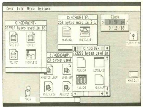
Digital Research's Graphics Environment Manager (GEM) software turns the screen on IBM PCs and compatibles into a near clone on Apple's Macintosh.
