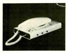
ing circuit that detects voice and data carrier and automatically passes the signal to the computer or telephone. A built-in 2" speaker lets you monitor the call, while a built-in clock/calendar feature lets you keep track of call length on your computer's video monitor screen.
