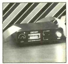
Cincinnati Microwave's popular Escort, which uses surface mounted device (SMD) construction.
