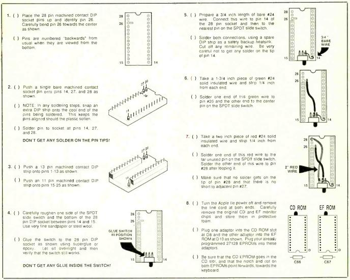
Fig. 1. How to install a dual monitor adapter in the Apple IIe computer. You need two adapters for the modification.
