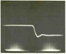
Fig. 2. Trace rise and fall times of 18 ns produce a 20-MHz bandwidth.
