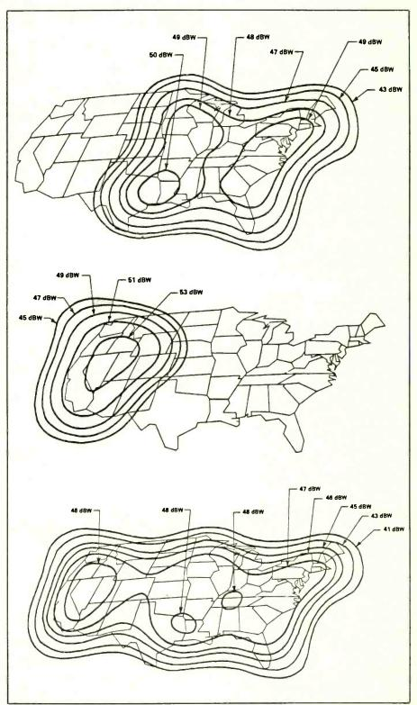
Fig. 2. This series of diagrams illustrates reception "footprints" possible with the new RCA Ku-band K Series satellites. Top diagram shows eastern U.S. coverage, center diagram western U.S. coverage and bottom diagram CONUS coverage. All are with K-2 in orbit at a nominal 77° west longitude assignment.
