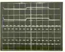
Fig. 4. A 16:1 frequency difference still locks all waveforms in sync.
