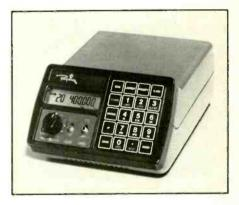
The multifunction lighted LCD display shows channel numbers during scanning, channel and frequency when a call is received, loss of power, delay function status, channel lockout and search mode selection. \$699.95.
