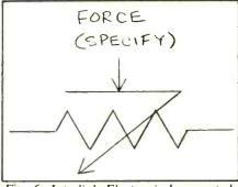
Fig. 6. Interlink Electronics' suggested schematic symbol for the FSR.
