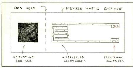
Fig. 3. Details of the Interlink pressure sensitive resistor.
