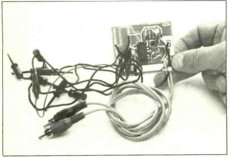
Interconnects from the small commercially available video adapter board connect to the CoCo via wires terminated in mini-clips. The two cables terminated in phono plugs are the new video and sound outputs.
