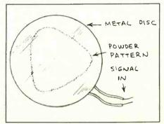
Fig. 2. Nodal pattern of an oscillating piezoelectric buzzer element.
