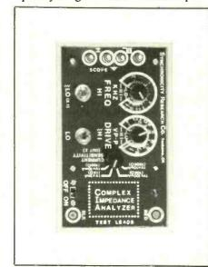
sible for the CIA to perform accurate inductance and capacitance measurements from less than 2 mH to beyond 200 H and from less than 100 pF to beyond 20  $\mu$ F. The impedance of complex networks and transducers can also be measured. The CIA is battery powered for convenient field-service use, but it can also be used on a testbench.
