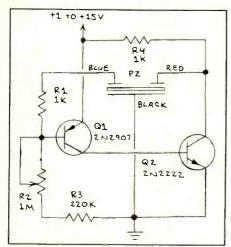
Fig. 9. Adjustable-frequency piezoelectric buzzer element driver.
