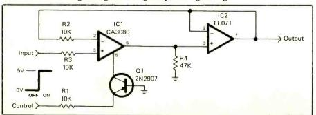
its input when triggered and continues to "hold" that level until another command is issued. When the control line goes high, the ICI OTA acts as a closed switch and charges CI until the input and output voltages are equal. With the line low, the "switch" opens so that the voltage is stored in C1. To prevent leakage currents from introducing errors, use a low input bias operational amplifier like the CA3140 or LM351 for IC2 and polyester or polystyrene capacitor for C1.
