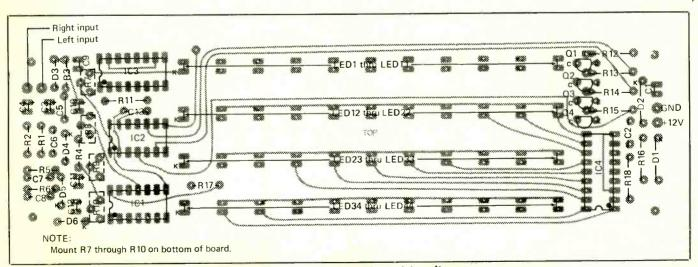
Fig. 4. Placement/orientation wiring diagram.
