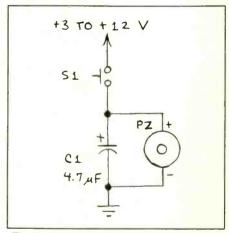
Fig. 5. Achieving a bell-like sound from a piezoelectric buzzer.
