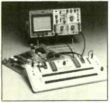
Connected to any dual-trace X-Y oscilloscope, Scopemate 2 tests for shorts opens, diode action and leakage by applying up to 14 volts rms at 300 mA to compare unpowered devices. It displays both good and bad signatures of the component being tested. Results are displayed as a graphic waveform, rather than in a numeric format that requires interpretation. Major differences in component signatures indicate a malfunction in the device being tested.
