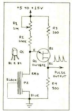
Fig. 10. Unijunction transistor piezoelectric buzzer element driver.
