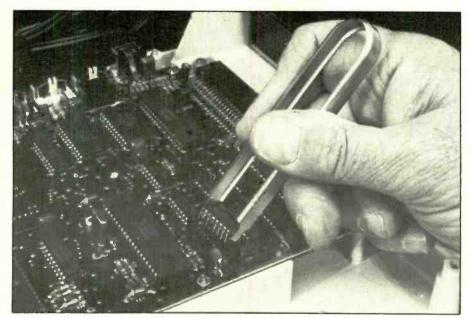
Use an extracting tool to remove the 16K RAM chips.
