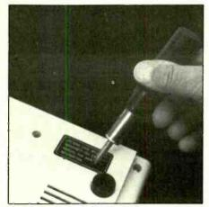
One of six screws that must be loosened to open the cabinet is hidden under the label that warns against opening the case. To get at it, push the tip of a Phillips screwdriver through the label.
