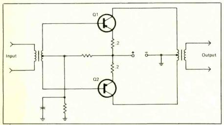
Fig. 6. A typical push-pull amplifier stage with transformer input and output.
