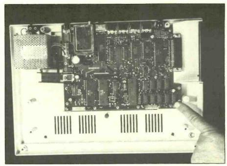
Eight socketed memory ICs are in the lower-right of the motherboard. Remove the factory-installed 16K chips and replace them with 64K chips.
