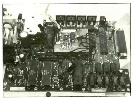
The video adapter mounts on top of an IC with double-sided tape (supplied with kit). Installing the adapter with holes to the right lets you tuck most of excess wire lengths under the board's front edge.
