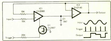
Fig. 5. A typical OTA sample/hold circuit.
