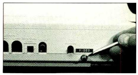
Instead of bringing the video cable through the cabinet, you can install a phono jack on the CoCo's cabinet to the right of the power switch and connect the cable to this. If you are using the audio option, do the same for its cable. Label jack(s) for easy identification.
