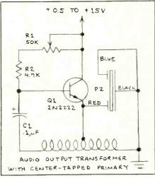
Fig. 8. Hartley oscillator piezoelectric buzzer element driver.
