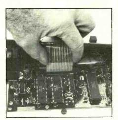
Do not grip the keyboard's ribbon cable as shown to unplug it from the motherboard; it might be damaged. Instead, grip it on both sides between thumb and forefinger and lift straight out.
