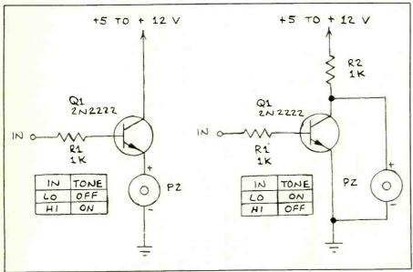
Fig. 6. Piezoelectric buzzer logic interfaces.
