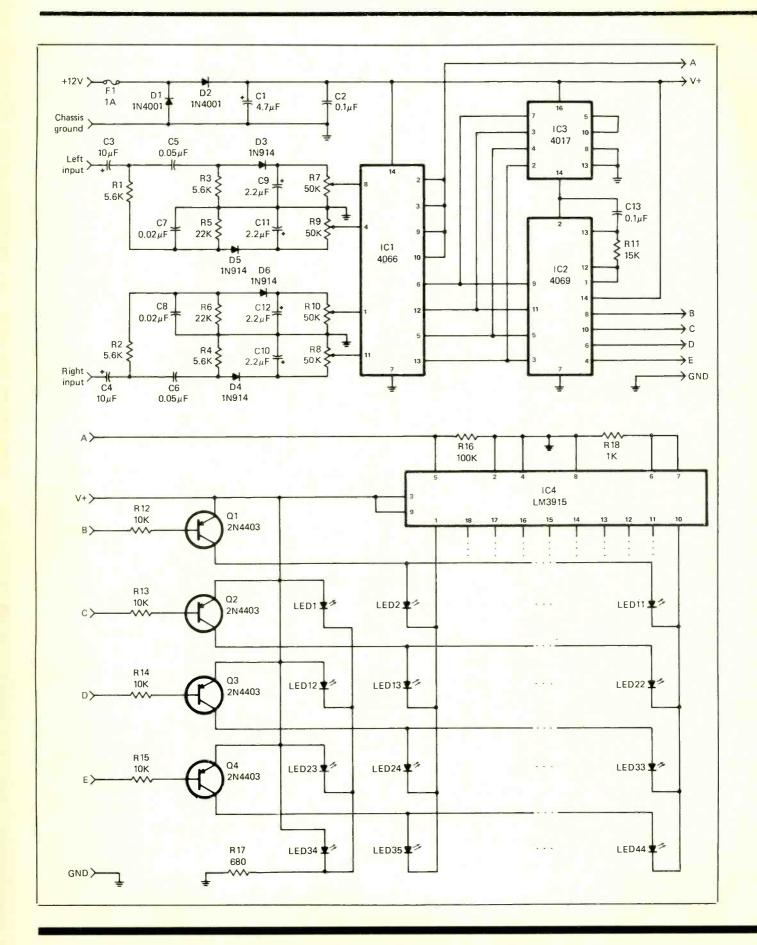
Fig. 2. Separate high- and low-frequency "bar" displays consist of 10 LEDs in each channel bar, plus one LED in each bar that comes on when dc power is applied. Only four LEDs are shown for each channel.
