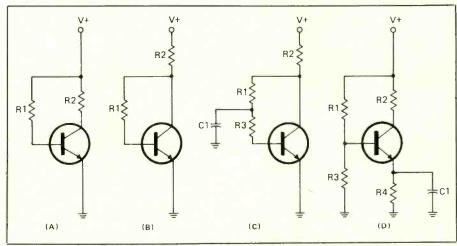
Fig. 1. Several of the most common methods for biasing transistors.
