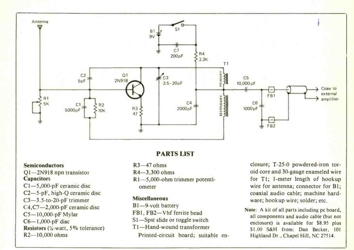
Fig. 1. Complete schematic diagram of Experimenter's Aviation Band Receiver.
