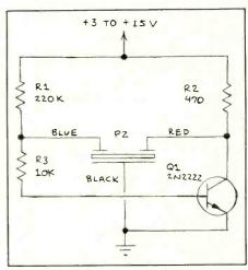
Fig. 7. Single-transistor piezoelectric buzzer element driver.
