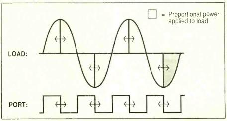
Fig. 4. Proportional power control requires precise timing.
