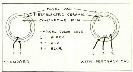
Fig. 1. Details of typical piezoelectric buzzer elements.
