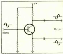
Fig. 8. A transistor phase inverter is one possible replacement for the in terstage (input) transformer needed for the opposite-polarity driving signals for the two halves of the pushpull amplifier circuit.
