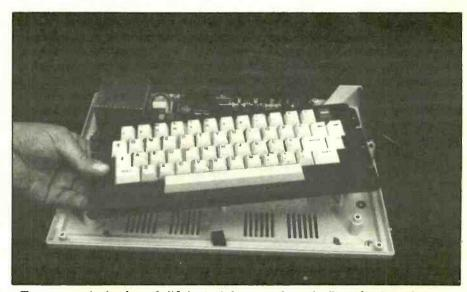
To remove the keyboard, lift it straight up and gently flip it back to the rear.
