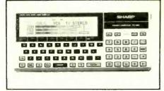
Featured are: 16K of RAM (expandable to 80K); a 4-line by 26-character LCD display; the fiber-optic interface; an analog input; an RS-232C serial interface; separate alphabetic keyboard and numeric keypad; a 60-pin I/O bus; and BASIC interpreter in ROM. Options include the microfloppy drive with 128K capacity; a 4-color pen plotter/cassette interface and a 32K RAM module. The computer measures 8 "L × 3.5 "W and weighs less than 1 lb. \$345.
