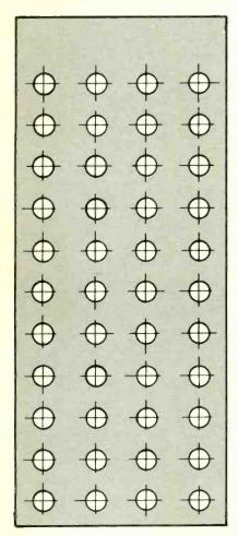
Fig. 5. Actual-size alignment template for LED installation.
